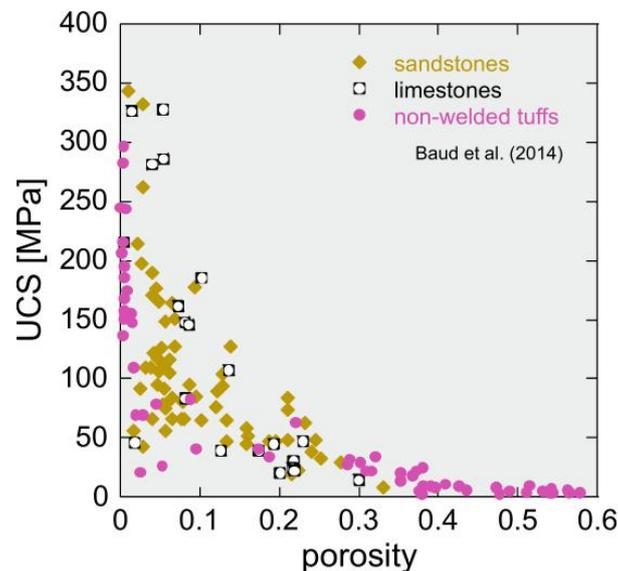
**Figure 1.9** Compilations of published data for the evolution of uniaxial compressive strength (UCS) with porosity (after Baud et al., 2014). Data points are results of deformation laboratory experiments on samples of sandstones (yellow), limestones (black) and non-welded tuffs (pink).
