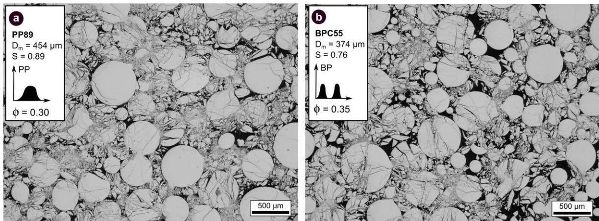
**Figure 5.4** Representative backscattered scanning electron microscope images showing the microstructure of synthetic samples deformed under hydrostatic loading up to an effective stress beyond  $P^*$  for (a) a polydisperse grain size distribution and porosity of 0.30 and (b) a bidisperse distribution and a porosity of 0.35. Extensive grain crushing is observed for both types of distributions. Black: porosity, grey: glass.
