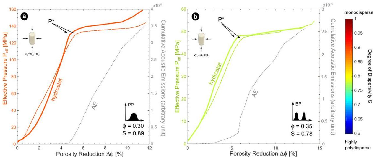
**Figure 5.3** Mechanical data (solid lines) and acoustic emission (AE) energy (dashed grey lines) for the hydrostatic compression of (a) polydisperse synthetic samples and (b) bidisperse
