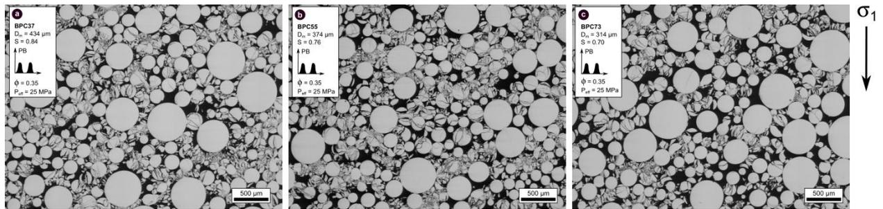
**Figure 5.10** Representative backscattered scanning electron microscope images of the microstructure of bidisperse synthetic samples deformed under triaxial compression up to stresses beyond  $C^*$ . From (a) to (c), the ratio of small grains to big grains decreases. For all distributions, delocalised compaction, where small grains are crushed while bigger grains remain intact, is observed. Black: porosity, grey: glass.
