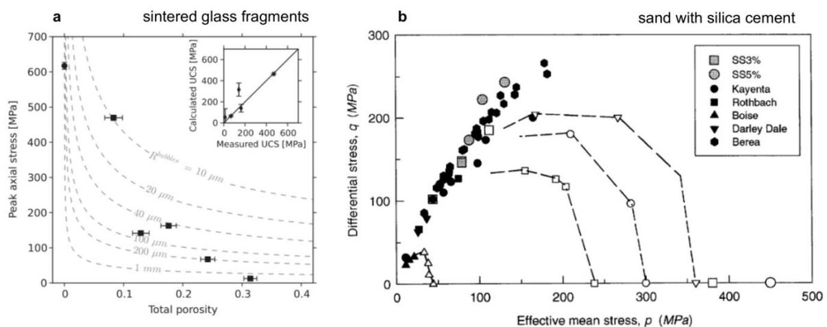
**Figure 1.13** Mechanical behaviour of synthetic rocks made of (a) sintered glass fragments (Vasseur et al., 2013) and (b) sand with variable proportion of silica cement (SS3% contains 3%vol of cement and SS5%, 5%vol) (David et al., 1998).
