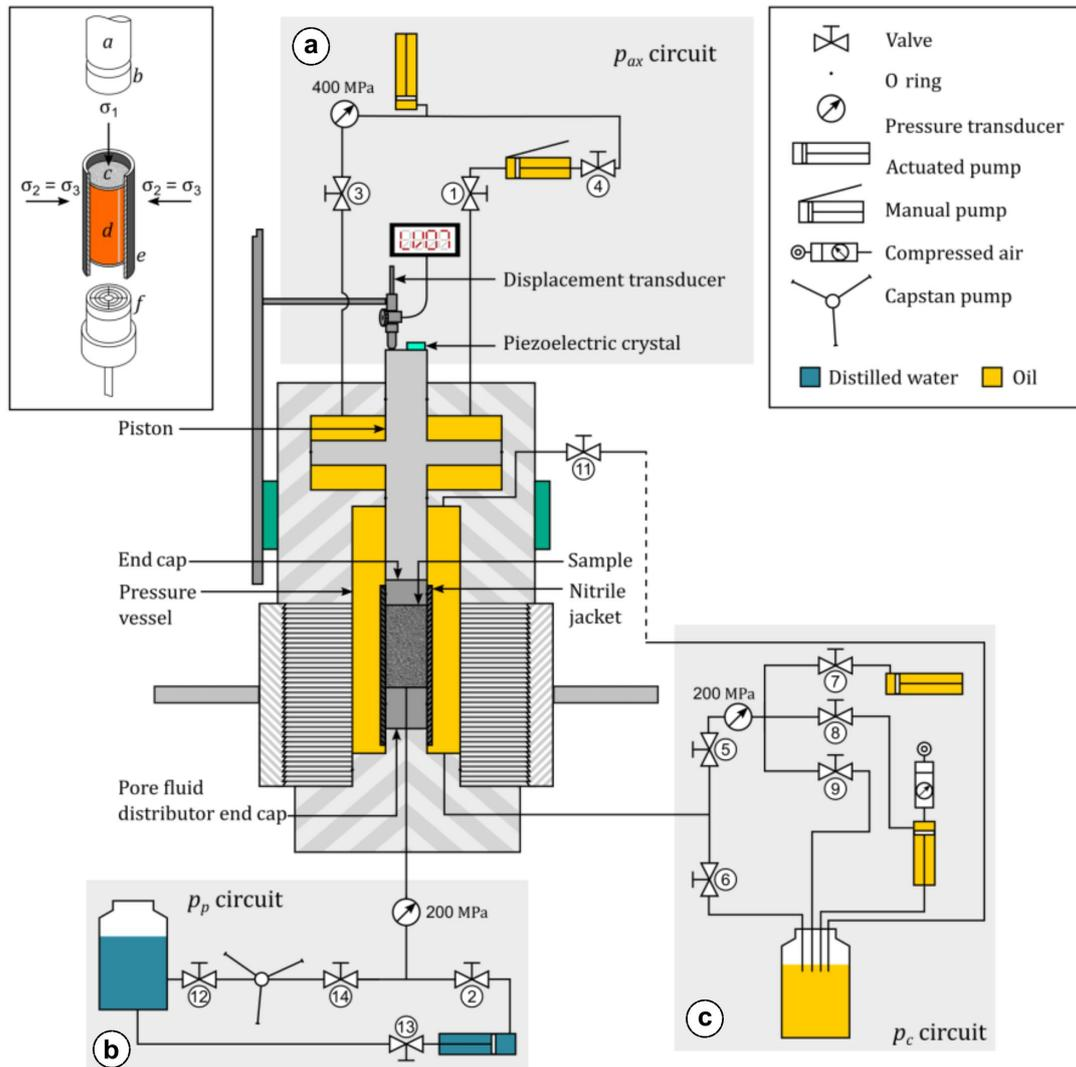
**Figure 3.11** Schematics of triaxial press used in this work (not to scale) (Farquharson et al., 2017). The apparatus allows for independently controlling the (a) axial pressure, the (b) pore pressure, i.e., the pressure of the fluid (water) in the pore space of the sample deformed, and the (c) confining pressure, i.e., the pressure in the fluid (kerosene) surrounding the sample.
