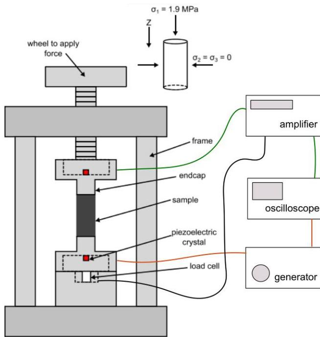
**Figure 3.2** Schematics of the experimental device for wave velocity measurements (adapted from [Heap et al., 2014](#)). Frequencies of 700 and 300 kHz were used to measure P- and S-waves velocity, respectively.
