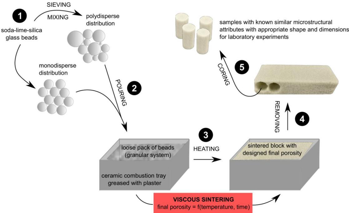
**Figure 2.5** Schematic representation of the experimental procedure for the preparation of sintered samples: the case of sintered blocks (not to scale). A detailed description of each step is provided in the main text.
