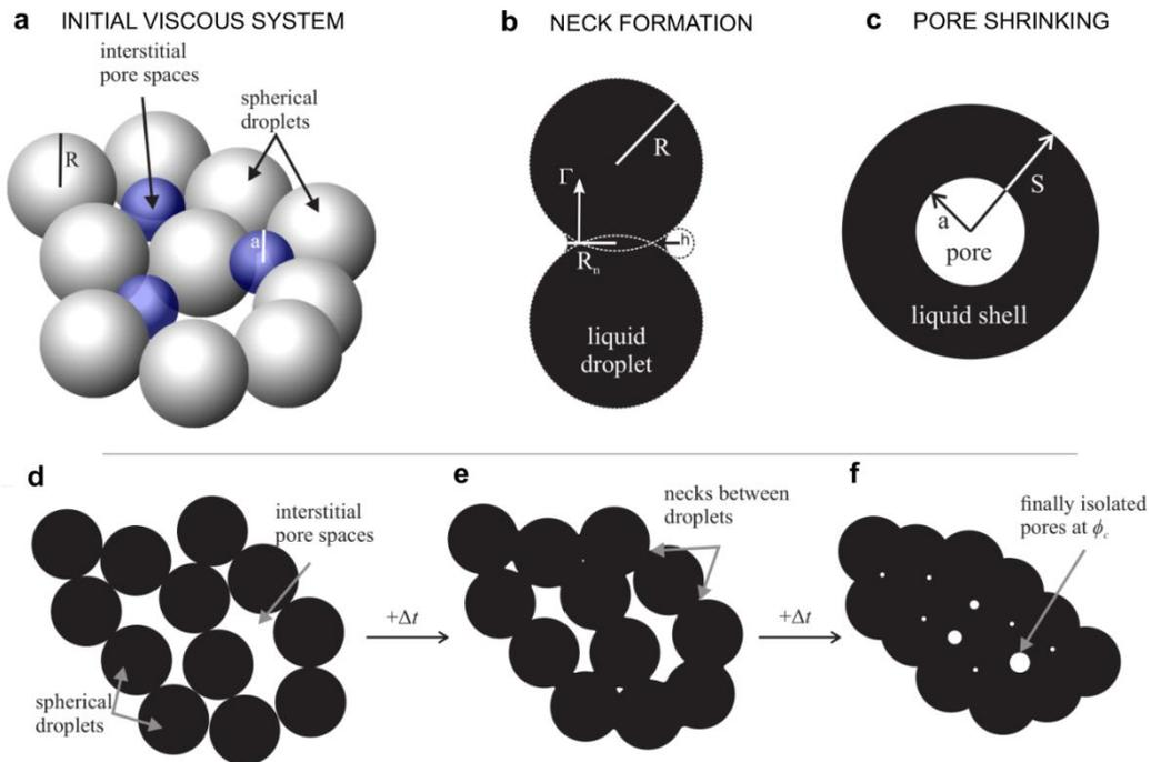
**Figure 2.1** Schematic representation of the coalescence of a many-droplet viscous system with time. (a, d) Initially, the system is composed of spherical droplets (grey) with initial radius  $R$  and interstitial spherical pores (blue) with initial radius  $a$ . The system undergoes
