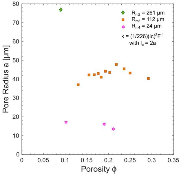
**Figure 3.10** Porosity dependency of the pore radius of monodisperse synthetic samples with mean grain radius of 261 (green diamond), 112 (orange squares) and 24 (pink stars)  $\mu\text{m}$ . Values were derived using the permeability model of [Katz and Thompson \(1986\)](#) (equation 3.14).
