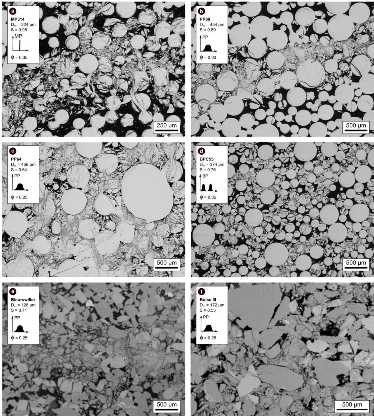
**Figure 5.13** Backscattered scanning electron microscope images of the microstructure of sintered glass bead samples with (a) a monodisperse grain size distribution, (b)(c) a polydisperse distribution and (d) a bidisperse distribution compared to that found in Bleurswiller and Boise sandstones (Cheung et al., 2012), after triaxial testing in the regime of
