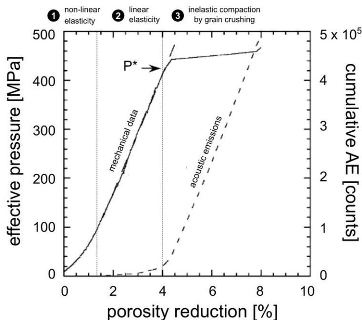
**Figure 1.3** Example of mechanical data for the hydrostatic loading of a porous crustal rock. Data were obtained during a hydrostatic experiment on water-saturated Bentheim sandstone. The effective pressure is represented against the porosity reduction (solid line) and compiled with the corresponding recording of acoustic emissions, presented in cumulative (dashed line).
