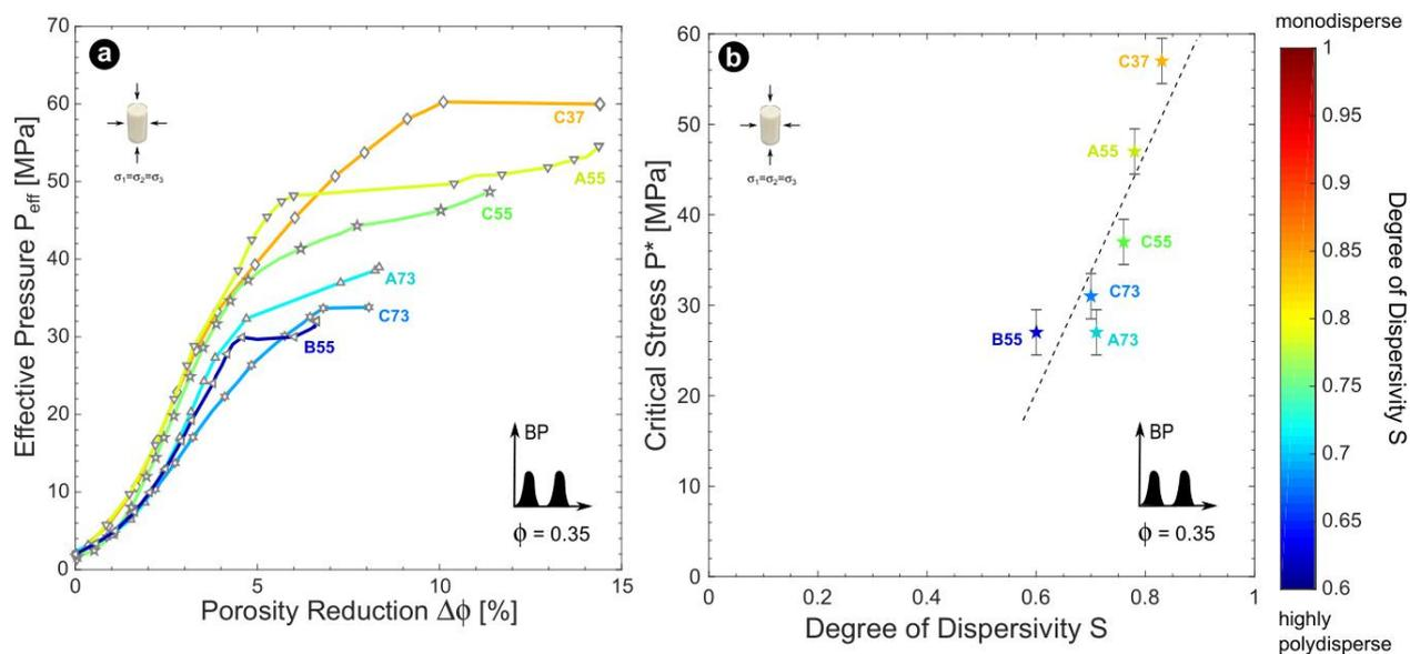
**Figure 5.5** Mechanical data for the hydrostatic compression of bidisperse synthetic samples with a porosity of 0.35. (a) The hydrostatic curves are shown as the effective pressure against
