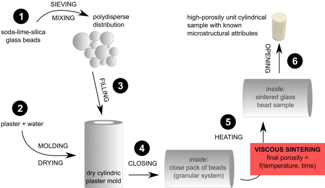
**Figure 2.7** Schematic representation of the experimental procedure for the preparation of sintered samples: the case of unit cylindrical samples (not to scale). A detailed description of each step is provided in the main text.
