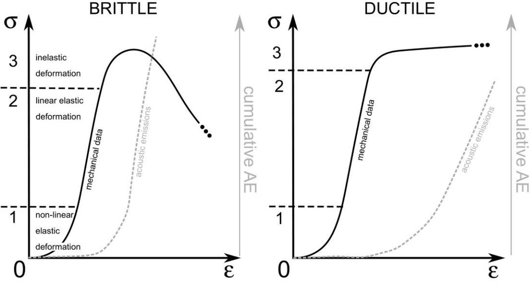
**Figure 1.1** Schematic of the typical stress-strain behaviour of porous sandstones deformed at room temperature in the brittle (left) and ductile (right) regime. The mechanical data (solid black) are plotted as  $\sigma$  the differential stress against  $\epsilon$  the axial strain and the corresponding acoustic emissions (AEs) are presented as the cumulative AEs against axial strain (dashed
