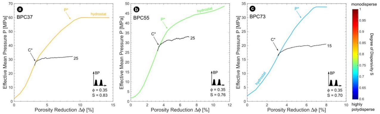
**Figure 5.8** Hydrostatic (coloured lines) and triaxial mechanical data (black lines) presented as the effective mean stress against the porosity reduction for bidisperse (BP) synthetic samples with a grain size distribution (a) C37, (b) C55 and (c) C73.
