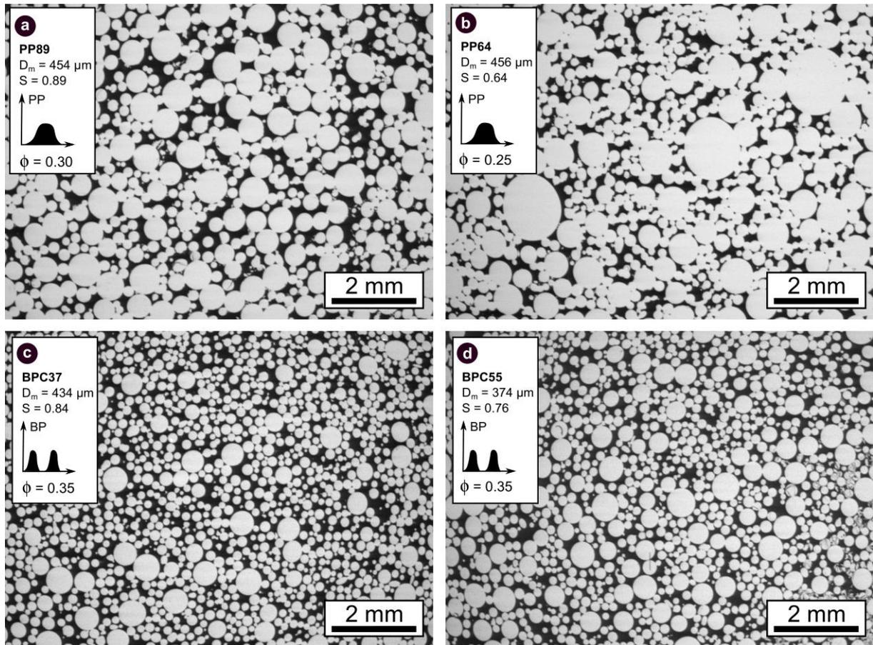
**Figure 5.2** Intact microstructure of samples with a polydisperse grain size distribution (a) PP89 and porosity of 0.30 and (b) PP64 and porosity of 0.25 and a bidisperse grain size distribution (c) BPC37 and porosity of 0.35 and (d) BPC55 and porosity of 0.35. The degree of dispersivity  $S$  is in the range 0-1, where 1 is the monodisperse limit.
