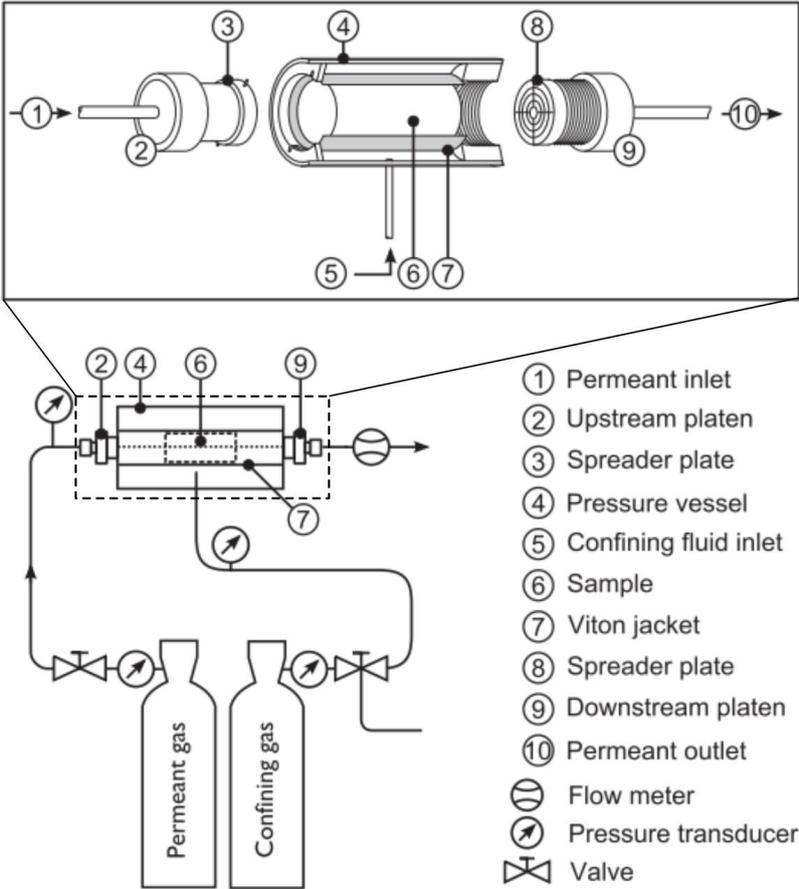
**Figure 3.7** Schematics of the benchtop steady state permeameter used in this work (not to scale) (modified from Farquharson et al., 2016). Nitrogen was used as both permeant (pore fluid) and confining gas. Using the indices (1–10) to refer to the different parts of the set-up, a detailed description of the experimental procedure for the permeability measurements is given in the main text.
