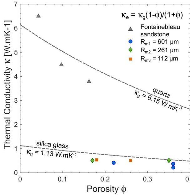
**Figure 3.5** Dry thermal conductivity as a function of porosity for the synthetic samples with mean grain radius of 601 (blue circles), 261 (green diamonds) and 112 (orange squares)  $\mu\text{m}$  and Fontainebleau sandstone samples (Zamora et al., 1993). Grey dashed lines are model predictions for the porosity-thermal conductivity curves computed using the Rayleigh–Maxwell equation (equation 3.5) for quartz and the soda-lime silica glass of the synthetic samples.
