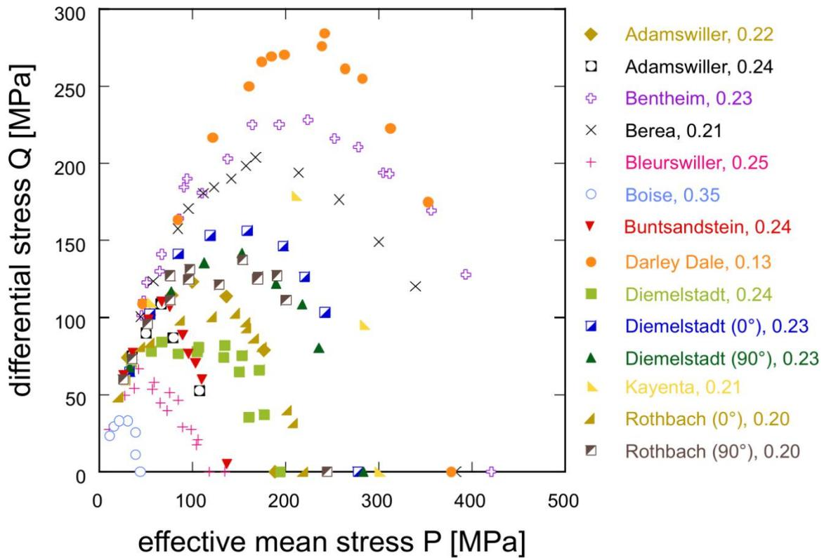
**Figure 1.10** Compilation of failure envelopes for porous sandstones with porosity ranging from 0.13 to 0.35 (data for Muschelkalk from a personal communication, [Carbillet \(2018\)](#); other data from [Wong & Baud, 2012](#)).
