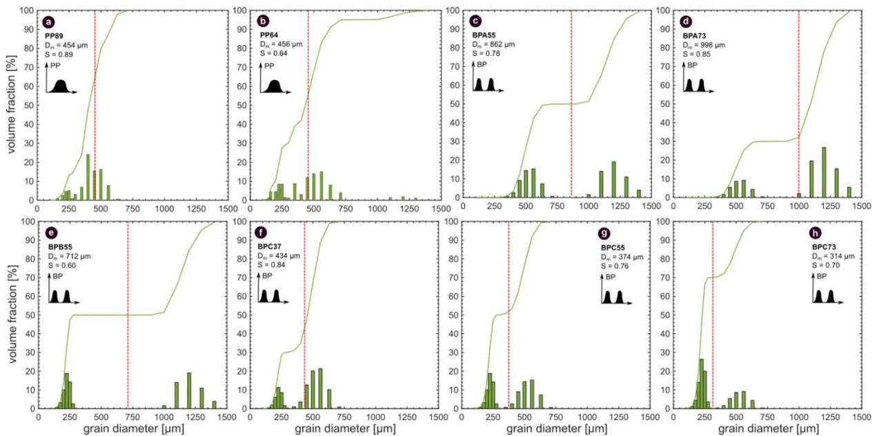
**Figure 5.1** Grain size distributions of the synthetic samples. The distributions are presented in terms of volume fraction against grain diameter [ $\mu\text{m}$ ], with the cumulative volume fraction (green solid lines) and the first moment of the distribution, i.e., the mean grain diameter (dashed red lines). Distributions (a) P89 and (b) P64 are polydisperse distributions, and
