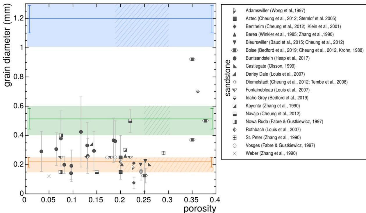
**Figure 4.11** Compilation of porosity and grain diameter for laboratory sandstones. All data are from the literature, references are given in the legend. Coloured areas correspond to the range of porosity-grain diameter accessible by sintering glass beads. The dashed areas correspond to the range specifically investigated in this study. The error bars give the standard deviation of the grain diameter distribution, when it has been reported.
