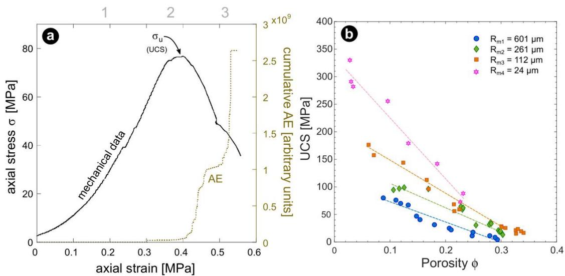
**Figure 3.12** (a) Representative mechanical data for the axial stress change with axial strain during uniaxial deformation of a synthetic sample with a porosity of 0.11 and mean grain radius of  $601 \mu\text{m}$ . The peak stress at brittle failure is marked  $\sigma_u$ . The cumulative acoustic
