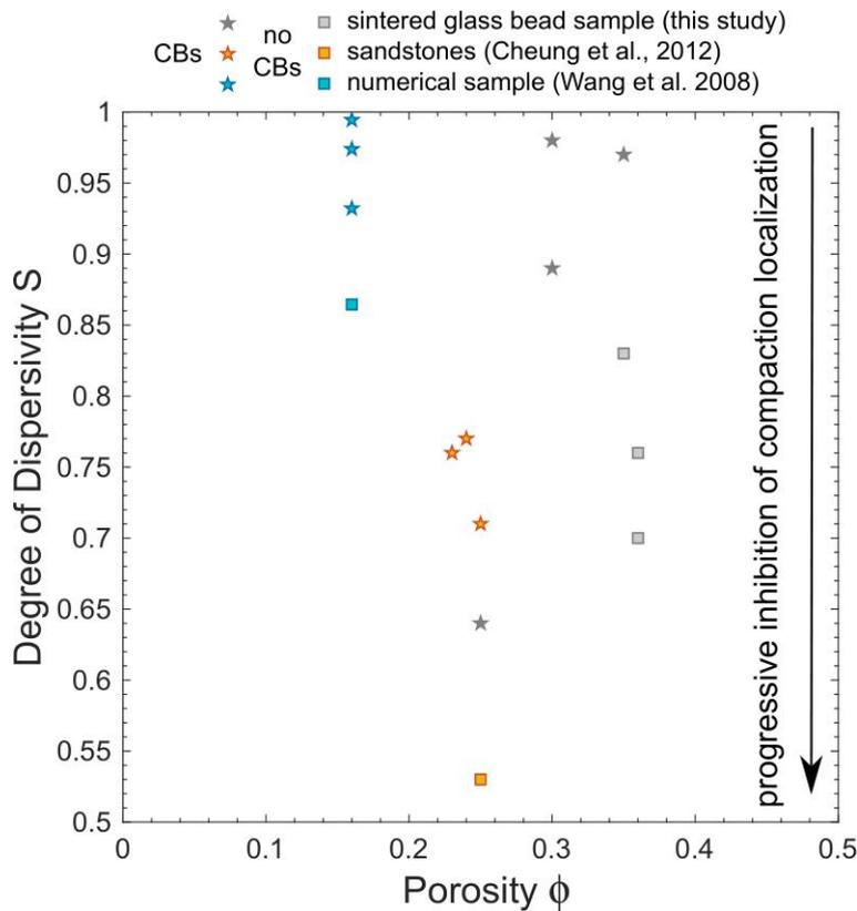
**Figure 5.14** The influence of the degree of dispersivity and the porosity on the propensity for compaction localisation. Results for sintered glass bead samples are compiled with that reported by Wang et al. (2008) for numerical samples and that for natural sandstones by Cheung et al. (2012).
