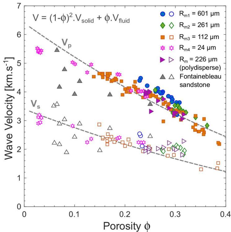
**Figure 3.3** Porosity dependency of P- (solid symbols) and S-wave (open symbols) velocity in monodisperse synthetic samples with a mean grain radius of 601 (blue circles), 261 (green diamonds), 112 (orange squares) and 24 (pink stars), polydisperse synthetic samples (degree of polydispersivity  $S = 0.89$ ) with a mean grain radius of 226  $\mu\text{m}$  (purple right triangles) and
