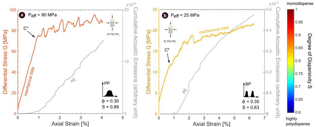
**Figure 5.6** Mechanical data (solid lines) and cumulative acoustic emission energy (dashed grey lines) for triaxial tests performed on (a) a polydisperse (PP) synthetic sample and (b) a bidisperse (BP) synthetic sample in the ductile regime.
