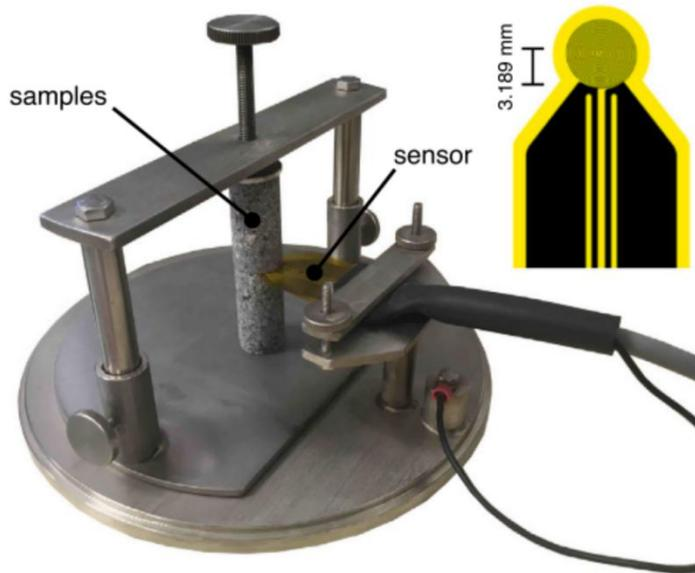
**Figure 3.4** Experimental setup for thermal conductivity measurements. The sensor used, made of 10  $\mu\text{m}$ -thick nickel foil spirals encased and insulated with 30  $\mu\text{m}$ -thick kapton, is placed between two samples with similar microstructural attributes. The assembly is tightened using the screw on top on the set-up (Heap et al., 2022).
