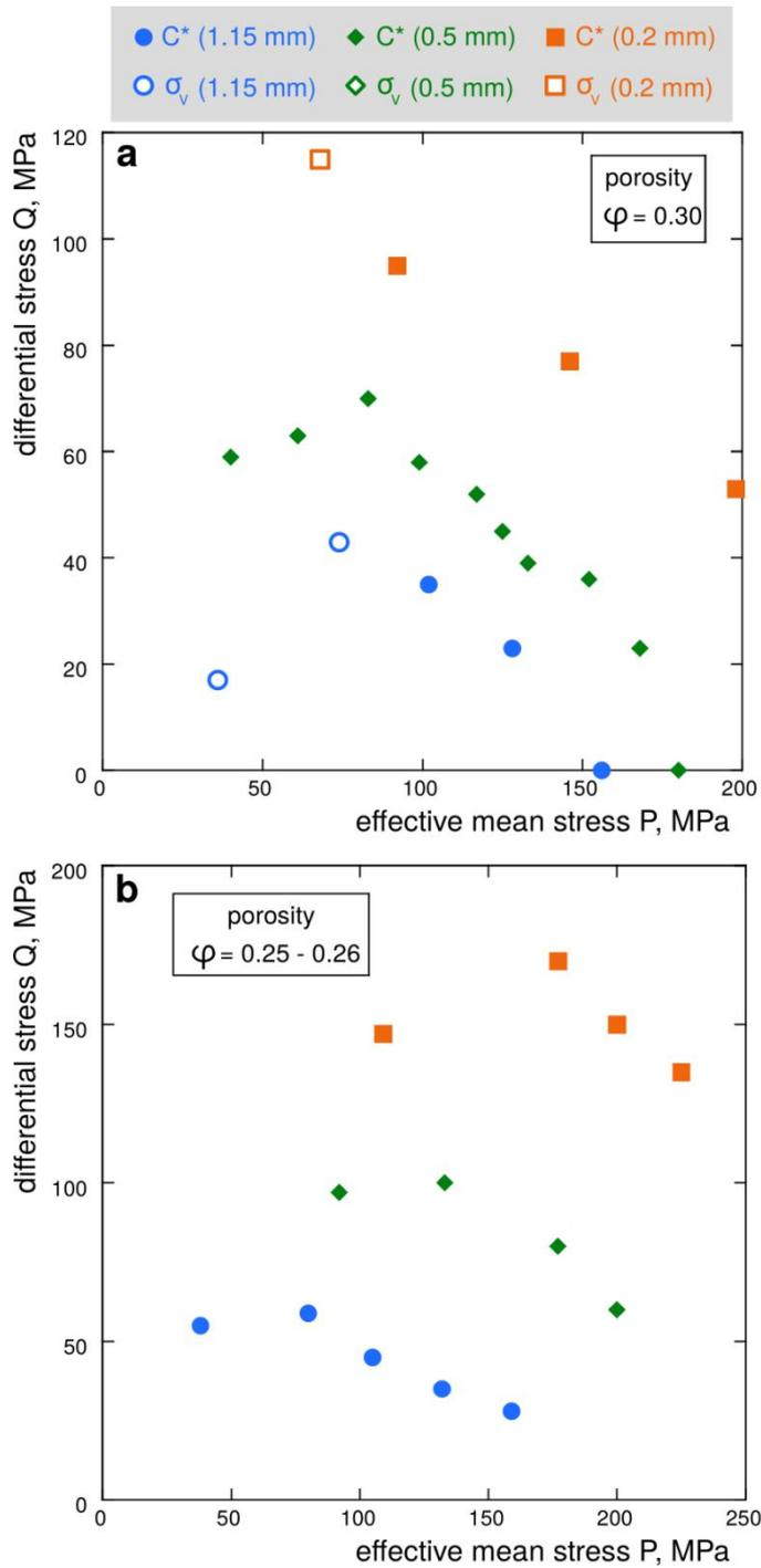
**Figure 4.7** Compilations of failure envelopes for synthetic samples with a porosity of (a) 0.30 and (b) 0.25. Mean grain diameter of the synthetic samples is indicated in the legend. Failure envelopes are mapped out by critical stresses  $\sigma_v$  (brittle triaxial test),  $C^*$  (ductile triaxial test) and  $P^*$  (hydrostatic test). Open symbols correspond to peak stress values and solid symbols to  $C^*$  values.  $P^*$  (also a solid symbol) anchors the envelope to the x-axis.
