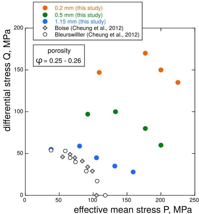
**Figure 4.13** Influence of grain diameter on the compactive yield strength. Compactive yield envelopes for synthetic samples with a porosity of 0.25 and a mean grain diameter of 0.2 mm (orange), 0.5 mm (green) and 1.15 mm (blue) are compiled with yield envelopes for Boise (open cross) and Bleurswiller (open circle) sandstones (data from Cheung et al., 2012).
