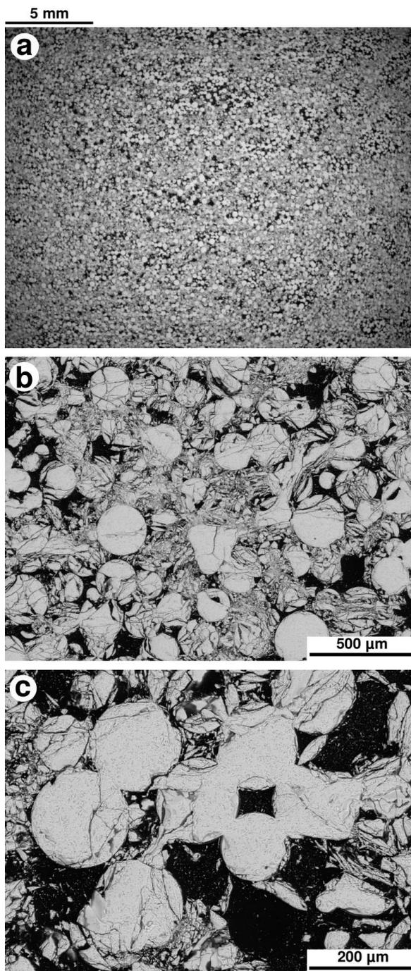
**Figure 4.8.** Representative scanning electron micrograph of the (a) microstructure of a synthetic sample deformed under hydrostatic loading up to an effective stress beyond  $P^*$ . (b)(c) Zooms in showing extensive grain crushing. Black: porosity, grey: glass.
