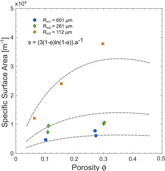
**Figure 3.1** Specific surface area of synthetic samples with porosity in the range 0.6–0.30 and mean grain radius of 112 (orange squares), 261 (green diamonds) and 601 (blue circles)  $\mu\text{m}$ . The experimental data are compiled with modelled curves computed using the method described by Wadsworth et al. (2016) (equation 3.3) (grey dashed line).
