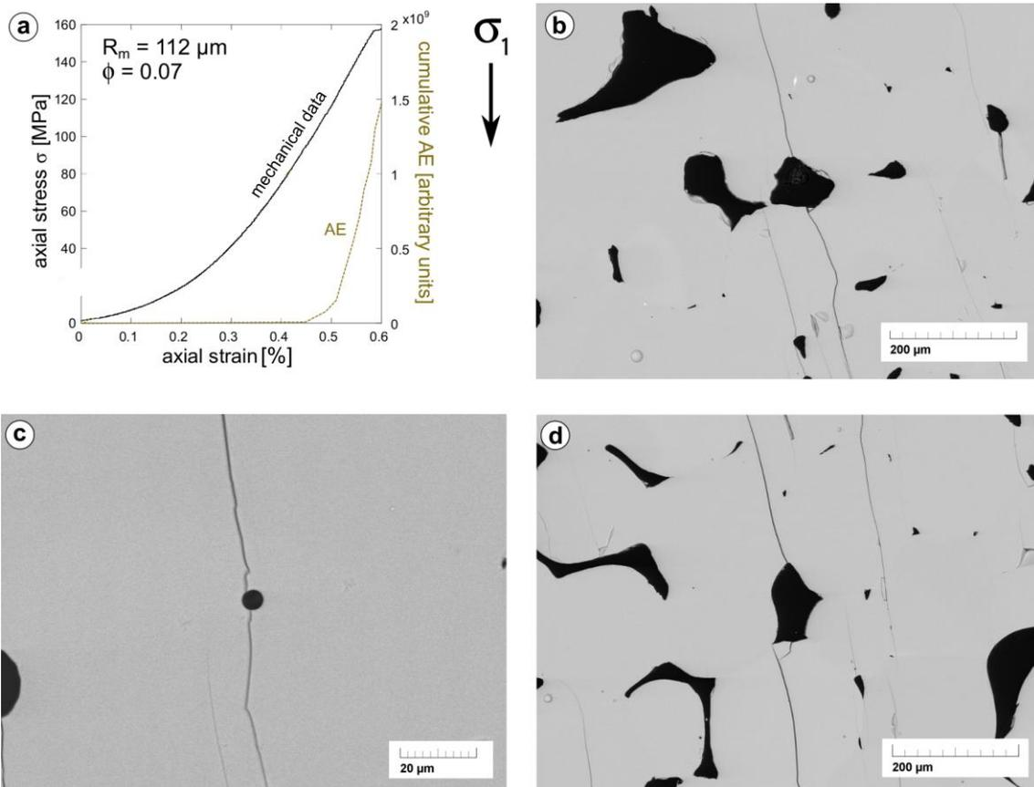
**Figure 3.14** (a) Mechanical data and (b)(c)(d) scanning electron micrographs for a synthetic sample with a porosity of 0.07 and mean grain size of 112  $\mu\text{m}$  deformed under uniaxial compression up to an axial strain of approximately 0.6%. The microstructure shows pore-emanated microcracks growing from the poles of pores.
