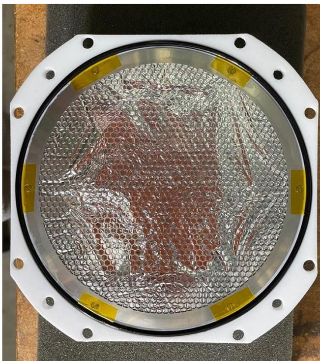
**Figure 19.** Aluminized Mylar window dismantled from the sRTC.
