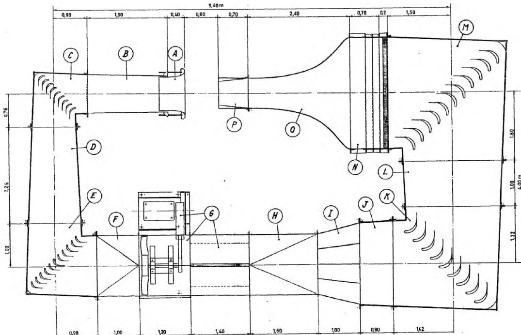
Figure 1.1 – ISL subsonic wind tunnel layout [Jaeggy, 1982]
