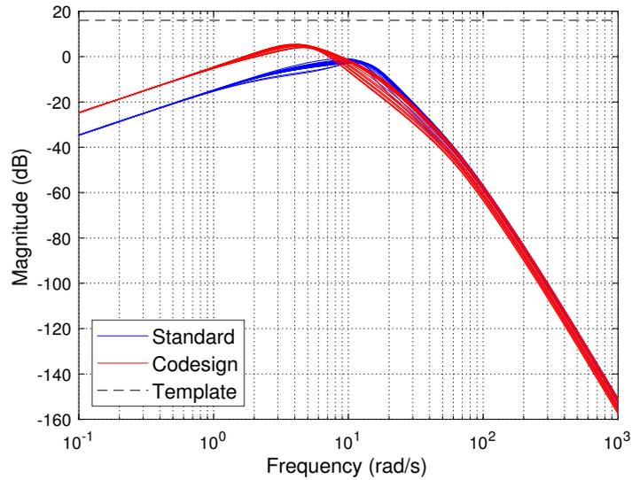
Figure 3.31 – Actuator to output transfer  $GS$  comparison
