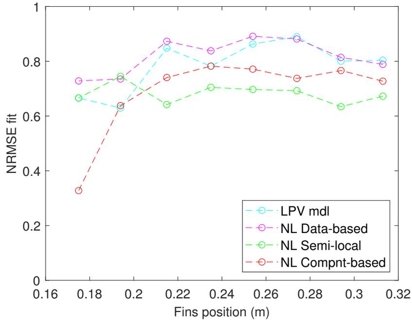
Figure 2.28 – Open-loop response fit for different fins positions
