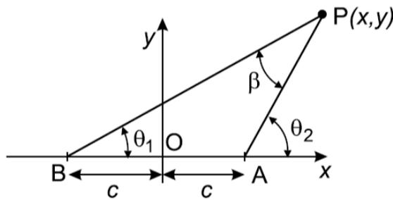
Figure 2.10 – Geometry of a source upstream of a sink (reproduced from [HC03])
