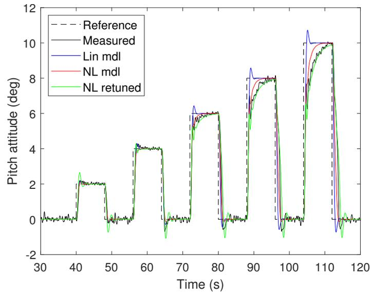
Figure 3.54 – Pitch attitude tracking of the dual-loop co-design
