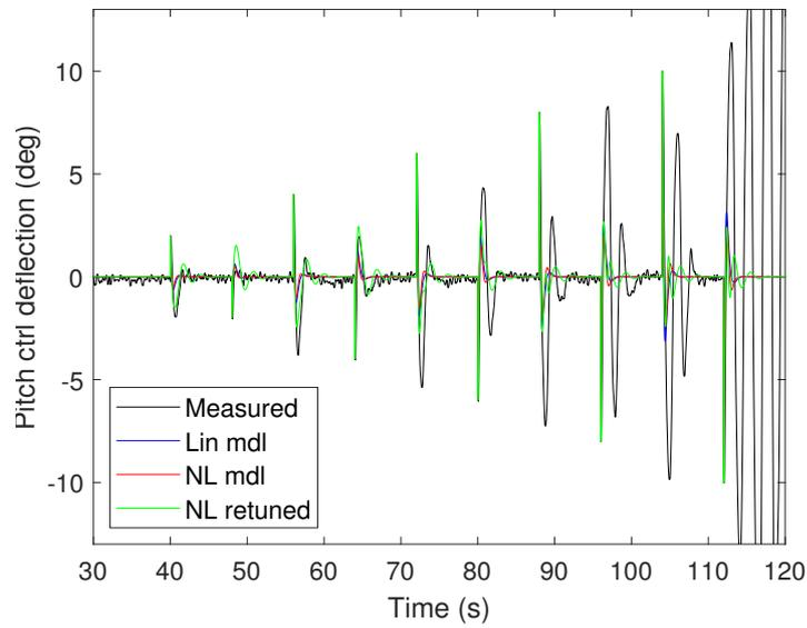
Figure 3.52 – Control action during disturbance rejection experiment
