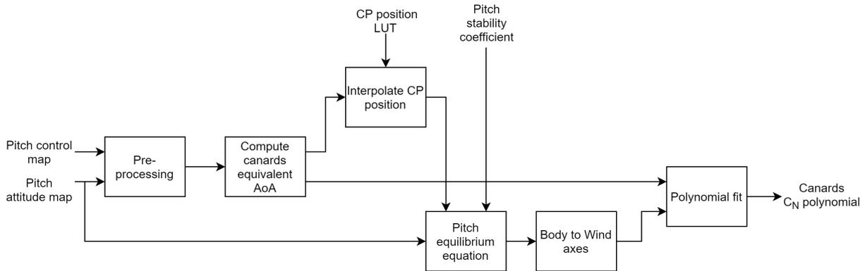
Figure 2.16 – FAST diagram of canard lift reconstruction routine
