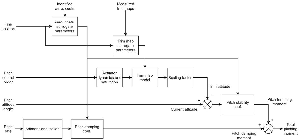
Figure 2.22 – FAST diagram of data-based model
