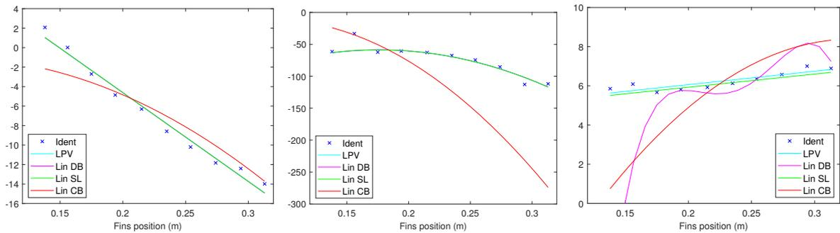
Figure 2.32 – Comparison of  $Cm_\alpha$  (left),  $Cm_q$  (center) and  $Cm_{\delta_m}$  (right) from system identification and models linearization
