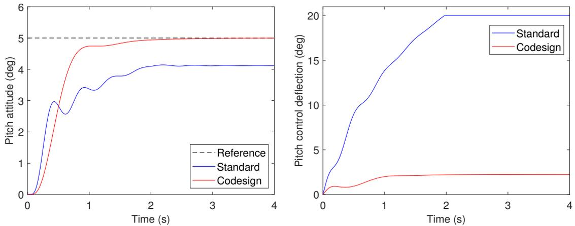
Figure 3.32 – Reference tracking of standard and optimized airframes
