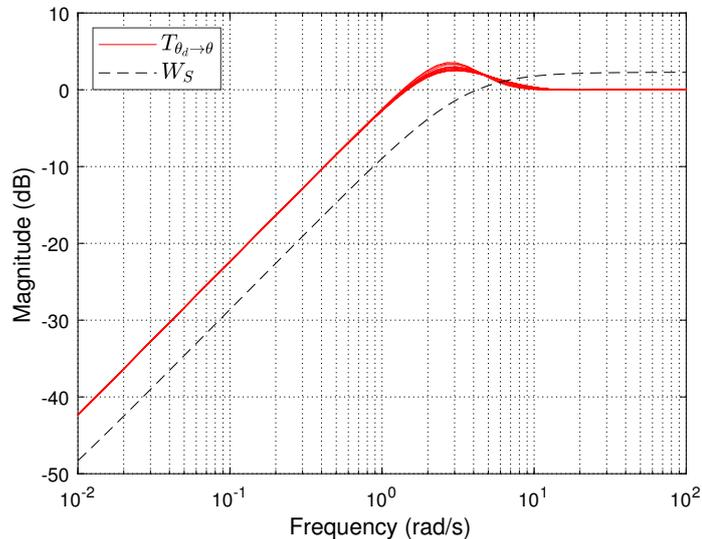
Figure 3.34 – Disturbance rejection transfer  $S$  and associated template
