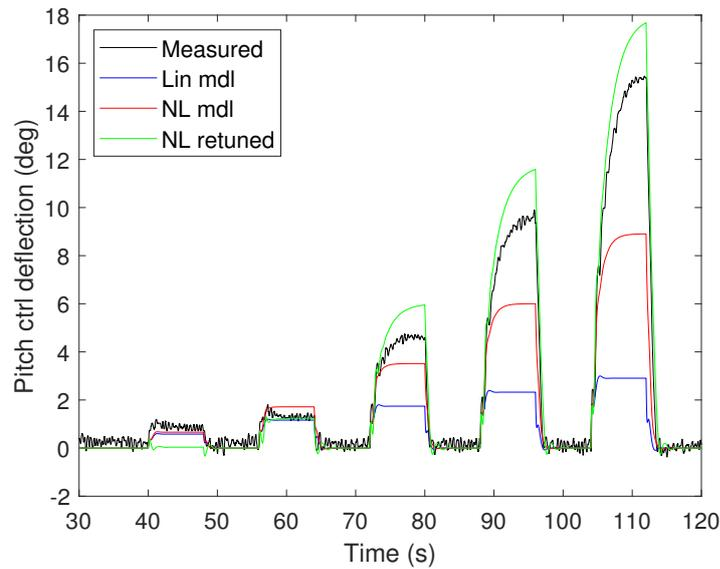
Figure 3.55 – Control action during reference tracking experiment
