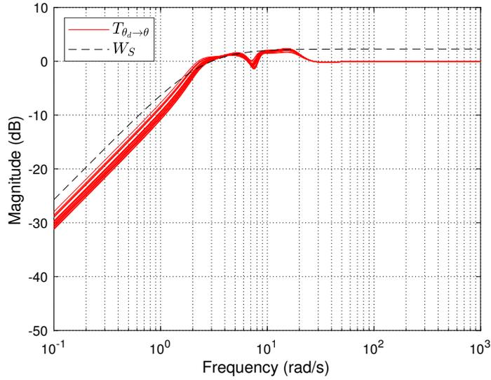
Figure 3.14 – Disturbance rejection transfer  $S$  and associated template
