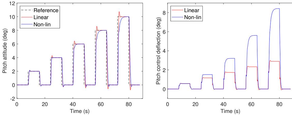
Figure 3.26 – Step tracking of the dual-loop controller for increasing amplitudes
