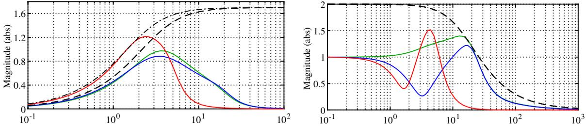
Figure 1.17 – Disturbance rejection transfers  $\mathbf{T}_{\mathbf{d} \rightarrow \mathbf{e}}$  (left) and  $\mathbf{T}_{\mathbf{d} \rightarrow \mathbf{u}_c}$  (right) *The roll (green), pitch (blue) and yaw (red) channels are compared to the templates (dashed for roll and pitch, dash-dotted for yaw); frequency is in rad/s*
