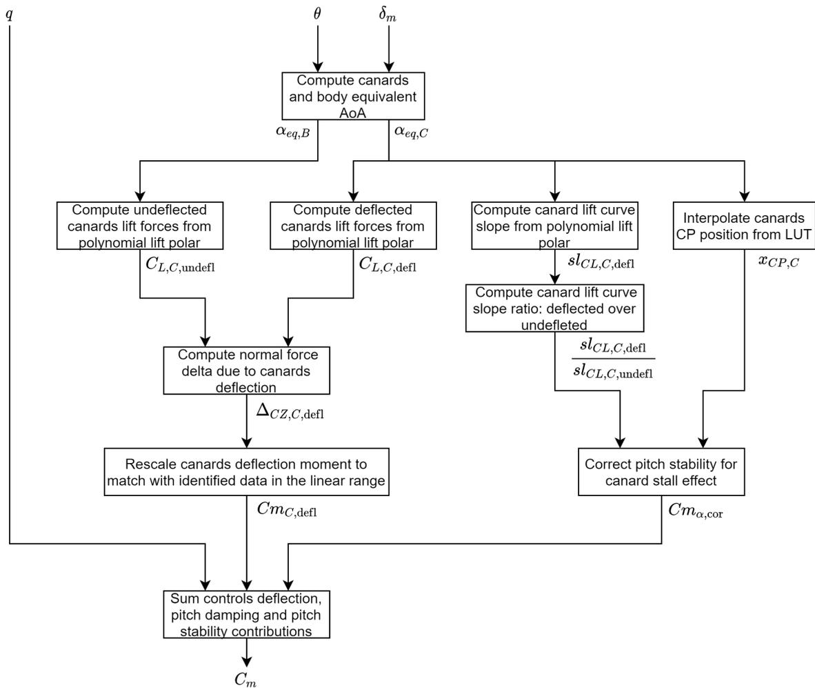
Figure 62 – Flowchart of the semi-local model
