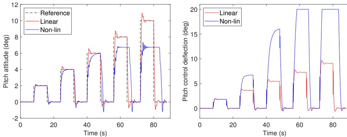
Figure 3.18 – Step tracking of the state-space controller for increasing amplitudes
