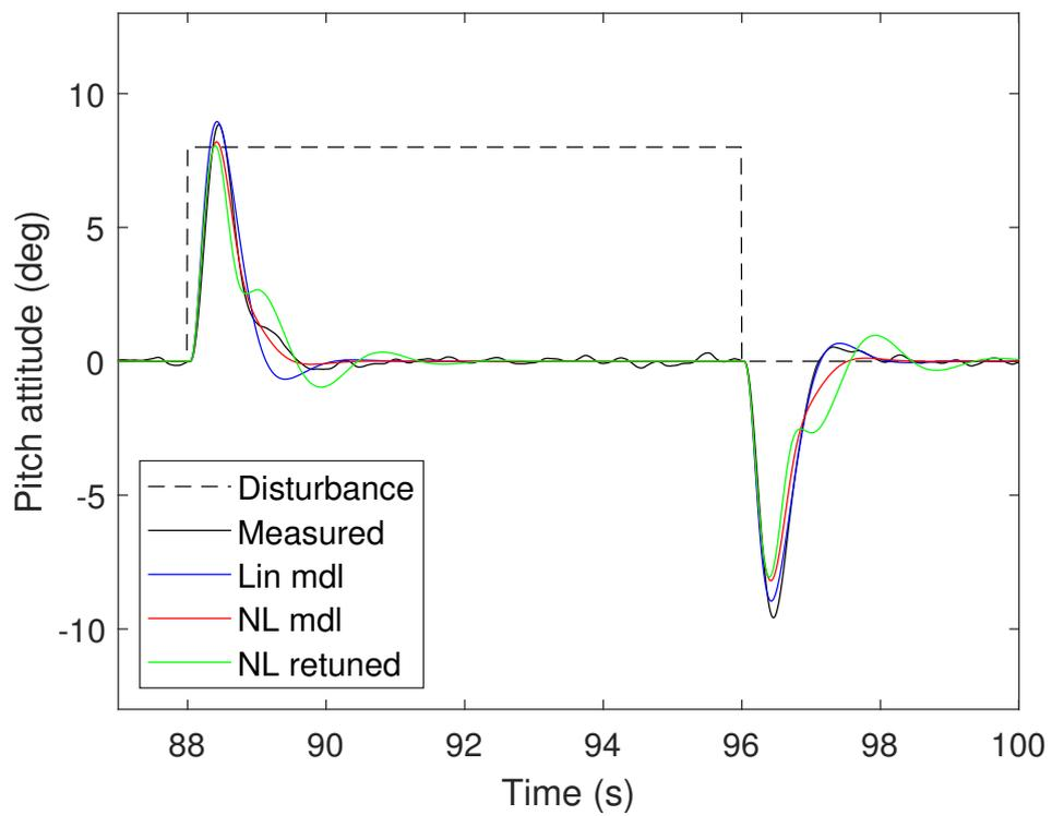
Figure 3.59 – Zoom on the 8° disturbance step rejection
