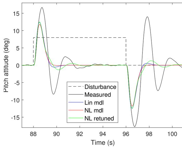
Figure 3.53 – Zoom on the 8° disturbance step rejection
