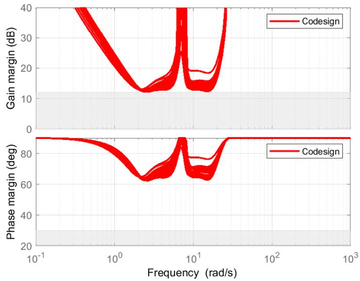
Figure 3.17 – Stability margin at the output  $\theta$
