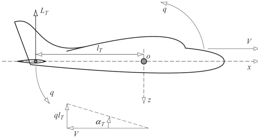
Figure 2.6 – Tailplane incidence due to pitch rate [Coo12]
