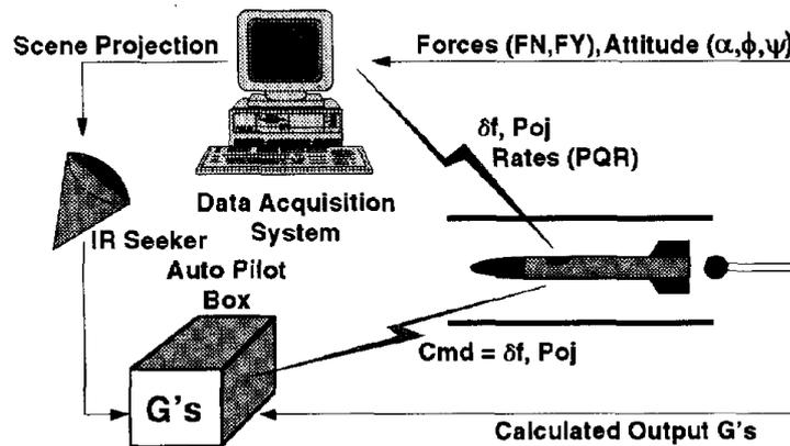
Figure 18 – The Virtual Flight Testing concept [RM95]
