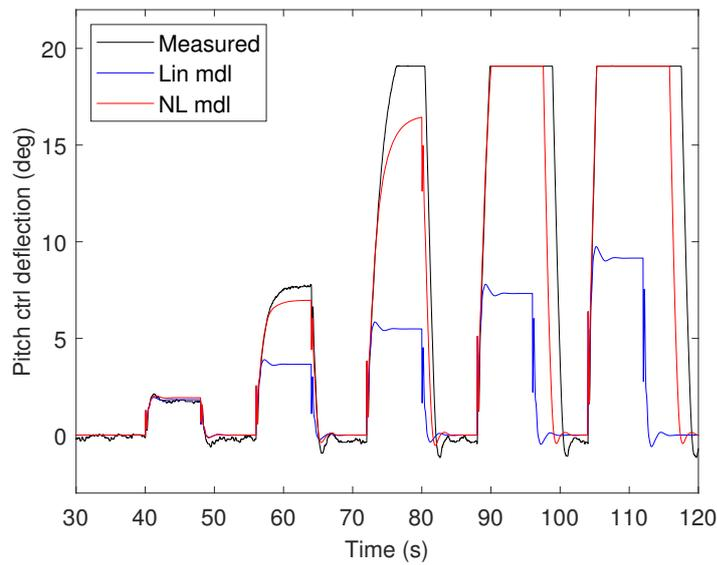
Figure 3.44 – Control action during reference tracking experiment
