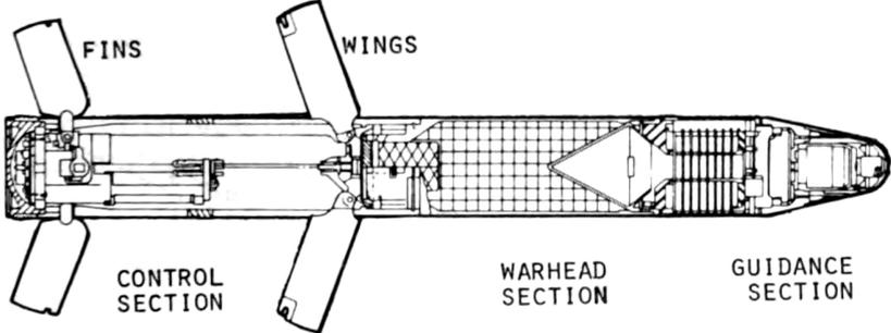
Figure 10 – Layout of the M712 Copperhead 155 mm guided shell
