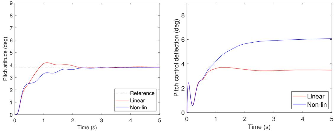
Figure 3.19 – Projectile step response at maximum control AoA
