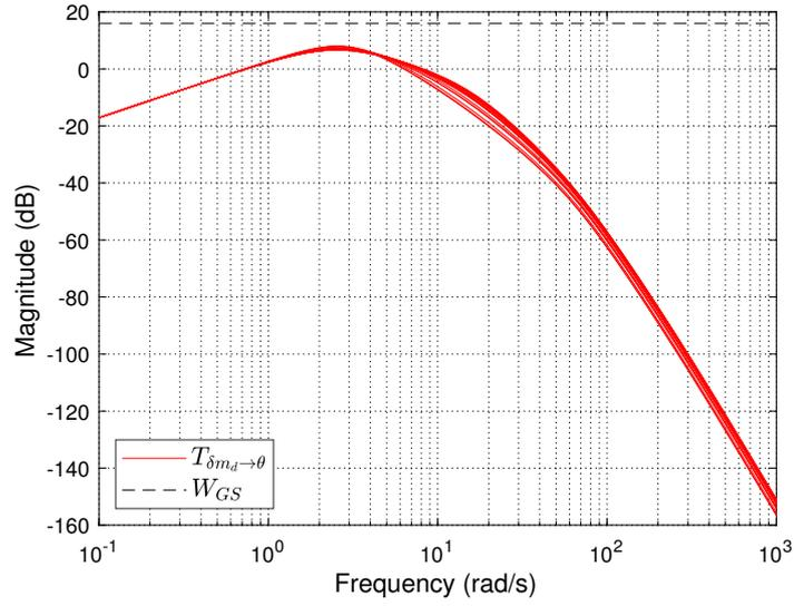
Figure 3.36 – Robustness transfer  $GS$  and associated template
