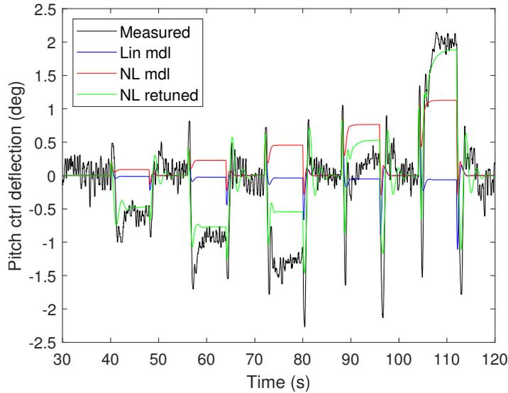
Figure 3.49 – Control action during reference tracking experiment
