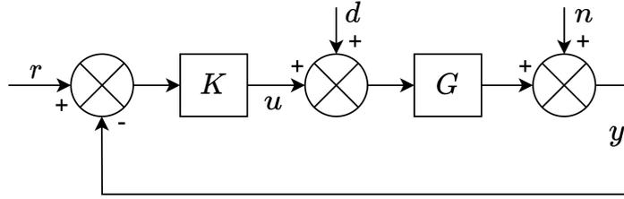
Figure 2.2 – Example of a closed-loop system
