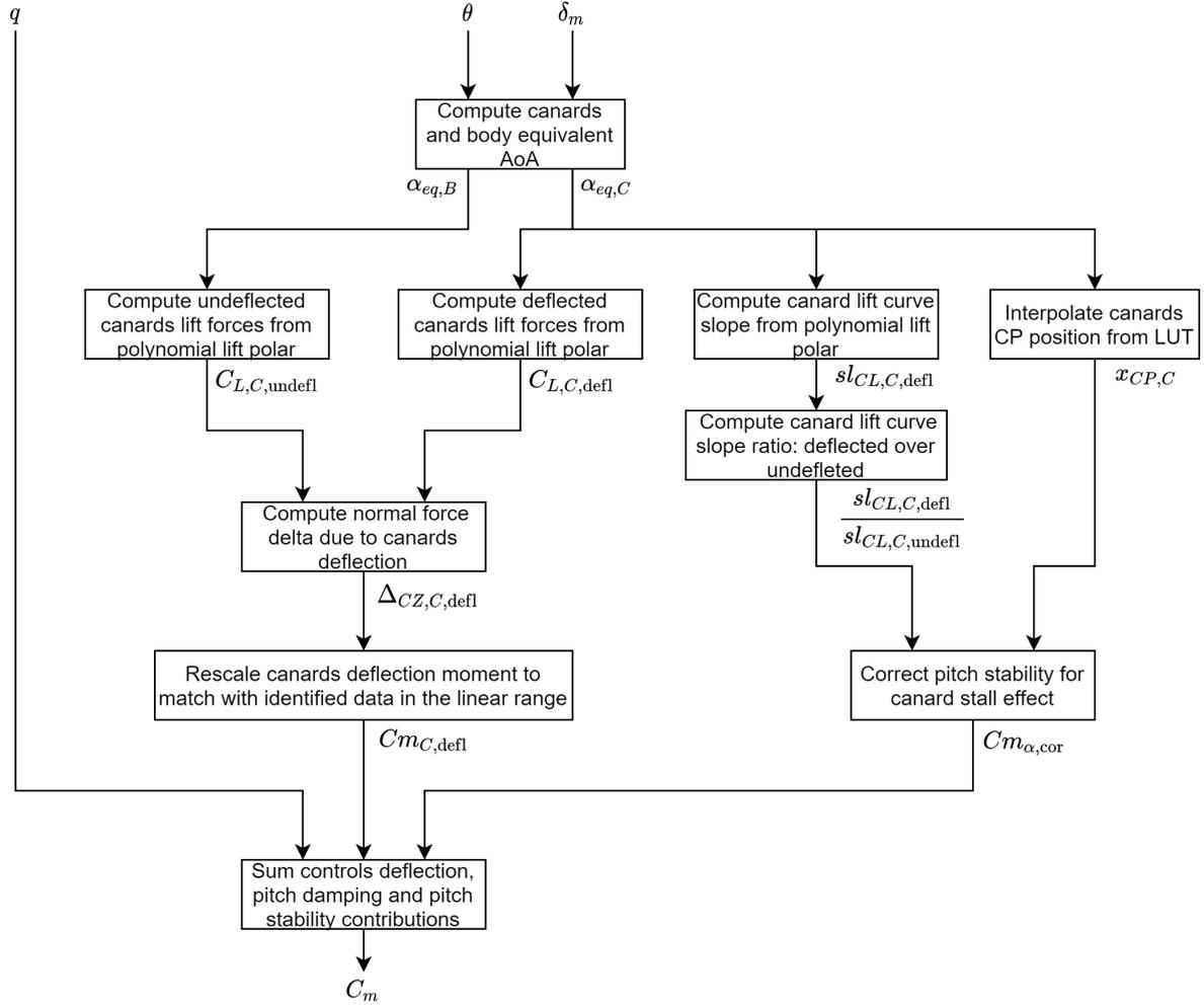
Figure 3.8 – Flowchart of the semi-local model
