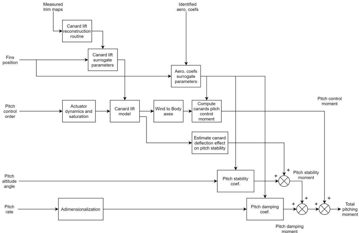
Figure 2.21 – FAST diagram of semi-local model
