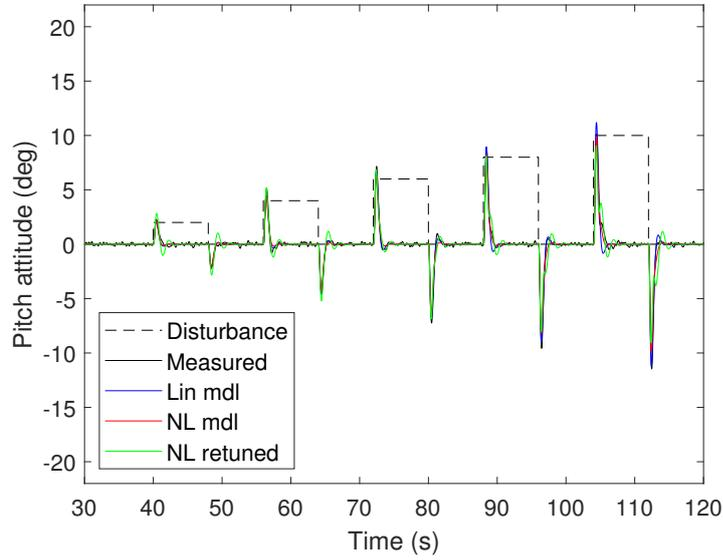
Figure 3.57 – Disturbance rejection of the dual-loop co-design
