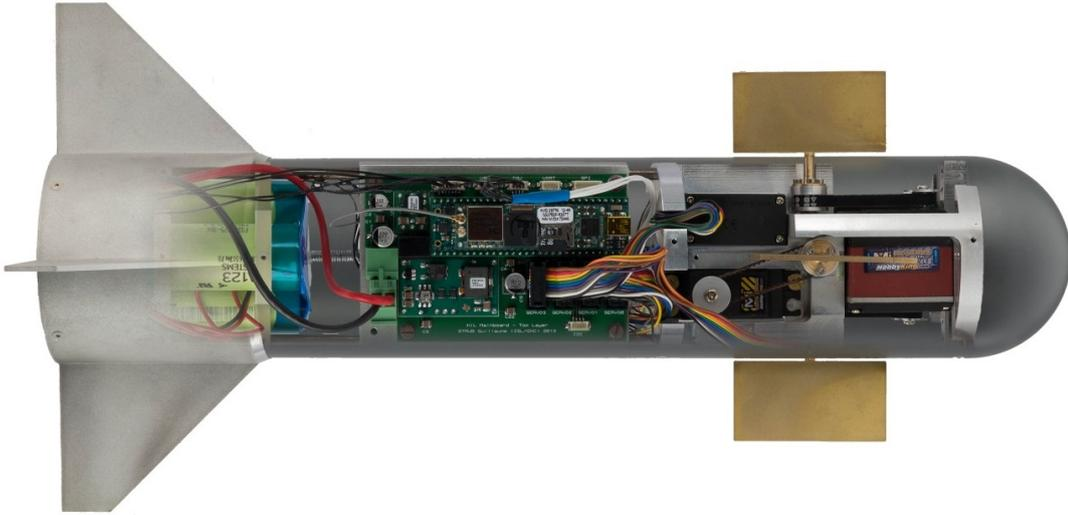
Figure 1.8 – Actuators and avionics of the HIL mock-up [Str16]
