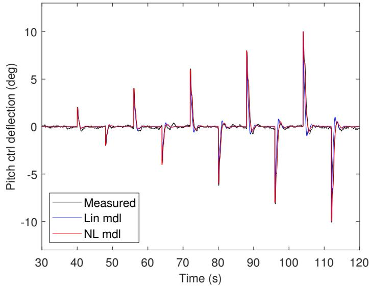
Figure 3.46 – Control action during disturbance rejection experiment
