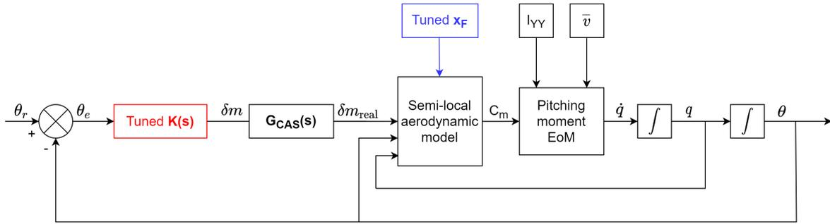
Figure 3.7 – Non-linear pitch dynamics simulator
