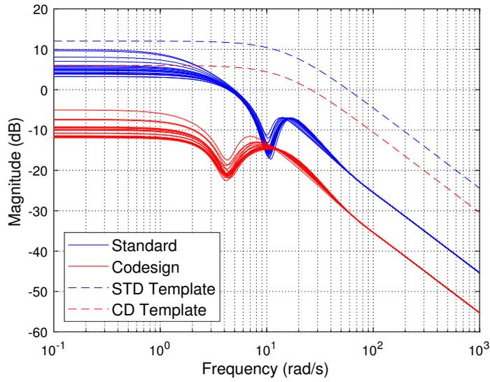
Figure 3.30 – Reference to actuator transfers  $KS$  comparison
