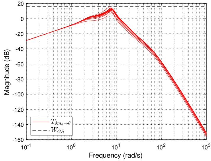
Figure 3.16 – Robustness transfer  $GS$  and associated template
