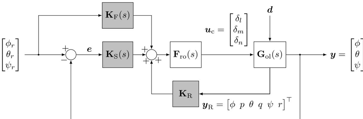
Figure 1.14 – Controller structure
