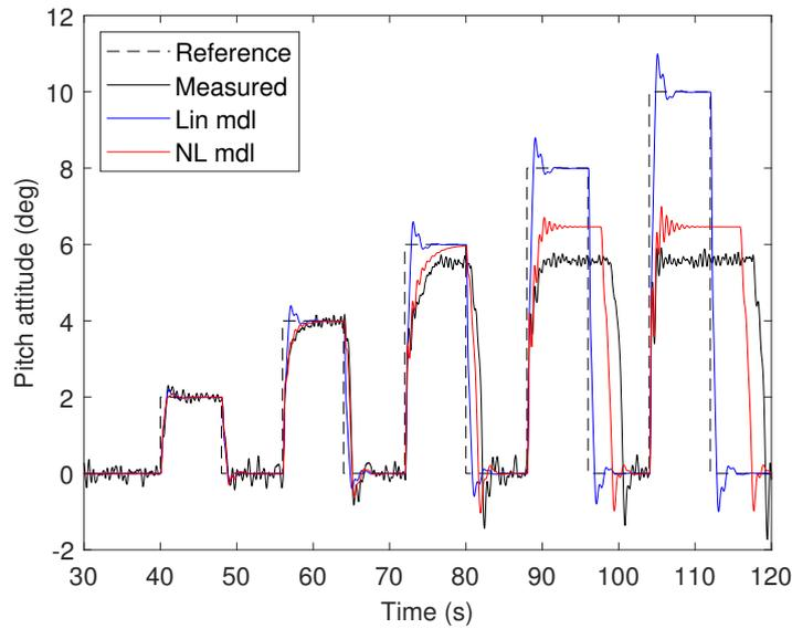
Figure 3.43 – Pitch attitude tracking of the state-space co-design
