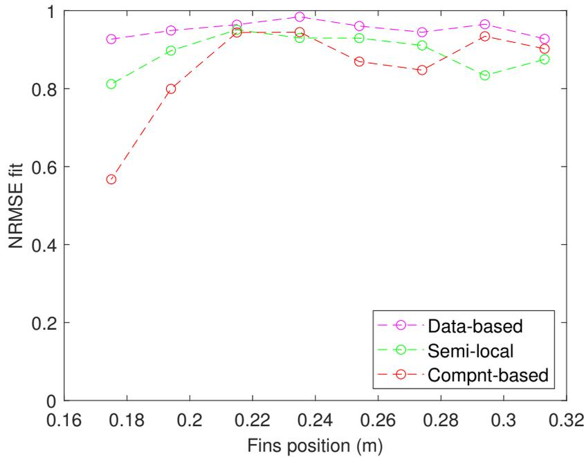
Figure 2.31 – Open-loop response fit for different fins positions
