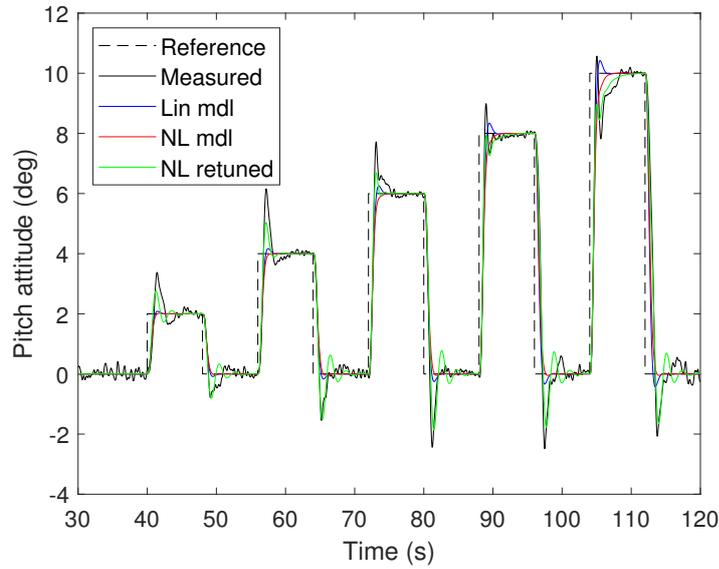
Figure 3.48 – Pitch attitude tracking of the RSS projectile
