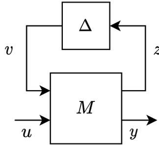
Figure 2.8 – Linear Fractional Representation of the parameter-dependent plant
