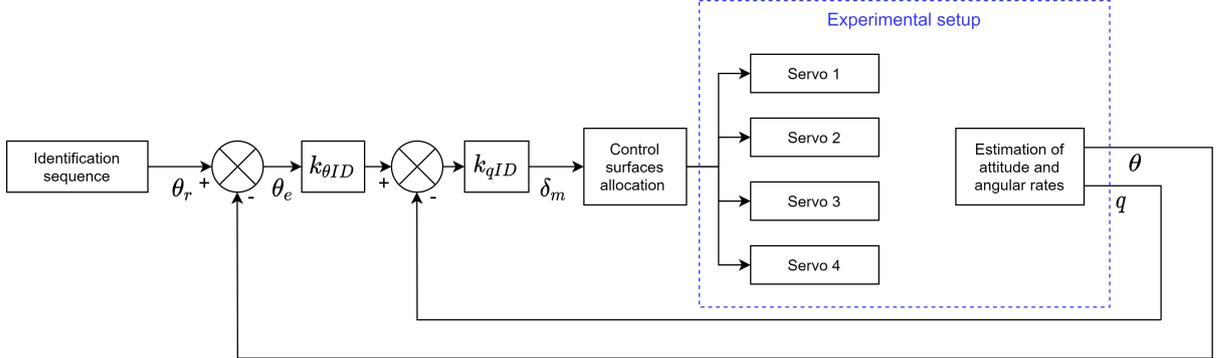
Figure 2.3 – Layout of the identification controller
