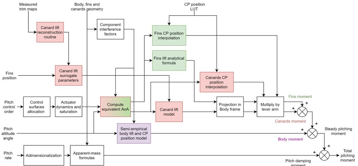
Figure 2.20 – FAST diagram of component-based model
