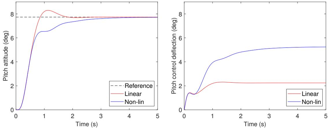
Figure 3.27 – Projectile step response at maximum control AoA
