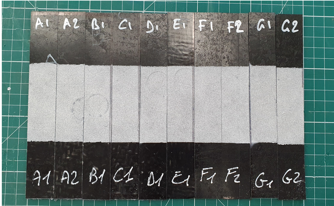
Figure 6.5: Samples painted with the speckle pattern.
