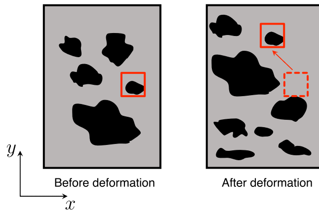
Figure A.1: Example of how the subset is tracked in the sample. The subset is represented by the red square, whose movement is observed going from the original position (dashed line) over to the updated position after deformation (solid line).
