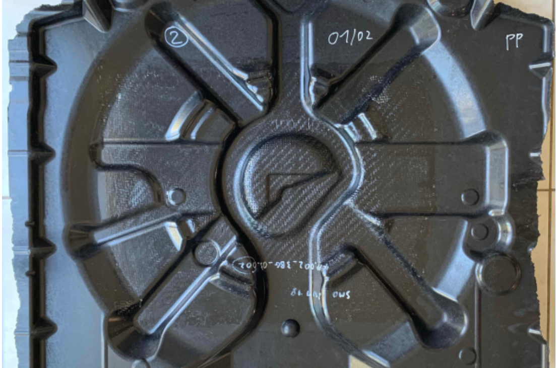
Figure 6.1: Spare wheel tray from where the samples for testing were obtained.
