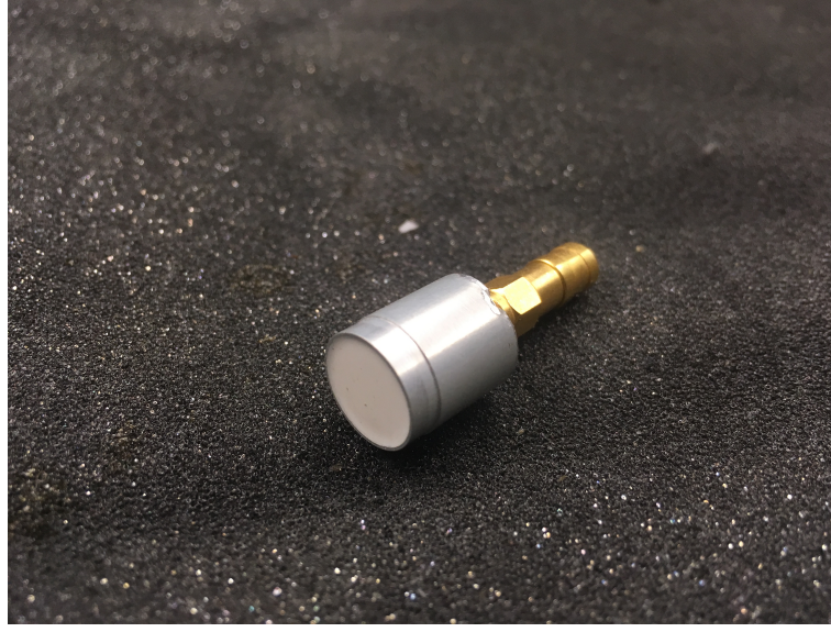
Fig. IV.5 Image of the ultrasound transducer used in the experiment. Diameter of the transducer is 12 mm and has emitting frequency of 230 kHz.
