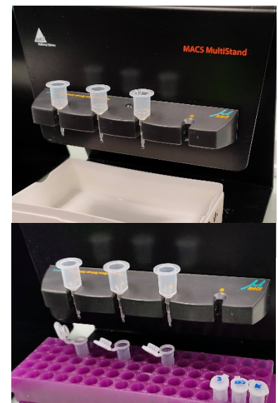
Figure 53 : Pictures to show how to use the \mu MACS columns in the magnetic stand. The top picture is when the columns are washed. The bottom picture is when the flowthrough is collected.
