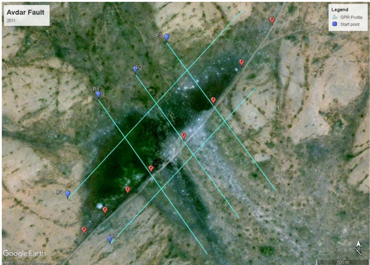
*Figure 2.24 Location map of ground penetrating radar profiles in Z2 zone. The zone location is shown in Figure 2.23. Light blue lines indicate the profiles at the RTA50 MHz, 500 MHz and 250 MHz antenna. The blue symbols are indicating the start points and name of profiles. The red symbols are representing fault trace.*
