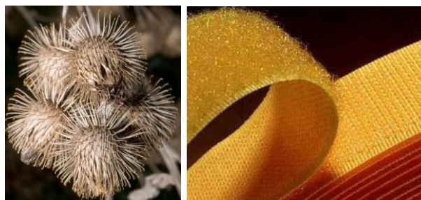
Figure 17 : The principle behind the burr (left) in Nature and the artificial imitation material, Velcro (right). [87]
