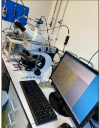
Figure V. 2 Solvent vapor annealing setup connected to an optical microscope and a Keithley machine.
