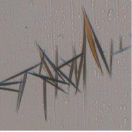
Figure V. 29 Needle type crystals of HDPPD grown upon exposure to vapor of chloroform.
