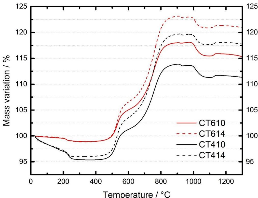
**Figure 97.** TGA curve of nanothermites obtained at 5°C min<sup>-1</sup> and 100 mL min<sup>-1</sup> of Ar/O<sub>2</sub> (98%/2%).
