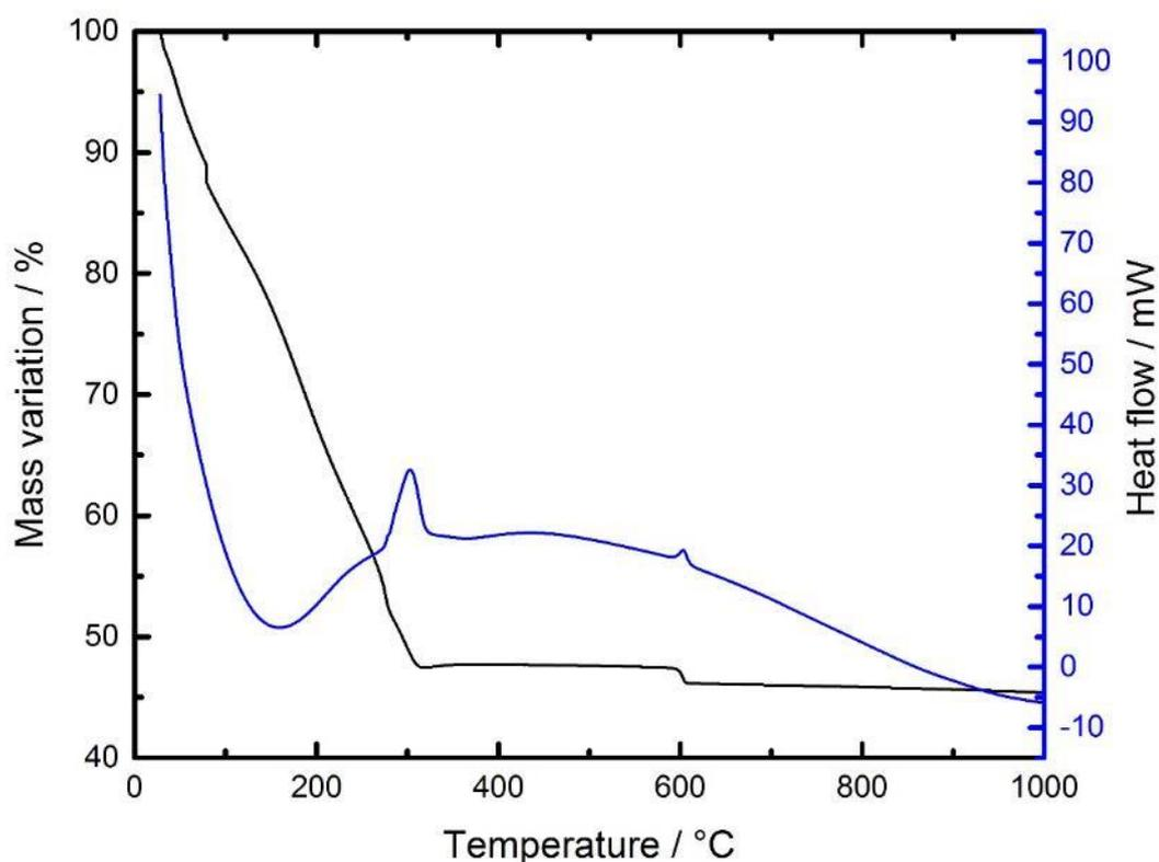
**Figure 52.** TG analysis of BiTi 1:1.35 powder.
