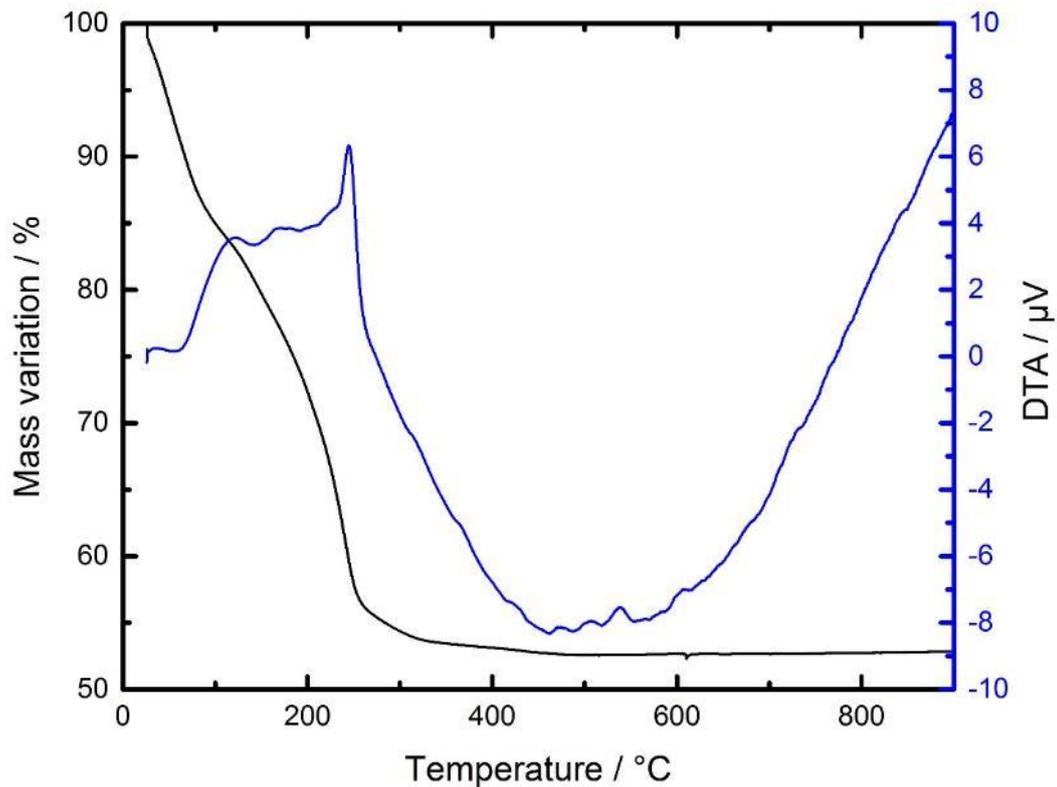
**Figure 81.** Thermogravimetric analysis of raw copper/titanium precursor mixture.
