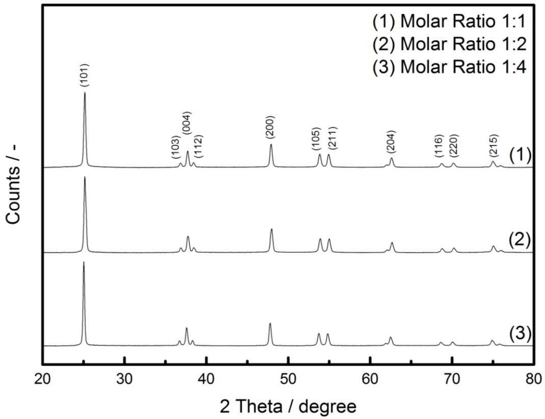
**Figure 23.** XRD patterns for  $TiO_2$  samples.
