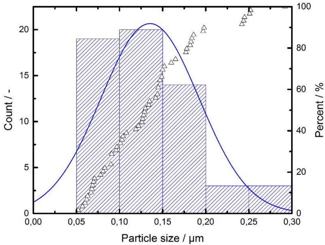
**Figure 68.** Histogram and cumulative particle size distribution for raw BiTi 2:1.
