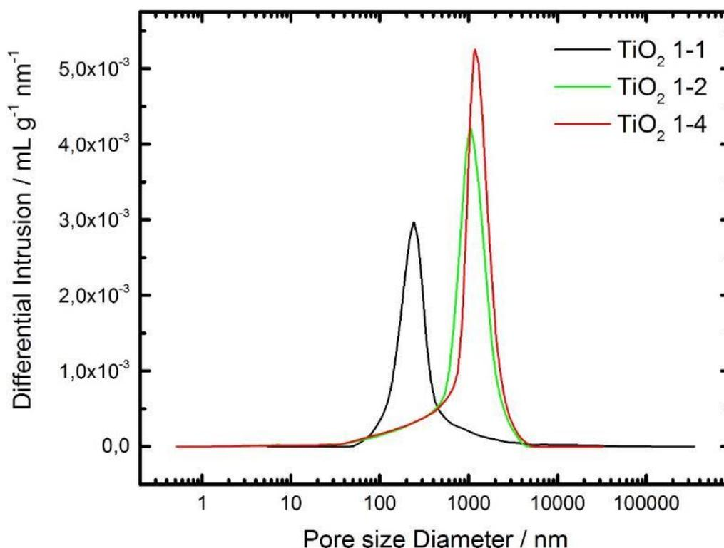
**Figure 28.** Pore volume distribution of the titanium oxide samples measured by mercury porosimetry.
