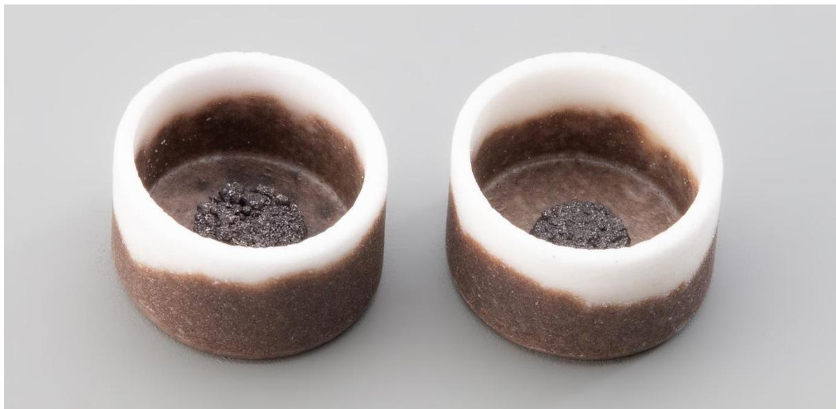
**Figure 98.** TGA sample holders after analysis of the nanothermites.
