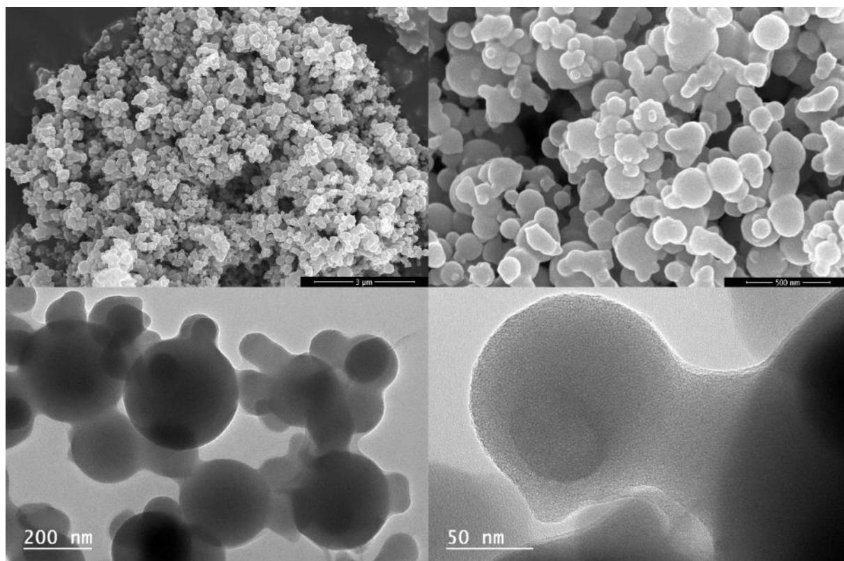
**Figure 9.** SEM and TEM images of 1:1 TiO<sub>2</sub> precursor.
