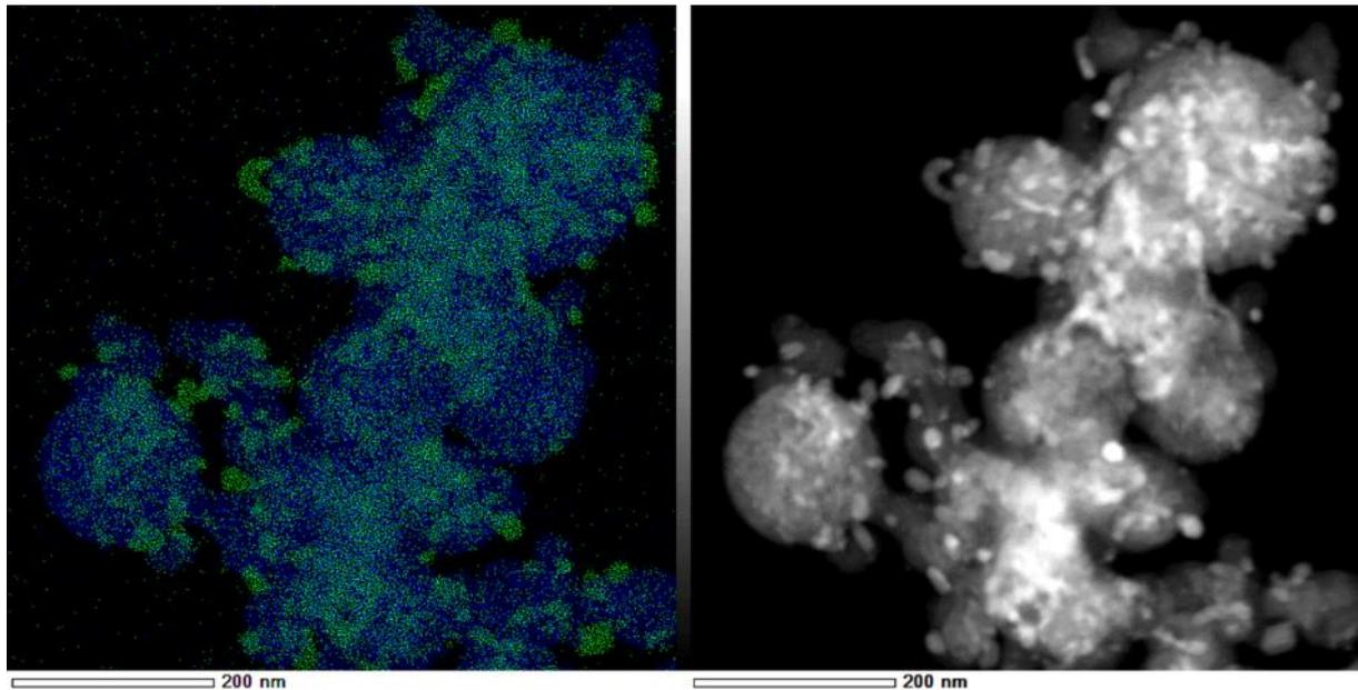
**Figure 34.** EDX of silver oxide covered titanium oxide (Blue: titanium; Green: silver).
