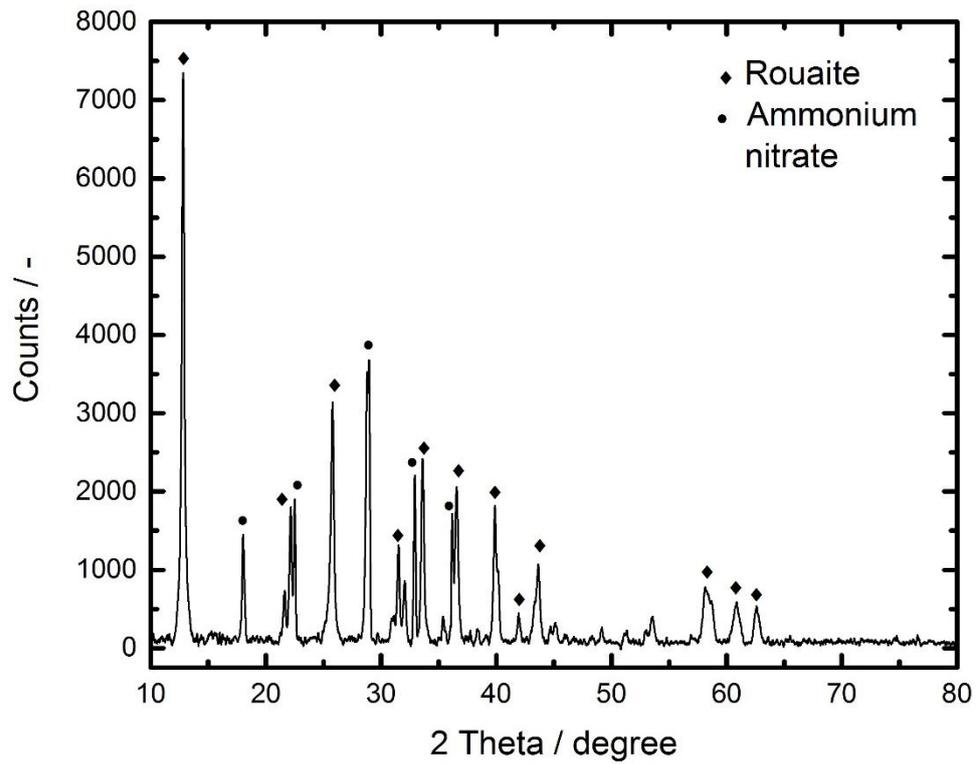
**Figure 9.** XRD pattern of raw copper/titanium precursor mixture.
