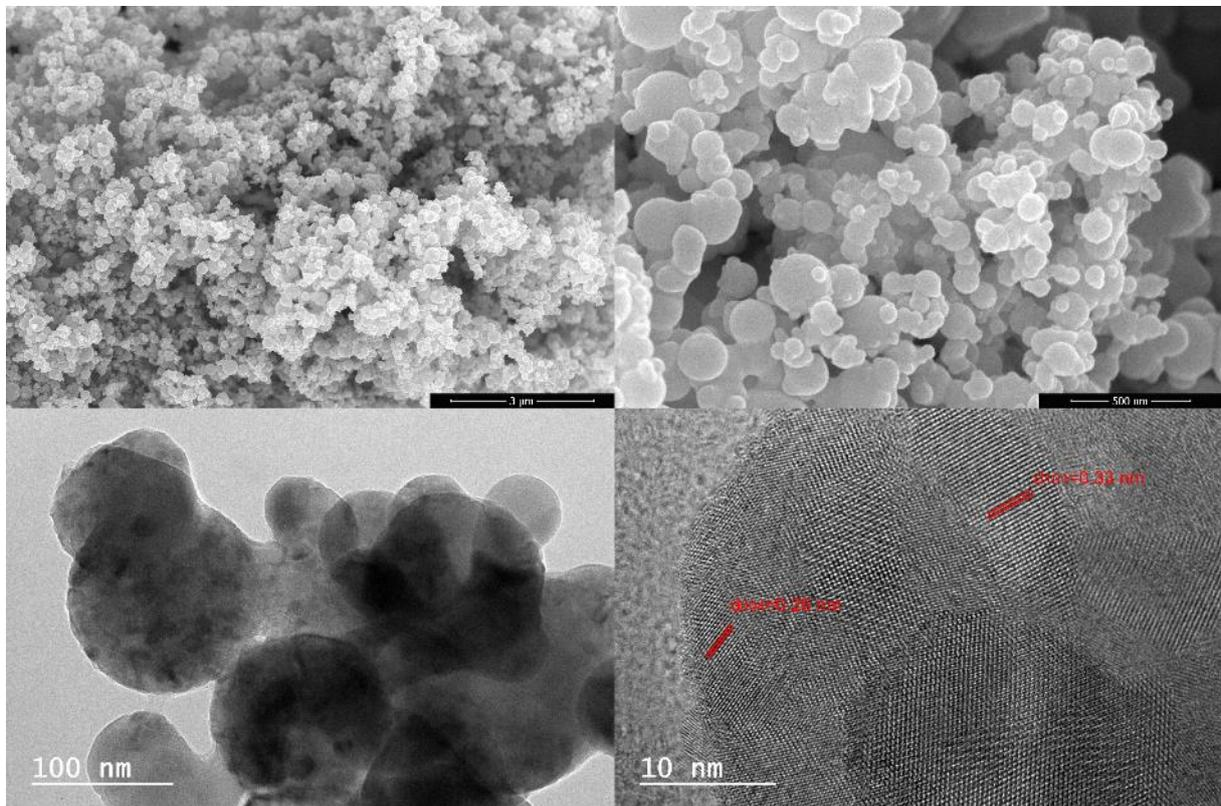
**Figure 1.** SEM and TEM images of TiO<sub>2</sub> 1:1.
