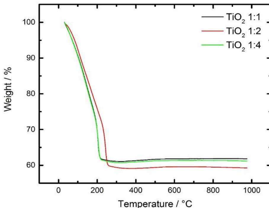
**Figure 12.** TGA curve for different  $TiO_2$  samples.
