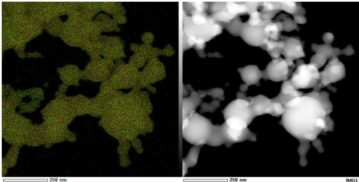
**Figure 69.** EDX image of particles of BiTi 2:1 (bismuth in green and titanium in red).
