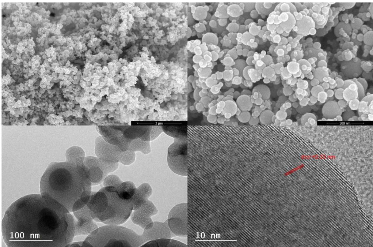
**Figure 20.** SEM and TEM images of  $\text{TiO}_2$  1:4.
