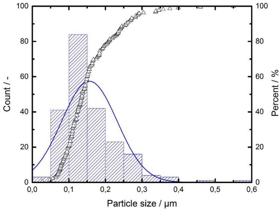
**Figure 30.** Histogram and cumulative particle size distribution for raw Ag@TiO<sub>2</sub>.
