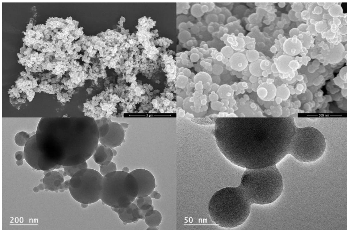
**Figure 11.** SEM and TEM images of 1:4  $\text{TiO}_2$  precursor.
