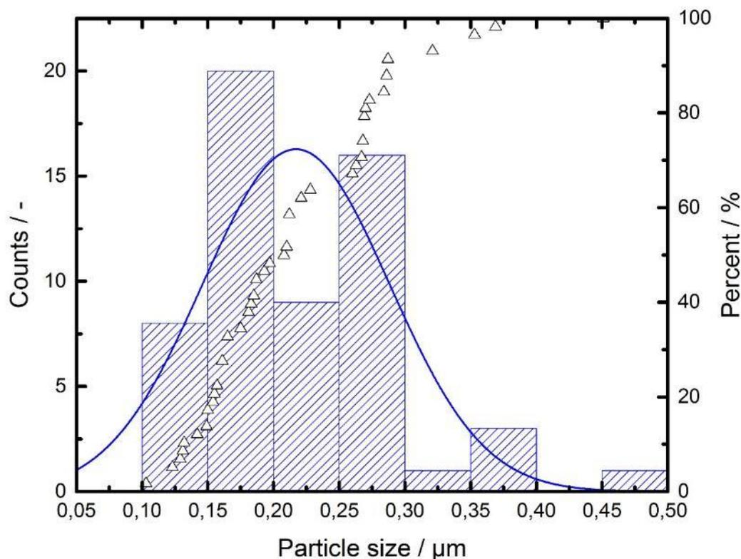
**Figure 90.** Histogram and cumulative particle size distribution for copper/titanium oxide mixture calcined at 600°C.
