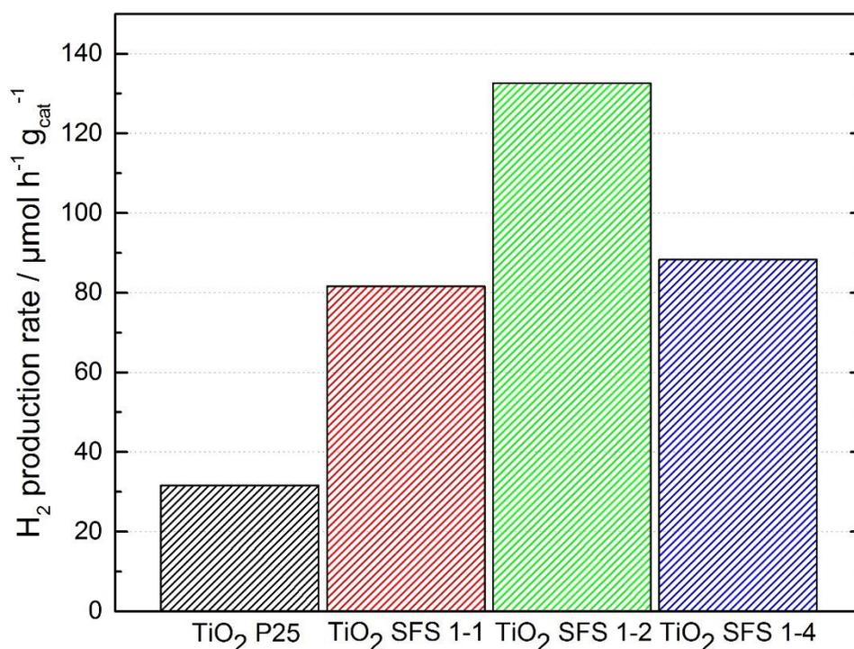
**Figure 106.** Hydrogen production by methanol photoreforming using SFS prepared TiO<sub>2</sub> in comparison to reference P25 (experimental conditions detailed in Chapter II: 6).
