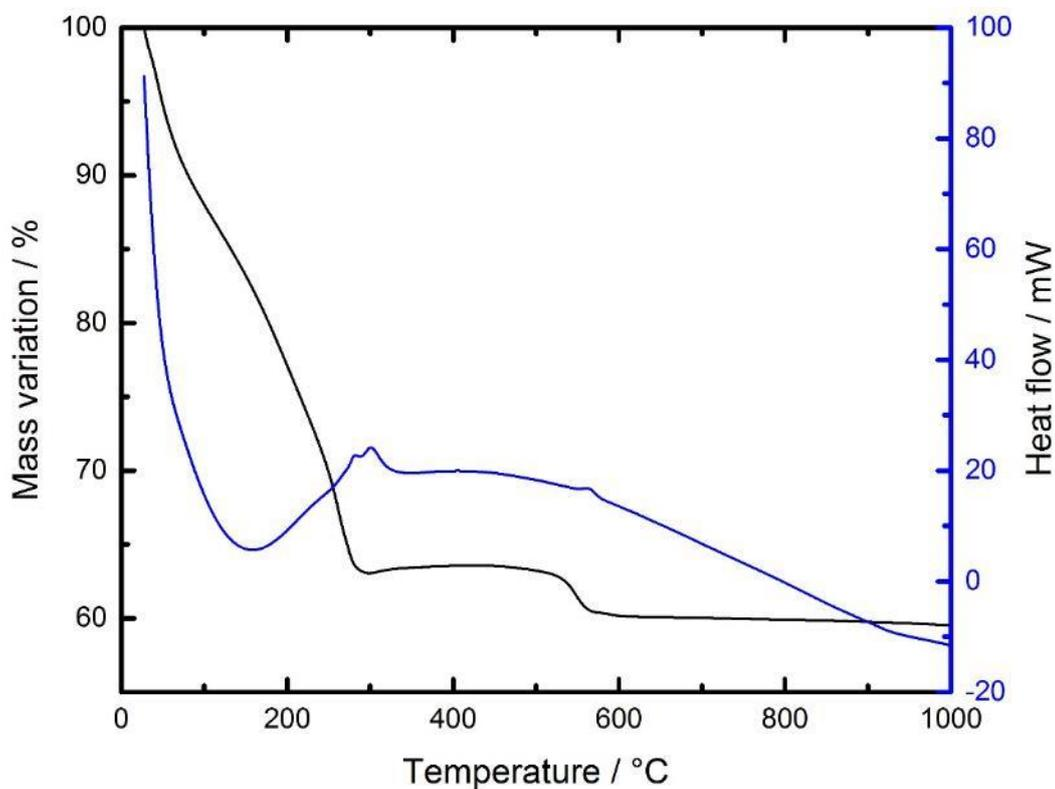
**Figure 61.** TG analysis of raw BiTi 1:1 molar ratio.
