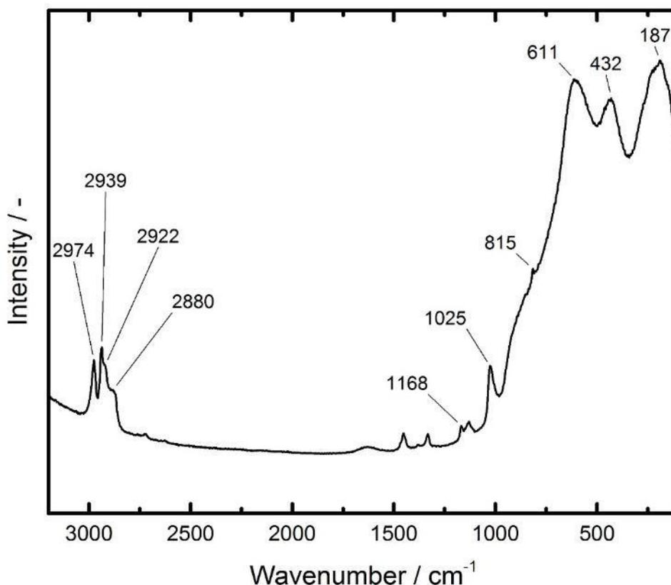
**Figure 15.** RAMAN spectra of uncalcined  $\text{TiO}_2$  1:2 sample.
