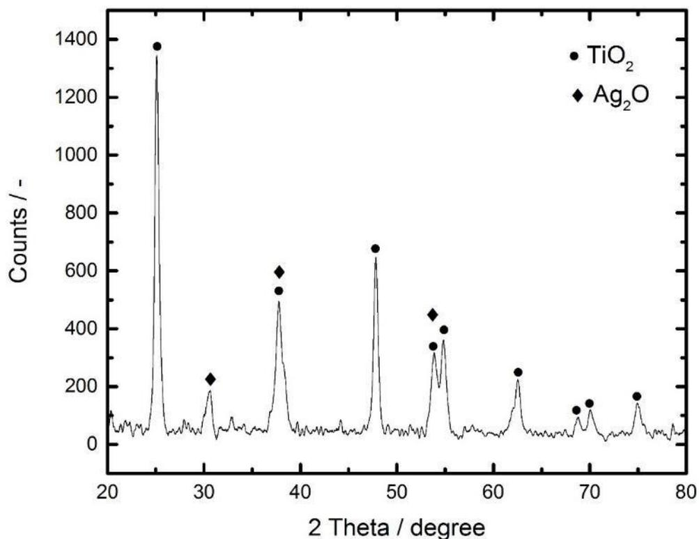
**Figure 35.** XRD pattern of Ag@TiO<sub>2</sub> sample calcined at 400°C.
