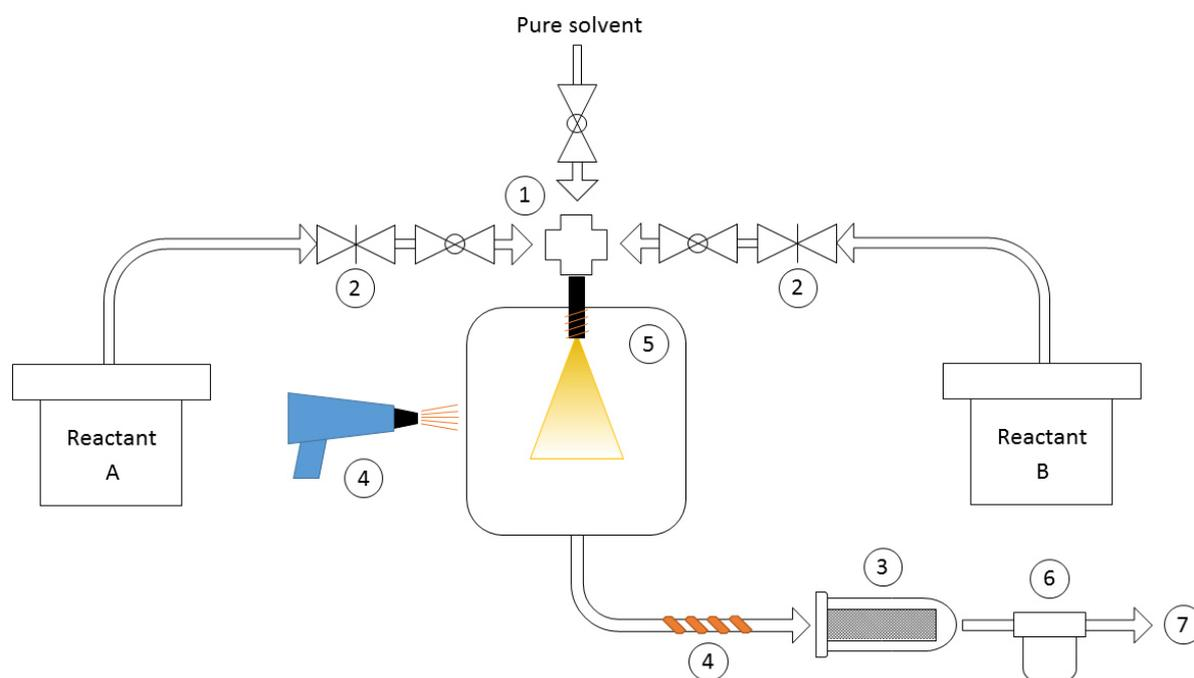
**Figure 5.** Schematic of the SFS system. 1. Mixing of liquids; 2. Flow rate control; 3. Powder recovery system; 4. Auxiliary heating system; 5. Joints and sealing; 6. Acid recovery device; 7. Vacuum pump
