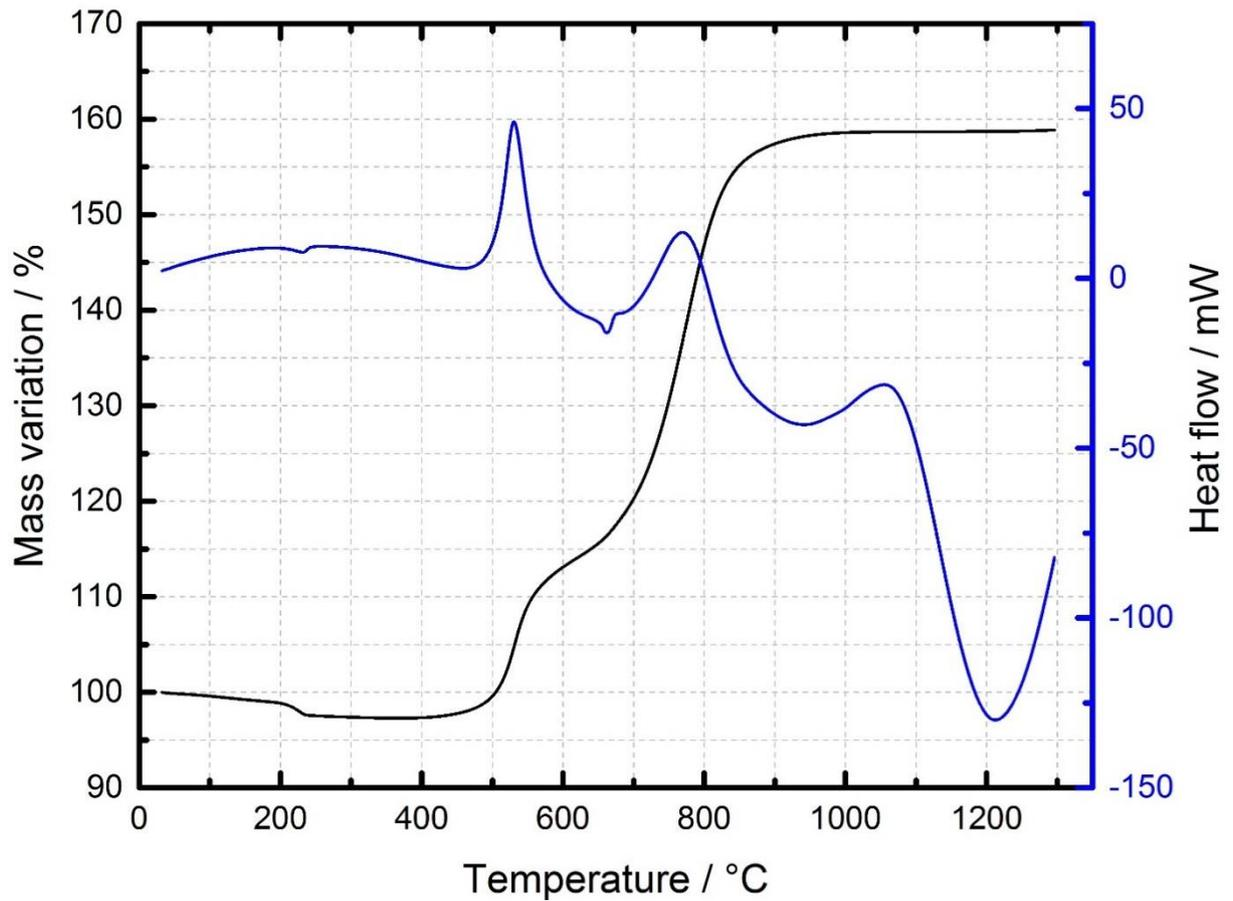
**Figure 93.** TGA and DTA curves of nano-aluminium powder obtained at 5°C/min and 100 mL/min of Ar/O<sub>2</sub> (98%/2%).
