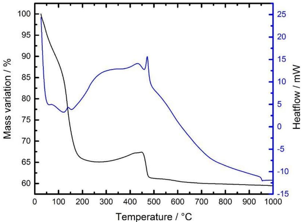
**Figure 31.** TG analysis of amorphous, silver loaded titanium oxide particles at a heating rate of 5°C/min with and 100 mL/min of Ar/O<sub>2</sub> 80%/20%.
