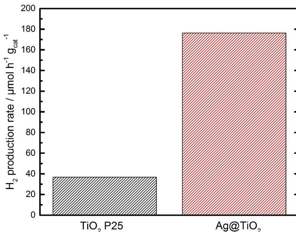
**Figure 108.** Hydrogen production by photoreformation using silver loaded TiO<sub>2</sub> in comparison to reference P25 (experimental conditions detailed in Chapter II: 6).
