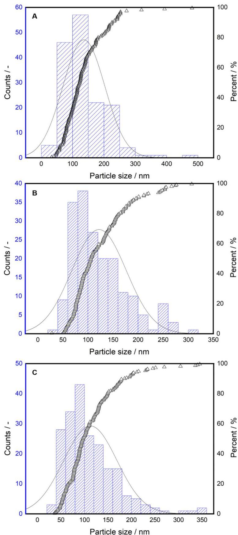
**Figure 25.** Histogram and cumulative particle size distribution for A) TiO<sub>2</sub> 1:1; B) TiO<sub>2</sub> 1:2 and C) TiO<sub>2</sub> 1:4.
