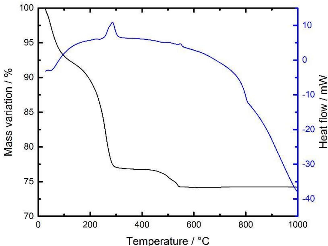
**Figure 70.** TG analysis of raw BiTi 2:1 molar ratio.
