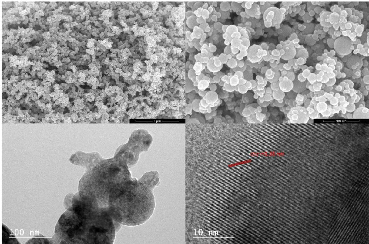
**Figure 2.** SEM and TEM images of  $\text{TiO}_2$  1:2.
