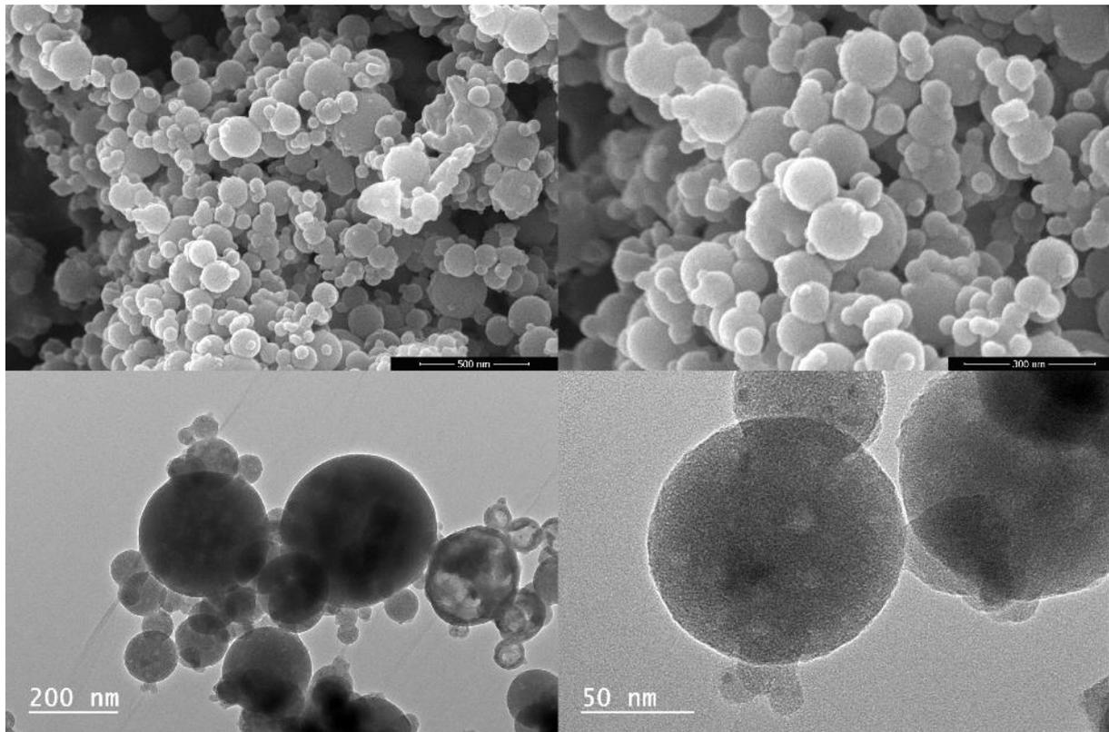
**Figure 8.** SEM images of raw copper/titanium precursor mixture.
