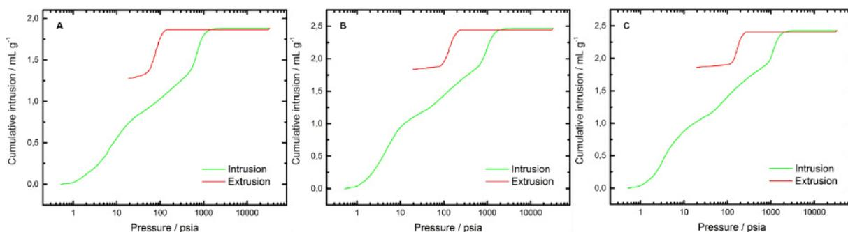
**Figure 27.** Mercury porosimetry intrusion curves of the titanium oxide samples for A) TiO<sub>2</sub> 1-1; B) TiO<sub>2</sub> 1-2 and C) TiO<sub>2</sub> 1-4.
