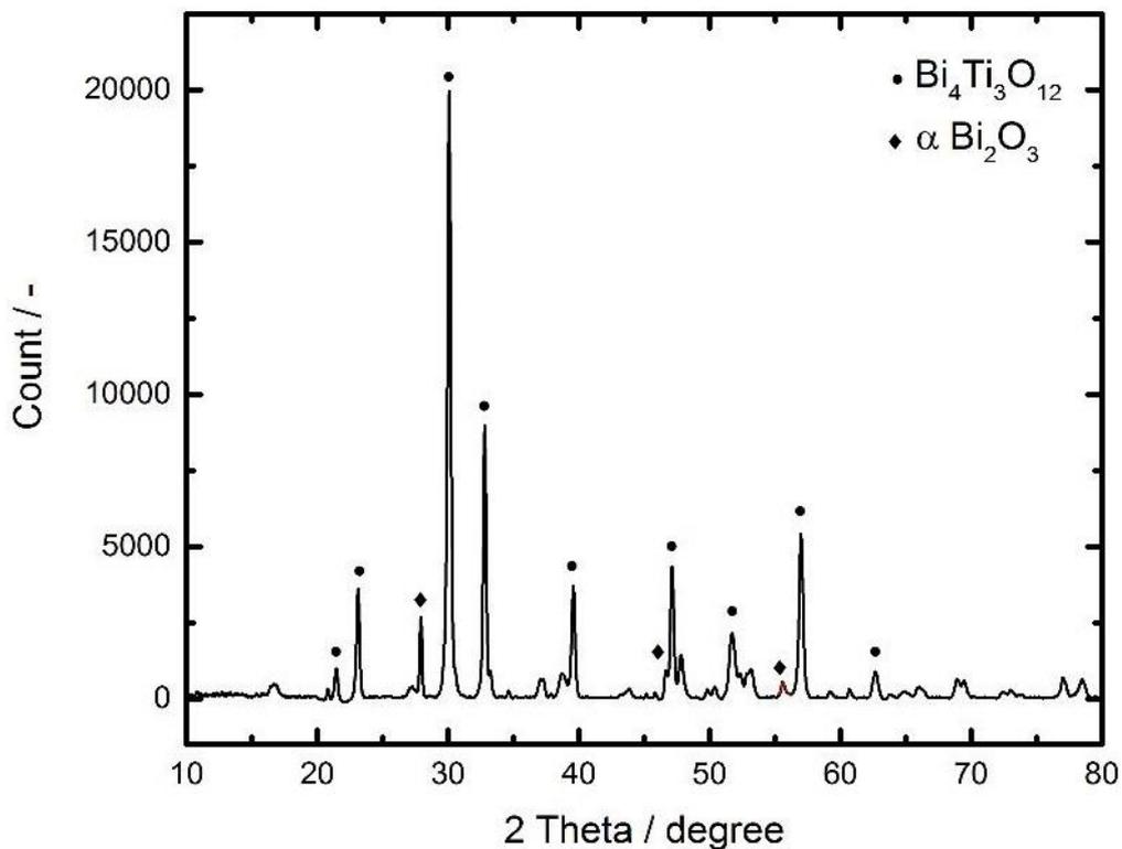
**Figure 72.** XRD pattern of BiTi 2:1 sample calcined at 650°C under air.
