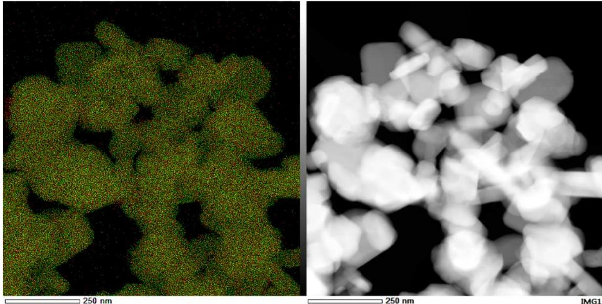
**Figure 73.** EDX image of particles of BiTi 2:1 (bismuth in green and titanium in red).
