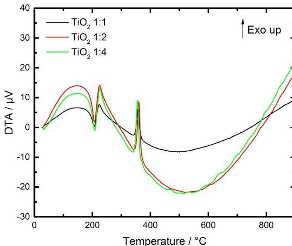
**Figure 14.** DTA curve for different  $\text{TiO}_2$  samples.
