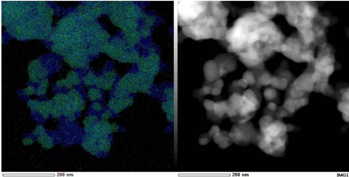
**Figure 53.** EDX image of particles of bismuth titanate BiTi 1:1.35 powder (Bismuth in green and titanium in blue).
