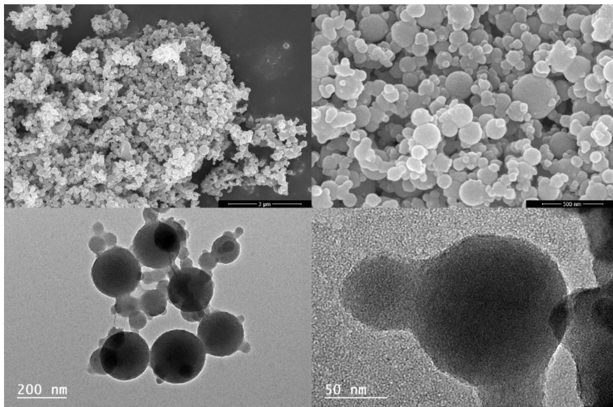
**Figure 10.** SEM and TEM images of 1:2  $\text{TiO}_2$  precursor.
