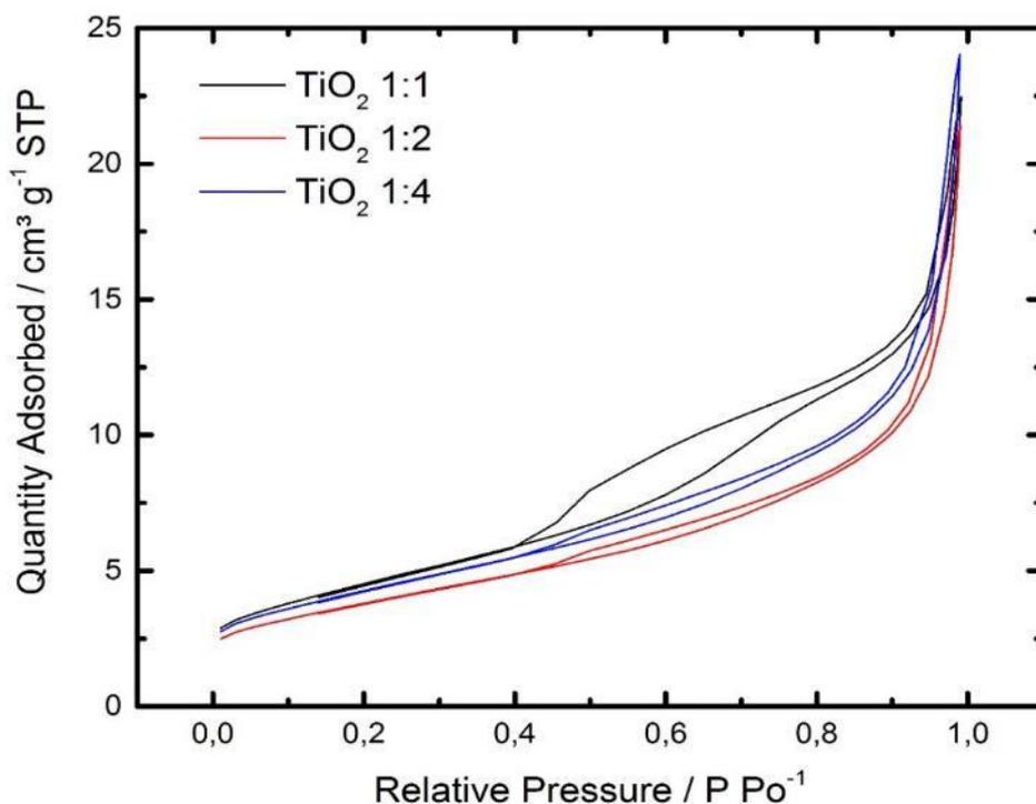
**Figure 26.** *TiO<sub>2</sub> samples isotherms by BET measurements.*
