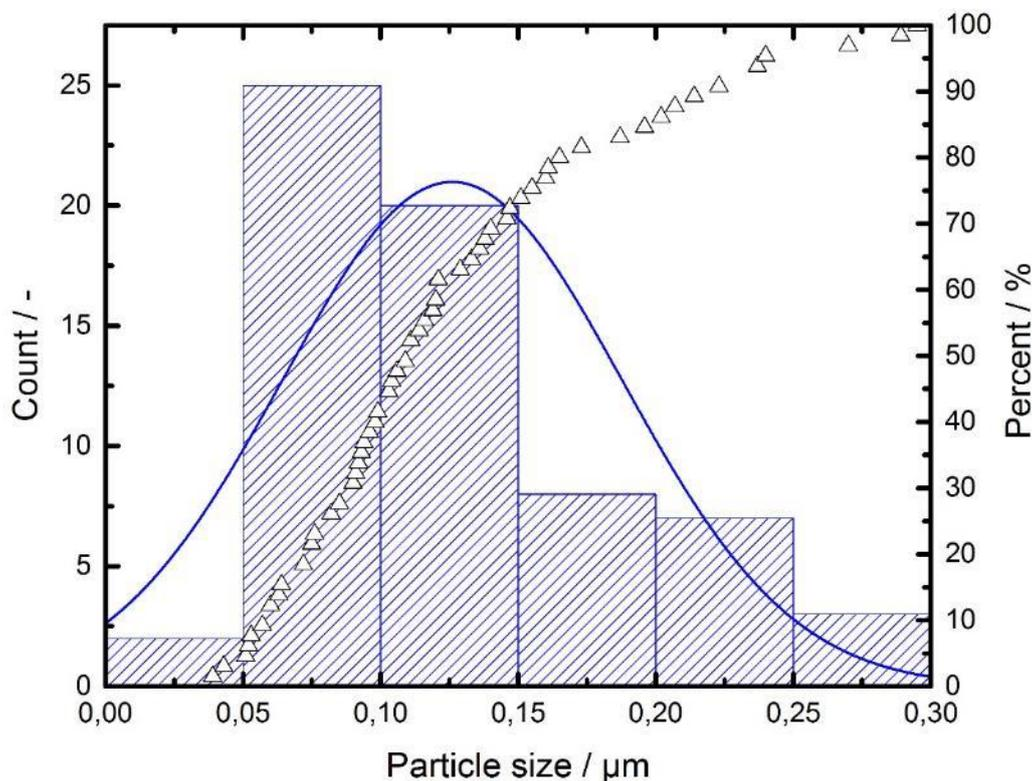
**Figure 7.** Histogram and cumulative particle size distribution for BiTi 1:1.
