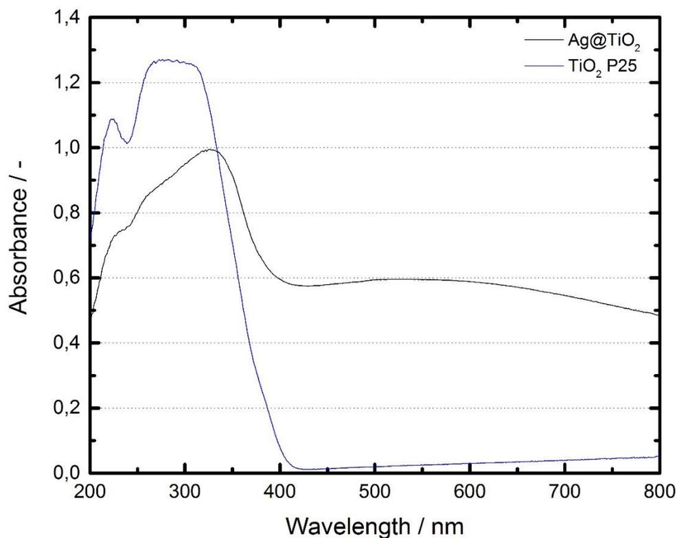
**Figure 107.** UV-Vis absorbance spectra of silver-modified titanium oxide prepared by SFS.
