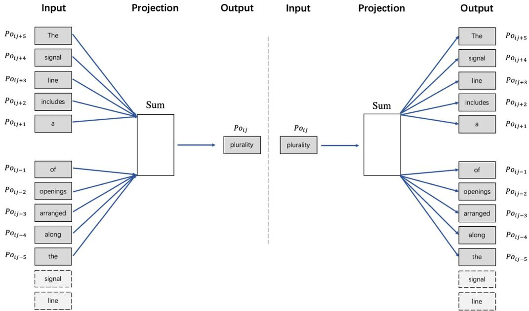
FIGURE 4.2: Architecture of Word2vec model: CBOw (left) and Skip-gram (right)
