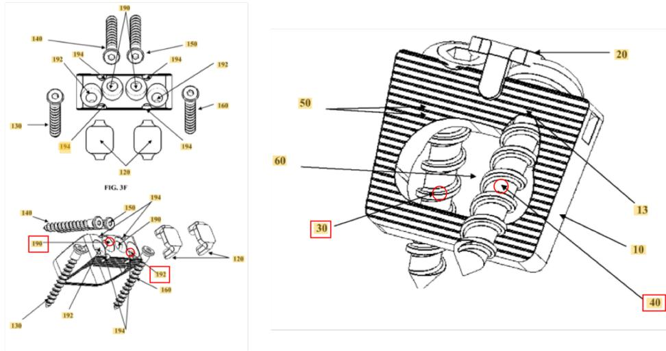
FIGURE 4.10: The illustration of the locking mechanism
