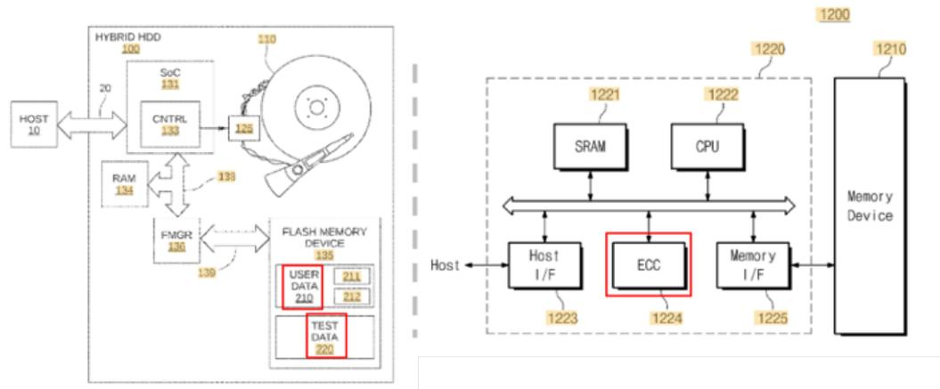
FIGURE 4.8: Diagrams of the hybrid HDD (left) and the memory systems (right)
