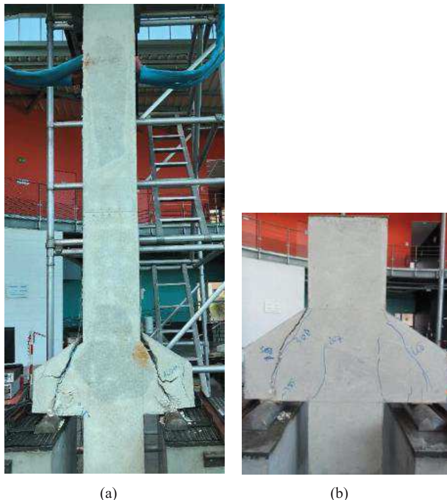
Figure III-15 : Fissuration et rupture (a) Poteau-console, (b) Console (b)
