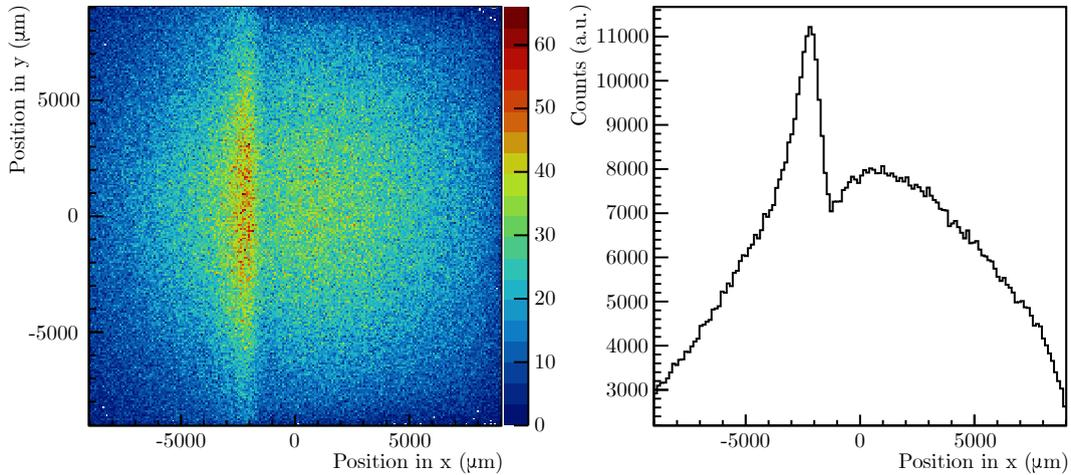
Figure 4.12: Two dimensional beam profile from MIMOSA-28 sensor (left panel), and its projection in  $x$  (right panel), for 150.14 MeV proton beam from the experimental measurements performed at MIT with the bone target placed along the beam axis.
