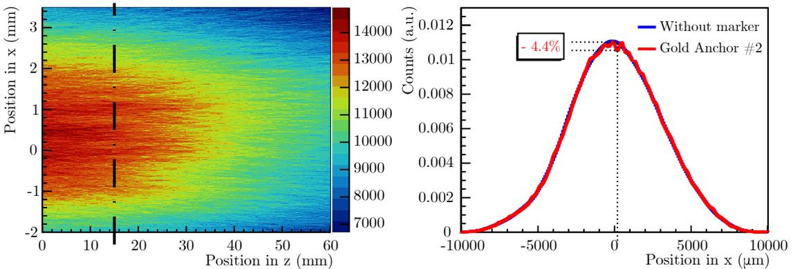
Figure 4.21: Reconstructed fluence map and beam profile for 310.61 MeV/u carbon ion beam through the Gold Anchor #2 marker placed at position zero in  $(x, z)$  coordinates. The panels description is the same as Figure 4.18.
