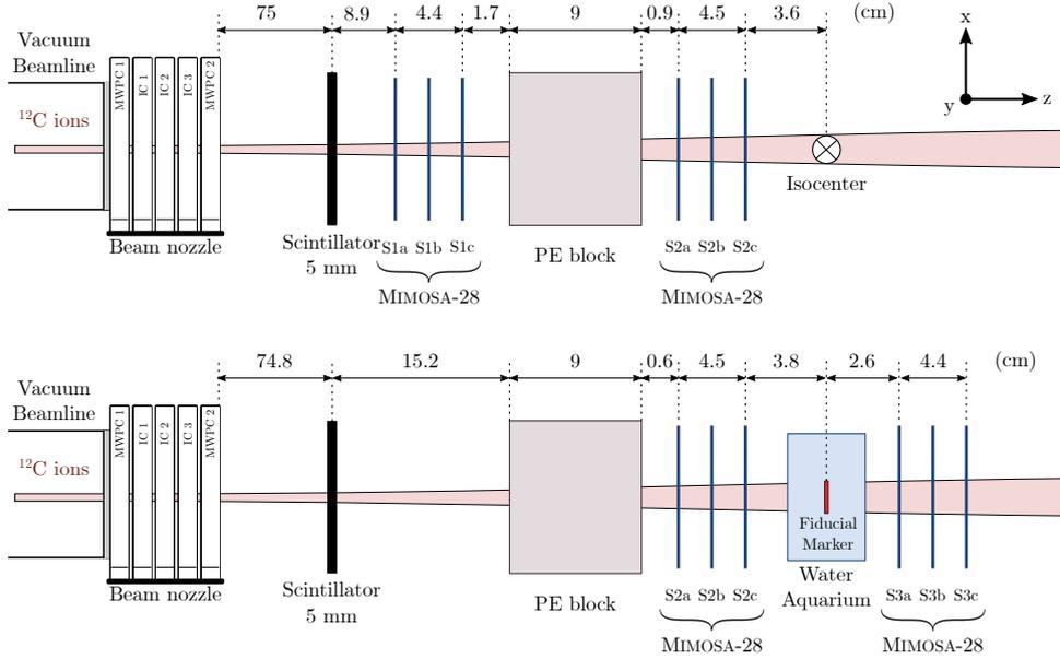
Figure 3.5: Experimental configurations used to measure the fluence perturbation of several carbon ion beams due to fiducial markers with six MIMOSA-28 pixel sensors placed along the beam axis.
