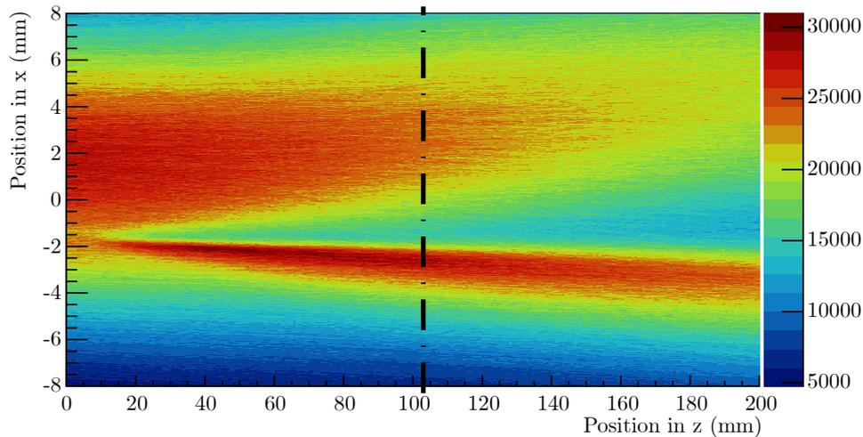
Figure 4.15: Reconstructed fluence map for 150.14 MeV proton beam passing through the gold hammer target placed at position zero in  $(x, z)$  coordinates. The fluence map was computed from all tracks reconstructed with MIMOSA-28 sensors. The vertical dotted line shows the position of the first sensor placed behind the target.
