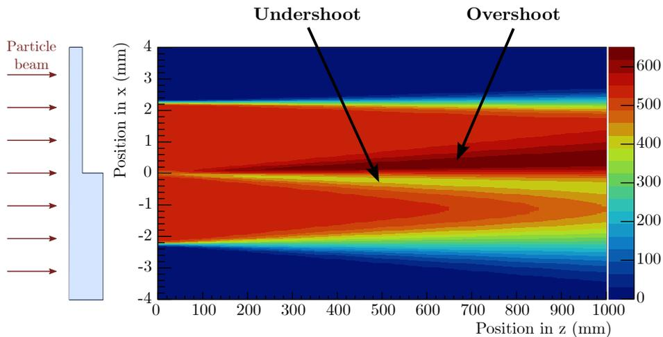
Figure 1.7: Inhomogeneous scattering of a beam particle passing through strong density gradients and sharp edges. The fluence perturbation from edge-scattering effects creates an under- and overshoot behind the target.
