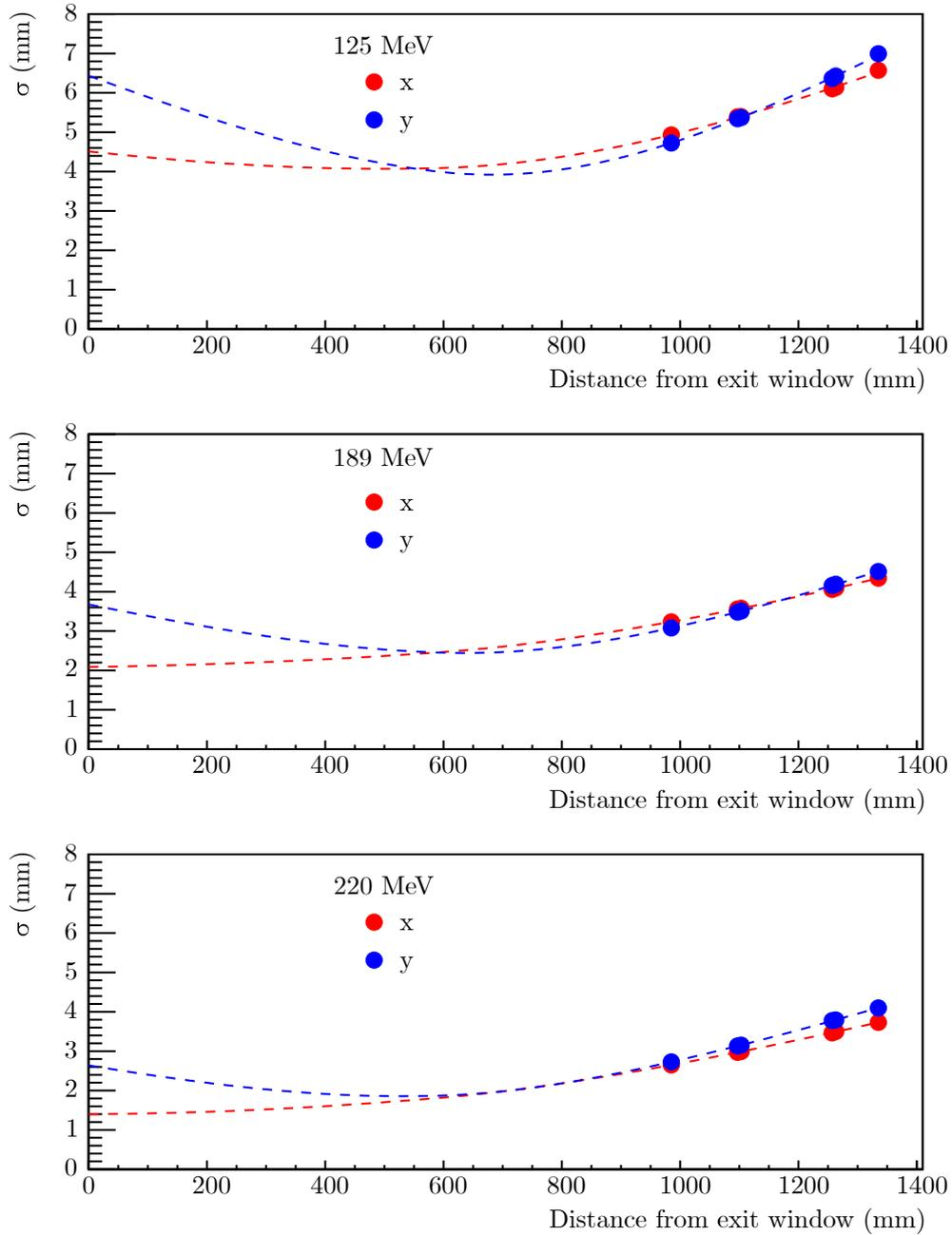
Figure 4.11: Lateral beam profile measurements of MIMOSA-28 sensors in  $x$  and  $y$ , and fitted with the transport code SCATTMAN for 125.3 MeV (top panel), 188.8 MeV (middle panel) and 219.8 MeV (bottom panel) proton beams. The data from the MIMOSA-28 sensors were recorded in the experimental room at the Proton Therapy Center in Trento.
