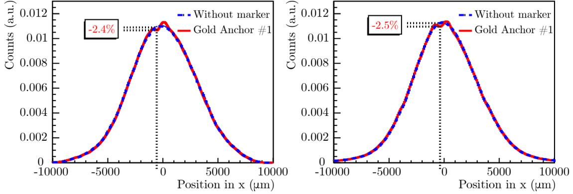
Figure 4.17: Experimental measurements of the beam profiles in  $x$  for 294.97 MeV/u carbon ion beam taken from MIMOSA-28 sensor S3a (left panel) and EBT3 radiochromic film F3 (right panel). The perturbation induced by the Gold Anchor #1 placed inside the aquarium (red line) is compared to the system without any perturbation (dashed blue line).
