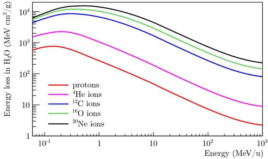
Figure 1.4: Stopping power as a function of the energy for protons (red line),  $^4\text{He}$  (magenta line),  $^{12}\text{C}$  (blue line),  $^{16}\text{O}$  (green line) and  $^{20}\text{Ne}$  (black line) ions in water. The energy loss values were calculated using LISE++ [50].
