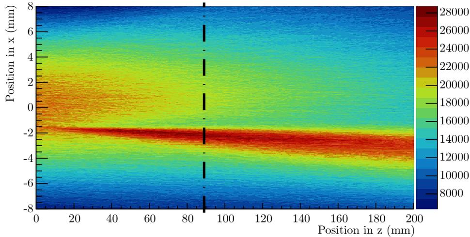
Figure 4.14: Reconstructed fluence map for 150.14 MeV proton beam passing through the bone target placed at position zero in  $(x, z)$  coordinates. The fluence map was computed from all tracks reconstructed with MIMOSA-28 sensors. The vertical dotted line shows the position of the first sensor placed behind the target.
