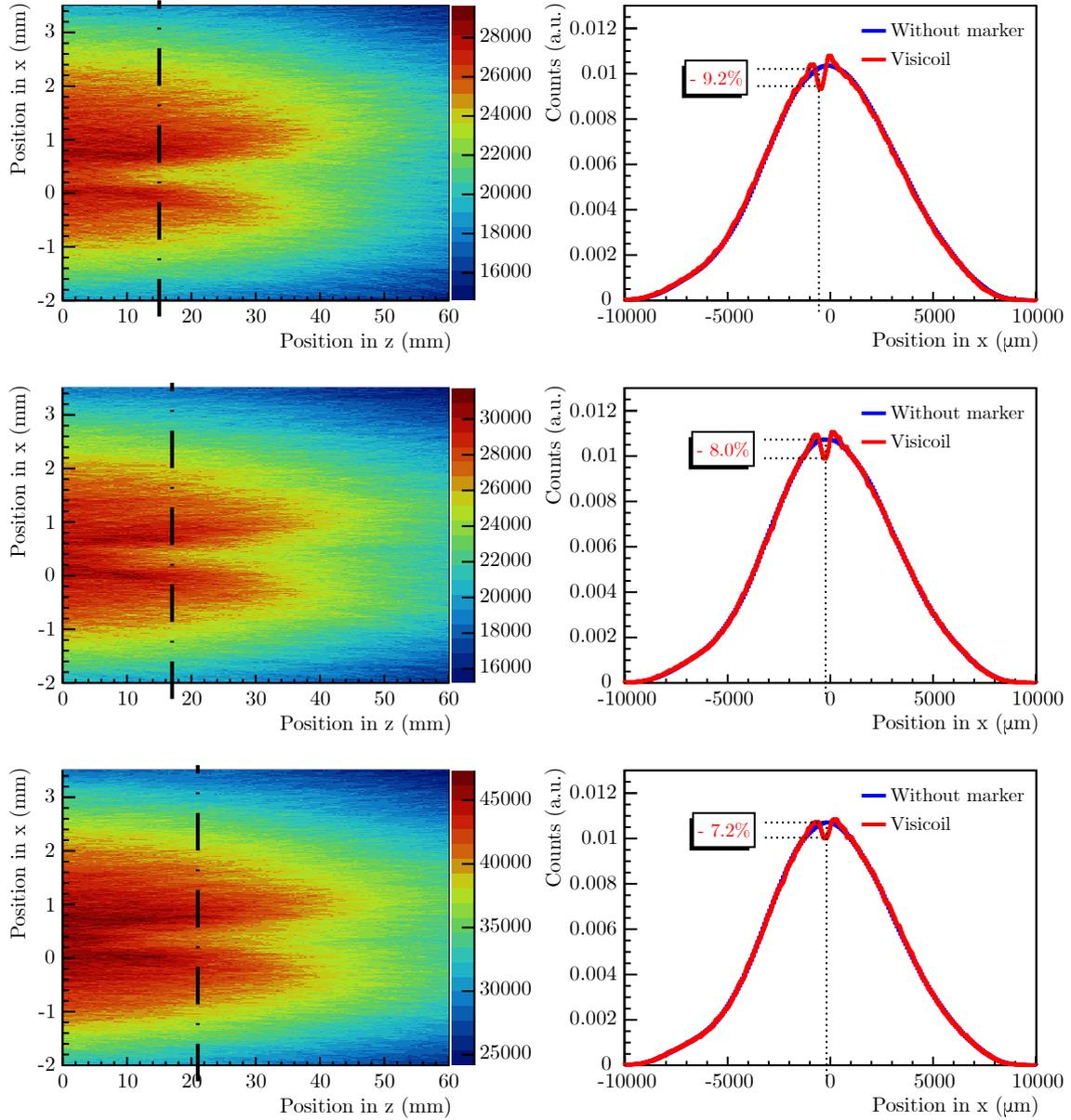
Figure 4.19: Reconstructed fluence maps and beam profiles of carbon ions at three different energies through the Visicoil marker placed at position zero in  $(x,z)$  coordinates. The panels description is the same as Figure 4.18.
