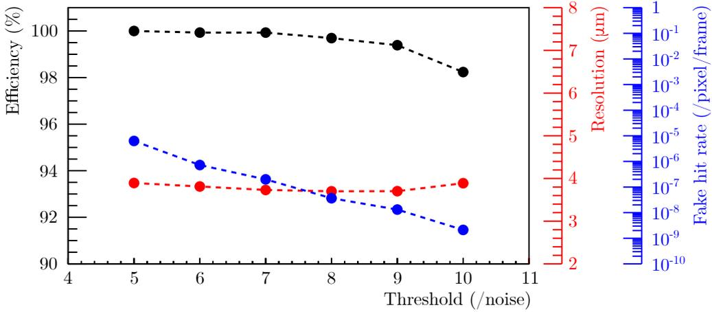
Figure 2.5: Performance of MIMOSA-28 as a function of the noise threshold measured at 30°C with minimum ionizing particles. The detection efficiency is shown in black, the single point resolution of the sensor is represented in red and the number of fake hits per pixel per readout frame is sketched in blue. Figure redrawn from [7].
