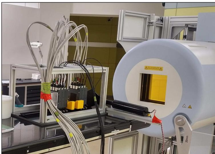
Figure 2.11: Photo of the MIMOSA-28 setup during an experiment performed at the Marburg Ion-beam Therapy Center, where six sensors are placed along an optical bench. All cables, connected to the sensor proximity boards, are clamped to a cage made from aluminum profiles.
