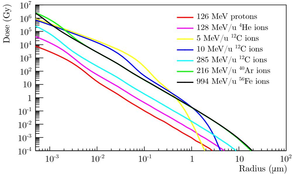
Figure 4.7: Radial dose distributions for 126 MeV protons (red line), 128 MeV/u <sup>4</sup>He ions (magenta line), 5 MeV/u <sup>12</sup>C ions (yellow line), 10 MeV/u <sup>12</sup>C ions (blue line), 285 MeV/u <sup>12</sup>C ions (cyan line), 216 MeV/u <sup>40</sup>Ar ions (green line) and 994 MeV/u <sup>56</sup>Fe ions (black line). These distributions were computed with the Monte Carlo code TRAX [67]. Data courtesy of Dr. Daria Boscolo.
