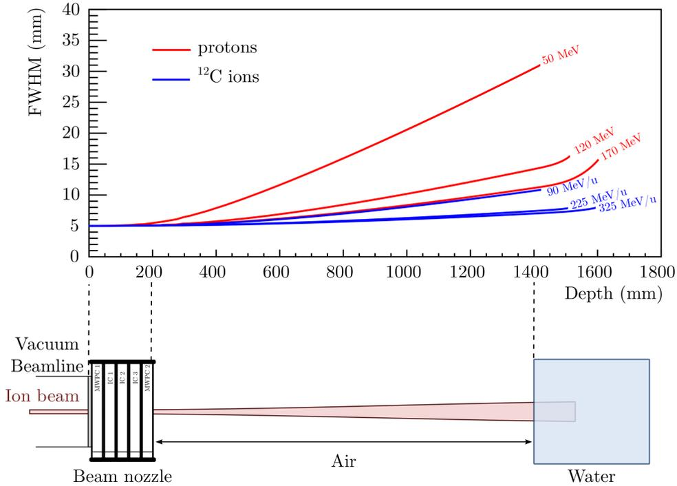
Figure 1.6: Lateral beam width as a function of the depth for protons (red lines) and carbon ions (blue lines) at different energies (top panel) for a setup representing a clinical case (bottom panel). The initial FWHM was set to 5 mm and the position 0 mm represents the exit window position. The calculations were performed with the transport code SCATMAN [5, 10].
