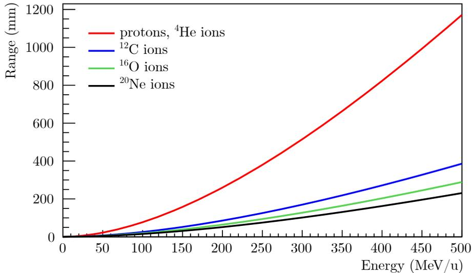
Figure 1.5: CSDA range in water as a function of the energy for protons (red line),  $^4\text{He}$  (red line),  $^{12}\text{C}$  (blue line),  $^{16}\text{O}$  (green line) and  $^{20}\text{Ne}$  (black line) ions. The range values were calculated with LISE++ [50].
