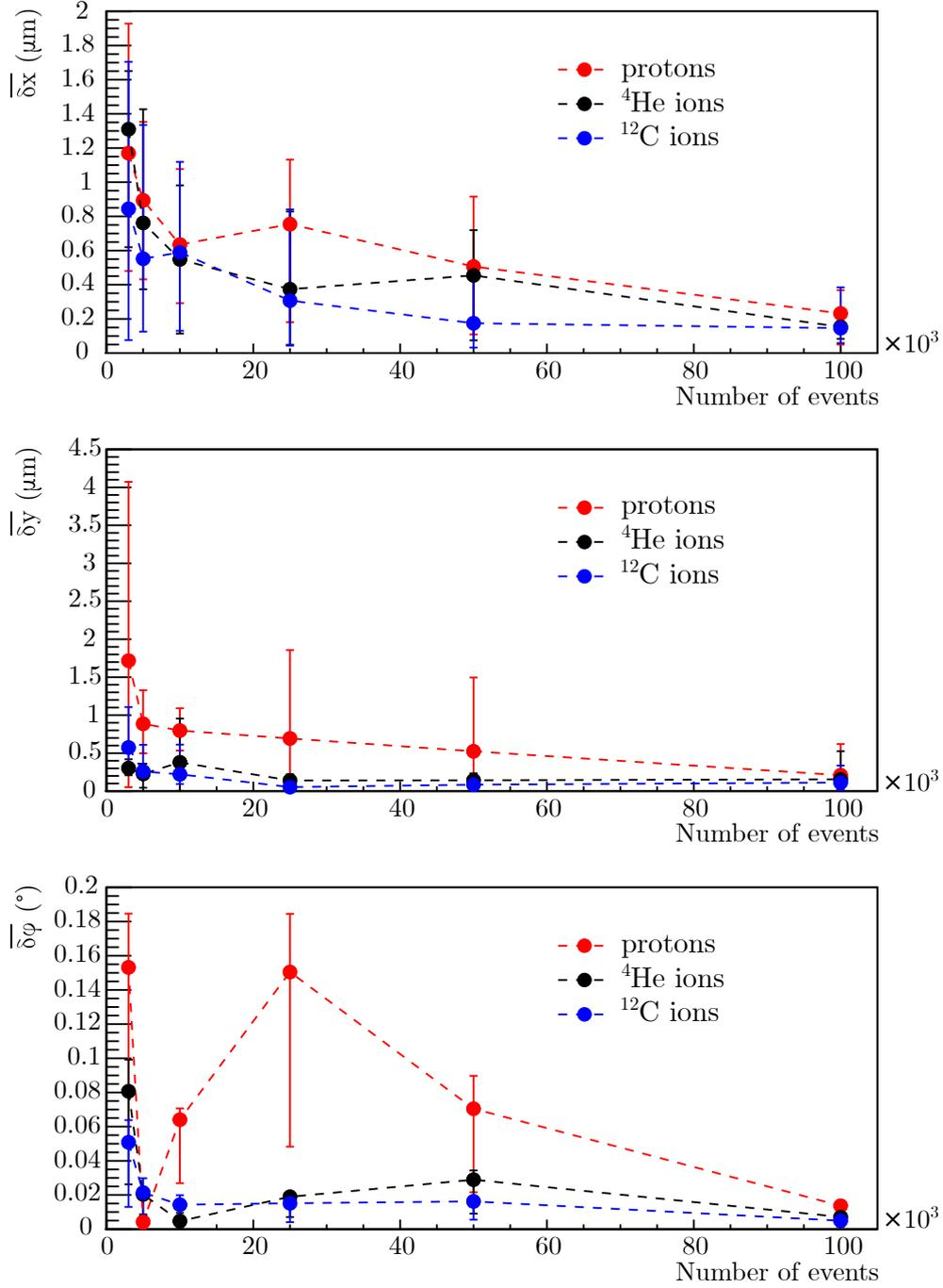
Figure 4.1: Average deviations  $\overline{\delta x}$  (top),  $\overline{\delta y}$  (middle) and  $\overline{\delta\phi}$  (bottom) between the calculated alignment parameters and set-misalignments, for the Monte Carlo simulations, as a function of the number of events, for 150 MeV/u protons, <sup>4</sup>He and <sup>12</sup>C ions with the scenario Geo2 – Mis3. The  $\delta$ -values are averaged over all sensors, and the error bars represent the range (min–max) of the  $\delta$ -values.
