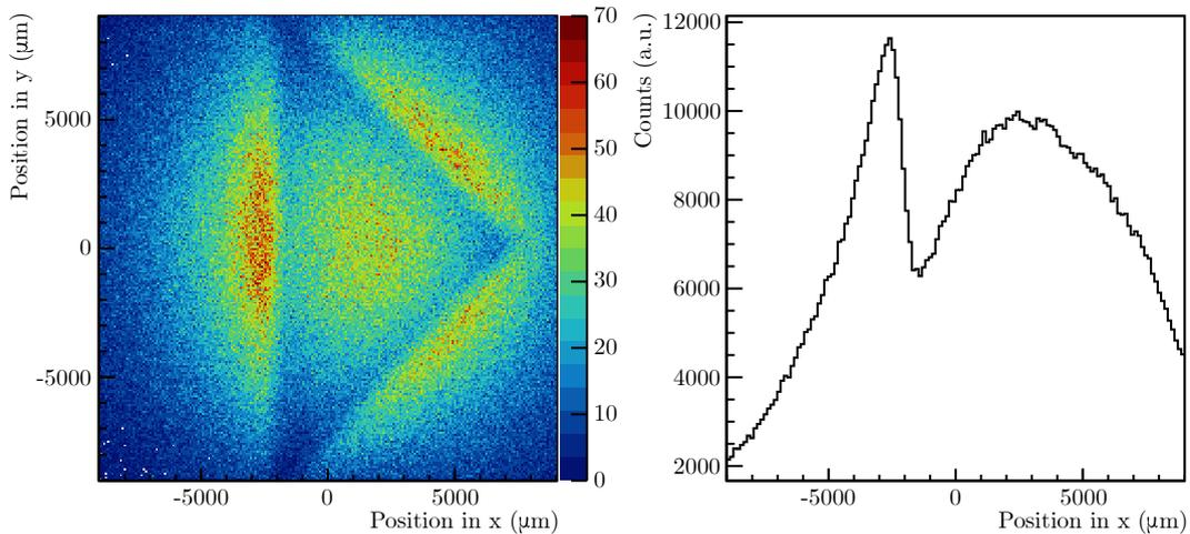
Figure 4.13: Two dimensional beam profile from MIMOSA-28 sensor (left panel), and its projection in  $x$  (right panel), for 150.14 MeV proton beam from the experimental measurements performed at MIT with the gold hammer target placed along the beam axis.
