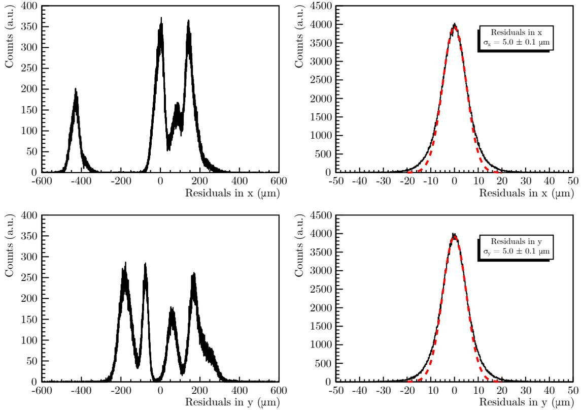
Figure 4.3: Histograms of the residuals in  $x$  (top panels) and  $y$  (bottom panels), before (left panels) and after (right panels) the alignment procedure ClusAlign for  $220.51 \text{ MeV/u}$   $^4\text{He}$  ions, for all sensors and all tracks (from the experimental data recorded at HIT). The red dotted line defines the Gaussian fit of the residuals.
