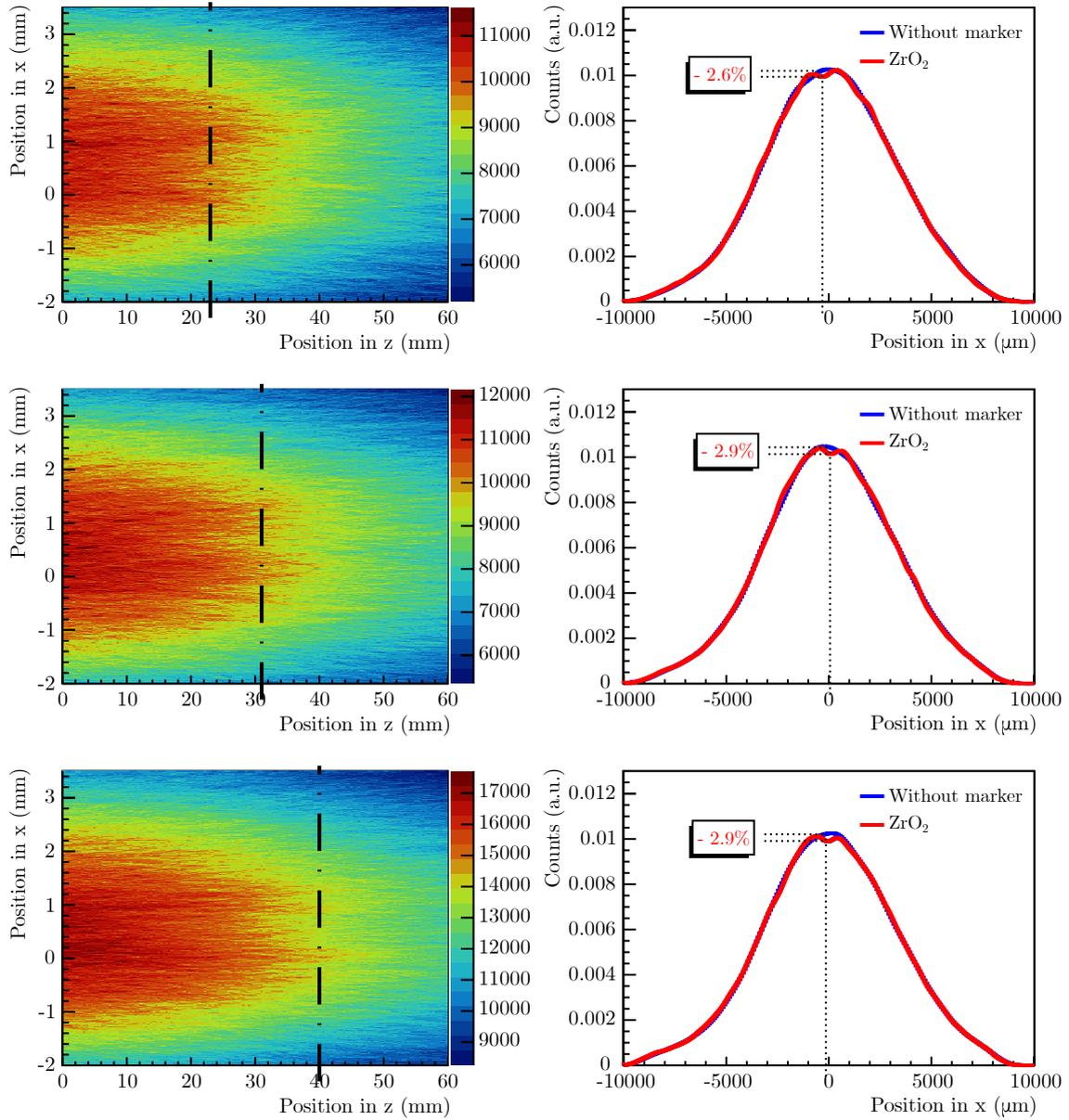
Figure 4.20: Reconstructed fluence maps and beam profiles of carbon ions at three different energies through the carbon-coated  $\text{ZrO}_2$  marker placed at position zero in  $(x,z)$  coordinates. The panels description is the same as Figure 4.18.
