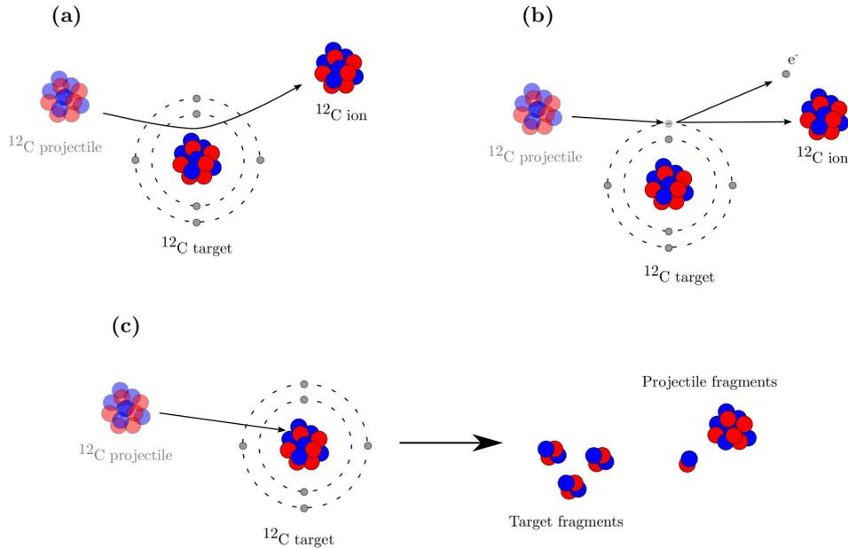
Figure 1.3: Interaction mechanisms relevant for particle therapy with the example of a  $^{12}\text{C}$  projectile interacting with a  $^{12}\text{C}$  target. The elastic and inelastic Coulomb interactions are represented in panels (a) and (b), while the inelastic nuclear interaction is illustrated in panel (c). Figure inspired by [42].
