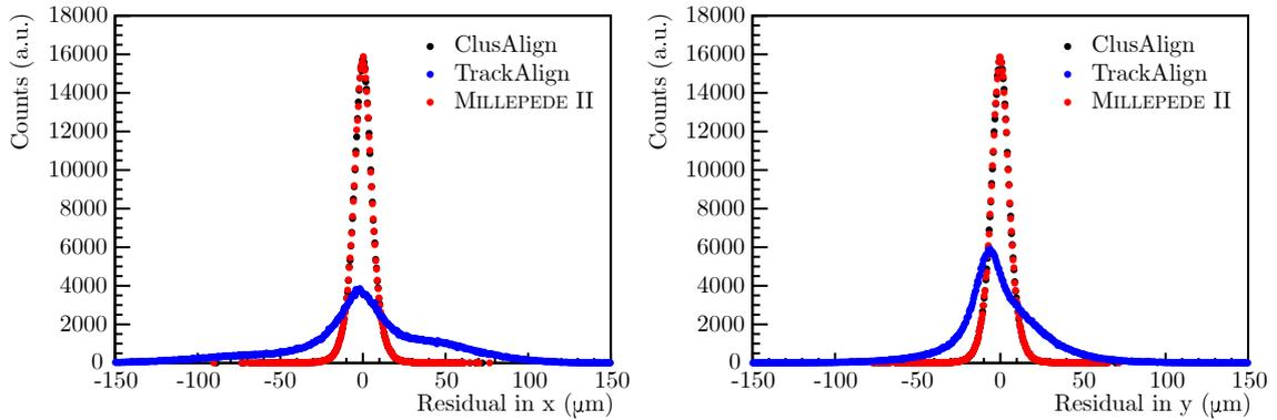
Figure 4.4: Histograms of the residuals in  $x$  (left panel) and  $y$  (right panel) after the alignment procedure with ClusAlign (black dots), TrackAlign (blue dots) and MILLEPEDE II (red dots) for 220.51 MeV/u  $^4\text{He}$  ions (from the experimental data recorded at HIT), for all sensors and all tracks.
