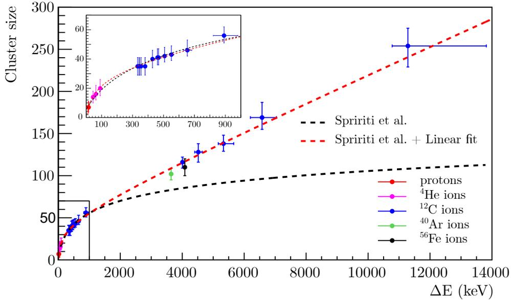
Figure 4.6: Measured cluster size as a function of the deposited energy in the active silicon layer of Mimosa-28.
