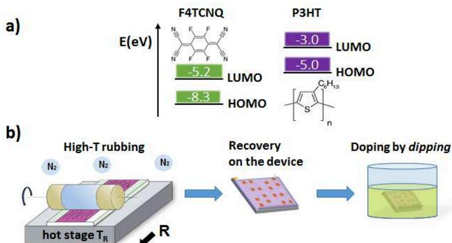
**Figure 1:** a) Chemical structures and schematic energy diagram of F<sub>4</sub>TCNQ and P3HT. b) Preparation method of in-plane oriented and conducting polymer films. First of all, chain alignment and crystallization of the P3HT films are generated by high-temperature rubbing (R is the rubbing direction). Thin oriented films are floated on distilled water and recovered on glass substrates with gold electrodes and doped by dipping into the solution of F<sub>4</sub>TCNQ in acetonitrile (AcN).
