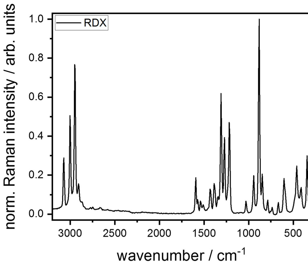
**Figure 4.14.** Raman spectrum of RDX in a spectral range between 3200 cm<sup>-1</sup> and 300 cm<sup>-1</sup>.
