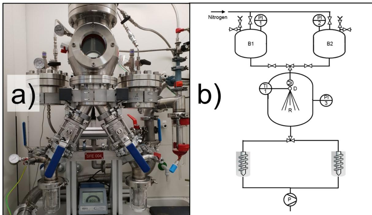
**Figure 4.1.** a) Photograph of a medium sized vertical SFE - reactor. b) Flow-chart of SFE setup. Final product is collected with axial cyclones (marked in grey). B1, B2: solvent and solution tank; R: reaction chamber; D: hollow cone nozzle, P: vacuum pump; PI: pressure sensor; TIC: temperature sensor.
