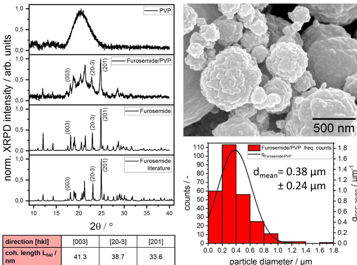
**Figure 5.2.** Left: XRPD pattern of Furosemide and PVP precursors, Furosemide/PVP sub-micron particles and a reference XRD pattern of Furosemide. The coherence lengths derived from the XRPD pattern of Furosemide/PVP indicates the formation of nano-structured Furosemide crystals. Right: SEM image of Furosemide/PVP particles characterized by a rough cauliflower-like surface. Furosemide/PVP particles provide a mean size of  $0.38 \mu\text{m}$  ( $\pm 0.24 \mu\text{m}$ ).
