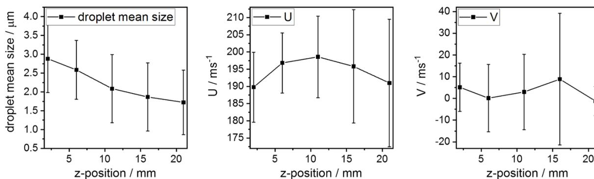
**Figure 4.19.** Left: Evolution of the droplet mean size as a function of the distance from the nozzle. Middle: Axial velocity U as a function as a function of the distance from the nozzle. Right: Axial velocity U as a function as a function of the distance from the nozzle.
