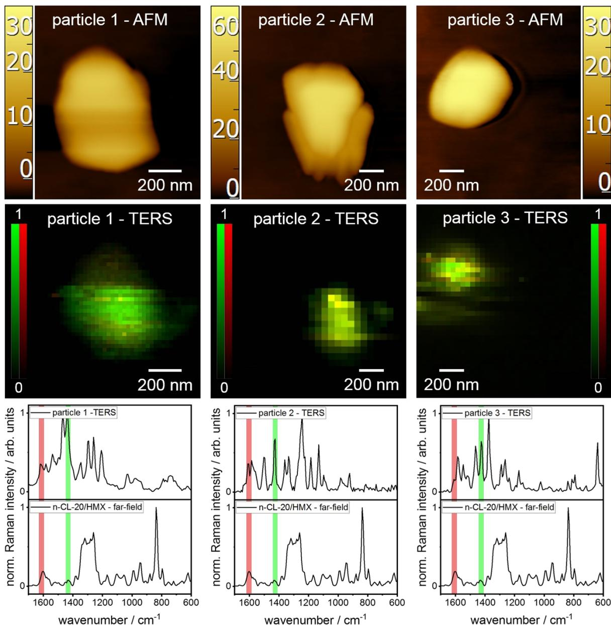
**Figure 3.10.** AFM topography images, TERS maps and corresponding spectra of n-CL-20/HMX nano-plates. TERS spectra represent the average over all TERS spectra on the particle surfaces. At all measured surface areas an intensity inversion between CL-20 and HMX marker bands occur. TERS maps and TERS spectra are normalized for better comparability. AFM topography images were recorded after TERS mapping. **Step sizes:** particle\_1 20 nm, particle\_2 and particle\_3 50 nm.
