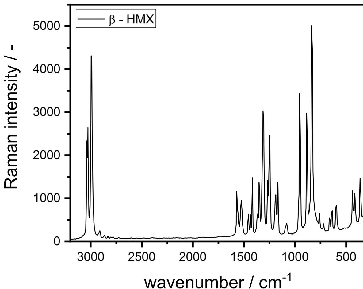
Figure 3.17. Raman spectrum of  $\beta$ -HMX in a spectral range between 3200 cm<sup>-1</sup> and 300 cm<sup>-1</sup>.
