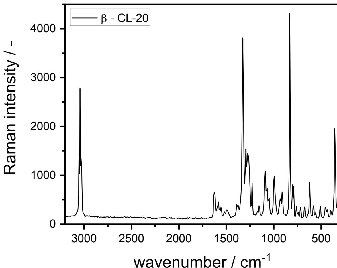
Figure 3.15. Raman spectrum of  $\beta$ -CL-20 in a spectral range between 3200 cm<sup>-1</sup> and 300 cm<sup>-1</sup>.
