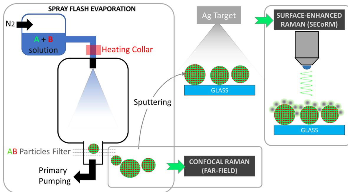
**Figure 5.1.** Schematic representation of the performed experiments. Furosemide/PVP sub-micron composites are produced by the Spray Flash Evaporation process. The structure of these particles is evaluated by comparing the results of bulk-sensitive confocal far-field Raman microscopy and surface-sensitive surface enhanced confocal Raman microscopy (SECoRM).
