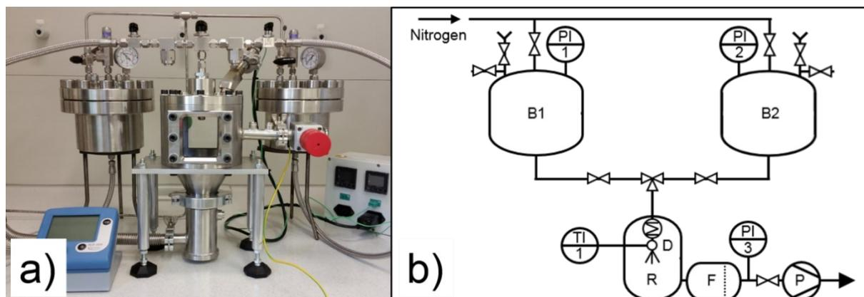
**Figure 3.1.** a) Photography of a lab version SFE - reactor. b) Flow-chart of SFE setup. B1, B2: solvent and solution tank; R: reaction chamber; D: hollow cone nozzle, F: filter, P: vacuum pump; PI: pressure sensor; TI: temperature sensor.
