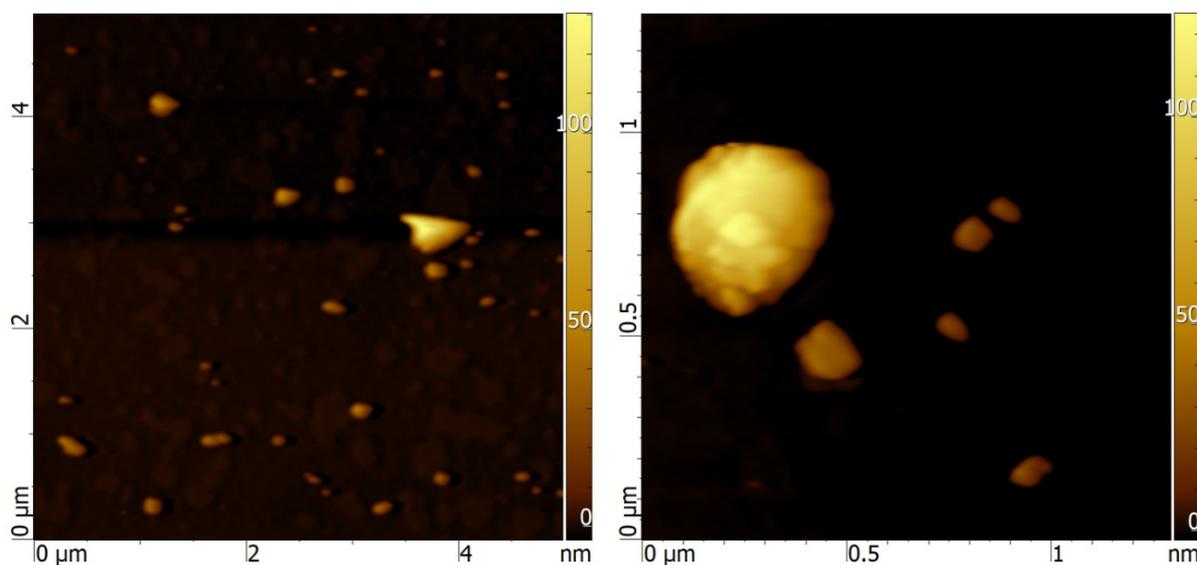
**Figure 3.13.** Left: AFM topographic mappings of several n-CL-20/HMX nano-plates. Single nano-plates show a height of ~30 nm. n-CL-20/HMX nano-plates built up agglomerates along their crystallographic bc-planes. Right: Single n-CL-20/HMX nano-plates and a CL-20/HMX nano-plate agglomerate.
