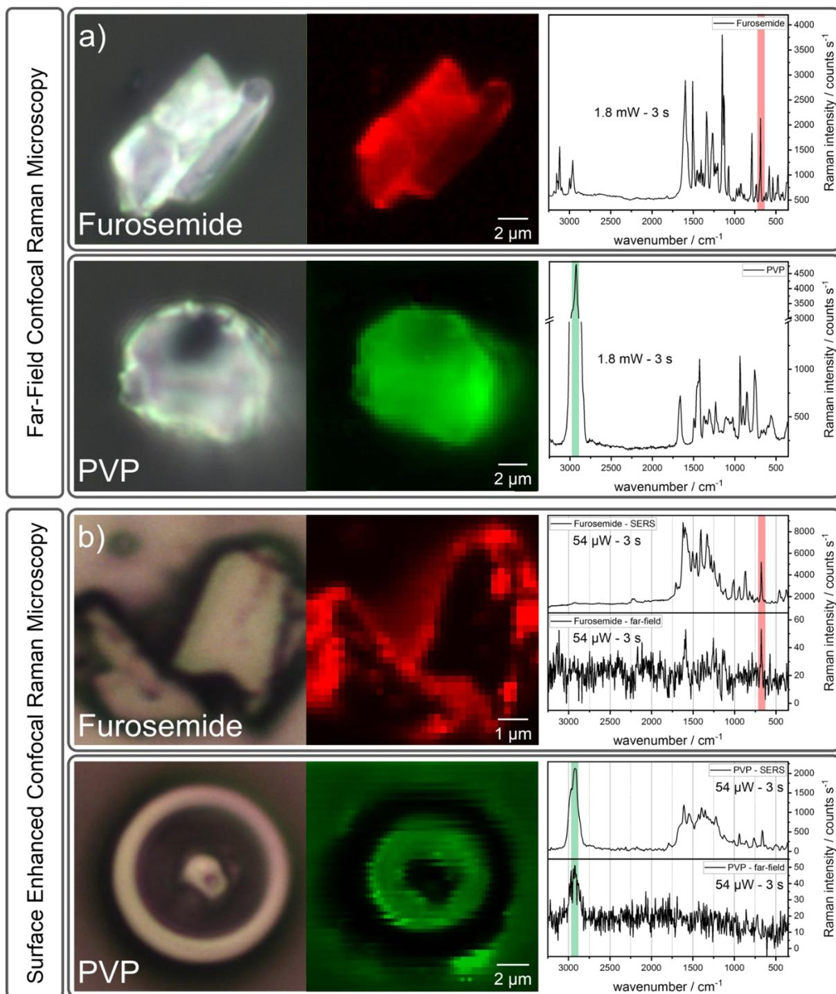
**Figure 5.3.a)** Optical microscopy images and the corresponding far-field Raman maps and spectra for pure Furosemide and PVP. The in-plane ring bending vibration localized at 686 cm<sup>-1</sup> (red) is chosen as marker band for Furosemide and the CH<sub>2</sub> asymmetric stretching vibrations of PVP at 2924 cm<sup>-1</sup> (green) is selected for PVP identification. **b)** SCoRM maps and SERS spectra of silver coated Furosemide and PVP showing the presence of the chosen marker bands.
