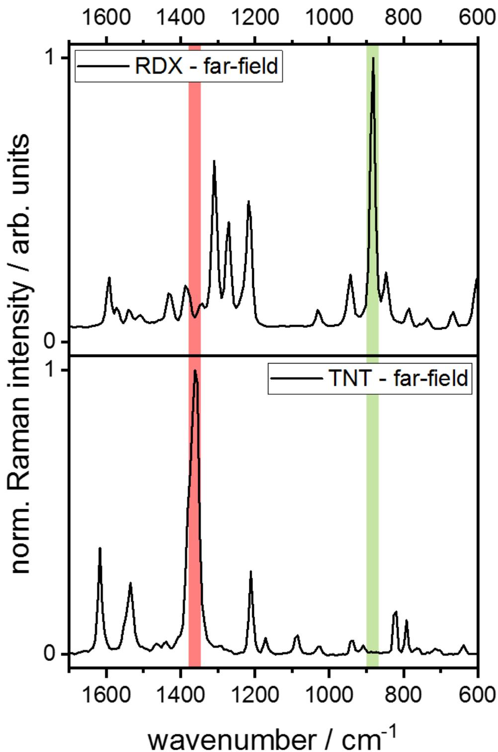
**Figure 4.3.** Far-field Raman spectra of RDX and TNT nanoparticles in the range between 1700  $\text{cm}^{-1}$  and 600  $\text{cm}^{-1}$ . The RDX marker band (882  $\text{cm}^{-1}$ ; ring breathing) is highlighted in green. The TNT marker band (1358  $\text{cm}^{-1}$  - 1371  $\text{cm}^{-1}$ ; three  $\text{NO}_2$  symmetric stretching vibrations) is marked in red.
