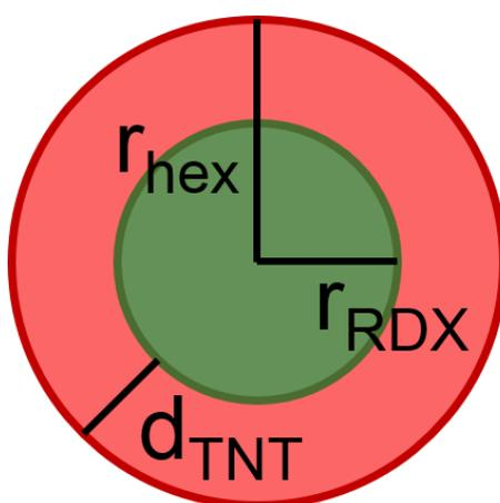
**Figure 4.20.** Schematic representation of an isotropic hexolite RDX/TNT core/shell nanoparticle;  $r_{hex}$  gives the particle radius,  $r_{RDX}$  represents the radius of the RDX core and  $d_{TNT}$  the TNT shell thickness.
