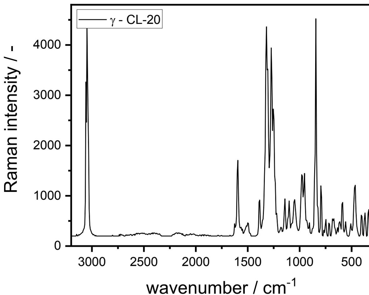
Figure 3.16. Raman spectrum of  $\gamma$ -CL-20 in a spectral range between 3200 cm<sup>-1</sup> and 300 cm<sup>-1</sup>.
