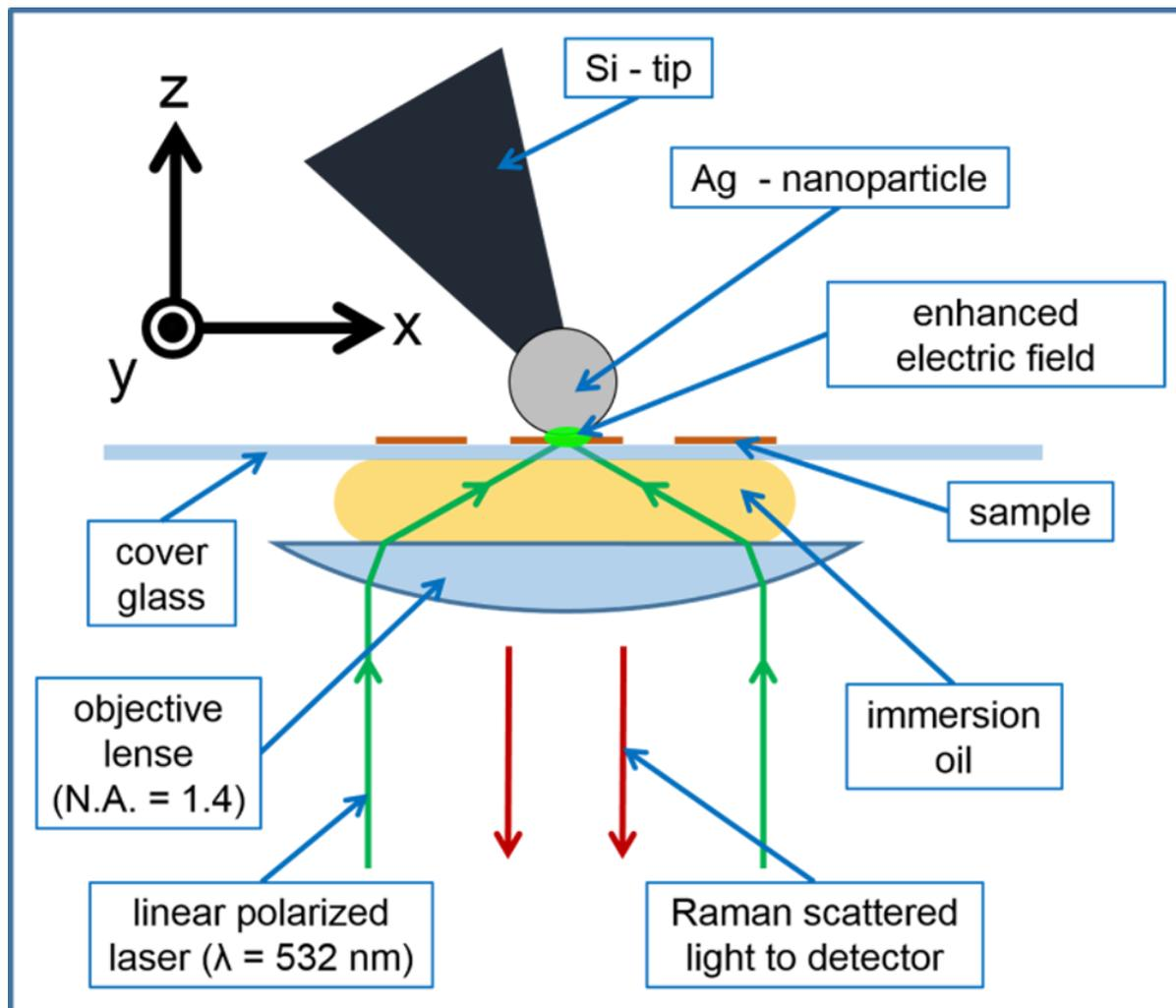
Figure 3.3. Schematic representation of the experimental setup.
