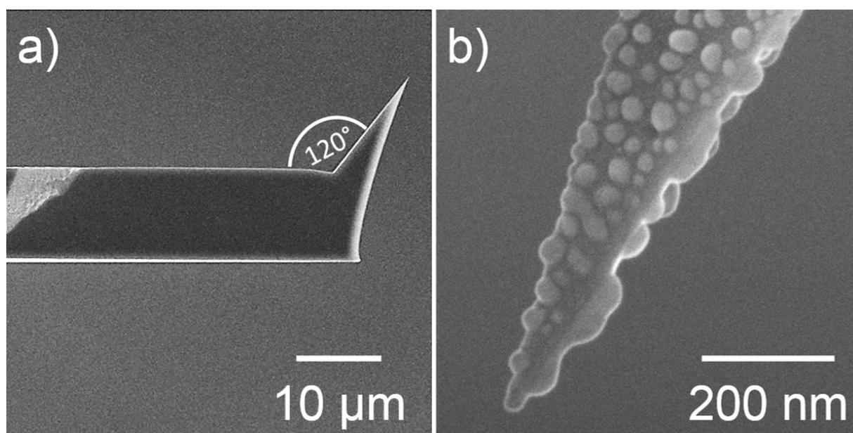
**Figure 4.2.** a) Pristine AppNano Access-NC AFM probe. The tip is mounted onto the cantilever at an angle of  $120^\circ$ . b) Si – tip sputtered with a 5 nm layer of Ti and a 25 nm layer of Ag. After the sputtering process the tips were annealed in a muffle furnace.
