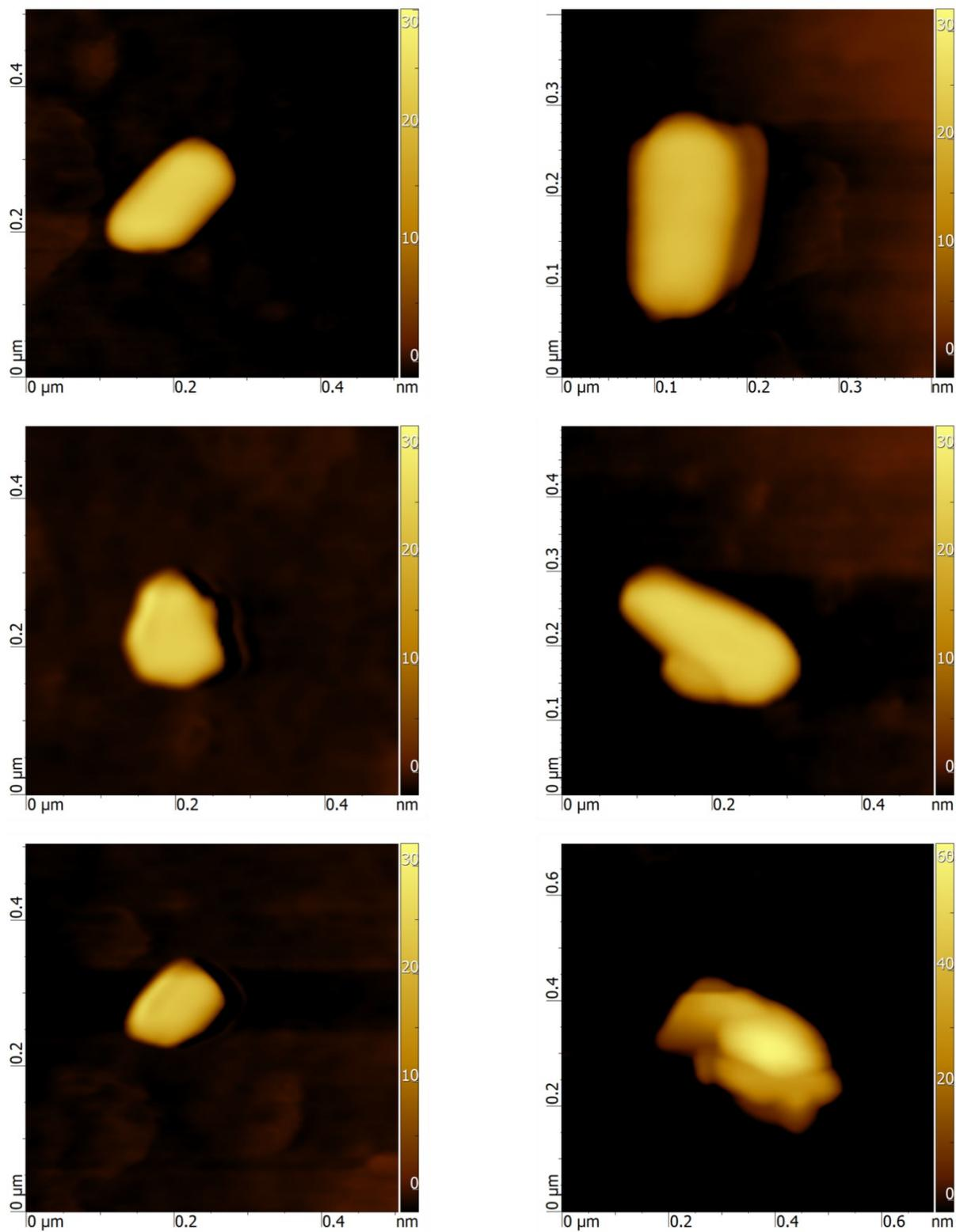
**Figure 3.14.** Selection of single and agglomerated n-CL-20/HMX nano-plates.
