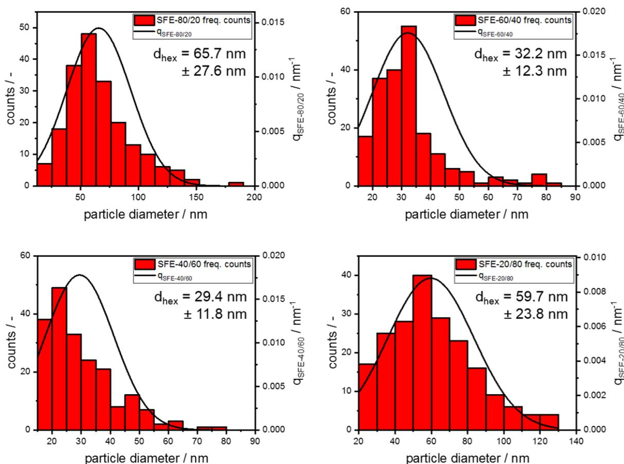
Figure 4.16. Size distribution of SFE-produced hexolite nanoparticles.
