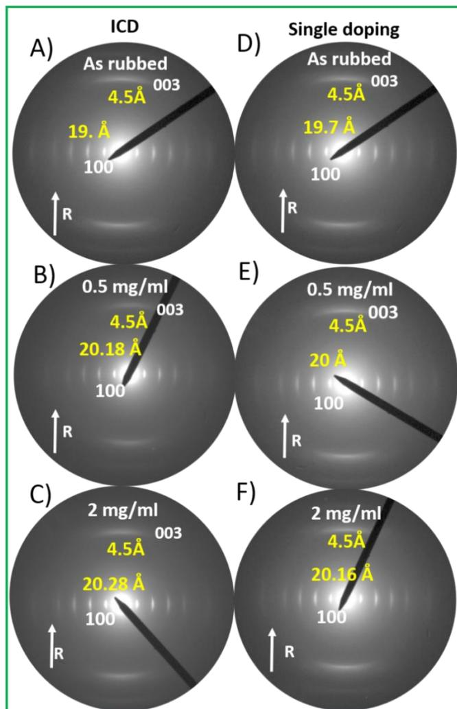
**Figure 4.13.** Evolution of the electron diffraction patterns of F<sub>6</sub>TCNNQ doped C<sub>12</sub>-PBTTT (A-C) sequential addition (D-F) single doping as a function of dopant concentration represent the rubbing direction
