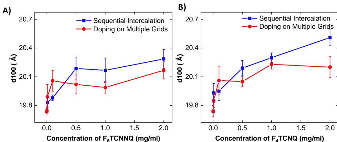
**Figure 4.14.** Evolution of  $d_{100}$  spacing of the sequentially and directly doped C<sub>12</sub>-PBTTT. A) Variation of  $d_{100}$  spacing of sequentially and singly doped F<sub>6</sub>TCNNQ/C<sub>12</sub>-PBTTT. A) Variation of  $d_{100}$  spacing of sequentially and singly doped F<sub>4</sub>TCNQ/C<sub>12</sub>-PBTTT
