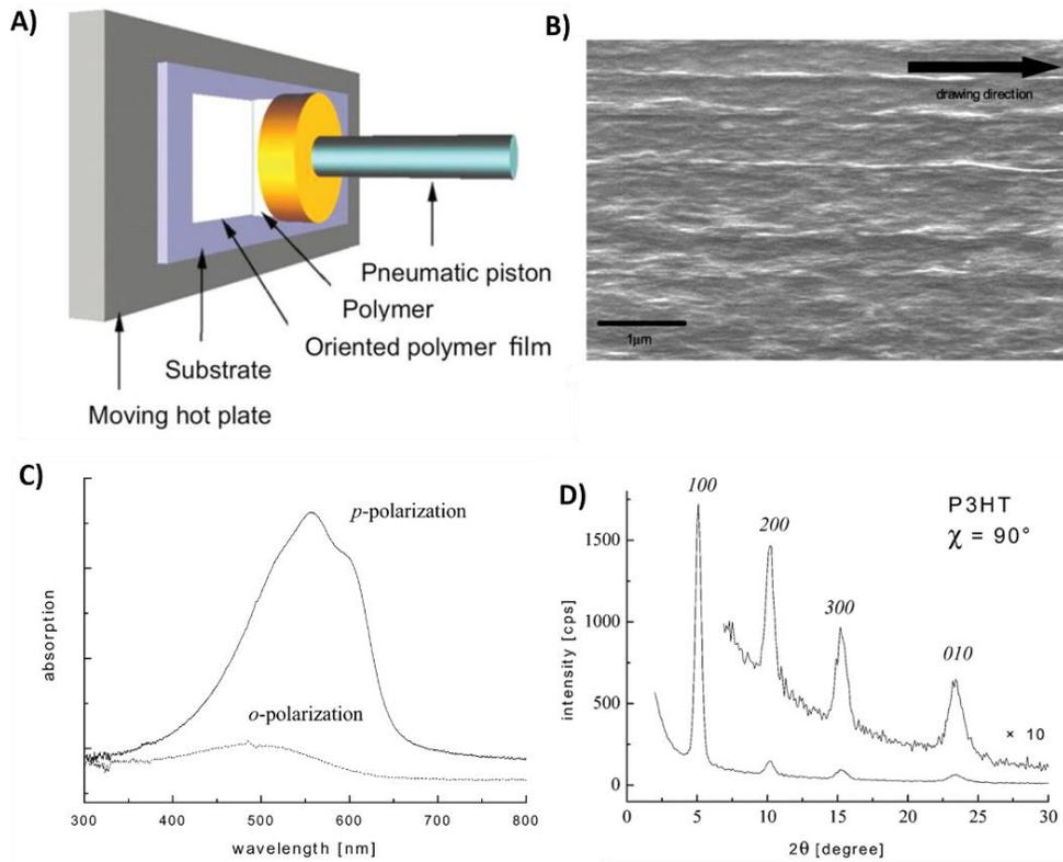
**Figure 1.17.** A) Schematic representation of the friction transfer deposition method. B) SEM image of an aligned P3HT film-oriented by friction transfer. C) and D) represent corresponding polarized Uv-Vis spectra along the parallel and perpendicular direction and the section profile from Grazing incidence X-ray diffraction respectively. Reproduced from (49&50)
