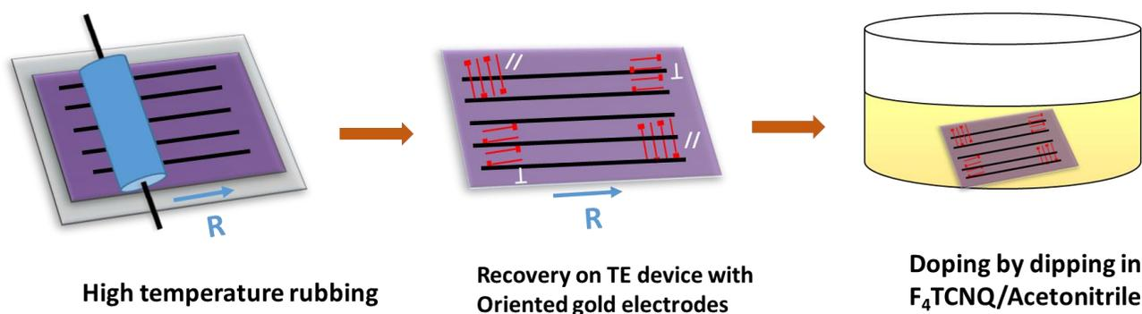
**Figure 4.** Schematic representation of high temperature rubbing and recovery of oriented thin films on patterned devices with oriented electrodes // and  $\perp$  to the rubbing direction. The TE device is dipped in the corresponding dopant solution for successful doping.
