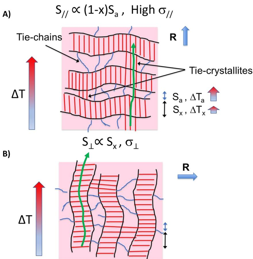
**Figure 3.9.** Schematic representation for the observed differences in the Seebeck coefficient of oriented polymer films. A) When the rubbing direction is // to the applied temperature gradient and B) Rubbing direction is perpendicular to the applied temperature gradient.
