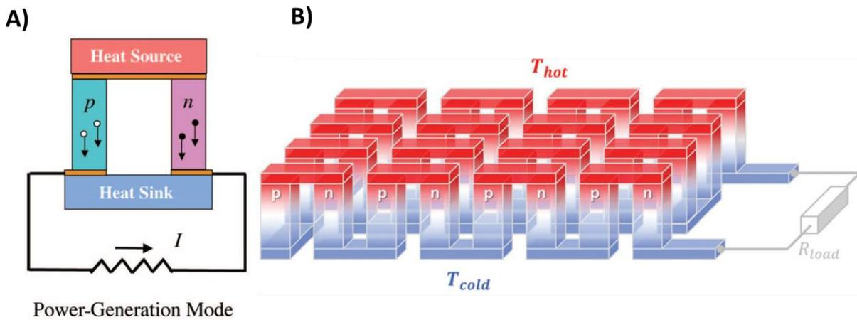
**Figure 1.21.** A) Diagram of a thermocouple made of n-type and p-type materials. Power generation or refrigeration modes are possible depending on the configuration.  $I$  is the current. B) A conventional thermoelectric module that comprises an array of elements, which are connected electrically in series but thermally in parallel. Reproduced from (3&66)
