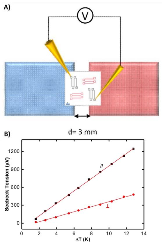
**Figure 5.** Schematic illustration of the experimental setup used for measuring the Seebeck coefficient of oriented PBTTT thin films along the direction parallel and perpendicular to the rubbing direction. The two curves represent the Seebeck coefficients measured along the parallel (black) and perpendicular (red) directions. Figure 4A is reproduced from reference 9.
