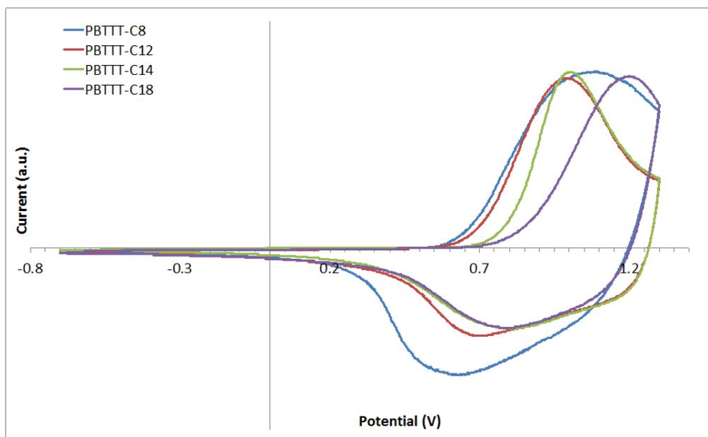
**Figure 2.7.** Cyclic voltammograms, in the anodic region, of PBTTT thin-films in ACN containing 0.1 M tetra-*n*-butylammonium hexafluorophosphate at 20 °C; scan rate 100 mVs<sup>-1</sup>. All peaks were calibrated against ferrocene (Fc<sup>+</sup>/Fc) at E<sub>1/2</sub> = 0.41 V vs SCE.
