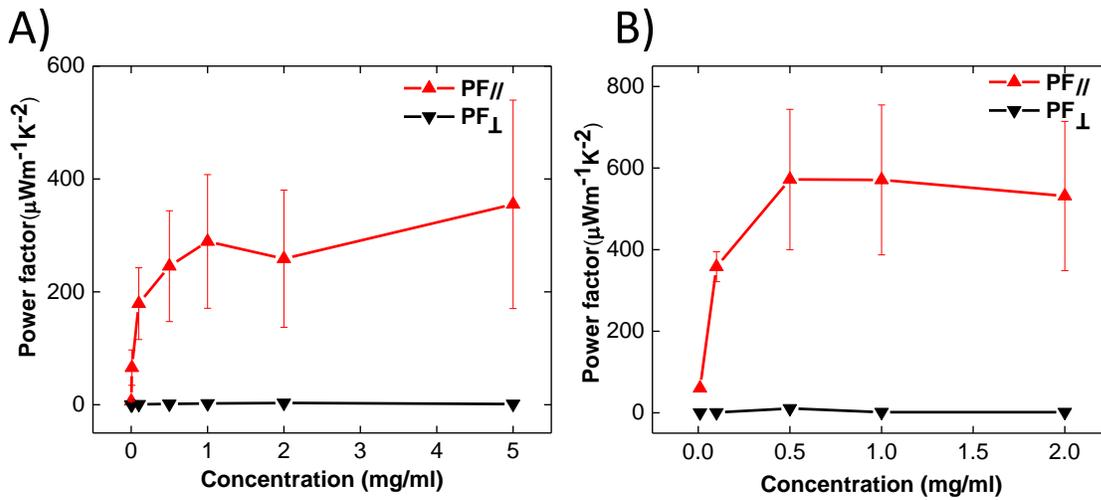
**Figure 4.10.** Evolution of the power factor as a function of increasing doping concentration of A) F<sub>4</sub>TCNQ and B) F<sub>6</sub>TCNNQ doped films of C<sub>12</sub>-PBTBT. Films were oriented by high temperature rubbing at 125°C and doped by incremental increase of doping concentration.
