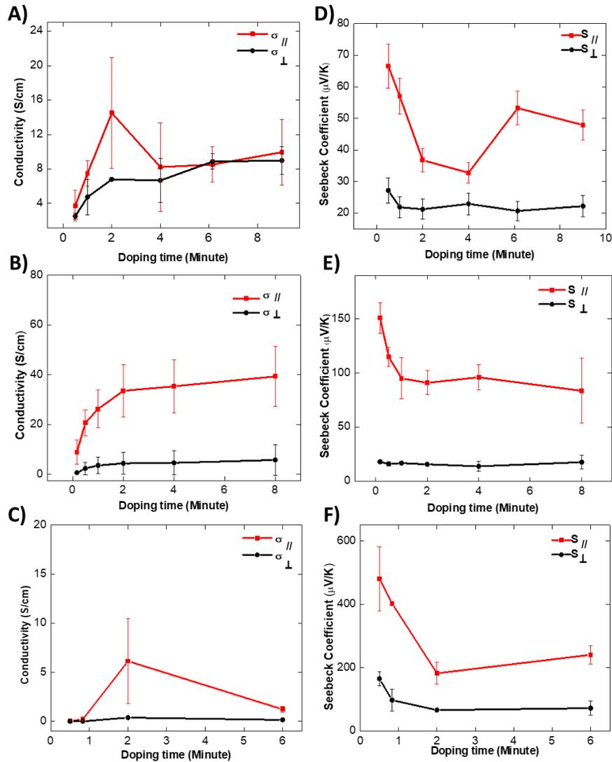
**Figure 2.15.** (A-C) Evolution of the charge conductivity versus doping time for  $C_8$ -PBTTT,  $C_{14}$ -PBTTT and  $C_{18}$ -PBTTT respectively. (D-F) Evolution of the Seebeck coefficient versus doping time for  $C_8$ -PBTTT,  $C_{14}$ -PBTTT and  $C_{18}$ -PBTTT respectively. All values are measured along the directions parallel (//) and perpendicular ( $\perp$ ) to the rubbing.
