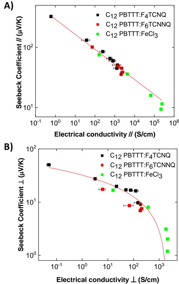
**Figure 4.11.** Correlation between Seebeck coefficient  $S$  and electrical conductivity  $\sigma$  in highly oriented thin films of C<sub>12</sub>-PBTTT ( $T_R=125^\circ\text{C}$ ) doped with F<sub>4</sub>TCNQ (black squares), F<sub>6</sub>TCNNQ (red squares) and FeCl<sub>3</sub> (green squares). The full lines correspond to the results of the fit using the scaling laws  $S_{//} \propto \sigma_{//}^{-1/4}$  and  $S_{\perp} \propto -\ln(\sigma_{\perp})$ .
