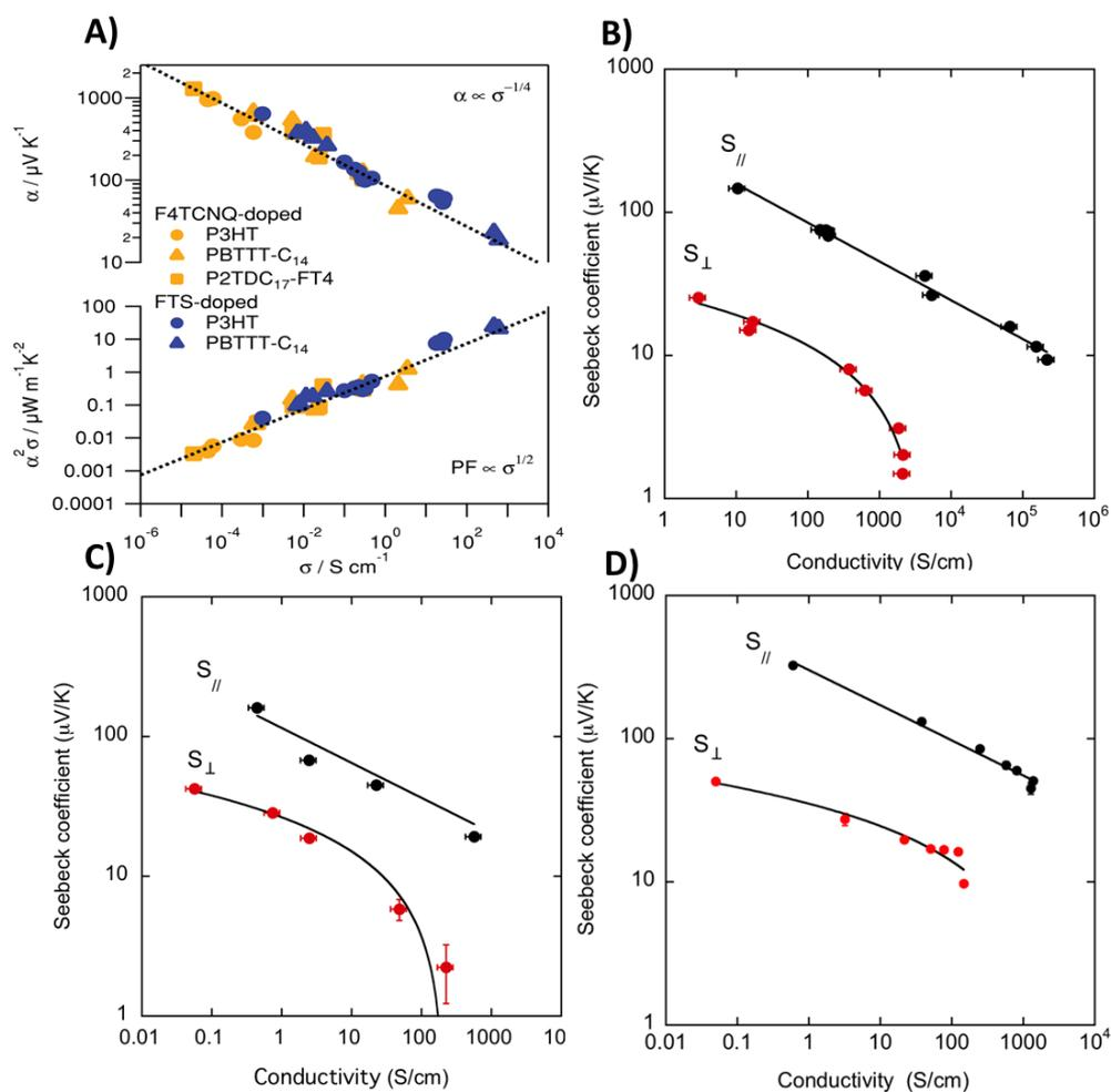
**Figure 3.8.** Correlation between thermopower  $S$  and charge conductivity. A)  $\text{F}_4\text{TCNQ}$  and FTS doped non-oriented films of PBTTT, P3HT,  $\text{P}_2\text{TDC}_{17}\text{-FT}_4$ , which follows the relation  $S_{\parallel} \propto \sigma^{-1/4}$ . B) Highly oriented thin films of  $\text{C}_{12}$ -PBTTT ( $T_R = 125^\circ\text{C}$ ) and C) P3HT ( $T_R = 180^\circ\text{C}$ ) doped with  $\text{FeCl}_3$ .  $\parallel$  and  $\perp$  refer to the direction of the measurements
