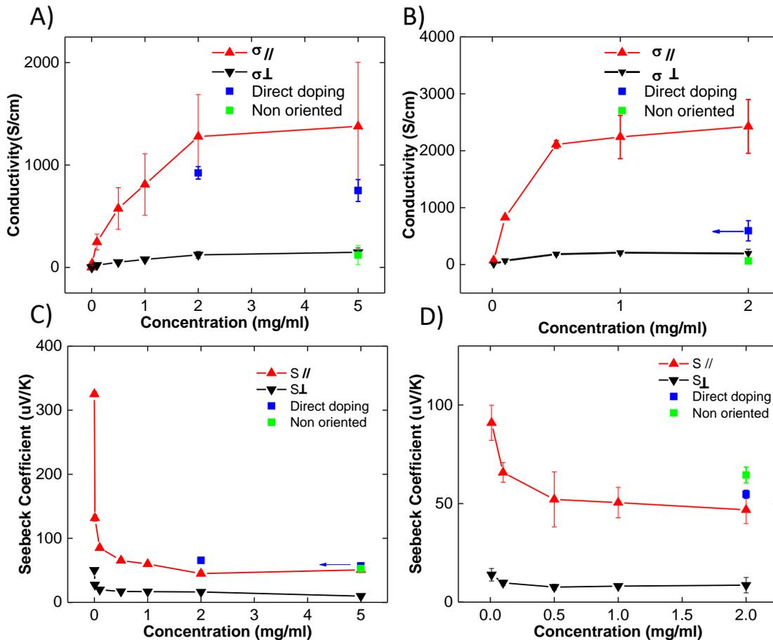
**Figure 4.8.** Evolution of the charge conductivity (A and B) and of the Seebeck coefficient (C and D) as a function of increasing doping concentration of F<sub>4</sub>TCNQ and F<sub>6</sub>TCNNQ in oriented films of C<sub>12</sub>-PBTTT, respectively. The curves correspond to the sample doped by incremental increase of doping concentration (ICD). Both S and  $\sigma$  are measured parallel (red) and perpendicular (black) to the rubbing directions. For comparison, we also show the
