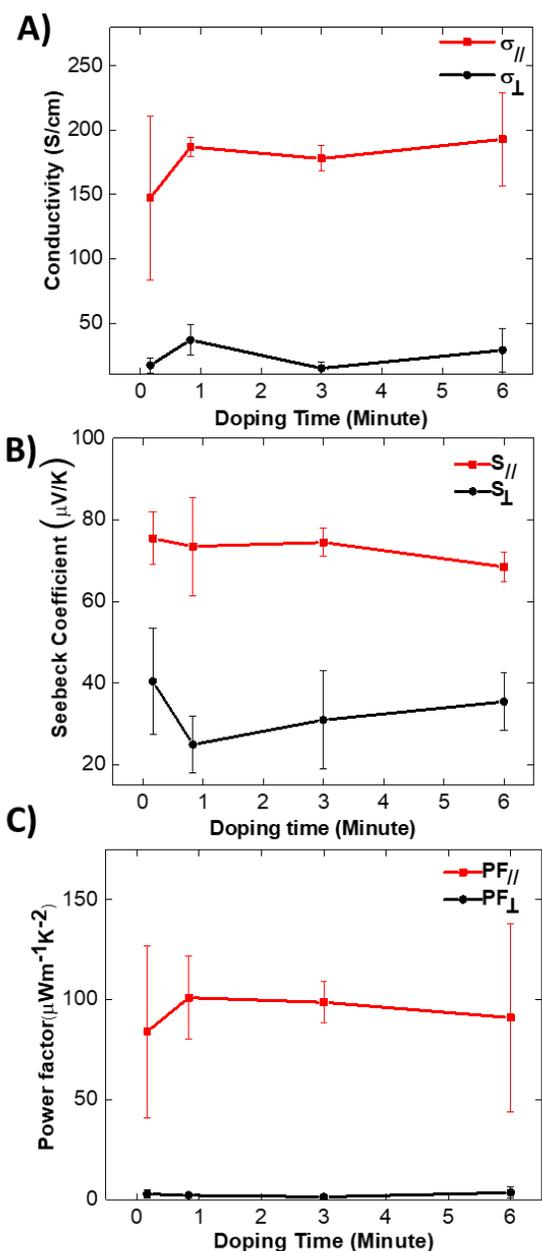
**Figure 2.13.** Evolution of the charge conductivity, Seebeck coefficient and power factor as a function of increasing doping concentration of  $F_4\text{TCNQ}$  for oriented thin films of  $C_{12}$ -PBTTT. All values are measured along the directions parallel ( $//$ ) and perpendicular ( $\perp$ ) to the rubbing.
