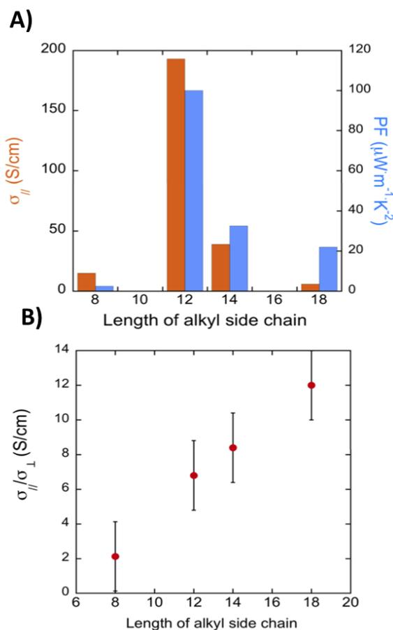
**Figure 2.16.** Evolution of the maximum conductivity ( $\sigma_{//}$ ) and power factor (PF) along the rubbing direction (a) and of the average charge conductivity anisotropy  $\sigma_{//}/\sigma_{\perp}$  (b) versus side chain length in F<sub>4</sub>TCNQ-doped PBTTT films oriented by high temperature rubbing.
