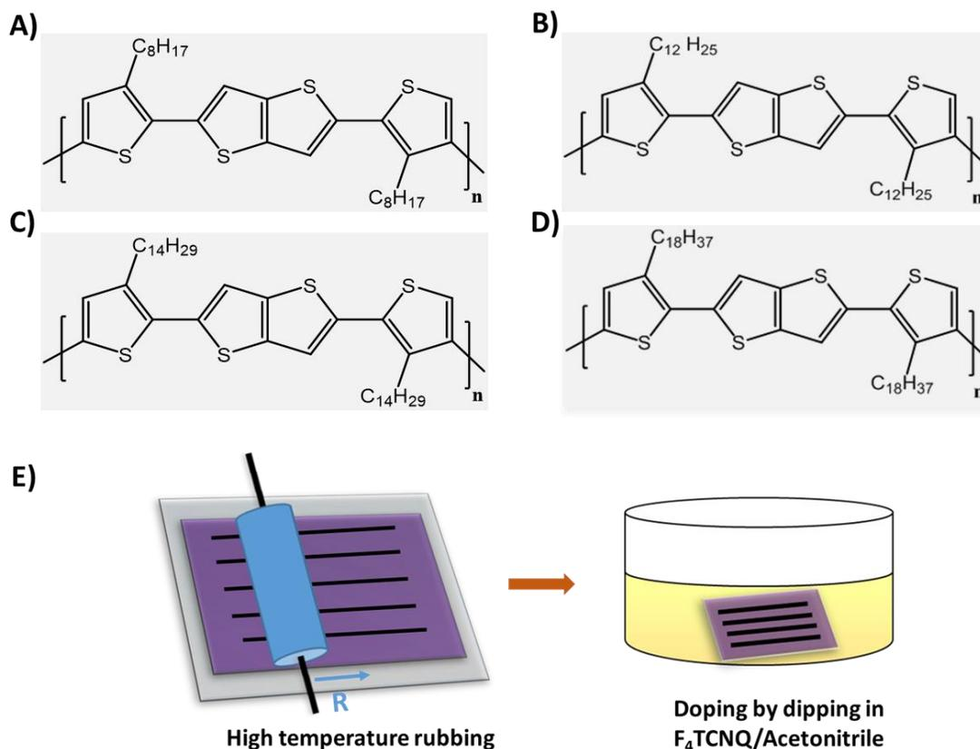
**Figure 2.1.** Chemical structures of A) C<sub>8</sub>-PBTTT B) C<sub>12</sub>-PBTTT C) C<sub>14</sub>-PBTTT and D) C<sub>18</sub>-PBTTT. E) Schematic illustration of high temperature rubbing and doping of PBTTT thin films by dipping in the dopant F<sub>4</sub>TCNQ solution in acetonitrile.
