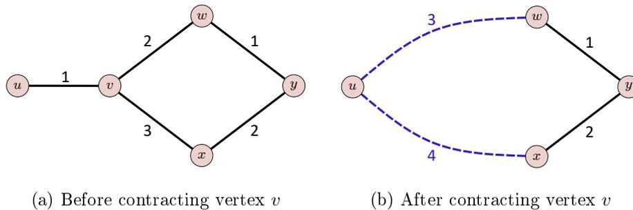
Figure 2.9: Contracting vertex  $v$ : two shortcut edges  $(u, w)$  and  $(u, x)$  are inserted. However, no shortcut is added between vertices  $w$  and  $x$  because  $(w, v, x)$  is not a shortest path.
