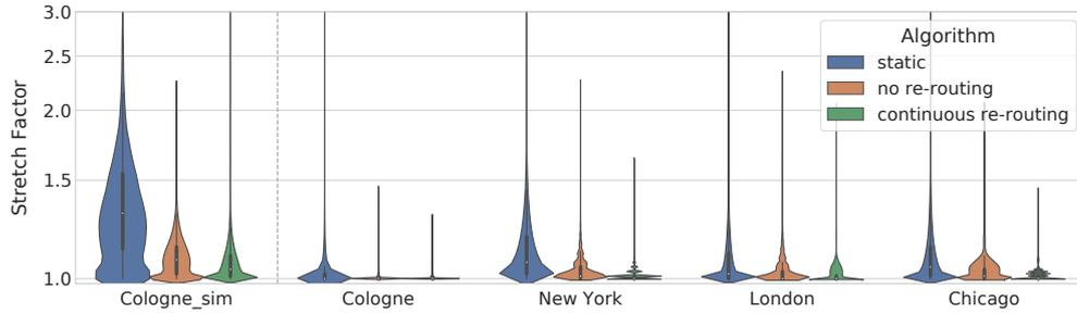
Figure 4.5: Stretch factor of the static, no re-routing and continuous re-routing algorithms on both the TAPAS (left) and the real (right) datasets.
