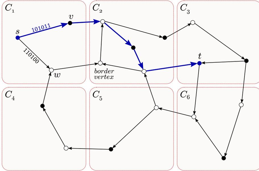
Figure 2.8: The graph is partitioned into six regions and their border vertices are outlined. The shortest  $st$  path is shown in bold blue edges. During the query, Arc Flags algorithm prunes edge  $(s, w)$  because the third bit-flag is not set.
