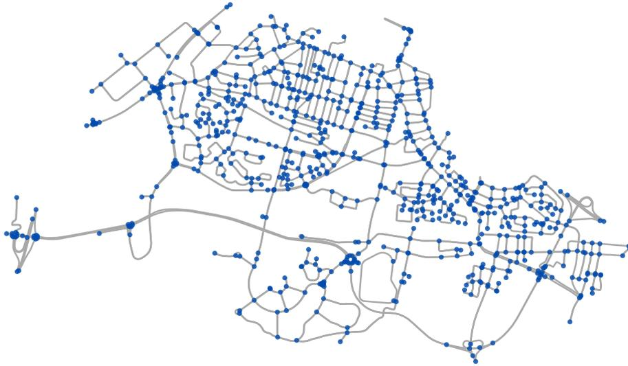
Figure 2.1: Graph representation of Illkirch's road network in Strasbourg, France. The dots are the graph's vertices and the segments are the edges, drawn to preserve the original shape of the road segments.
