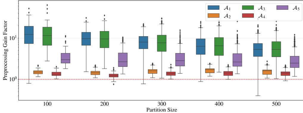
Figure 5.9: The preprocessing Gain Factor denoting the speedup of the many-to-many ( $lcD_{pRegLC}$ ) over the one-to-many ( $D_{pRegLC}$ ) strategy for each automaton and partition size. The horizontal red line corresponds to a gain of 1 and imply no speedup.
