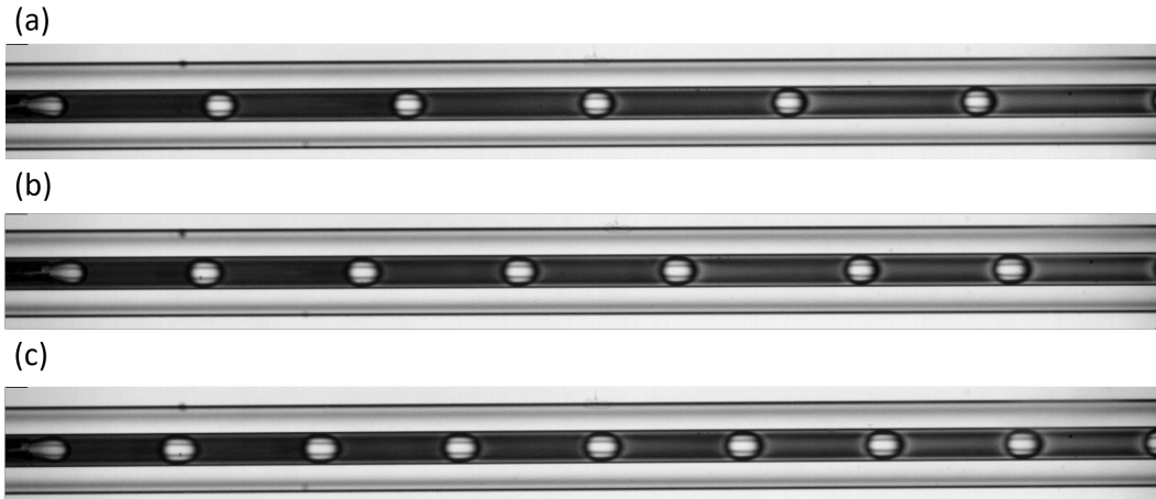
Figure E.7 – Images of two-phase segmented flow of CO_2 and H_2O at the first measurement spot for 10 MPa and 303 K where \dot{V}_{H_2O} = 350 \mu\text{L min}^{-1} : (a) \dot{V}_{CO_2} = 76.6 \mu\text{L min}^{-1} , (b) \dot{V}_{CO_2} = 94.2 \mu\text{L min}^{-1} and (c) \dot{V}_{CO_2} = 111.9 \mu\text{L min}^{-1} .
