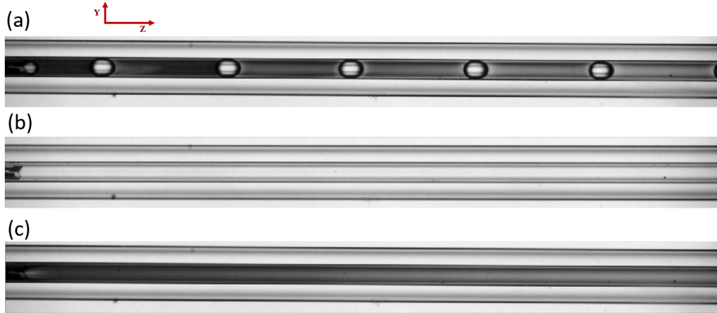
Figure 5.15 – (a) Image of a two-phase segmented flow of CO_2 + H_2O + BPB at 10 MPa and 303 K. (b) blank image in the bubble generation zone (spot 1). (c) Averaged image of the 1800 images taken in spot 1.
