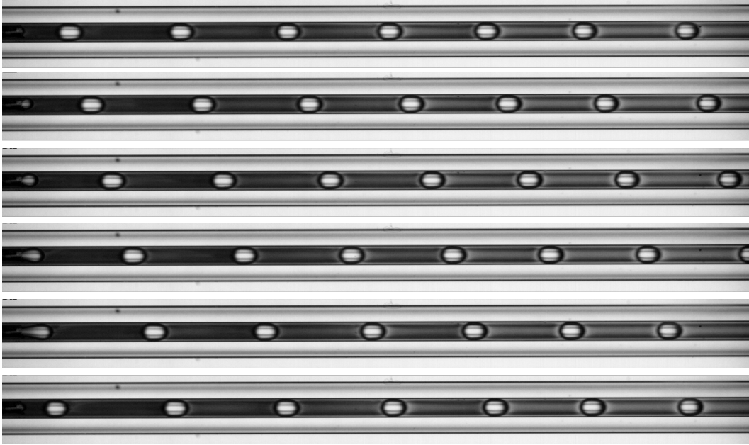
Figure E.9 – Images of a two-phase segmented flow evolution of CO_2 and H_2O at the first measurement spot for 10 MPa and 303 K where \dot{V}_{CO_2} = 82.5 \mu\text{L min}^{-1} and \dot{V}_{H_2O} = 300 \mu\text{L min}^{-1} (1/600 second between each image).
