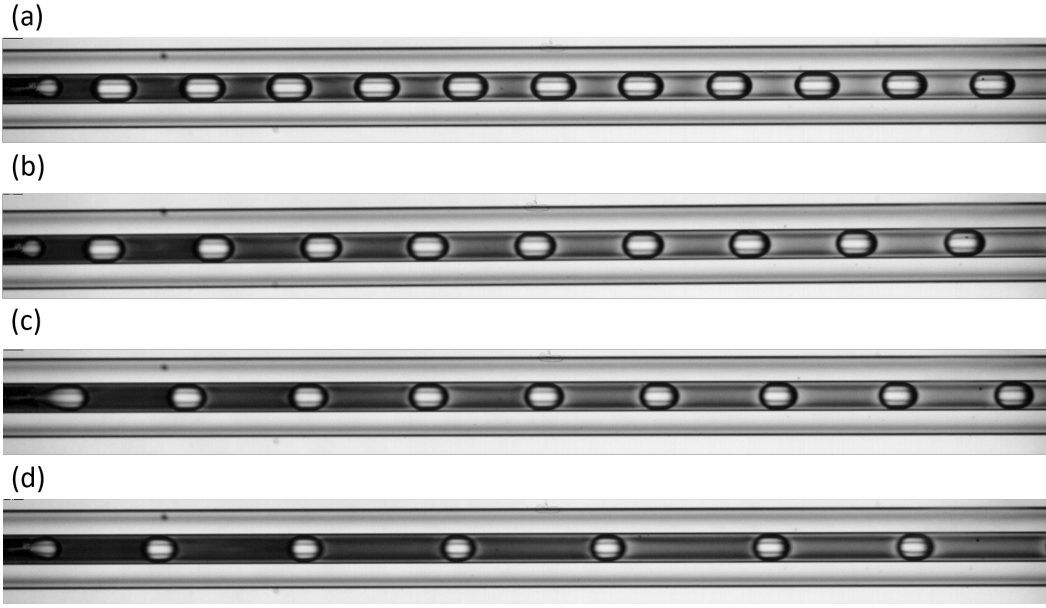
Figure E.8 – Images of two-phase segmented flow of CO_2 and H_2O at the first measurement spot for 10 MPa and 303 K where \dot{V}_{CO_2} = 82.5 \mu\text{L min}^{-1} : (a) \dot{V}_{H_2O} = 110 \mu\text{L min}^{-1} , (b) \dot{V}_{H_2O} = 150 \mu\text{L min}^{-1} , (c) \dot{V}_{H_2O} = 200 \mu\text{L min}^{-1} and (d) \dot{V}_{H_2O} = 300 \mu\text{L min}^{-1} .
