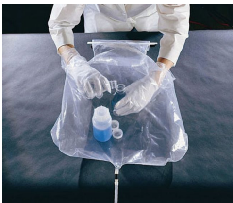
Fig 76. Picture of a glove bag from Cole-Parmer®
