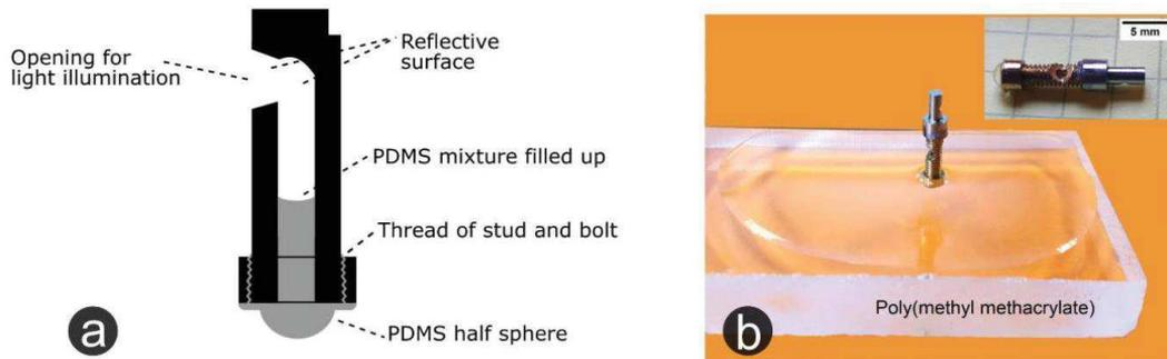
**Figure 2** Simplified sketch of the tip assembly (a) showing that the PDMS tip is embedded within the tip assembly holder. (b) A PDMS liquid mixture is filled up inside the hole due to capillary action, and a photograph of actual the PDMS tip attached to the tip holder (in up-right corner of image b).
