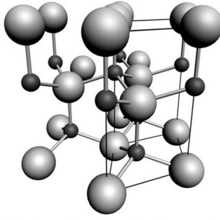
Figure 0.10.: Wurzite structure of ZnO. Zn atoms are represented by large gray spheres and O atoms by small black ones. Reprinted from (Jagadish & Pearton, 2011), Copyright (2011), with permission from Elsevier.
