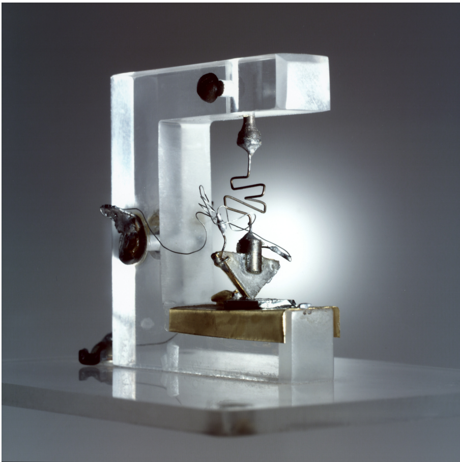
Figure 8: Picture of the first transistor ever assembled at Bell Labs in 1947.
