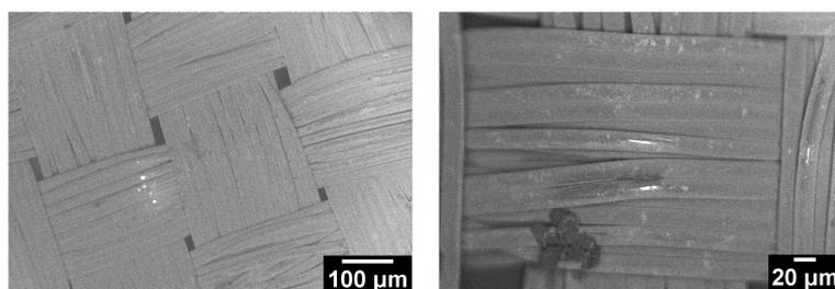
Appendix 14 : SEM images of PEI/PSS/TiO<sub>2</sub> film acquired with ESB detector equipped to the apparatus.
