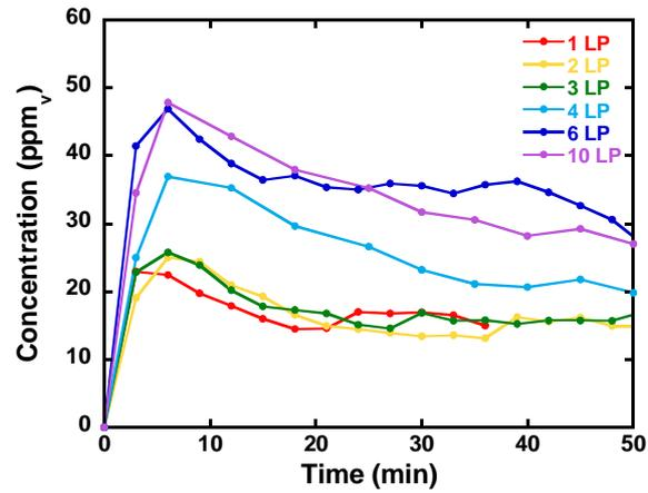
Appendix 5 : Evolution of CO<sub>2</sub> formation during photocatalysis tests without HCOOH
