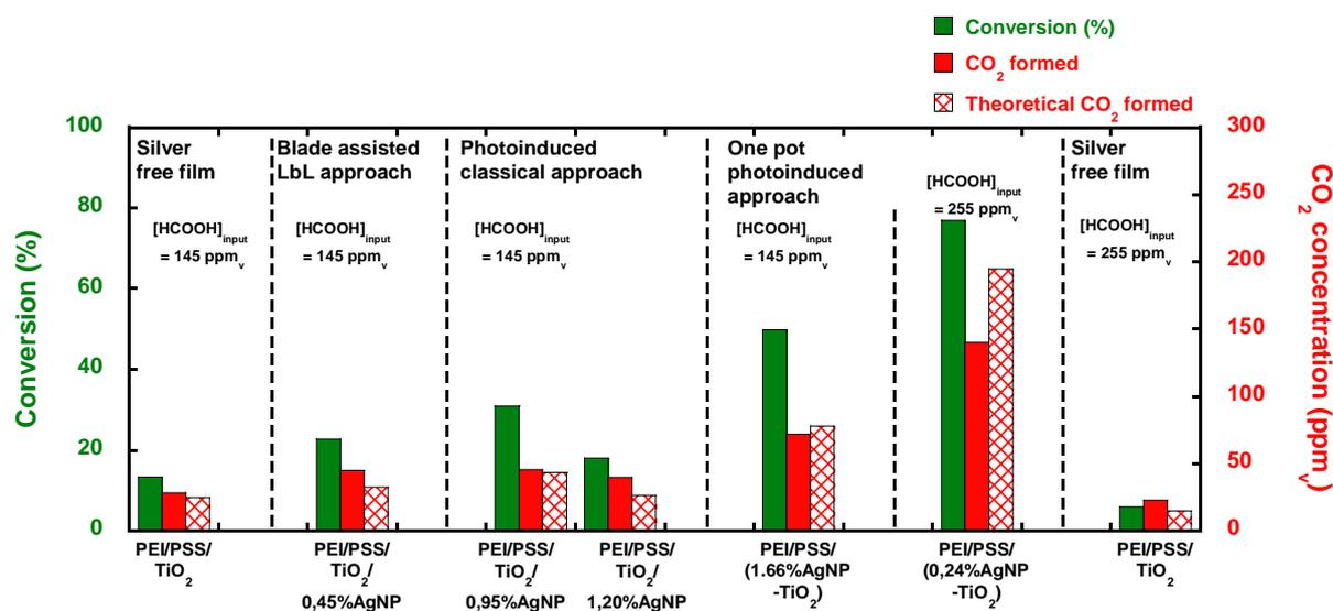
Figure 90: Comparison of the photocatalytic performances shown by Ag-TiO<sub>2</sub> films prepared via the three approaches.
