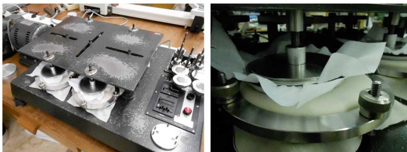
Figure 102 : (Left) Functionalised textiles placed against wool reps for abrasion test. (Right) zoom of the interface between the textile and the wool rep.
