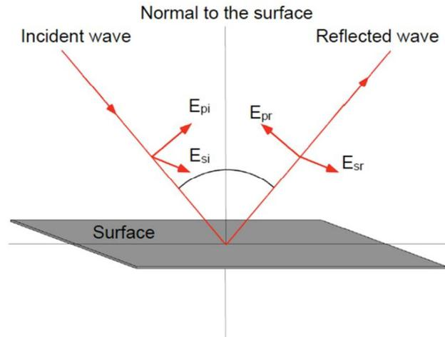
Figure 22: Schematic representation of an electromagnetic wave reflecting off a surface.
