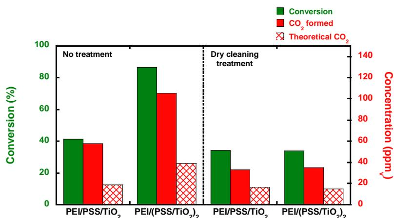
Figure 112 : Photocatalytic performances of functionalised textiles before and after dry cleaning treatment. Experimental parameters: [HCOOH] = 45 ppm<sub>v</sub>, air flow = 20 mL/min, speed = 0.7 cm/s, UV-A irradiance = 2.5 mW/cm<sup>2</sup>, films built on polyester textile.
