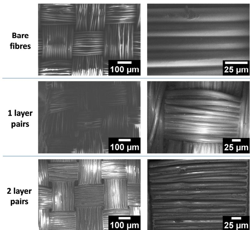
Figure 104: SEM images of textiles after abrasion test.
