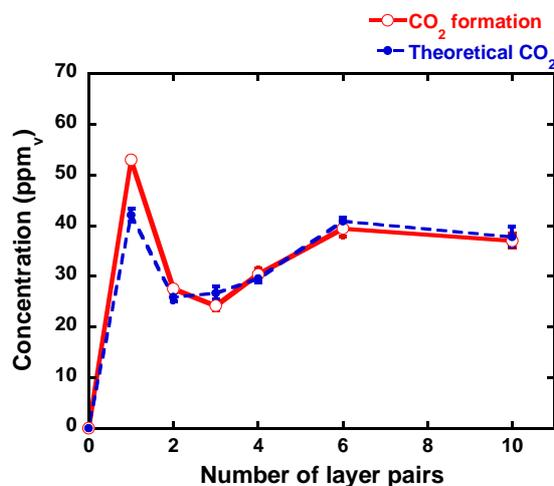
Figure 53: CO<sub>2</sub> formation on TiO<sub>2</sub> LbL films in regards to number of layer pairs during photocatalysis test with formic acid.
