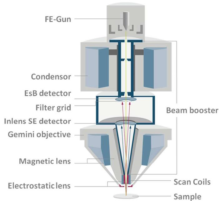
Figure 24 : Schematic cross-section of Gemini optical column with beam booster, Inlens detectors and Gemini objective ([www.zeiss.com](http://www.zeiss.com))
