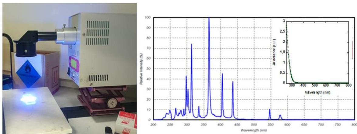
Figure 20: (Left) the UV lamp used in the photoinduced AgNP synthesis. (Right) irradiance spectra of UV lamp, with transmission UV-visible spectrum of a glass slide in the inset.
