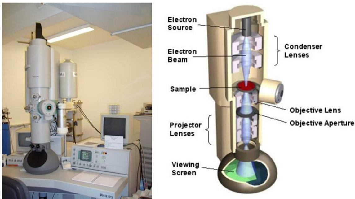
Figure 25: Picture of Philips CM200 TEM (left) and a schematic representation of TEM components (right).
