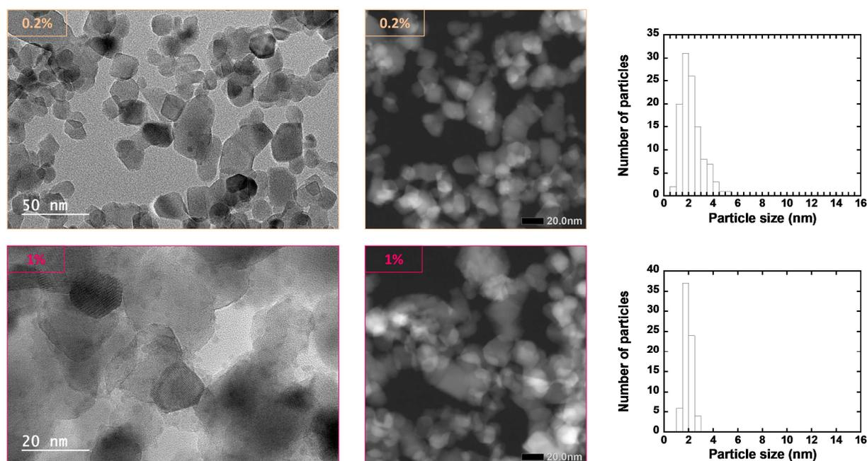
Figure 84 : TEM and STEM images of  $\text{PEI/PSS}/(0.2\%\text{Ag-TiO}_2)$  and  $\text{PEI/PSS}/(1\%\text{Ag-TiO}_2)$  films, with their particles counting assessed on STEM image ( $0.2\%\text{Ag-TiO}_2$ ) and TEM image ( $1\%\text{Ag-TiO}_2$ ).
