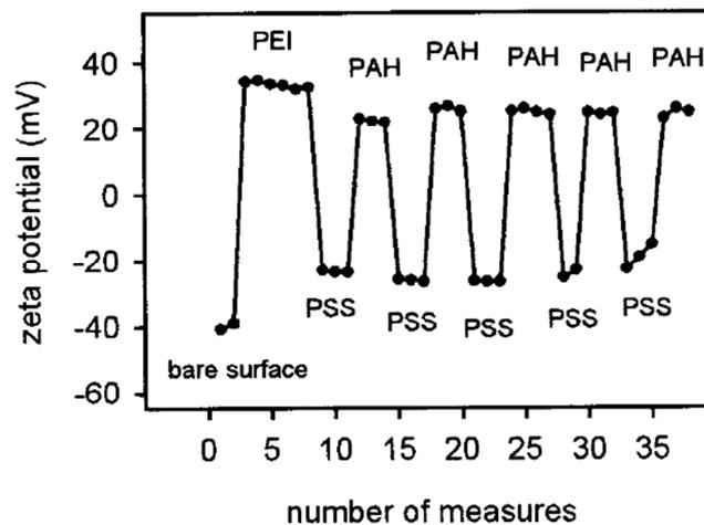
Figure 15: Zeta potential measurement of a PEI/(PSS/PAH)<sub>5</sub> film showing the inversion of charge during film construction [141].
