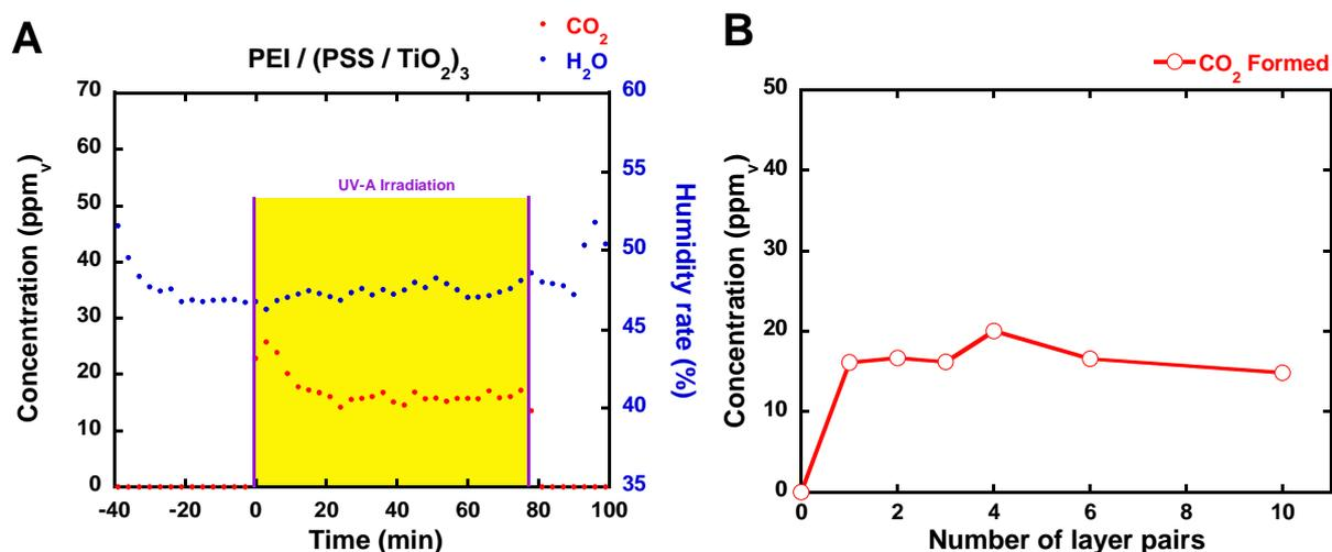
Figure 54: (A) Evolution of concentration curve for a 3 layer pairs LbL film; stabilisation is reached after 18 min. (B) Results of CO<sub>2</sub> concentration formed during UV-A irradiation in regards to the number of layer pairs deposited.
