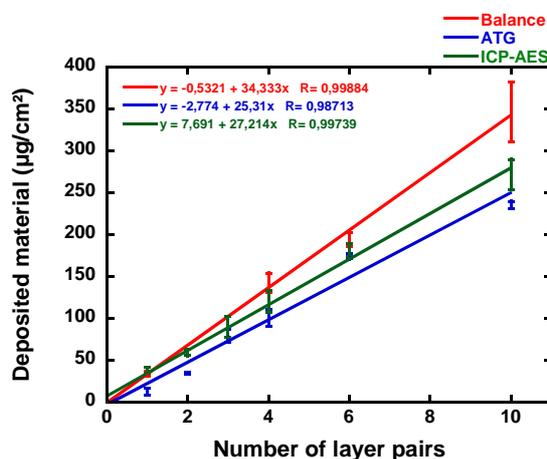
Figure 95 : Comparison of the amount of deposited material on textile surface using different characterisation methods.
