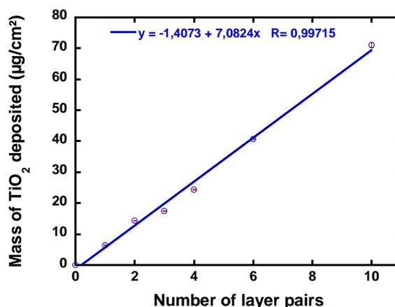
Figure 51: Mass of TiO<sub>2</sub> deposited investigated by chemical analysis ICP-AES. Error bars are too small to be clearly shown on the graph.
