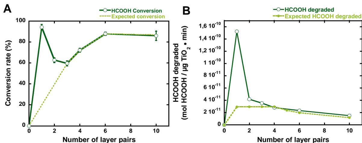
Figure 52: (A) Evolution of HCOOH conversion in regards to the number of layer pairs deposited in LbL films. (B) HCOOH degraded in mol per μg of TiO<sub>2</sub> per min in regards to the number of layer pairs. Experimental parameters: [HCOOH] = 45 ppm<sub>v</sub>, air flow = 20 mL/min, speed = 0.7 cm/s, UV-A irradiance = 2.5 mW/cm<sup>2</sup>, films built on 36 cm<sup>2</sup> silicon wafers.
