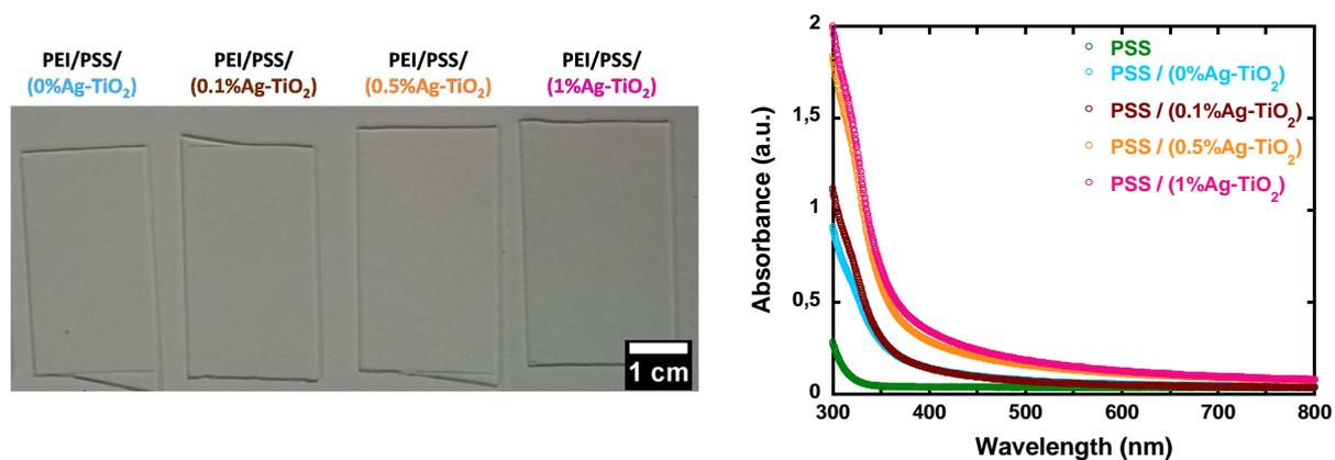
Figure 79 : Characterisations of PEI/PSS/(x%Ag-TiO<sub>2</sub>) film, with x = 0, 0.1, 0.5 and 1wt% AgNO<sub>3</sub>. (Left) Pictures of irradiated films constructed on glass slides. (Right) Transmission mode UV-Visible spectra of the films after being UV irradiated for AgNP one-pot synthesis.
