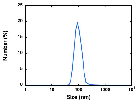
Figure 40 : Dynamic light scattering characterisation of the TiO<sub>2</sub> P25 suspension used for LbL films construction.
