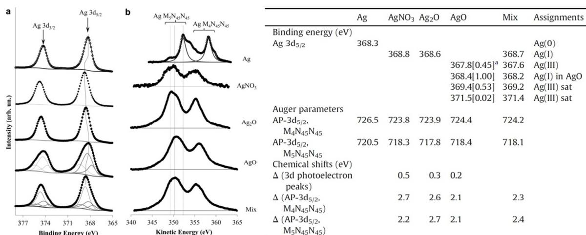
Figure 27 : Investigation on Auger parameters of different silver powders from Ferrara et al., "Mix" is a mechanical mixture of Ag<sub>2</sub>O and AgO [200]. (Left) XPS spectrum with binding energy of Ag 3d (a) and kinetic energy of Ag MNN (b). (Right) modified table results from XPS spectrum and Auger parameters with their assignments.
