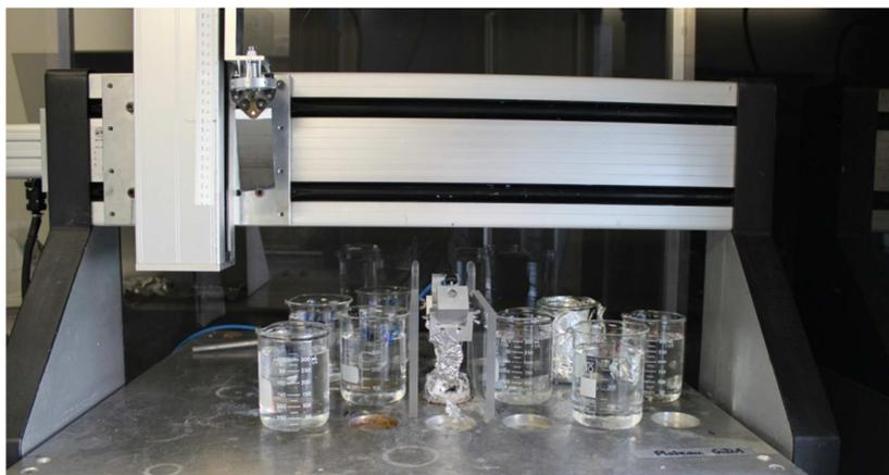
Figure 19: Dipping robot apparatus used for LbL film construction. The silicon wafer is held by the motorised arm. The drying station is located in the middle of two groups of 4 beakers.
