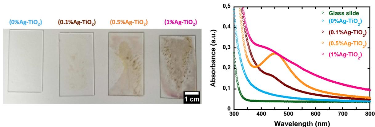
Figure 77: Characterisations of photoinduced AgNP synthesised on glass slide with TiO<sub>2</sub>-based x%AgNO<sub>3</sub>-TiO<sub>2</sub> photosensitive suspensions, containing different amounts of AgNO<sub>3</sub>. (Left) Pictures of the photosensitive suspensions on glass slides after UV irradiation. (Right) Corresponding transmission mode UV-Visible spectra.
