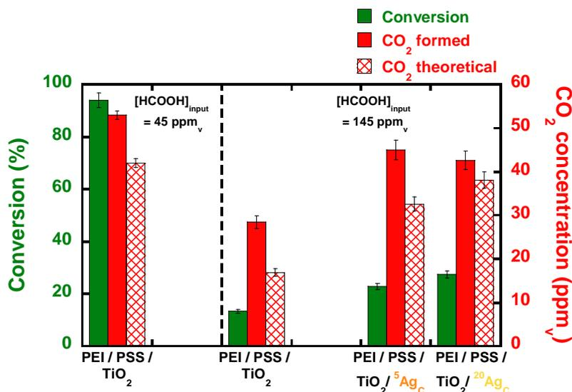
Figure 69: Photocatalytic activity of PEI/PSS/TiO<sub>2</sub> and PEI/PSS/TiO<sub>2</sub>/Ag<sub>c</sub> films expressed in terms of HCOOH conversion and CO<sub>2</sub> formation. Experimental parameters: [HCOOH] = 145 ppm<sub>v</sub>, relative humidity = 50%, air flow = 20 mL/min, speed = 0.7 cm/s, UV-A irradiance = 2.5 mW/cm<sup>2</sup>, films built on 36 cm<sup>2</sup> silicon wafers.
