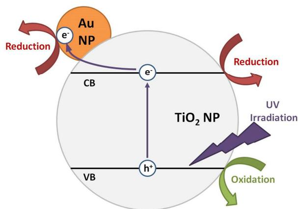
Figure 9: Association of TiO<sub>2</sub> with gold nanoparticles (AuNP) which act as an electron trap once TiO<sub>2</sub> is irradiated by UV light. The figure is based on schematic of Friehs *et al.* [93].
