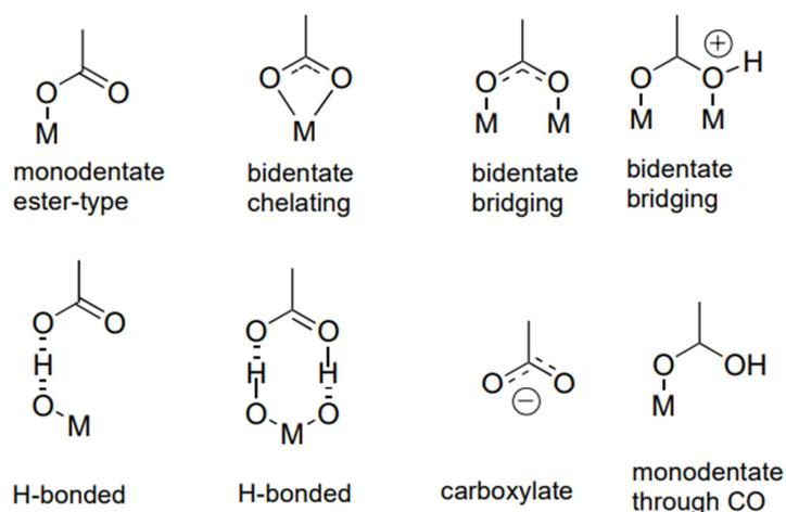
Figure 17 : Possible binding modes of a COOH group with a metal oxide (TiO<sub>2</sub>) [185]
