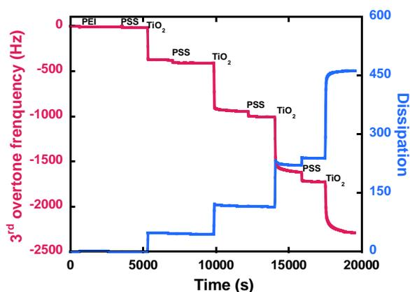
Figure 45: Monitoring PEI/(PSS/TiO<sub>2</sub>)<sub>n</sub> film construction by QCM-D at the 3<sup>rd</sup> overtone. 4 PSS/TiO<sub>2</sub> layer pairs were deposited.
