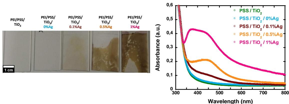
Figure 72: Classical photoinduced AgNP synthesis on PEI/PSS/TiO<sub>2</sub> films on glass slides (left) and the UV-Visible characterisation of PEI/PSS/TiO<sub>2</sub>/x%Ag films in transmission mode (right).
