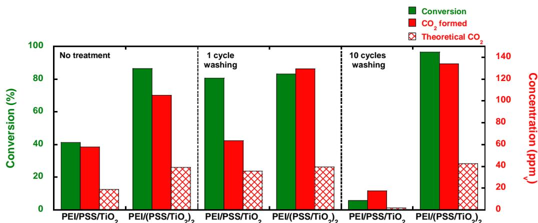
Figure 109 : Photocatalytic performances of functionalised textiles before and after 1 and 10 cycles washing. Experimental parameters: [HCOOH] = 45 ppm<sub>v</sub>, air flow = 20 mL/min, speed = 0.7 cm/s, UV-A irradiance = 2.5 mW/cm<sup>2</sup>, films built on polyester textile.
