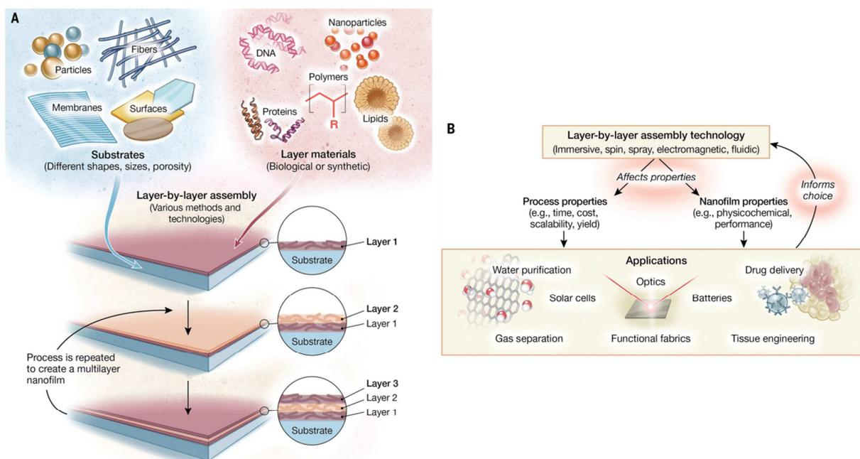
Figure 16: (A) Schematic overview of LbL self-assembly. (B) Influence of LbL self-assembly on films, process properties and applications area [145].
