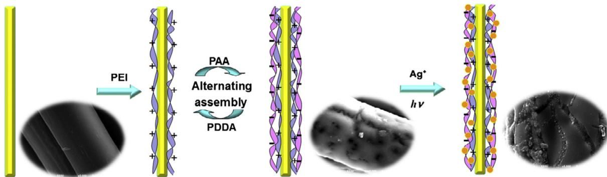
Figure 18: AgNP photoinduced synthesis on PEI/(PAA/PDDA)<sub>8</sub> LbL film constructed on silk fibers [193].
