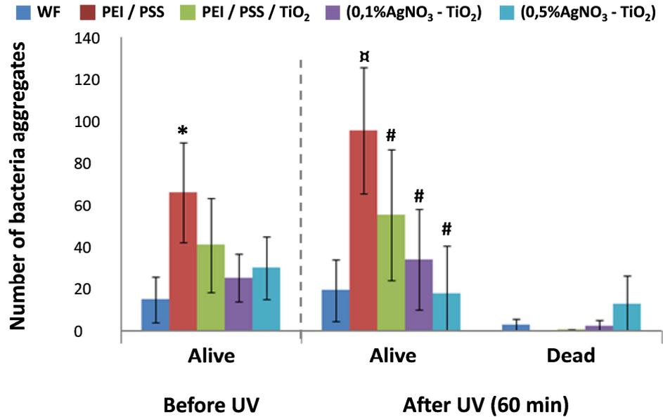
Figure 92 : Number of bacteria aggregates before and after UV-A irradiation of the films. Tested bacteria: *Echerichia Coli*, UV-A irradiance = 2.5 mW/cm<sup>2</sup>, irradiation time = 60 min, films built on 2 cm<sup>2</sup> silicon wafers. (\*) significantly different than WF before UV ( $p$ -value < 0.05); (α) significantly different than WF after UV (ALIVE) ( $p$ -value < 0.05); (#) significantly different than PEI/PSS after UV (ALIVE) ( $p$ -value < 0.05).
