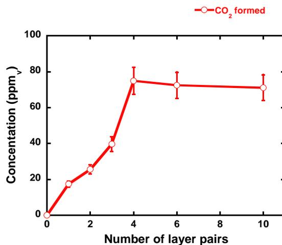
Figure 98 : Evolution of CO<sub>2</sub> formation UV-A irradiation, in the absence of HCOOH, in regards to the number of layer pairs deposited on textile surfaces. Experimental parameters: [HCOOH] = 0 ppm<sub>v</sub>, air flow = 20 mL/min, speed = 0.7 cm/s, UV-A irradiance = 2.5 mW/cm<sup>2</sup>, films built on polyester textile.
