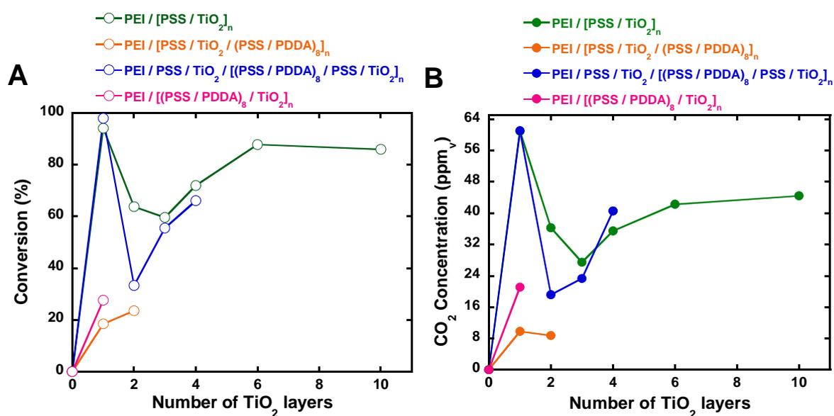
Figure 60 : Degradation of gas-phase HCOOH under UV-A light using LbL titania film with different types of architecture. (A) HCOOH conversion rate in regards of number of TiO<sub>2</sub> layers deposited; (B) CO<sub>2</sub> formation in regards of number of TiO<sub>2</sub> layers deposited. Experimental parameters: [HCOOH] = 45 ppm<sub>v</sub>, air flow = 20 mL/min, speed = 0.7 cm/s, UV-A irradiance = 2.5 mW/cm<sup>2</sup>, films built on 36 cm<sup>2</sup> silicon wafers.
