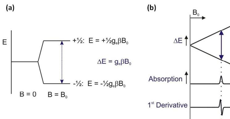
Figure 29: Energy level diagram of Zeeman interaction for an unpaired electron as function of the applied magnetic field  $\vec{B}_0$ . The vertical arrow represents the possible EPR transition according to the selection rule for  $\Delta m_s = \pm 1$  [205].
