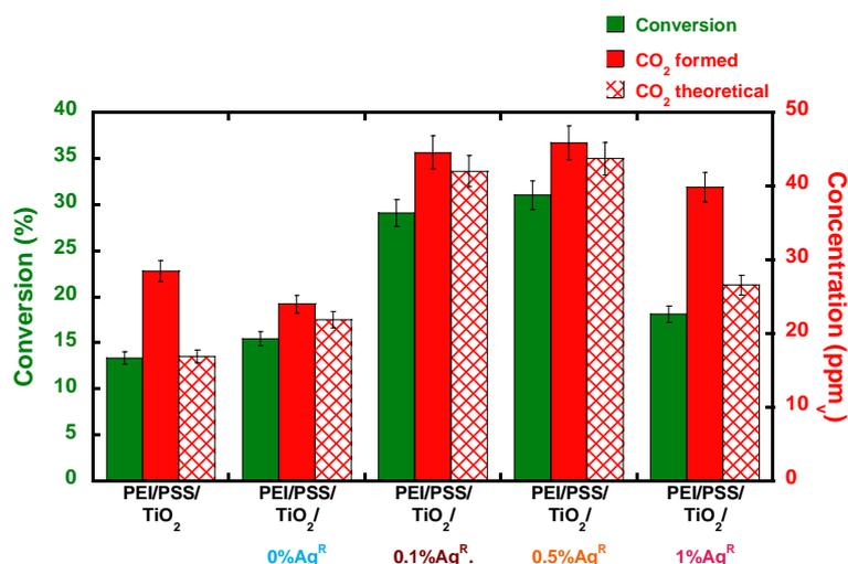
Figure 76: Photocatalytic performance of PEI/PSS/TiO<sub>2</sub>/x%Ag<sup>R</sup> films (with additional rinsing steps prior UV irradiation for AgNP photoinduced synthesis). Experimental parameters: [HCOOH] = 145 ppm<sub>v</sub>, air flow = 20 mL/min, speed = 0.7 cm/s, UV-A irradiance = 2.5 mW/cm<sup>2</sup>, films built on 36 cm<sup>2</sup> silicon wafers.
