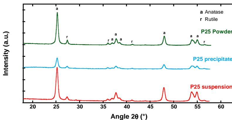
Figure 39 : XRD analysis of TiO<sub>2</sub> P25 as powder, precipitate and from the LbL suspension. a and r correspond to peak associated to anatase and rutile phase respectively.
