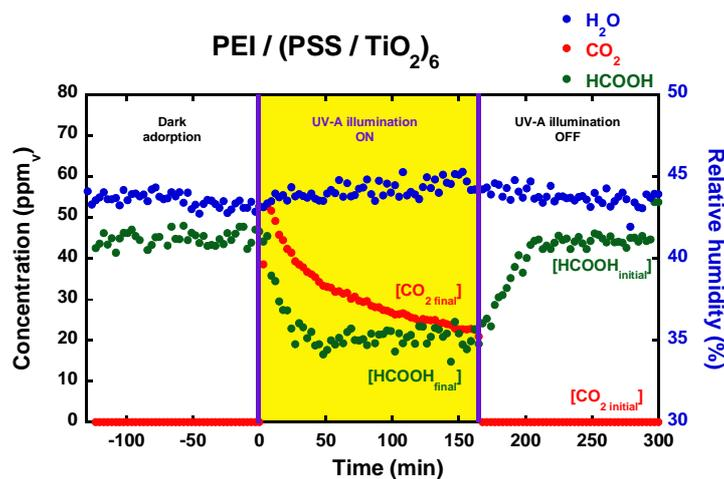
Figure 37: Photocatalytic activity of a PEI/(PSS/TiO<sub>2</sub>)<sub>6</sub> LbL film
