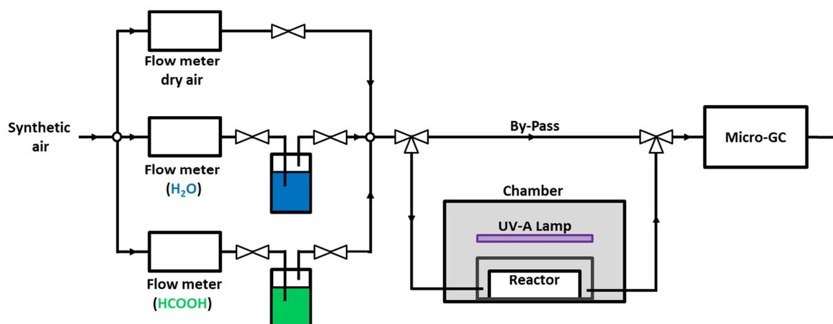
Figure 36: Gas-phase photocatalytic set-up.
