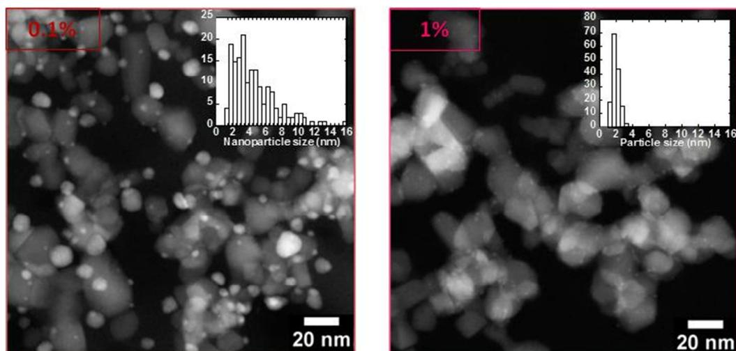
Figure 74 : STEM images of PEI/PSS/TiO<sub>2</sub>/0.1%Ag and PEI/PSS/TiO<sub>2</sub>/1%Ag.
