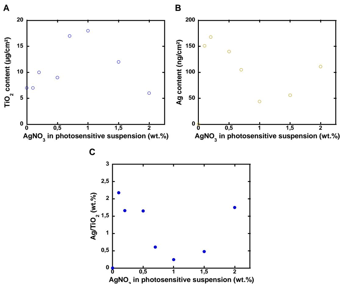
Figure 80 : (A) TiO<sub>2</sub> and (B) Ag content in regards to the AgNO<sub>3</sub> concentration in the TiO<sub>2</sub> photosensitive suspension. (C) Ag/TiO<sub>2</sub> wt.% in Ag-TiO<sub>2</sub> hybrid films in regards to the AgNO<sub>3</sub> concentration in TiO<sub>2</sub> photosensitive suspension.
