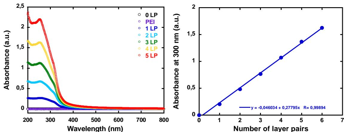
Figure 44: Transmission UV-Visible photospectrophotometry characterisation of PEI/(PSS/TiO<sub>2</sub>)<sub>n</sub> film. (Left) film deposition on quartz slide with absorbance increment after each layer pairs deposited. (Right) reported absorbance at 300 nm in regards to the number of layer pairs deposited.
