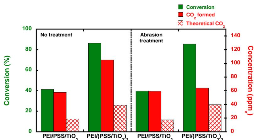
Figure 105 : Photocatalytic performances of functionalised textiles before and after dry abrasion treatment. Experimental parameters: [HCOOH] = 45 ppm<sub>v</sub>, air flow = 20 mL/min, speed = 0.7 cm/s, UV-A irradiance = 2.5 mW/cm<sup>2</sup>, films built on polyester textile.
