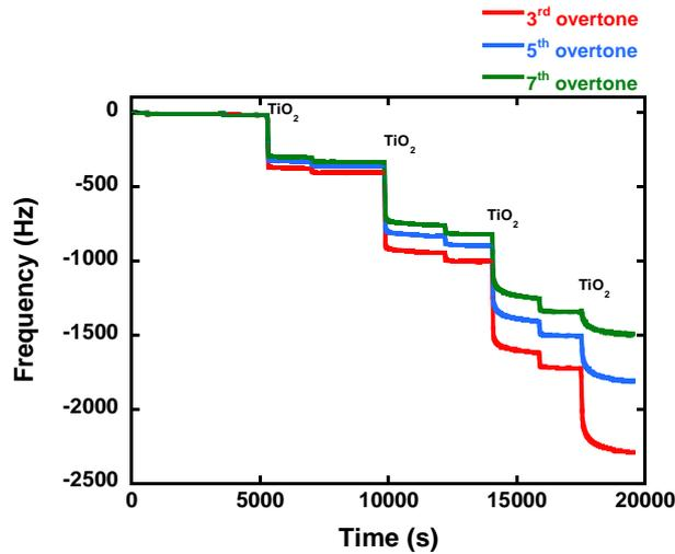
Appendix 3 : Change of frequency overlaying of 3<sup>rd</sup>, 5<sup>th</sup> and 7<sup>th</sup> overtones when film is constructed on QCM quartz slide.
