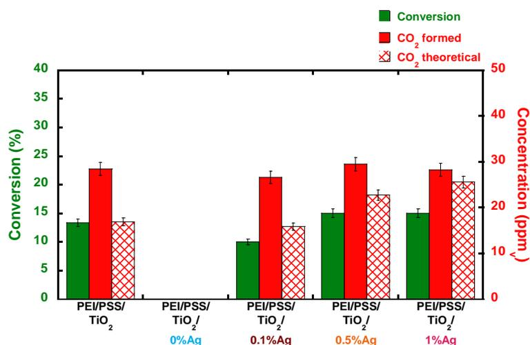
Figure 75 : Photocatalytic performance of PEI/PSS/TiO<sub>2</sub>/x%Ag films towards the degradation of gas phase HCOOH. Experimental parameters: [HCOOH] = 145 ppm<sub>v</sub>, air flow = 20 mL/min, speed = 0.7 cm/s, UV-A irradiance = 2.5 mW/cm<sup>2</sup>, films built on 36 cm<sup>2</sup> silicon wafers.
