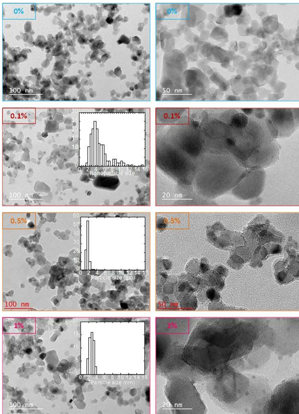
Figure 73 : TEM images of PEI/PSS/TiO<sub>2</sub>/x%Ag films. x = 0%, 0.1%, 0.5% and 1%. The size distribution was assessed only on 56 nanoparticles for the sample with x=1%.
