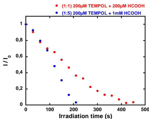
Figure 59 : Evolution of TEMPOL spin-scavenging by a PEI/(PSS/TiO<sub>2</sub>)<sub>10</sub> film, using a mixed solution of TEMPOL:HCOOH.
