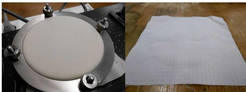
Figure 103 : Wool rep (left) and 2 layer pairs functionalised polyester textile (right) after an abrasion test of 500 cycles.
