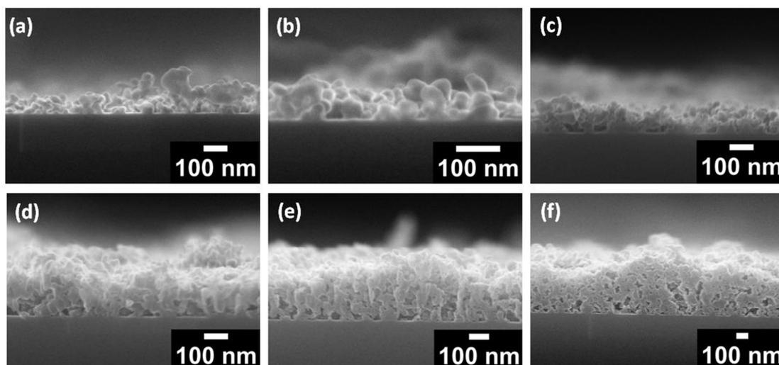
Figure 47: Cross section of PEI/(PSS/TiO<sub>2</sub>)<sub>n</sub> LbL films deposited on silicon wafers. n=1 (a and b), n=2 (c), n=4 (d), n=6 (e) and n=10 (f). Brightness and contrast of SEM images were treated with Image J®.
