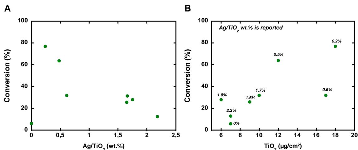
Figure 87 : (A) HCOOH conversion in regards to the Ag/TiO<sub>2</sub> content. (B) HCOOH conversion in regards to the amount of TiO<sub>2</sub> in PEI/PSS/(AgNP-TiO<sub>2</sub>) film. Experimental parameters: [HCOOH] = 255 ppm<sub>v</sub>, air flow = 20 mL/min, speed = 0.7 cm/s, UV-A irradiance = 2.5 mW/cm<sup>2</sup>, films built on 36 cm<sup>2</sup> silicon wafers.
