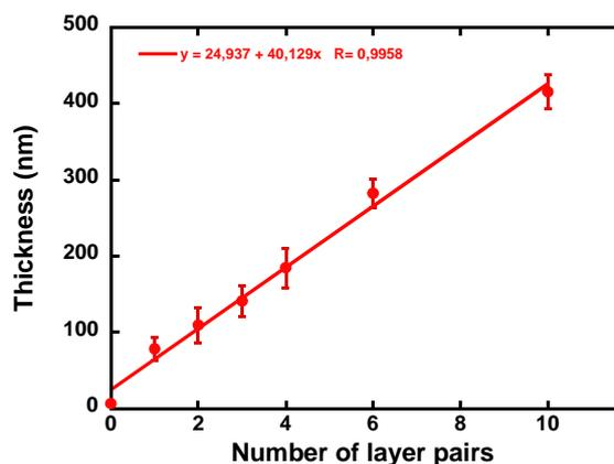
Figure 43: Ellipsometry characterisation of PEI/(PSS/TiO<sub>2</sub>)<sub>n</sub> films. A linear increase in thickness is observed after deposition of each PSS/TiO<sub>2</sub> layer pair.
