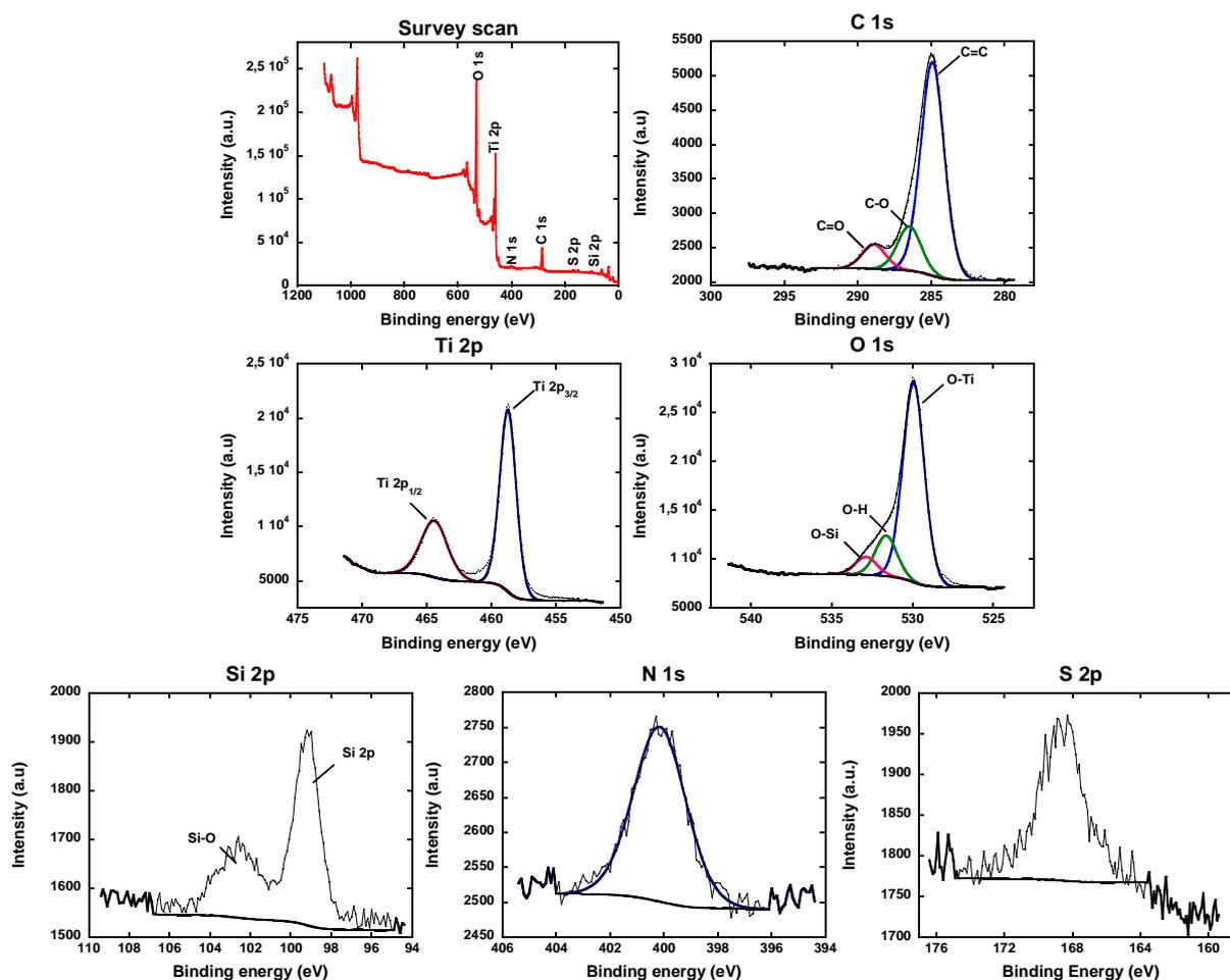
Figure 81 : XPS characterisation of the PEI/(PSS/TiO<sub>2</sub>)<sub>10</sub> LbL film.
