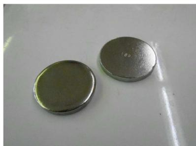
Figure 110: Stainless steel discs used in dry cleaning treatment.
