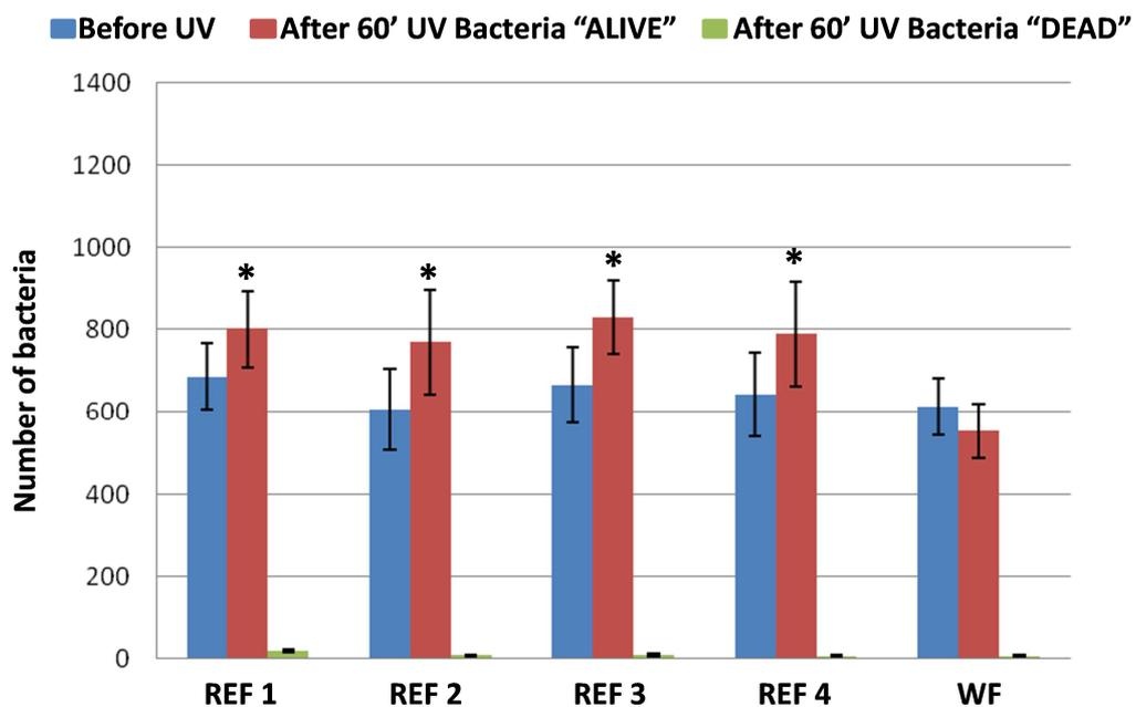
Figure 64: Bacteria assay on reference samples. Tested bacteria: *Echerichia Coli*, UV-A irradiance = 2.5 mW/cm<sup>2</sup>, irradiation time = 60 min, films built on 2 cm<sup>2</sup> silicon wafers. (\*) significantly different than WF (ALIVE) (*p*-value < 0.05)
