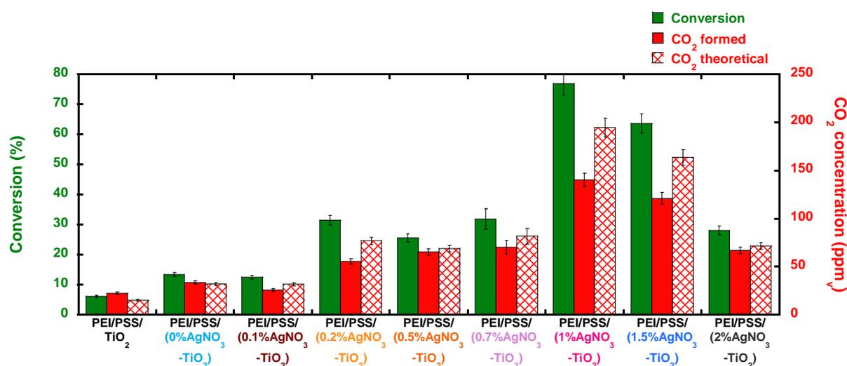
Figure 86 : Photocatalytic performance of PEI/PSS/(x%Ag-TiO<sub>2</sub>) films under 24h of UV-A irradiation. Experimental parameters: [HCOOH] = 255 ppm<sub>v</sub>, air flow = 20 mL/min, speed = 0.7 cm/s, UV-A irradiance = 2.5 mW/cm<sup>2</sup>, films built on 36 cm<sup>2</sup> silicon wafers.
