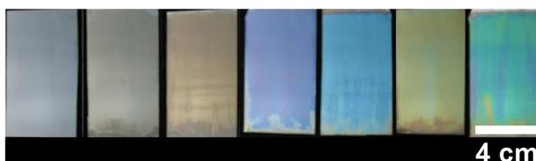
Figure 42 : Optical photographs of PEI/(PSS/TiO<sub>2</sub>)<sub>n</sub> film deposited on silicon wafers. From left to right: bare silicon wafer, PEI/PSS film, PEI/PSS/TiO<sub>2</sub>, PEI/(PSS/TiO<sub>2</sub>)<sub>2</sub>, PEI/(PSS/TiO<sub>2</sub>)<sub>4</sub>, PEI/(PSS/TiO<sub>2</sub>)<sub>6</sub> and PEI/(PSS/TiO<sub>2</sub>)<sub>10</sub>.
