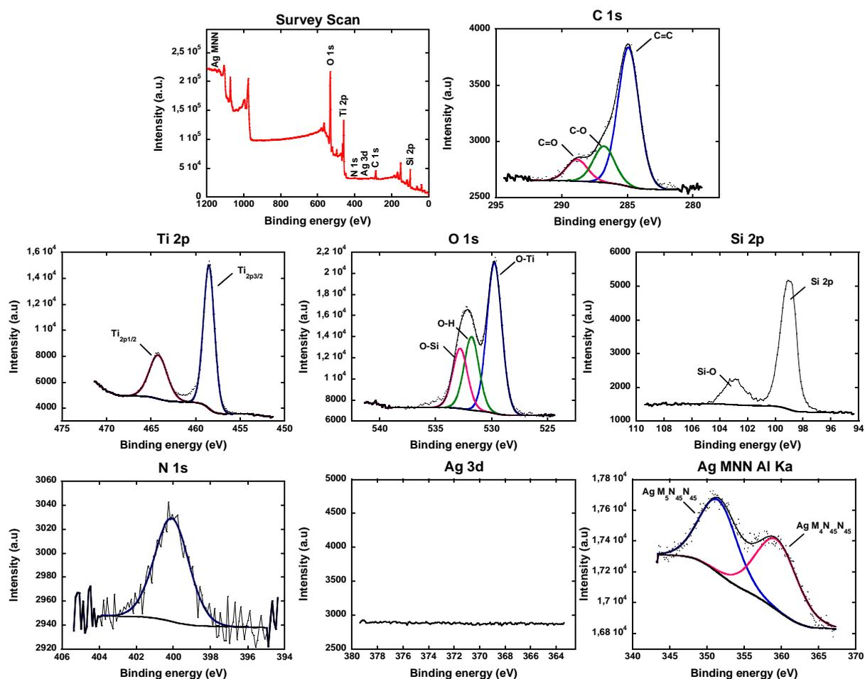
Figure 83 : XPS characterisations of PEI/PSS/(1%Ag-TiO<sub>2</sub>) LbL film
