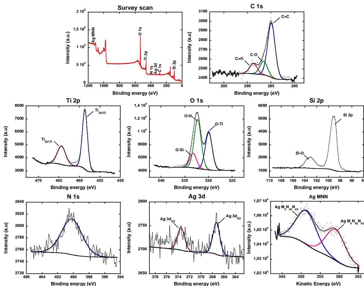
Figure 82: XPS characterisations of PEI/PSS/(0.2%Ag-TiO<sub>2</sub>) LbL film
