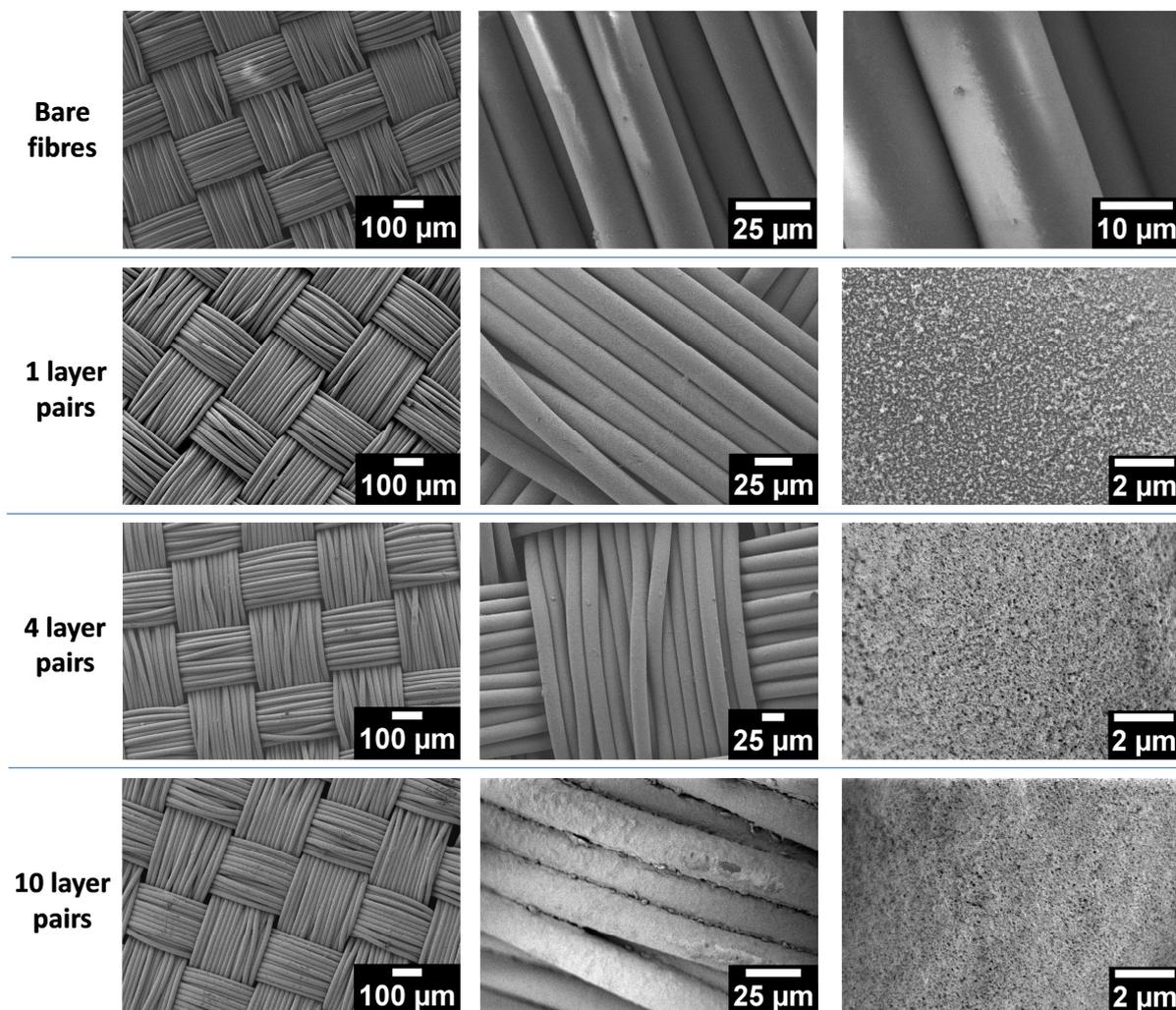
Figure 96 : SEM characterisation of PEI/(PSS/TiO<sub>2</sub>)<sub>n</sub> LbL films constructed on polyester textile surface.
