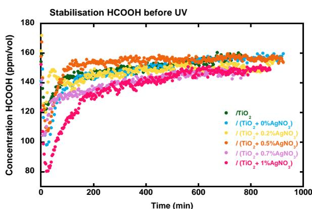
Appendix 9 : Stabilisation of PEI/PSS/(x%Ag-TiO<sub>2</sub>) samples prior UV-A irradiation of the films. Experimental parameters: [HCOOH] = 145 ppm<sub>v</sub>, air flow = 20 mL/min, speed = 0.7 cm/s, UV-A irradiance = 2.5 mW/cm<sup>2</sup>, films built on 36 cm<sup>2</sup> silicon wafers
