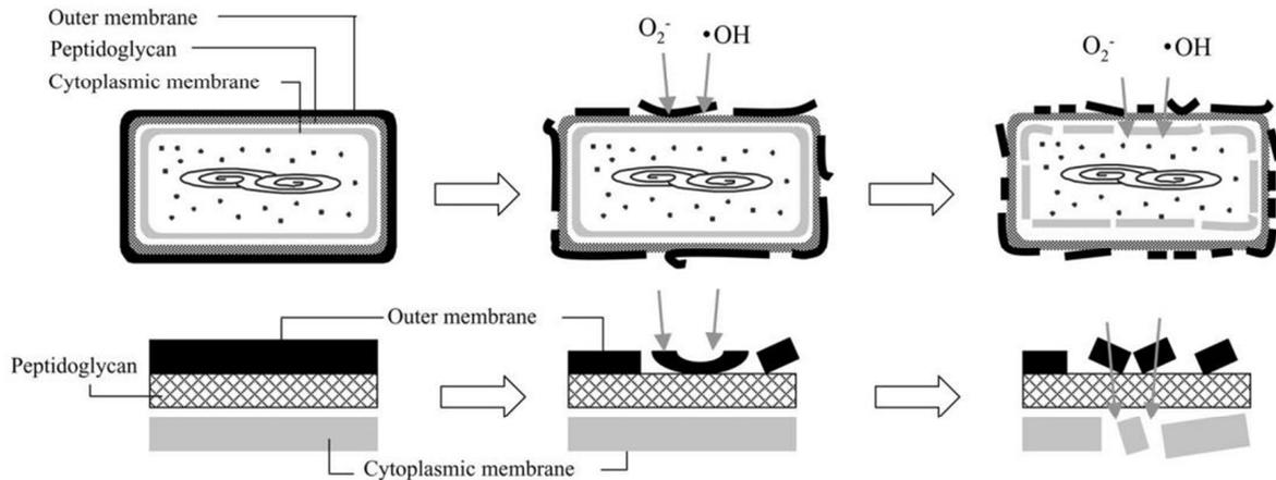
Figure 8: Degradation of the bacteria cell membrane by reactive oxygen species upon UV irradiation of  $TiO_2$  film [77]. The bottom images show a schematic magnification of the bacteria membrane during degradation.
