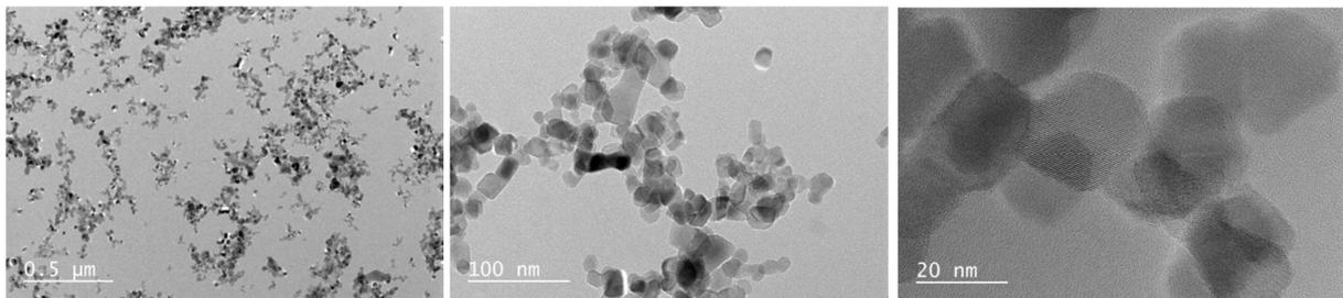
Figure 49: TEM images of a PEI/PSS/TiO<sub>2</sub> LbL film (single layer pair).
