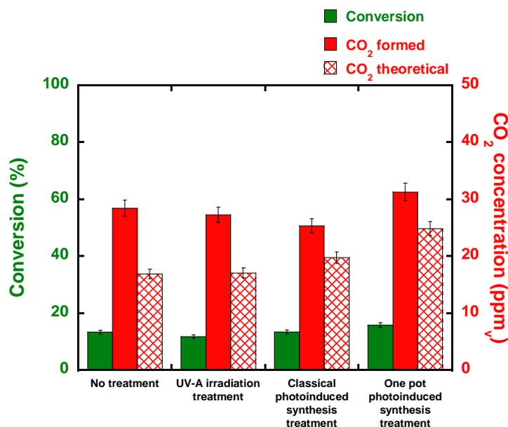
Figure 70 : Comparison of photocatalytic performances of PEI/PSS/TiO<sub>2</sub> films in terms of HCOOH conversion and CO<sub>2</sub> formation, after irradiation by the UV lamp used for AgNP photoinduced synthesis. Experimental parameters: [HCOOH] = 145 ppm<sub>v</sub>, air flow = 20 mL/min, speed = 0.7 cm/s, UV-A irradiance = 2.5 mW/cm<sup>2</sup>, films built on 36 cm<sup>2</sup> silicon wafers.
