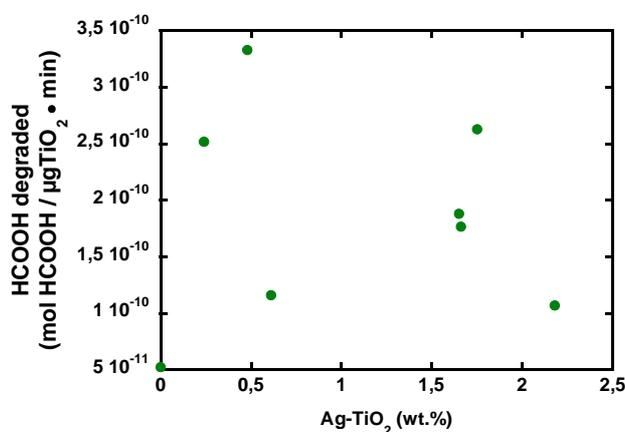
Appendix 10 : Degradation of HCOOH per μg TiO<sub>2</sub> • min, in regards to the silver content in PEI/PSS/(x%Ag-TiO<sub>2</sub>) films.
