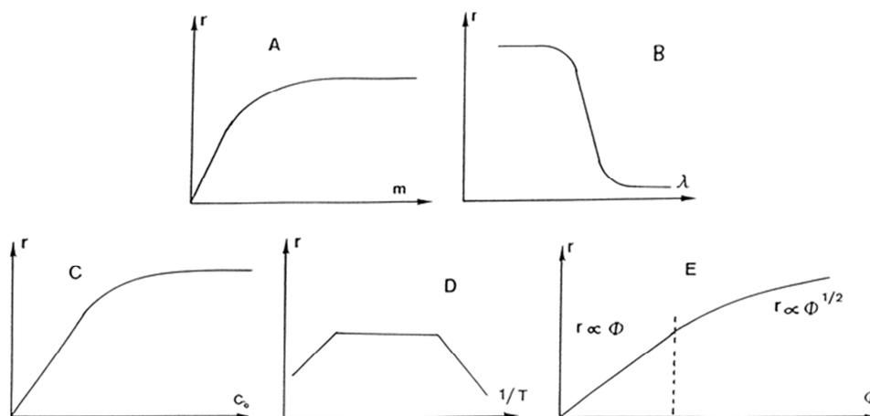
Figure 5 : Different parameters that influence the photocatalytic reaction rate  $r$ . (A) mass  $m$  of photocatalyst, (B)  $\lambda$  irradiation wavelength, (C) initial concentration  $C_0$ , (D) temperature  $T$  and (E) radiant flux  $\phi$  [6].
