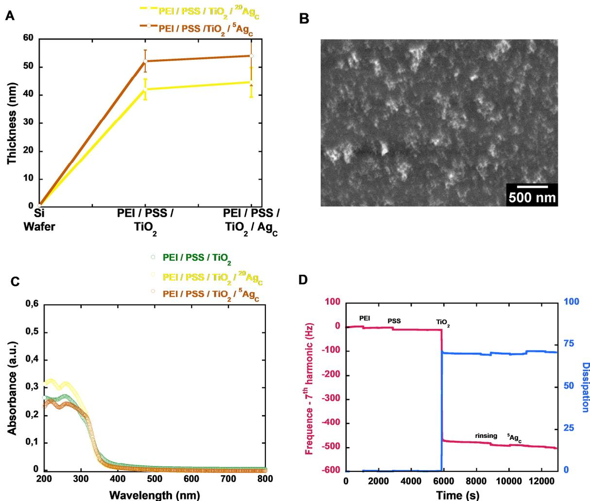
Figure 68 : Characterisation of PEI/PSS/TiO<sub>2</sub>/Ag<sub>c</sub> films. (A) ellipsometry performed on films constructed on silicon wafer, (B) SEM image of a PEI/PSS/TiO<sub>2</sub>/<sup>20</sup>Ag<sub>c</sub> film, (C) UV-Visible spectrophotometry of films constructed on quartz slides, and (D) QCM-D analysis of a PEI/PSS/TiO<sub>2</sub>/<sup>5</sup>Ag<sub>c</sub> film on QCM crystal slide.
