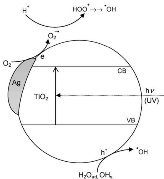
Figure 13: Photocatalytic pathway of TiO<sub>2</sub>-silver nanocomposite under UV-irradiation [130].
