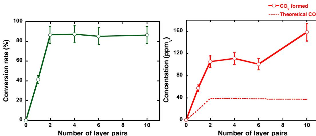
Figure 97 : (Left) Evolution of HCOOH conversion in regards to the number of layer pairs deposited in LbL films. (Right) Evolution of CO<sub>2</sub> formed upon irradiation of LbL films, in regards to the number of layer pairs. Experimental parameters: [HCOOH] = 45 ppm<sub>v</sub>, air flow = 20 mL/min, speed = 0.7 cm/s, UV-A irradiance = 2.5 mW/cm<sup>2</sup>, films built on polyester textile.
