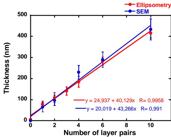
Figure 48 : Increase in thickness of PEI/(PSS/TiO<sub>2</sub>)<sub>n</sub> LbL films obtained by ellipsometry and SEM characterisations.
