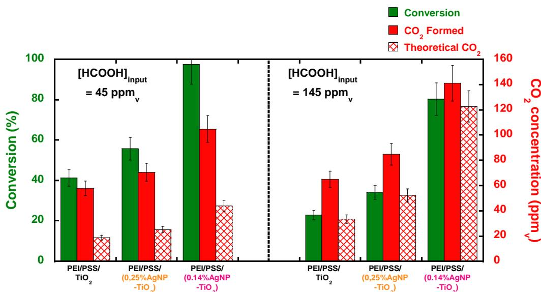
Figure 99 : Comparison of photocatalytic results of PEI/PSS/(AgNP-TiO<sub>2</sub>) films obtained at different input HCOOH concentrations. Experimental parameters: [HCOOH] = (left) 45 and (right) 145 ppm<sub>v</sub>, air flow = 20 mL/min, speed = 0.7 cm/s, UV-A irradiance = 2.5 mW/cm<sup>2</sup>, films built on polyester textile.
