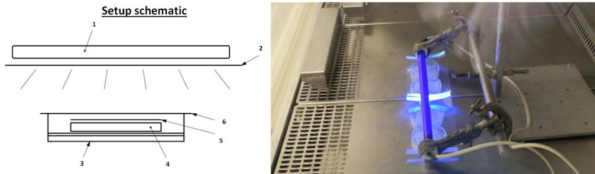
Figure 38 : Schematic (left) and picture (right) of the setup used in antibacterial assay on LbL films constructed on textile surfaces. 1 and 2 – UV-A lamp, 3 – Petri dish, 4 – textile placed on a support, 5 – glass slide, 7 – PCR sealing film.
