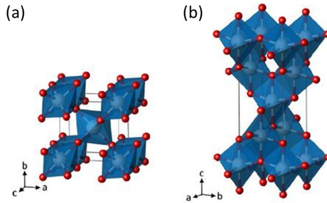
Figure 7: Crystal structure of  $\text{TiO}_2$  in its rutile (a) and anatase (b) phase (Ti (white); O (red)) [78].
