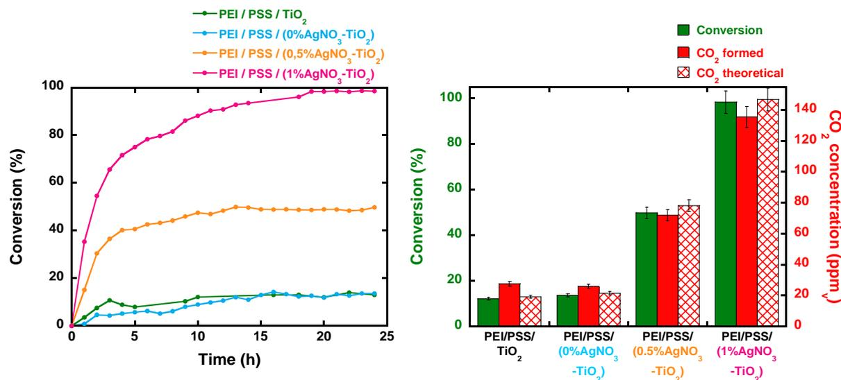
Figure 85 : (Left) Evolution of gas-phase HCOOH conversion during UV-A irradiation of PEI/PSS/(x%Ag-TiO<sub>2</sub>) films. (Right) Photocatalytic performance of PEI/PSS/(x%Ag-TiO<sub>2</sub>) films. Experimental parameters: [HCOOH] = 145 ppm<sub>v</sub>, air flow = 20 mL/min, speed = 0.7 cm/s, UV-A irradiance = 2.5 mW/cm<sup>2</sup>, films built on 36 cm<sup>2</sup> silicon wafers.
