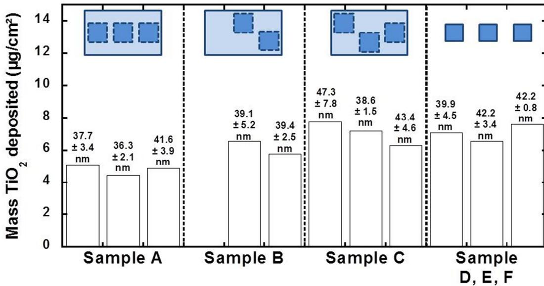
Appendix 4 : Amount of TiO<sub>2</sub> deposited in single layer pair films investigated by ICP-AES. Blue rectangles above every set of samples represent a 36 cm<sup>2</sup> silicon wafer and dash lines are the area where 4 cm<sup>2</sup> samples were cut for chemical analysis. Sample D, E and F were directly constructed on 4 cm<sup>2</sup> silicon wafer. Film thickness is reported above each histogram (measured by ellipsometry).
