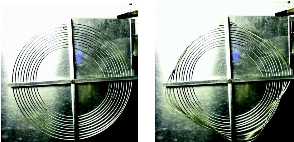
Figure 3.6: When clamping the spiral at one end, it continues to operate, storing elastic energy. The longer tests were performed until a buckling event as depicted on the right happened, the tests were stopped to prevent mechanical damage to the spirals.
