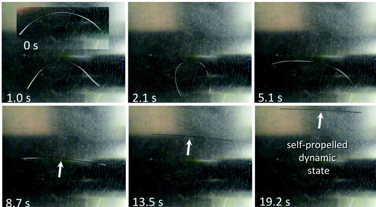
Figure 3.10: Slow annealing of a 800  $\mu\text{m}$  nylon fiber at 110°C results in some transient reshaping and eventually within the time course of 10-20 seconds leads to an ideally straight and rolling fiber.
