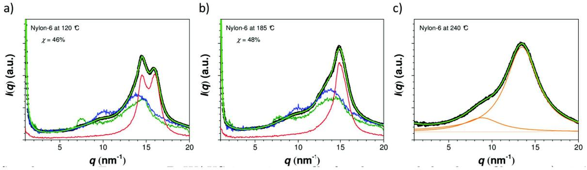
Figure A.3: 1D WAXS intensity profile for the annealed nylon-6 fiber at a)  $120^\circ\text{C}$ , b)  $185^\circ\text{C}$ , and c)  $240^\circ\text{C}$  and the corresponding fitting curve (light green curve). The red (equatorial), blue (45 degrees oblique) and dark green (meridional) curves correspond to the scattering profiles from the sections in Fig. A.2. The orange curves in c) are the amorphous peaks contributing to the signal for the polymer melt.
