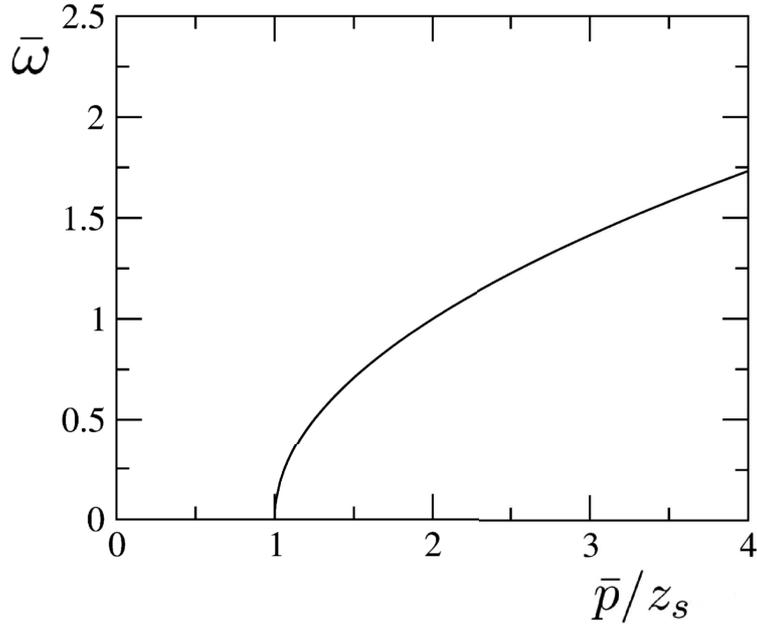
Figure 2.9: Continuous onset of rotation of a fiber closed to a ring as given by (2.22). Shown is the scaled angular velocity,  $\bar{\omega}$ , as a function of the rescaled effective driving  $\frac{\bar{p}}{z_s}$ .
