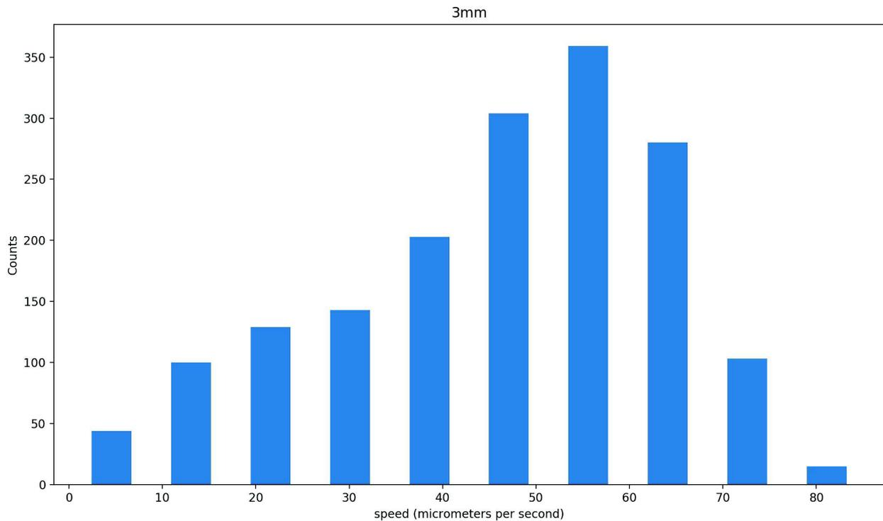
Figure 5.13: Histogram of the velocities represented in Fig. 5.12. Starting from zero velocity at the surface, the flow goes up to dozens of  $\mu\text{m}/\text{s}$  at 3mm above the surface.
