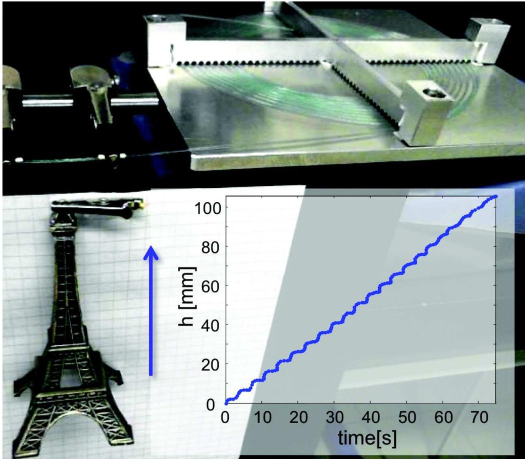
Figure 3.4: Spiral fiberdrive (fiber thickness 0.8mm, total spiral length 3.2m) realized according to the design showed in Fig. 2.10. It is rotating at  $185^{\circ}\text{C}$  lifting a payload (Eiffel Tower replica of weight 20 g). The fiber is guided from the spiral holder through two brass tubes and rotates freely there. Inset: position of the weight as it is lifted.
