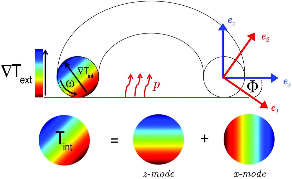
Figure 2.7: The geometry of the toroidal fiberdrive. The internal temperature profile  $T_{\text{int}}$  of each cross-section is decomposed in two modes. The thermal  $z$ -mode is pumped by the heat flux  $p$  normal to the substrate (represented by the red horizontal line). The  $x$ -mode  $\Delta T_x$  emerges from the  $z$ -mode  $\Delta T_z$  by frame rotation with the angle  $\Phi$ .
