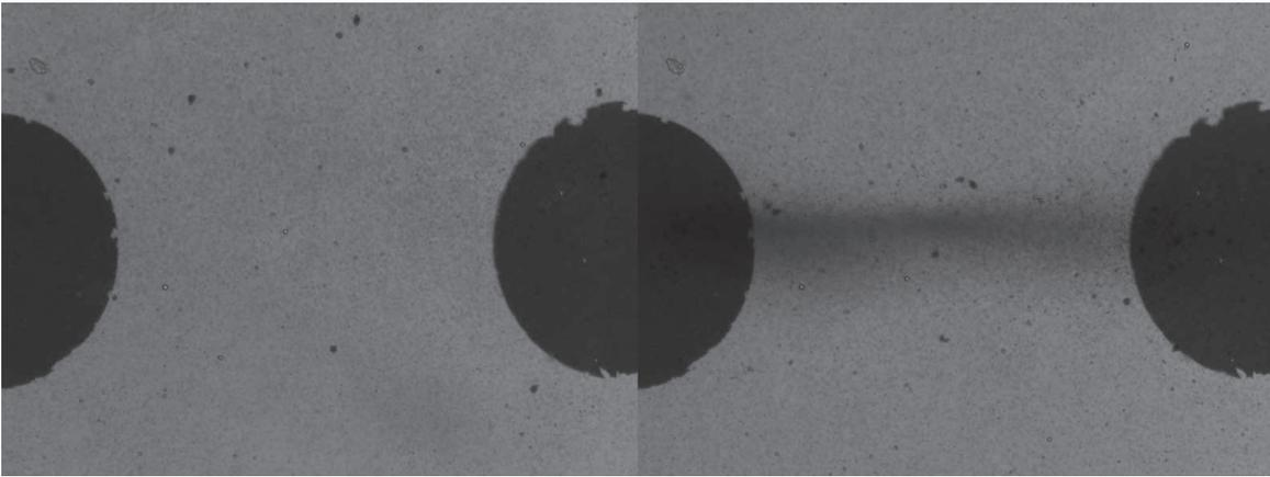
Figure 5.14: Glass slide with two disks of gold ( $500\mu\text{m}$  in diameter,  $1\text{mm}$  apart edge to edge). Left : at the start of the illumination. Right : after 26 minutes of continuous illumination. The convection flow induced by the two disks gathers the tracer particles on the line linking them.
