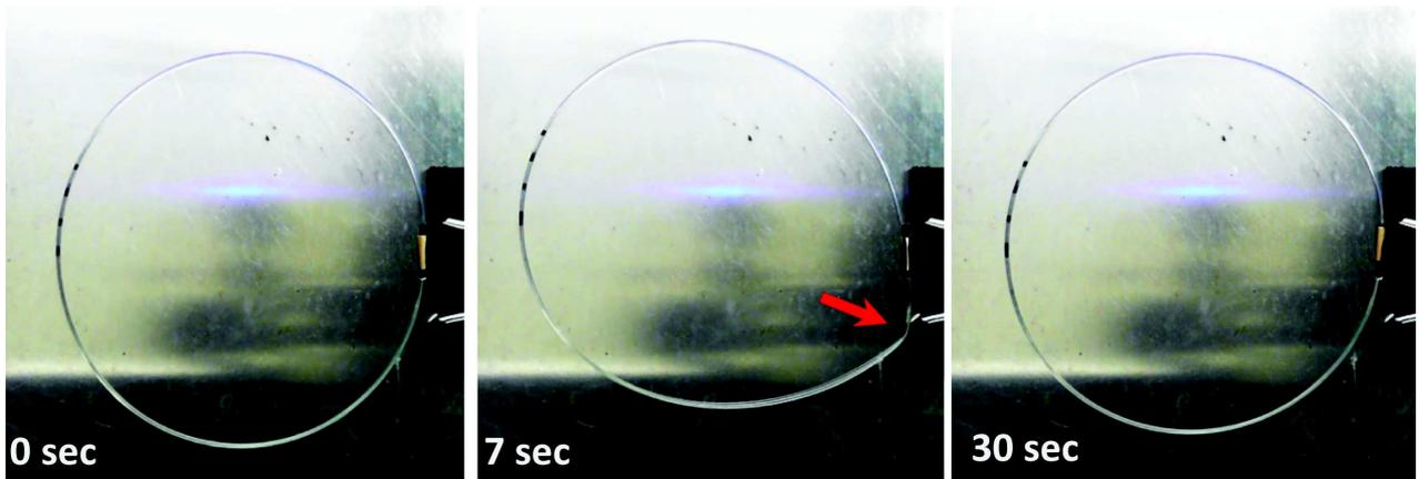
Figure 3.2: Collective spontaneous self-healing of defects in a circular fiber motor from nylon-6 rotating at 190°C. A strong deformation defect (kink) emerges at time  $t = 7$  s and persists for several seconds. The continued collective rotation of the fiber leads to a complete self-healing at a later time ( $t = 30$  s)
