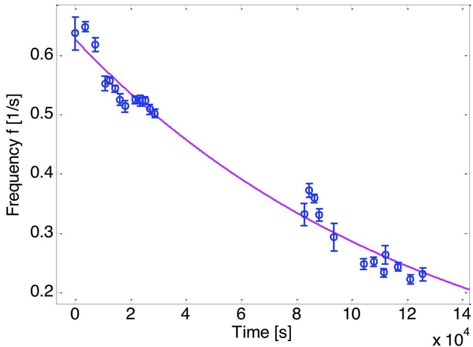
Figure 3.5: Continuous operation long time-testing of a spiral fiber motor. The fiber (nylon-6) is guided to a 13 turn, 0.6 mm diameter spiral and runs at  $T=160^{\circ}\text{C}$ . The magenta line is a fit to  $f(t) = f_0 \exp(-\frac{t}{t_r})$ , with  $f_0 = 0.63\text{Hz}$  and with the exponential frequency relaxation time of  $t_r = 34\text{h}$  ( $1.28 \times 10^5\text{s}$ ). The error bars are the standard deviations from 10 separate measurements.
