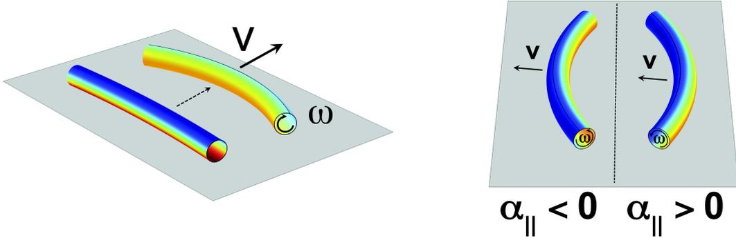
Figure 2.8: The temperature gradient between the hot plate and the ambient air bends the rod via thermal expansion or contraction. Due to the confinement (on the plate) the curving stays in-plane, which effectively creates a torque. The direction of the curvature  $\kappa$  relative to the velocity  $\mathbf{V}$  depends on the sign of the thermal expansion coefficient.
