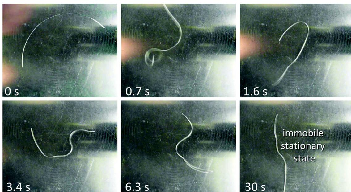
Figure 3.11: Exposing a nylon fiber ( $800 \mu\text{m}$ ) directly to an elevated temperature ( $180^\circ\text{C}$ ) results in rapid uncontrolled reshaping. The final shape remains stationary and does not move or roll over the surface.
