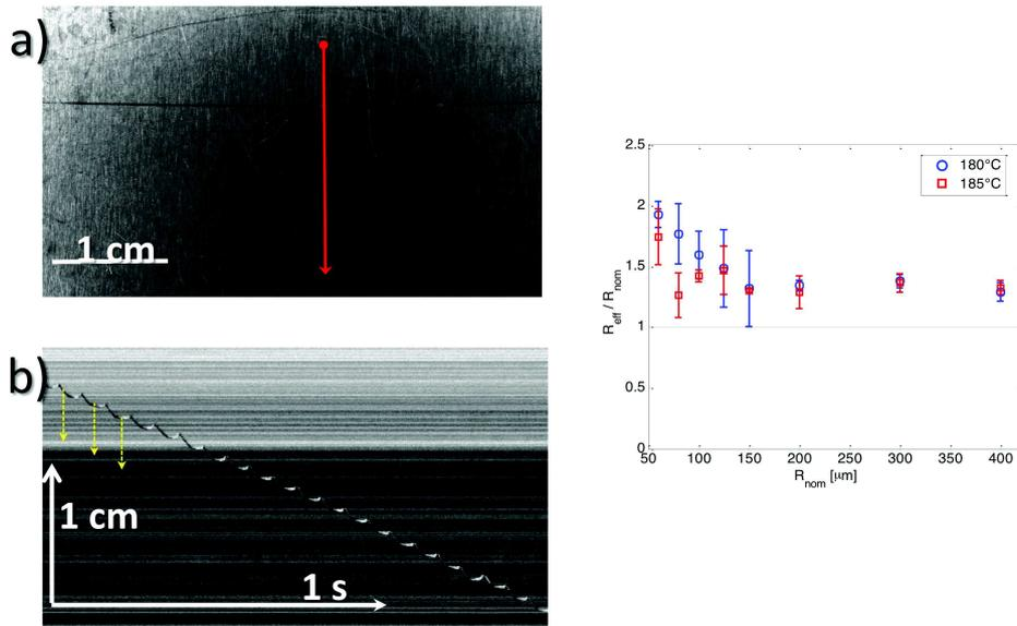
Figure 3.12: Measurement of linear and angular velocity. a) A nylon-6 fiber of radius  $60 \mu\text{m}$  rolling at  $185^\circ\text{C}$ . b) Kymograph of the motion along the red line in a). In addition to a constant velocity linear motion, the fiber displays a velocity modulation (yellow arrows) in phase with its rotary motion. On the right, the effective radius of the fiber is shown, deduced from the ratio of linear and angular velocity.
