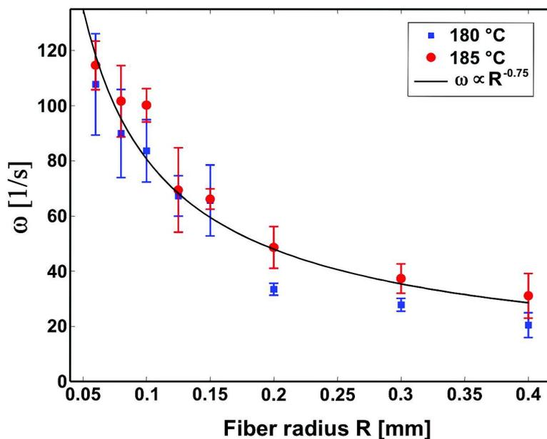
Figure 3.16: fibers with decreasing radii rotate with increasing angular frequencies: experimental data for two temperatures and a power-law fit  $R^{-\gamma}$  with  $\gamma = 0.75$ . The errors bar are calculated from the standard deviation of three different specimen.
