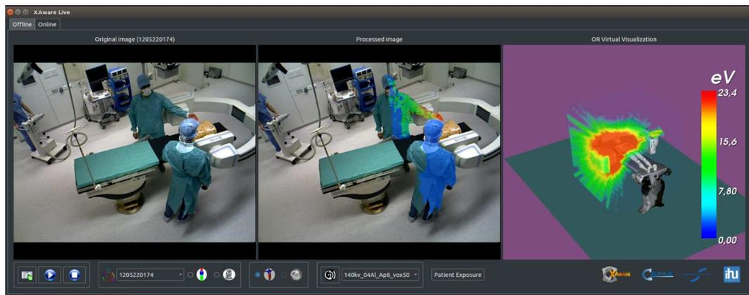
Figure 7.5: AR visualization of the current personnel’s body radiation exposure with *XAware-Live*.
