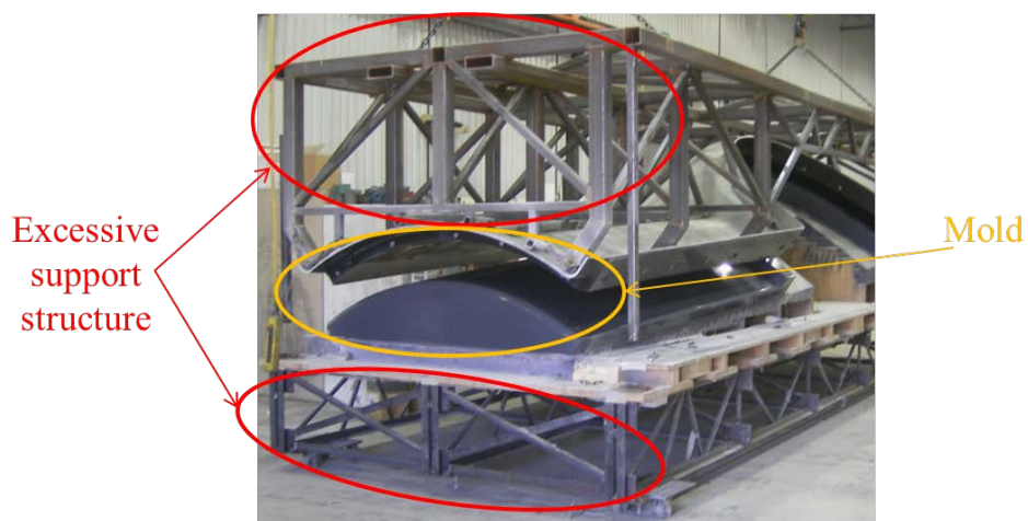
Figure 2.24 Picture of an industrial mold equipped with excessive support structure [25]
