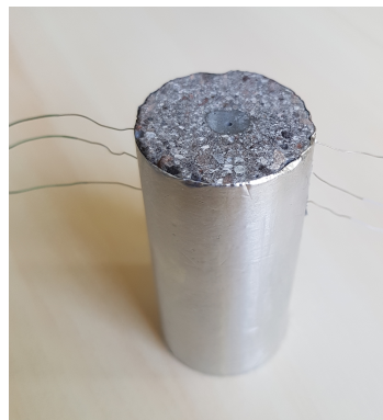
Figure 4.8: Specimen wrapped with adhesive aluminium tape
