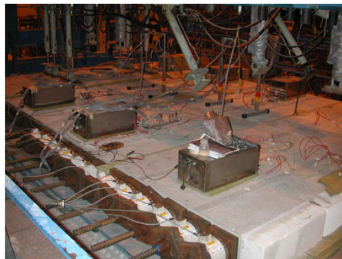
Figure 1.11: Example of full-scale fire test on a slab equipped with temperature and gas pressure sensors and loaded with post tensioning bars (Jansson and Boström, 2013)
