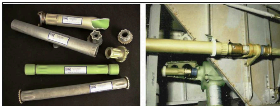
Figure 1.36: MPW application for aircraft flight control tubes [241]
