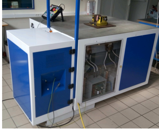
Figure 3.1: 50 kJ pulse generator at ECN
