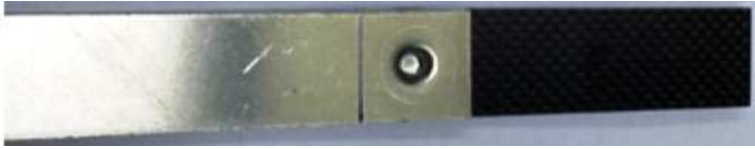
Figure 1.6: Al6061-T4 and CFRP joining by hole-clinching process [120]
