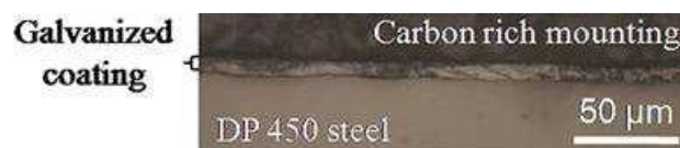
Figure 3.65: transverse cross section of the galvanized DP450 steel (light microscopy) [16]
