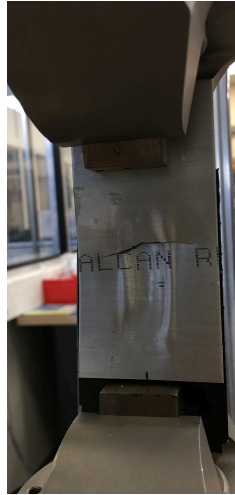
Figure 4.24: 5182 flyer metal tearing during fatigue test for the joint with FRPC using the steel DC04 metallic insert
