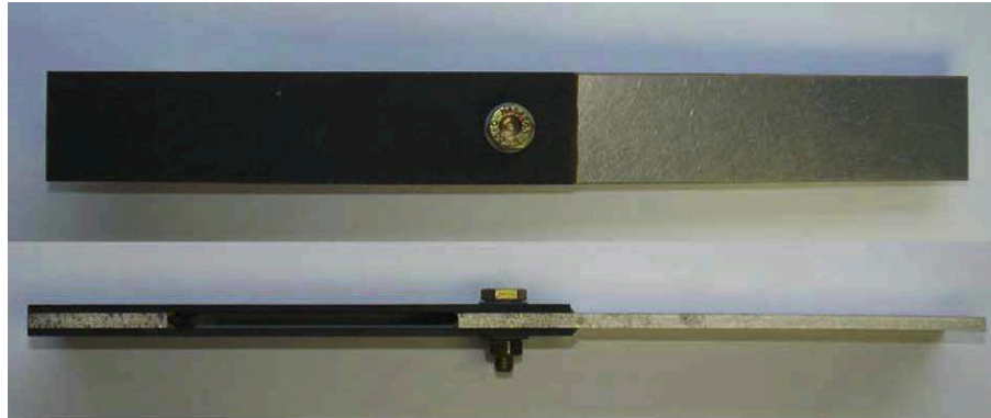
Figure 1.12: bonded/bolted hybrid joint CFRP/Al 7075-T62 [118]
