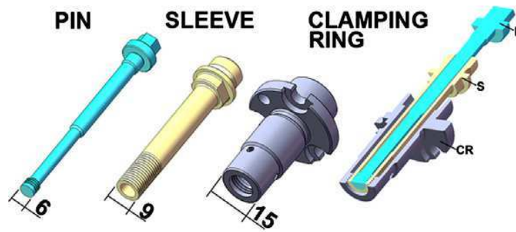
Figure 1.23: FSpJ tool system [72]
