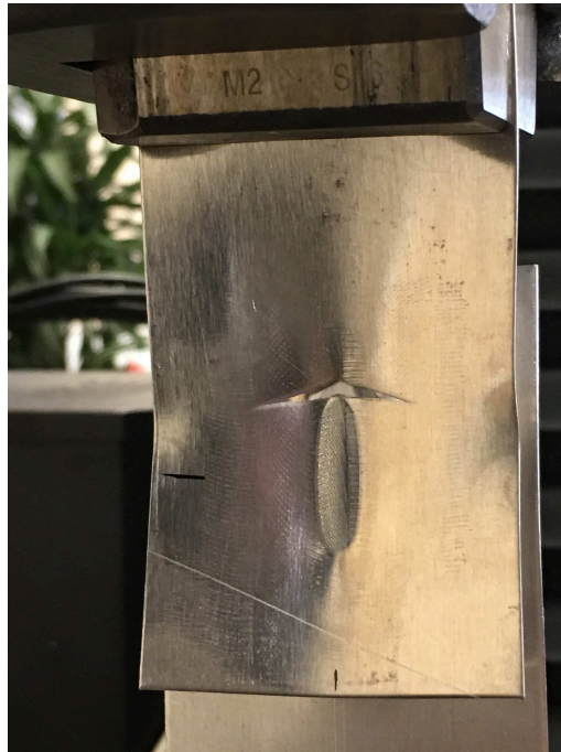
Figure 3.17: 5754 sheet teared during quasi-static lap shear test
