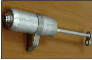
Figure 1.33: MPW application for automotive A/C receiver-dryer [62]
