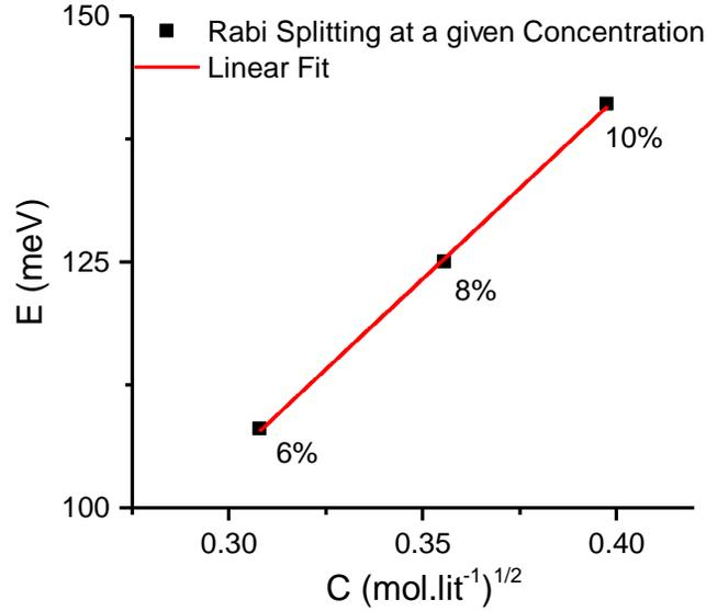
**Figure 4.9:** Variation of the Rabi splitting as a function of the square root of Ce6 concentration in DMF. The black squares are the Rabi splitting value corresponding to each concentration (6%, 8%, and 10% in weight in DMF), and the red line is their linear fit.
