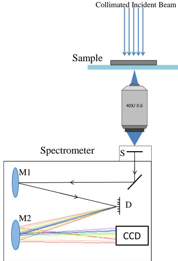
**Figure 3.18:** Schematic representation of the acquisition of transmission spectra showing the passage of the incident beam through the sample towards different parts of the system: the microscope objective, the spectrometer, and finally the CCD camera.
