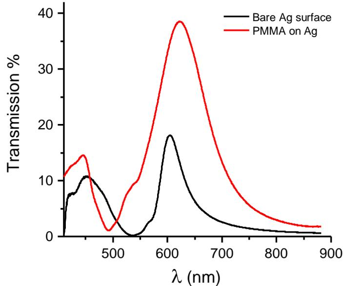
**Figure 3.10:** The zero-order transmission spectra at normal incidence for a hexagonal hole-array ( $a_0 = 380$  nm) before (black curve) and after (red curve) the deposition of a 100 nm layer of PMMA on its surface.
