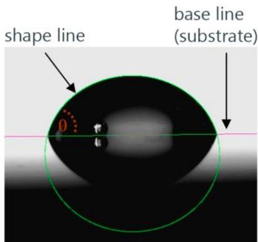
**Figure 3.20:** Image of a sessile drop taken by the DSA100 instrument with its fitted contour (shown in green). The figure is reproduced from (<https://www.kruss.de/services/education-theory/glossary/drop-shape-analysis/>)
