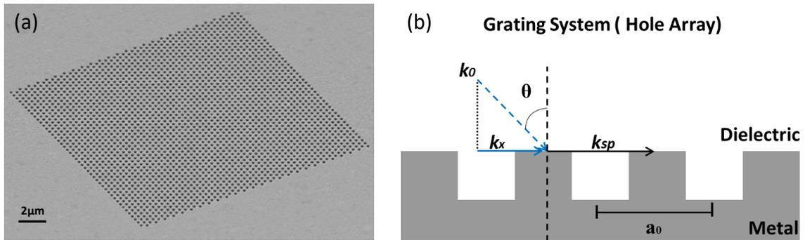
**Figure 3.6:** (a) SEM image of a hexagonal hole-array with periodicity  $a_0 = 440$  nm and hole diameter  $D = 200$  nm milled in  $t = 200$  nm thick Ag film. (b) Schematic representation of  $k_{SP}$  the grating system of periodicity  $a_0$ , showing the propagation wavevector of SPPs ( $k_{SP}$ ) generated by the horizontal component of the incident beam  $k_x$ .
