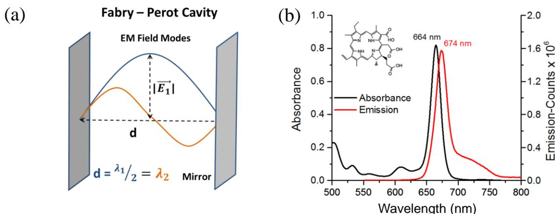
**Figure 4.3:** (a) Schematic illustration of the amplitude of the first and second Fabry-Perot (FP) cavity modes confined between two metallic mirrors. (b) Absorbance and emission spectra of Chlorin e6 in DMF and its molecular structure.
