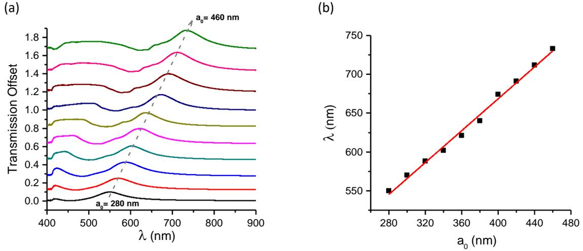
**Figure 3.8:** (a) The zero-order transmission spectra at normal incidence of hexagonal hole-arrays with varying periodicities ( $a_0$ ) from 280 nm to 460 nm milled in Ag film. The grey dashed arrow marks the peaks of the (1, 0)<sub>g</sub> modes. (b) The wavelength of the (1, 0)<sub>g</sub> SPPs resonances as a function of the array periodicity. The red line is a linear fit.
