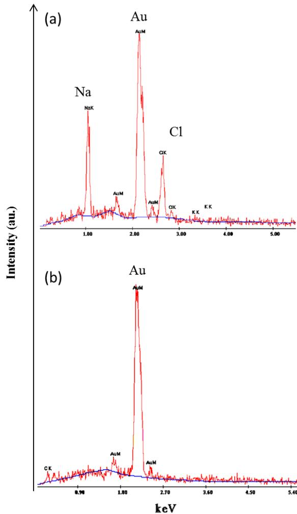
**Figure 3.28:** EDX analysis spectra showing the elemental analysis on sample of Figure 3.25 (a) when probing the features (b) when probing the Au surface away from features. The blue curve represents the background signal.
