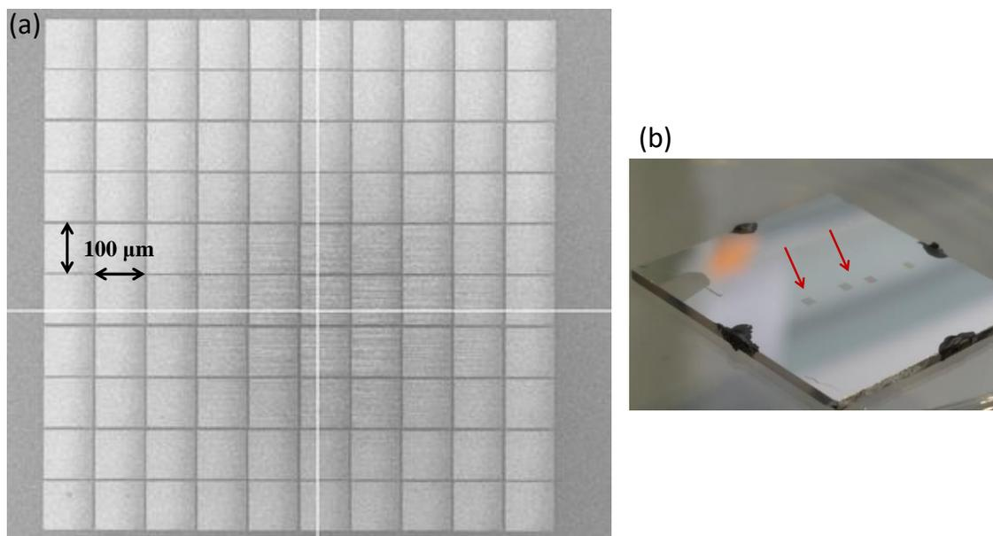
**Figure 3.21:** (a) SEM image of a  $\sim 1$  mm<sup>2</sup> large plasmonic array milled in 120 nm Ag film by using Auriga FIB machine. The small squares are identical hexagonal hole-arrays ( $a_0 = 250$  nm,  $D = 120$  nm) separated by 5 μm from each side. (b) A captured photo for the sample carrying arrays different periodicities indicated by the red arrows.
