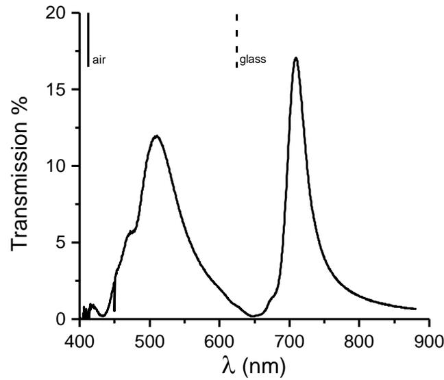
**Figure 3.7:** Zero-order transmission spectra of hole-array (square periodicity) at normal incidence. The array is milled on Ag film with periodicity 500 nm. The vertical solid and dashed lines correspond to the theoretical  $(1, 0)$  SP resonances at the air-metal and glass-metal interfaces respectively (see text).
