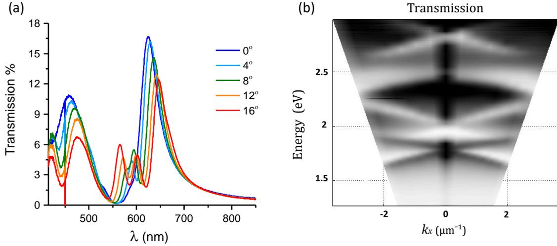
**Figure 3.9:** (a) The zero-order transmission spectra as a function of incident angle of the light in TM mode. Spectra were taken every  $4^\circ$  up to  $16^\circ$  for hexagonal array in Ag ( $a_0 = 400$  nm, hole diameter = 205 nm, film thickness = 200 nm). (b) The energy-momentum dispersion of the same spectra present in (a) in addition to their symmetric values for negative angles. The bright lines represent peaks and dark ones represent dips.
