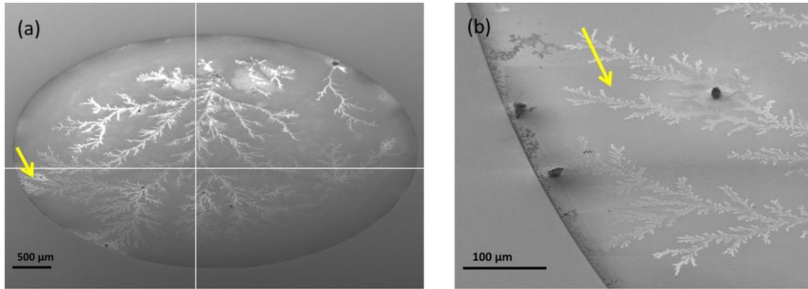
**Figure 3.26:** SEM image of the feature present in Figure 3.25 due to the water droplet. (a) The whole feature showing a contrast at the circumference. (b) A magnified SEM image of the area pointed by yellow arrow in (a).
