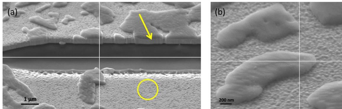
**Figure 3.27:** SEM images: (a) at 23K times magnification and shows the cross cut at the features. A clear contrast between the original Au film and the features is pointed by the yellow arrow. (b) At 90K times magnification, showing the area inside the yellow circle of (a) and highlighting the roughness modification to the surface imposed by the features.
