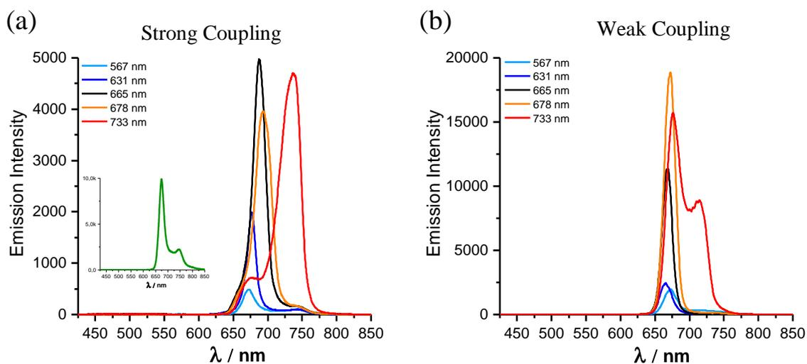
**Figure 4.8:** Emission spectra of Ce6 in DMF in cavities obtained at normal incidence for (a) high concentration (strong coupling regime) and (b) low concentration (weak coupling regime) and for different cavity detunings (indicated by the cavity peak wavelengths in neat DMF, 665 nm the resonant case). The inset in (a) is the emission spectrum of Ce6 at high concentration taken from a one-mirror channel.
