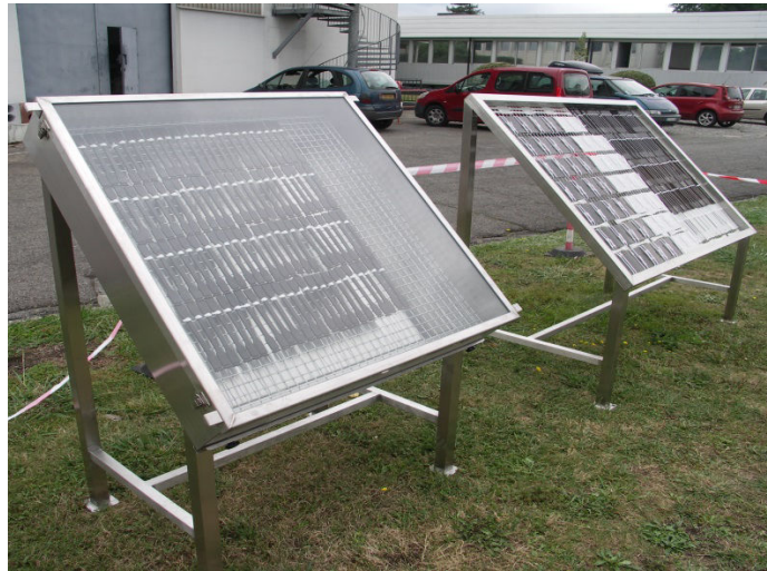
Figure 2 - Exterior and under glass exposure racks
