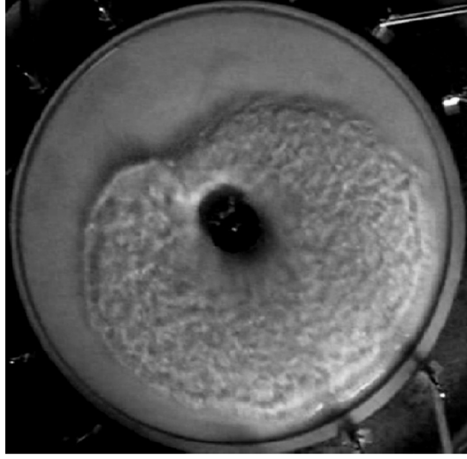
Figure 1: The shape of the rotating hydraulic jump observed in the SWASI experiment. The rotating singular (angular) point occurs as a result of non-linear behavior of the free surfaces.
