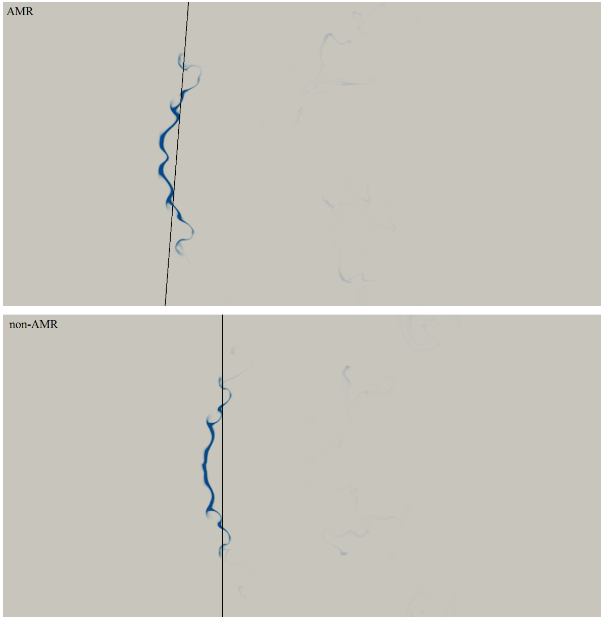
Figure 4.15: Two different magnified views of the simulation of the atomization of the cylindrical column by the high speed flow behind the shock wave of Mach number 1.3 in atmospheric air propagating from the left to the right. 2D simulations using the AMR (top) and non-AMR (bottom) methods (AMR using the volume fraction, mixture pressure and mixture velocity variations. Results are shown at time 2,000\mu s with volume fraction visualization. Drift of the AMR results is observable due to non-symmetrical amplification.
