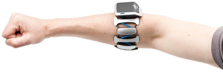
Figure 3.2. – VibroTac, brassard vibrotactile ( Schatzle, Ende, Wusthoff et al. 2010 ).
