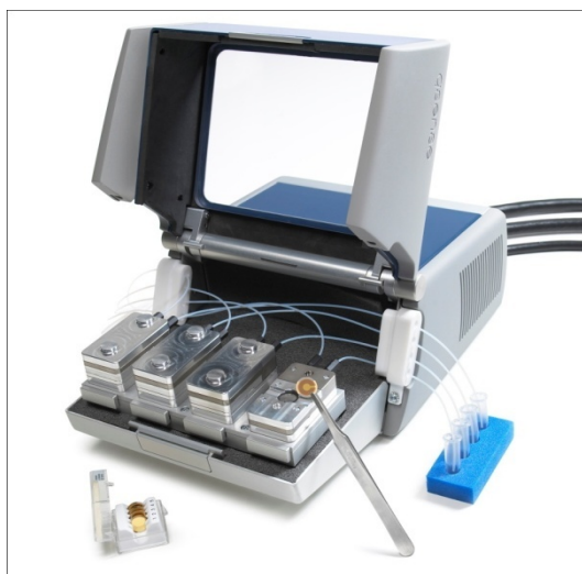
Fig. 2.24. Scheme of E4 QCM-D system adjusted for flow mode
