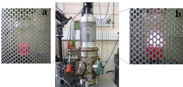
Fig.1. (Color on line) Plasma enhanced chemical vapour deposition, PECVD Bell jar reactor, (a) during thermal annealing, (b) during hydrogen plasma treatment.
