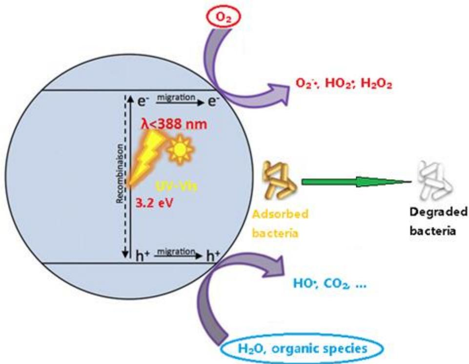
Fig 6: Schematic view of photocatalytic reactions occurring with activated  $\text{TiO}_2$ .<sup>111</sup>
