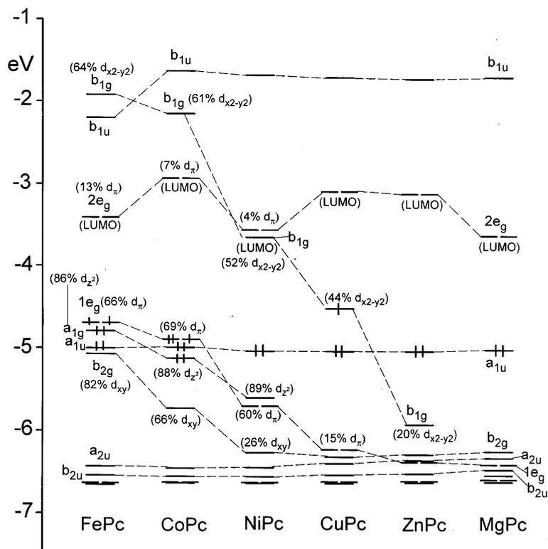
**Figure 5.3: The outer orbitals energy levels of MPcs.** The result of DFT calculation revealing the HOMO of FePc to have a high degree of Fe- $d$  character. By increasing the atomic number of a metal ion the HOMO of MPc becomes more Pc determined. The orbital occupancy in percentage is indicated in parentheses. The figure taken from ref. 299.
