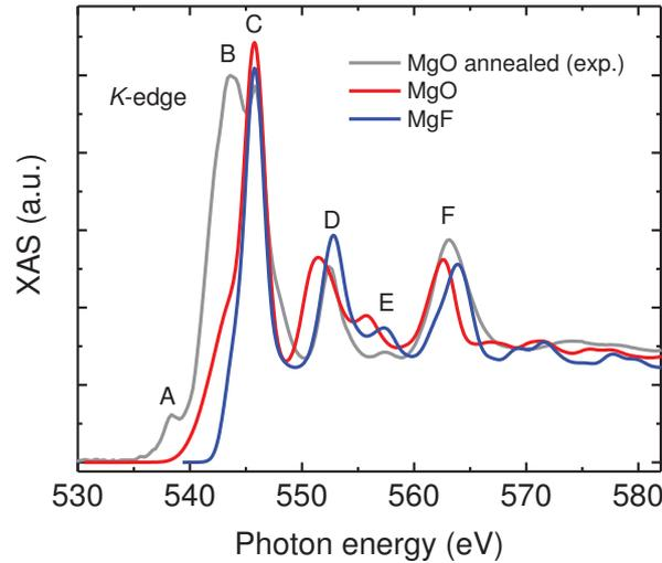
**Figure 4.33: Theoretical XAS spectra of MgO and MgF.** The result of calculation for the  $K$ -edge shape of the oxygen (fluorine) within MgO (MgF). The spectra are energy-shifted and compared to the experimental data acquired on annealed CoFeB/MgO stack. The peaks C, D, E, and F well reproduce the experimental result. The substitution of the oxygen sites with fluorine preserves the same set of allowed dipolar transitions.
