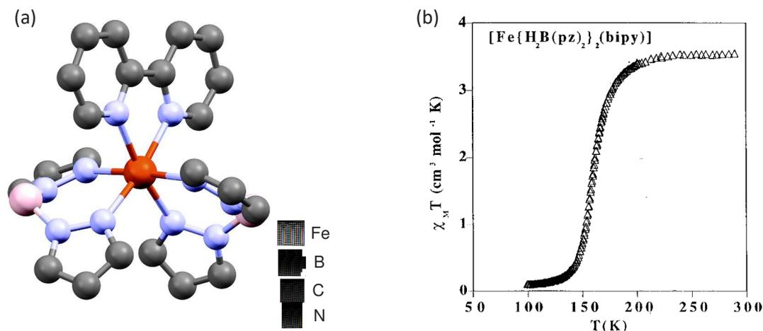
**Figure 7.35: Fe(bpz)<sub>2</sub>(bpy).** (a) Molecular model of Fe(bpz)<sub>2</sub>(bpy). The crystallographic data used for visualisation was taken from ref. 409. The hydrogen atoms were omitted for clearance. (b) Thermal spin transition of Fe(bpz)<sub>2</sub>(bpy) measured with a pendulum-type susceptometer. Figure taken from ref. 402.
