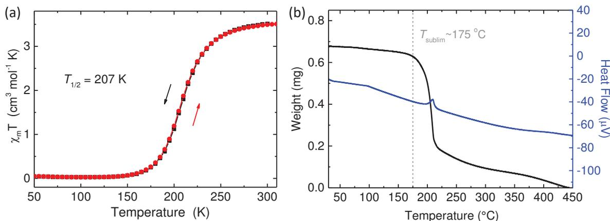
**Figure 7.37: Spin transition and sublimability of  $\text{Fe}(\text{bpz})_2\text{C}_1\text{-bpy}$ .** (a) Magnetic moment measurement as a function of temperature acquired with SQUID on  $\text{Fe}(\text{bpz})_2\text{C}_1\text{-bpy}$  powder. The new material preserves the complete spin transition of parent complex. (b) Thermogravimetric analysis of  $\text{Fe}(\text{bpz})_2\text{C}_1\text{-bpy}$  proving the sublimability of the compound.
