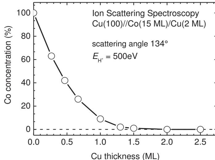
**Figure 5.12:** Ion scattering spectroscopy measurement of **Cu(100)//Co(15 ML)/Cu(2 ML)**. The Co concentration reaches 10% for 1 ML of Cu coverage and becomes zero for thicknesses above 1.3 ML. The measurement was performed with  $H^+$  ions with an energy of 500 eV and a scattering angle of  $134^\circ$ .
