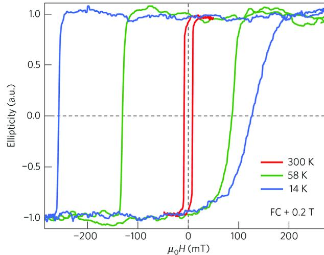
**Figure 5.8: Exchange bias of Co induced by organic MnPc layer.** Magnetic hysteresis loops as determined by MOKE experiment on stack Cu(100)//Co(20 ML)/MnPc(25 ML)/Au(20 ML) for  $T = 300$  K, 58 K, and 14 K. The curves acquired at  $T = 58$  K and 14 K were subjected to field cooling with  $H = +0.2$  T. Figure taken from ref. 21.
