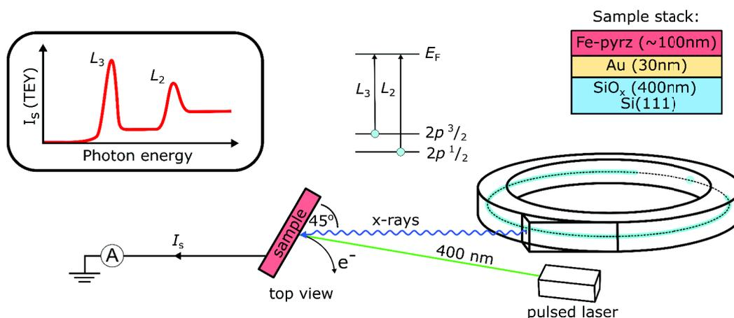
**Figure 7.6:** Studies of the LIESST effect in the Fe-pyrz film at the TEMPO beamline. Top view of the experimental set-up geometry with a pumping 400 nm pulsed laser (alternatively white LED). The spectra were recorded in total electron yield detection at  $45^\circ$  x-ray incidence.
