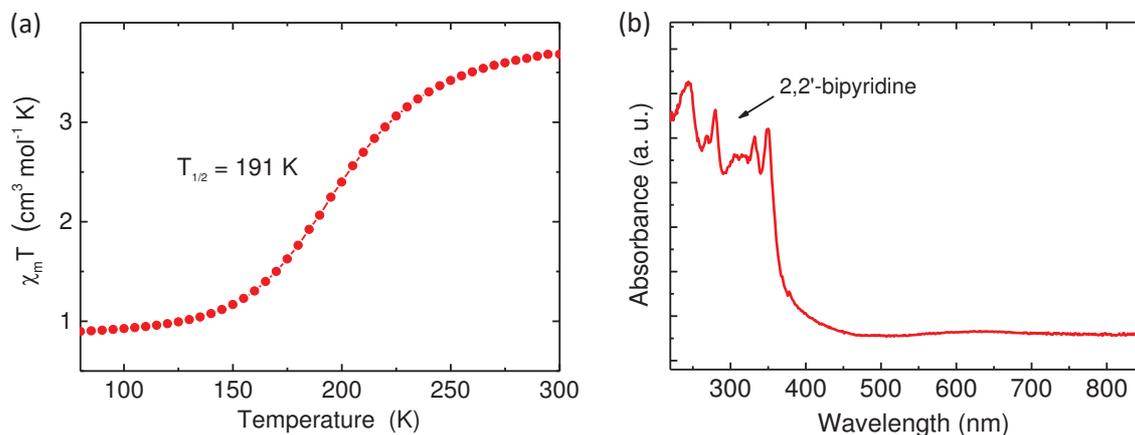
**Figure 7.44: SCO and sublimability of Fe(bpz)<sub>2</sub>Py-bpy.** (a) Magnetic susceptibility measurement as a function of temperature measured with SQUID on Fe(bpz)<sub>2</sub>Py-bpy powder confirming the preserved SCO with a gradual transition and  $T_{1/2} = 191 \text{ K}$ . (b) Absorbance of a sublimed Fe(bpz)<sub>2</sub>Py-bpy thick film exhibiting a proper spectra of the bipyridine ligands and the preservation of the octahedral Fe(II) environment.
