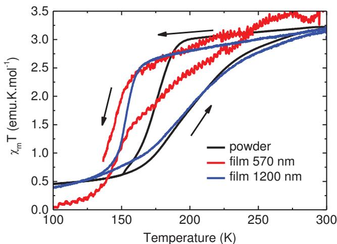
**Figure 7.4: SCO of the Fe-pyrz powder and sublimed film.** Magnetic susceptibility as a function of temperature for the Fe-pyrz powder and two thick films sublimed onto SiO<sub>x</sub>. Note the preserved SCO and the shift in transition temperature for the thick film samples. The measurement was performed with SQUID at magnetic field  $H = 4$  T. The arrows indicate a field sweep direction. Figure taken from ref. 31.
