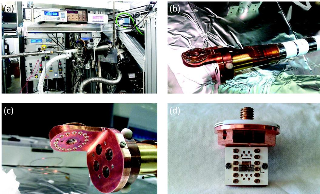
**Figure 4.26: Test measurements of V<sup>2</sup>TI.** (a) V<sup>2</sup>TI mounted at the side port of the cryo-magnet endstation of the DEIMOS beamline. (b)-(c) Outside picture of the insert's head. (d) Sample holder with mounted chip and the sample containing MgO-based MTJs.
