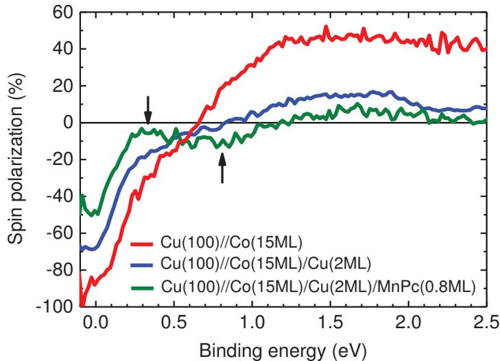
**Figure 5.14: Spin polarization for the consecutive steps of the stack fabrication.** Spin polarization calculated from data in Fig. 5.13 according to Equation 1.2. Note the attenuation of the signal after deposition of Cu and MnPc. The features marked by the arrows originate from the deposition of the MnPc molecules and cannot be explained by a simple attenuation of the Co induced valence band structures.
