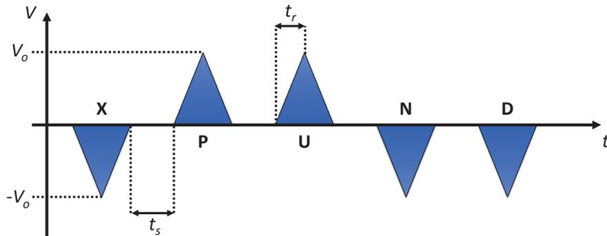
**Figure 6.4: PUND measurement.** Sequence of voltage pulses applied during PUND (P - positive, U - up, N - negative, D - down) measurement. We used pulses of maximum bias voltage  $V_0 = \pm 10\text{ V}$ , rise time  $t_r = 250\ \mu\text{s}$  and separation between the pulses  $t_s = 1\text{ s}$ . "X" denotes the pre-pulse applied to ensure the procedure to be always performed at the same conditions.
