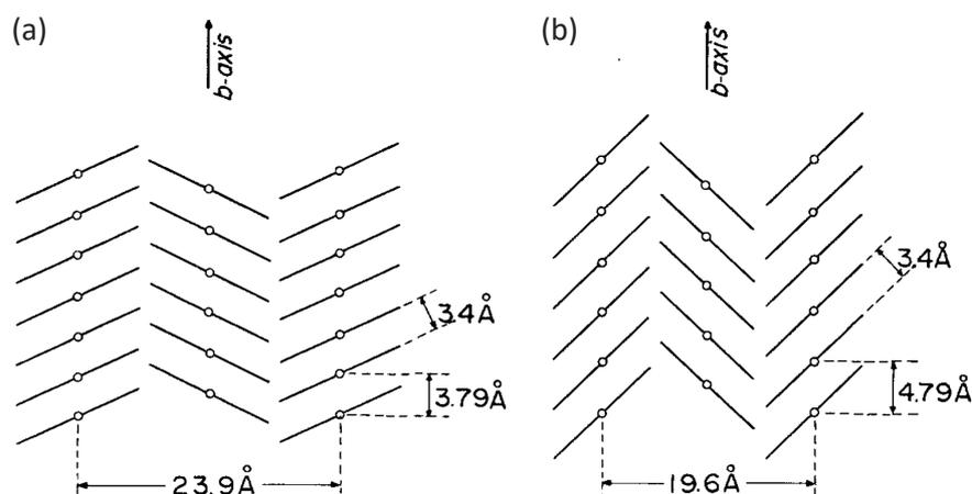
**Figure 5.2: Polymorphism of CuPc.** Two polymorphic (a)  $\alpha$ , and (b)  $\beta$  forms of CuPc stacking arrangement with a  $65^\circ$  and  $45^\circ$  angle of molecular plate to b-axis respectively. Figure taken from ref. 294.
