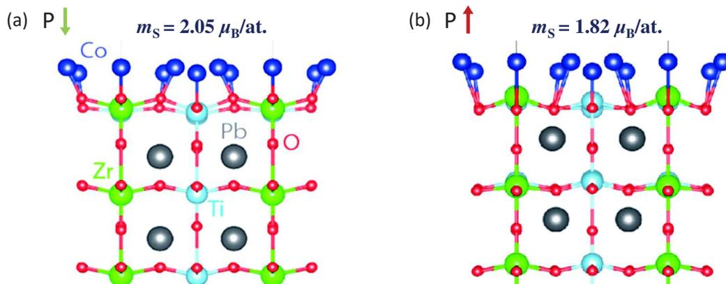
**Figure 6.2: Magnetoelectric coupling at PZT/Co interface.** The first principles calculations of 1 ML of Co atop PZT for two ferroelectric polarization states  $P \uparrow$  and  $P \downarrow$ . Formation of the Co-O bonds at the interface and the interatomic distance variation upon the FE polarization reversal alters the Co spin magnetic moment from  $2.05 \mu_B/\text{atom}$  for upward to  $1.82 \mu_B/\text{atom}$  for downward polarization. Figure taken from ref. 28.
