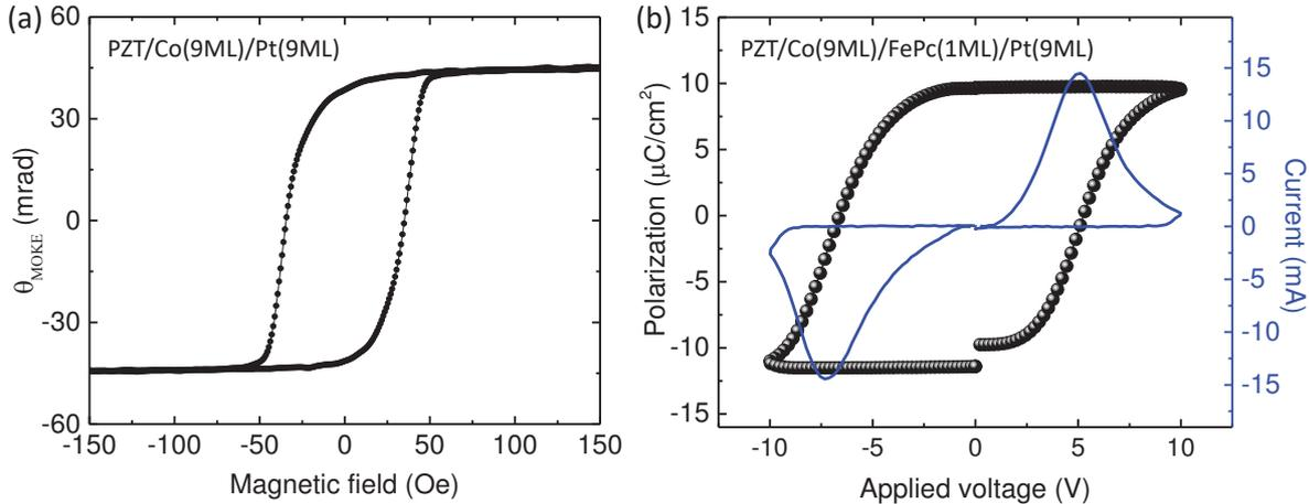
**Figure 6.5: Ferromagnetic and ferroelectric testing of the magnetoelectric-organic device.** (a) Result of MOKE measurement performed on PZT/Co(9ML)/Pt(9ML) test sample confirming proper ferromagnetic properties of Co layer. (b) Result of PUND measurement on complete PZT/Co(9ML)/FePc(1ML) device. The peaks in the  $I(V)$  curves reveal two ferroelectric states of the device with polarization of  $\sim \pm 12 \mu\text{C}/\text{cm}^2$ .
