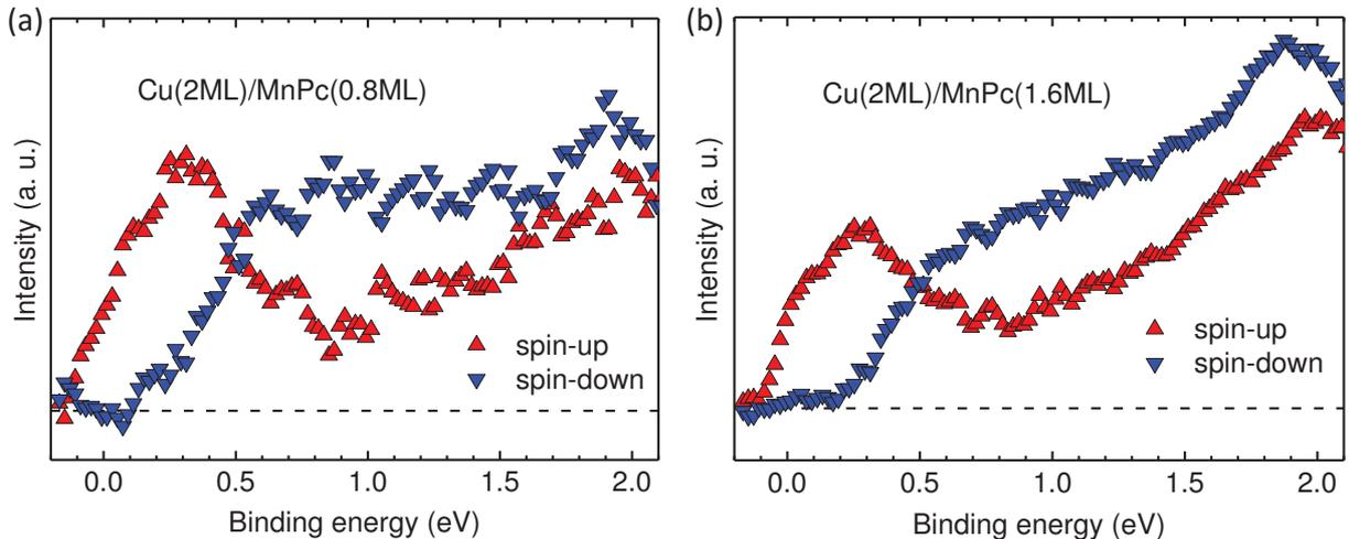
**Figure 5.15: Spin-resolved electron distribution curves for Cu(2 ML)/MnPc interface.** Spin-resolved difference spectra, *i.e.*, the spin-resolved spectra of Co/Cu(2 ML)/MnPc after subtraction of the suitably normalized referential curves acquired on Co/Cu(2 ML) stack, for (a) 0.8 ML and (b) 1.6 ML of MnPc thickness. Note a strong positive spin polarization at the Fermi level and its reversal at  $\sim 0.5$  eV.
