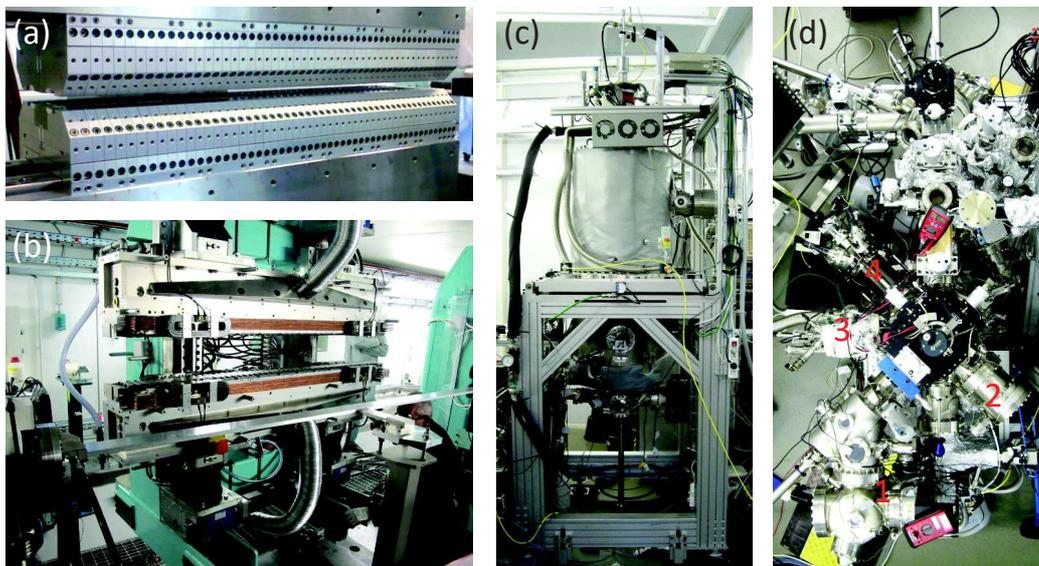
**Figure 4.22: DEIMOS beamline.** (a) Apple II HU52, and (b) EMPHU65 undulators, (c) cryo-magnet endstation, and (d) sample preparation environment of the DEIMOS beamline. 1 - variable temperature Omicron STM, 2 - LEED apparatus, 3 - EFM-3 metal evaporator, 4 - AES analyzer.<sup>237</sup>
