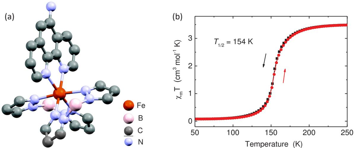
**Figure 7.19: Fe(bpz)<sub>2</sub>NH<sub>2</sub>-phen.** (a) Molecular model of Fe(bpz)<sub>2</sub>NH<sub>2</sub>-phen. Note the position of the NH<sub>2</sub> group by comparing with the model in Fig. 7.15 (a). (b) Magnetic moment measurement as a function of temperature for the Fe(bpz)<sub>2</sub>NH<sub>2</sub>-phen powder measured by SQUID.
