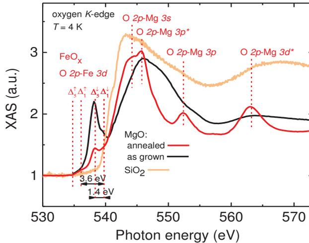
**Figure 4.29: The referential XAS spectra of MgO and  $\text{SiO}_2$ .** X-ray absorption acquired on the annealed and non-annealed CoFeB/MgO, and glass/ $\text{SiO}_2$  non-processed stacks. The peak assignment is based on the literature<sup>37,259</sup> and reflects the allowed transitions from oxygen 1s core to the final state indicated in red.
