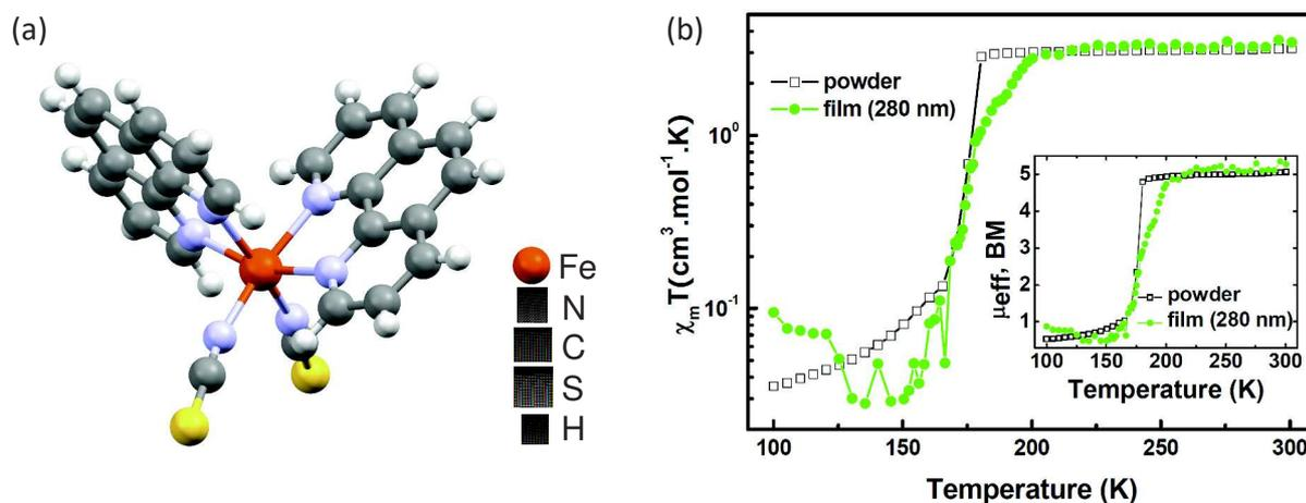
**Figure 7.1: Fe(phen)<sub>2</sub>(NCS)<sub>2</sub> (Fe-phen).** (a) Model of the Fe-phen molecule. (b) Magnetic susceptibility as a function of temperature for the Fe-phen powder and a 280 nm thick UHV sublimed film. Measurement performed with SQUID. Figure taken from ref. 379.
