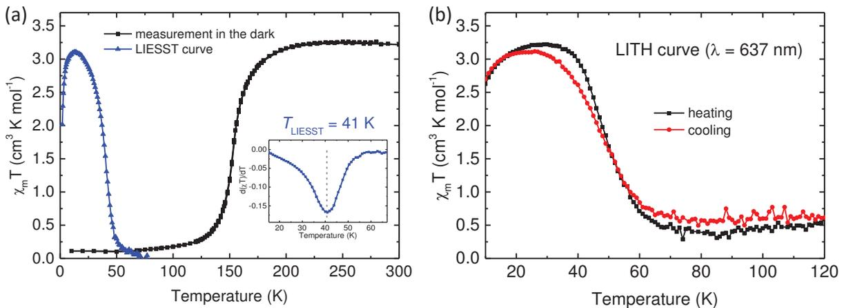
**Figure 7.20: LIESST and LITH of Fe(bpz)<sub>2</sub>NH<sub>2</sub>-phen powder.** (a) Thermal spin transition along with the LIESST curve measured on Fe(bpz)<sub>2</sub>NH<sub>2</sub>-phen powder. The derivative  $d(\chi T)/dT$  (inset) was used to determine  $T_{\text{LIESST}}$ . (b) Light induced thermal hysteresis (LITH) curve obtained by heating up and cooling down the sample with a permanent irradiation by a 637 nm laser.
