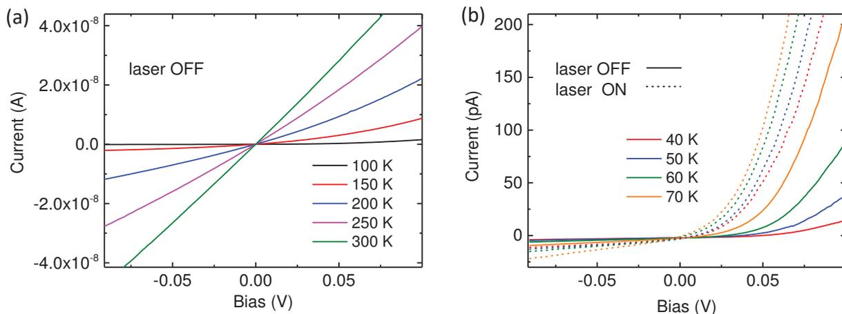
**Figure 7.30: Current-voltage characteristics of  $\text{Fe}(\text{bpz})_2\text{NH}_2\text{-phen}$  junction.** (a) Selected  $I(V)$  curves for a few temperatures revealing nearly linear evolution at RT and increasing non-linearity with decreasing temperature. (b)  $I(V)$  curves highlighting the rectifying character of the junction at low temperatures. Note the impact of the laser radiation (dashed lines) strongly pronounced on the positive bias branch.
