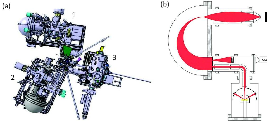
**Figure 4.20: Measurement endstations of the CASSIOPEE beamline.** (a) Top view of the spin-resolved (1) and angle-resolved (2) photoemission spectroscopy dedicated endstations along with the preparation MBE chamber (3) at the CASSIOPEE beamline. (b) Cross section of a Scienta SES 2002 hemispherical electron-energy analyzer coupled to a custom made Mott detector installed at the SR-PES endstation of the beamline.
