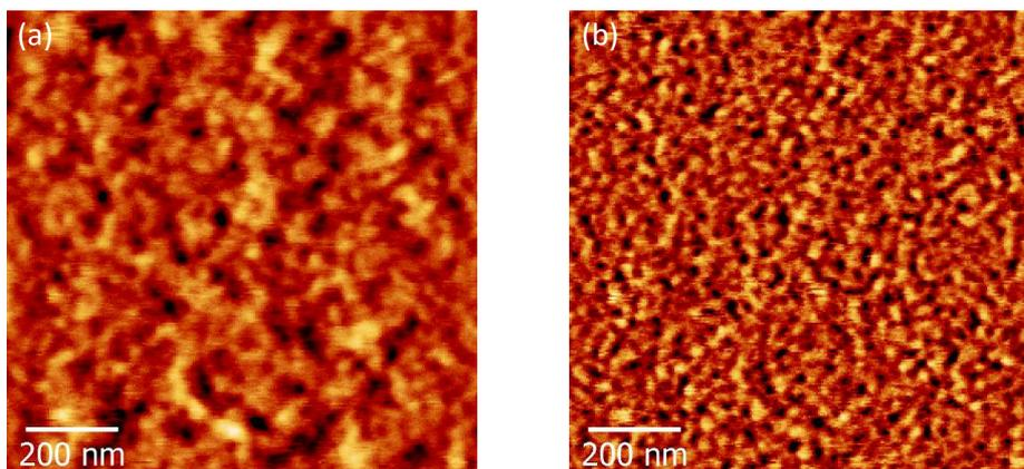
**Figure 7.26: Morphology of  $\text{Fe}(\text{bpz})_2\text{NH}_2\text{-phen}$  film on silica and platinum surface.** Surface topography measurement by RT ambient pressure AFM in tapping mode of a 40 nm thick film of  $\text{Fe}(\text{bpz})_2\text{NH}_2\text{-phen}$  sublimed onto (a)  $\text{Si}/\text{SiO}_x(400\text{ nm})$ , and (b)  $\text{Si}/\text{SiO}_x(400\text{ nm})/\text{Cr}(2\text{ nm})/\text{Pt}(13\text{ nm})$ .
