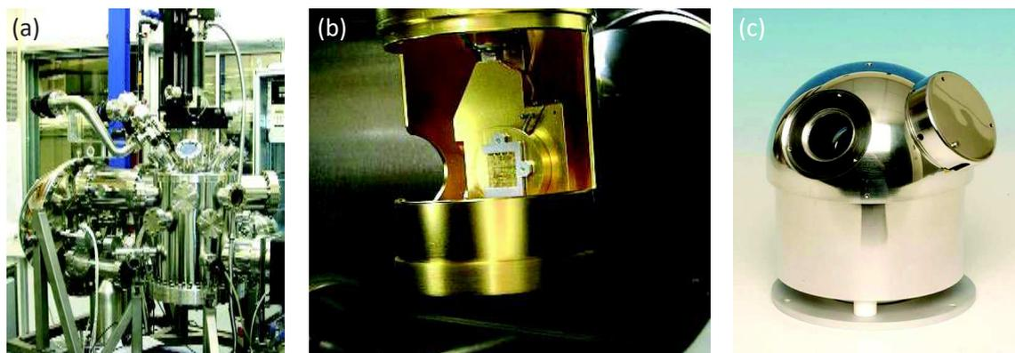
**Figure 4.21: SR-PES endstation of the CASSIOPÉE beamline.** Picture of (a) the SR-PES-dedicated endstation, (b) the sample inside the SR-PES measurement chamber (in the back visible input of the energy-analyzer), and (c) the Mott detector with one of the channelplates removed. Pictures taken from ref. 235 and 236.
