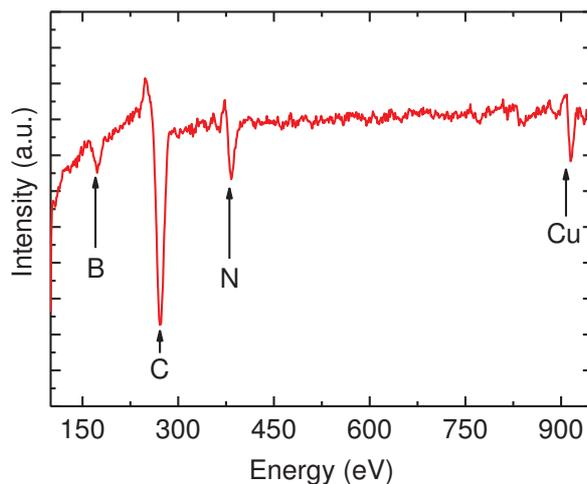
**Figure 7.11: AES of Cu(100)//Fe-pyrz(2 nm).** Result of Auger electron spectroscopy measurement performed on Cu(100)//Fe-pyrz(2 nm) proving the presence of the molecule constituting elements (boron, carbon and nitrogen) on the surface. Due to only one Fe site per molecule the signal arising from the Fe ions could not be resolved.
