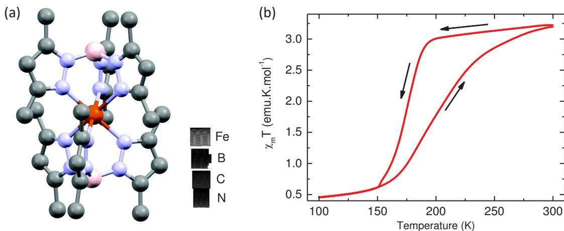
**Figure 7.3:**  $\text{Fe}\{[3,5\text{-dimethylpyrazolyl}]_3\text{BH}_2\}_2$  (**Fe-pyraz**). (a) Molecular model of Fe-pyraz. The hydrogen atoms are omitted for clearance. (b) Magnetic susceptibility of the Fe-pyraz powder as a function of temperature measured by SQUID at  $H = 0.5$  T.
