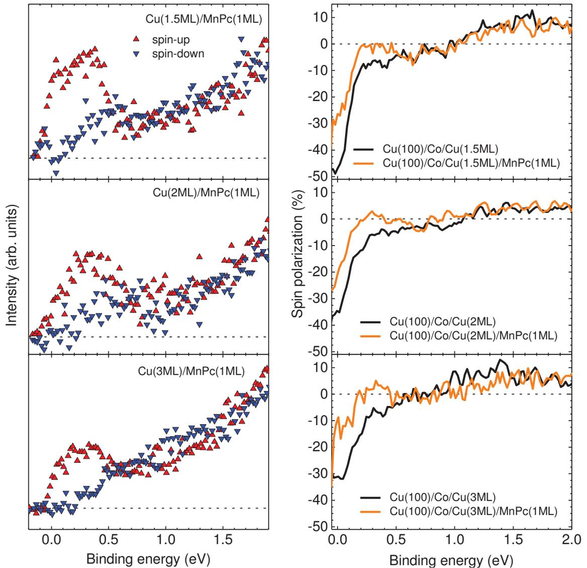
**Figure 5.16: Spin polarization of  $\text{Cu}(d_{\text{Cu}})/\text{MnPc}(1 \text{ ML})$  for different Cu thicknesses.** Difference spectra of the Cu/MnPc(1 ML) interface (left) and spin polarization of the untreated (*i.e.*, before subtraction) spin-resolved spectra (right) for  $d_{\text{Cu}} = 1.5 \text{ ML}$  (top panels), 2 ML (middle panels) and 3 ML (bottom panels).
