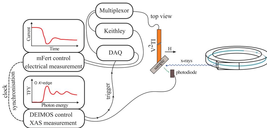
**Figure 4.27: Integrated XAS and electrical measurement with use of the V<sup>2</sup>TI.** The mFert bench was employed to record the device current (resistance) vs. time and the DEIMOS control station to acquire the XAS spectra. The time-stamp synchronization between the two measurement lines allowed a simultaneous measurement in the current - photon energy space.
