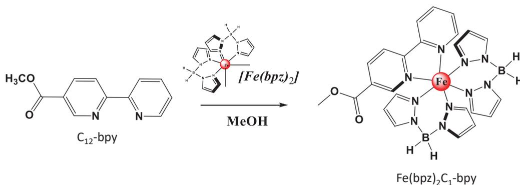
**Figure 7.36: Synthesis of Fe(bpz)<sub>2</sub>C<sub>1</sub>-bpy.** C<sub>1</sub>-bpy is used as a precursor for the functionalizable Fe(bpz)<sub>2</sub>C<sub>1</sub>-bpy complex via a carboxylic group -COOH.
