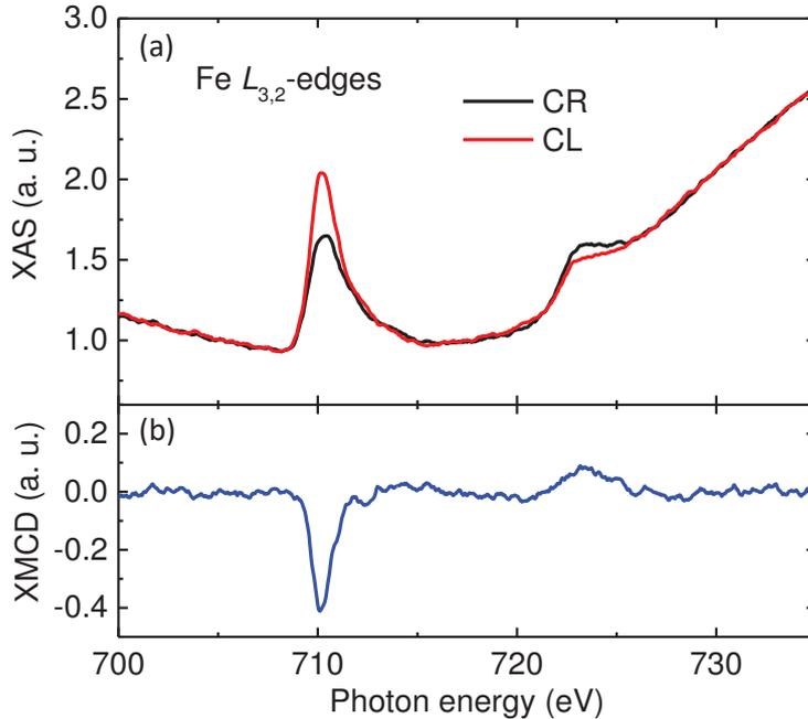
**Figure 6.9: XAS and XMCD at the  $L_{3,2}$ -edges of Fe in FePc molecules.** (a) X-ray absorption spectra acquired for both circular left (CL) and right (CR) x-ray polarization at the Fe  $L_{3,2}$ -edges of Fe in FePc, and (b) the resulting XMCD. A non-zero dichroic signal originates from the FM coupling of the Fe magnetic moments to the underlying Co. The spectra were acquired in total electron yield mode at both directions of the magnetic field  $|H| = 0.1$  T.
