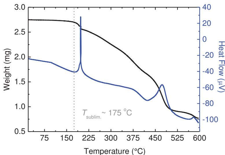
**Figure 7.21: Thermogravimetric analysis of Fe(bpz)<sub>2</sub>NH<sub>2</sub>-phen powder at ambient Ar pressure.** The powder weight loss and heat release at  $T \sim 175$  °C proves that Fe(bpz)<sub>2</sub>NH<sub>2</sub>-phen undergoes thermal sublimation.
