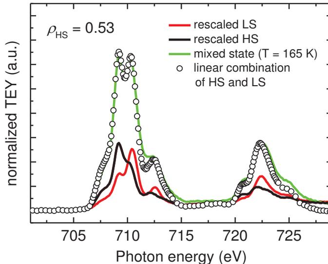
**Figure 7.7: HS proportion determination by fitting the referential spectra.** XAS at the Fe  $L_{3,2}$ -edges of Fe-pyraz film acquired for the mixed state at  $T = 165$  K fitted with two normalized LS and HS referential spectra recorded at 80 K and RT respectively. The fitting yields the high spin proportion  $\rho_{\text{HS}} \sim 0.5$ .
