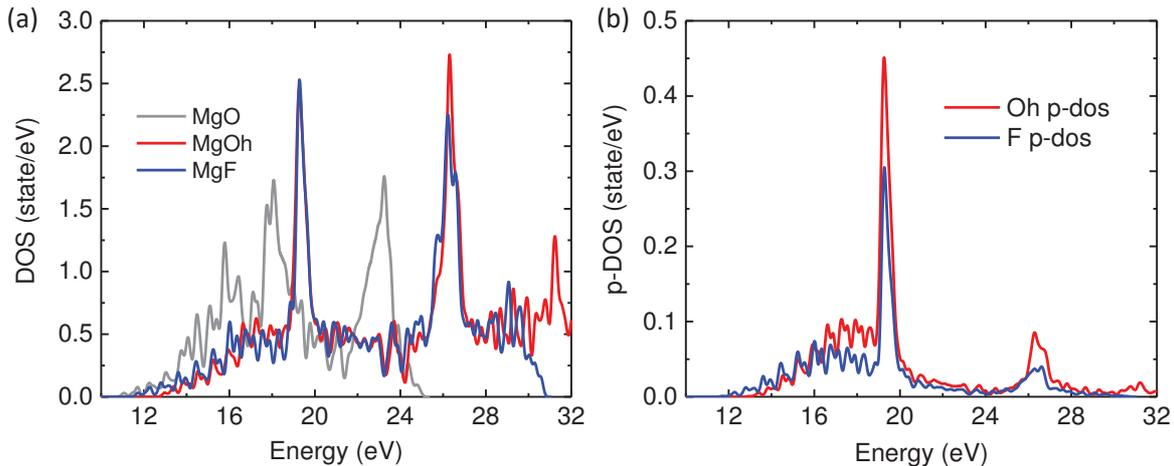
**Figure 4.34: Calculation of the MgO and MgF ground state density of states.** The total (a) and  $p$ -projected (b) conduction band DOS of MgF, MgO, and MgOh with "Oh" denoting the inclusion of the core hole.
