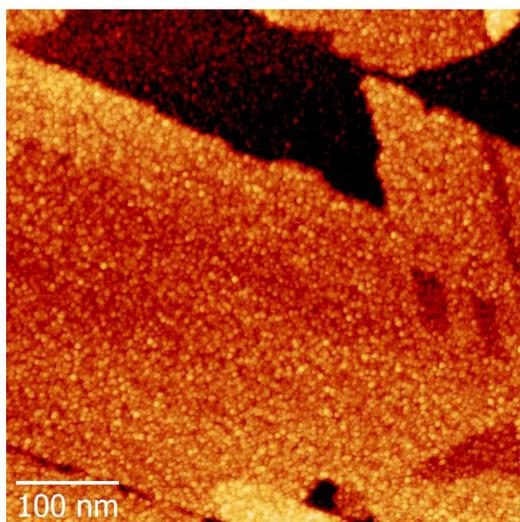
**Figure 7.13: Growth morphology of Fe-pyrz on Cu(100) at higher coverage.** Surface topography images of Cu(100)//Fe-pyrz(3.5 ML) acquired in constant current STM mode at RT. The reduced interaction of the topmost molecular layers with the substrate leads to the formation of grains. The terraces have surface roughness of rms  $\sim 0.3$  nm.  $I = 100$  pA,  $V = 1$  V.
