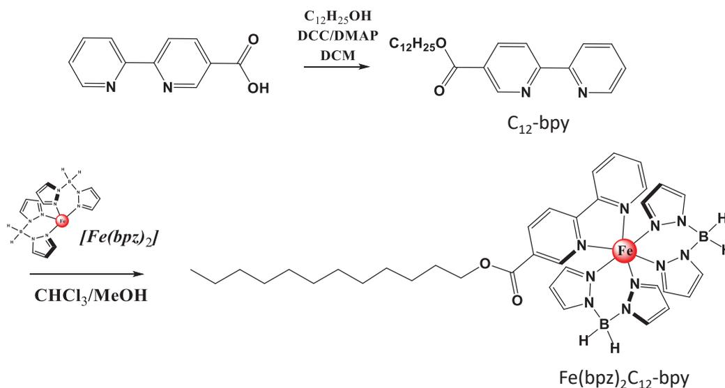
**Figure 7.38: Synthesis of  $\text{Fe}(\text{bpz})_2\text{C}_{12}\text{-bpy}$ .**  $\text{C}_1\text{-bpy}$  is extended with a linear  $\text{C}_{12}$  alkyl chain and used as a precursor to produce  $\text{Fe}(\text{bpz})_2\text{C}_{12}\text{-bpy}$  complex.
