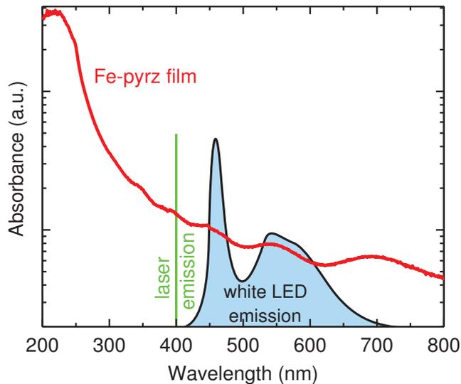
**Figure 7.9: Absorbance of the Fe-pyrz film in the ultraviolet-visible region.** Comparison of the Fe-pyrz film absorbance with the emission spectra of a white LED and a monochromatic 400 nm laser. Note that the absorption at the laser wavelength (400 nm) is  $\sim 30\%$  greater than at the main emission peak of the white LED (450 nm). The laser and white LED emission spectra are schematic and their intensities are insignificant.
