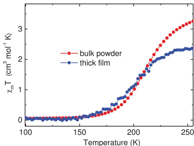
**Figure 7.40: SCO of  $\text{Fe}(\text{bpz})_2\text{C}_{12}\text{-bpy}$  thick film and powder.** Results of the SQUID measurements comparing the spin transition of the bulk powder and the sublimed thick film. Approximately 73% of the molecules in thick film undergo the transition.
