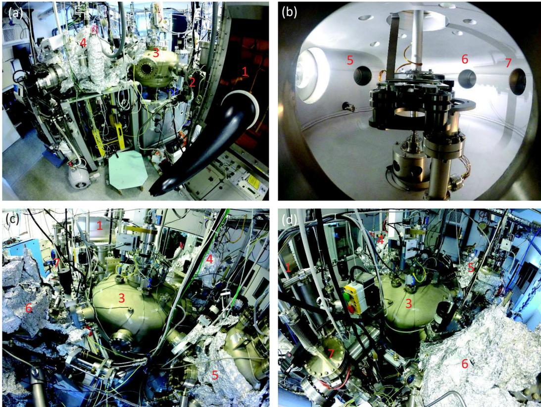
**Figure 3.2: Hybrid system.** (a) Side, and (c)-(d) top view pictures of the Hybrid system. (b) Inside of the robot chamber with a transfer arm and visible valve gates to the functional chambers. 1 - glove box, 2 - load-lock, 3 - robot, 4 - sputtering, 5 - evaporation, 6 - organic molecular beam epitaxy, and 7 - annealing chambers.
