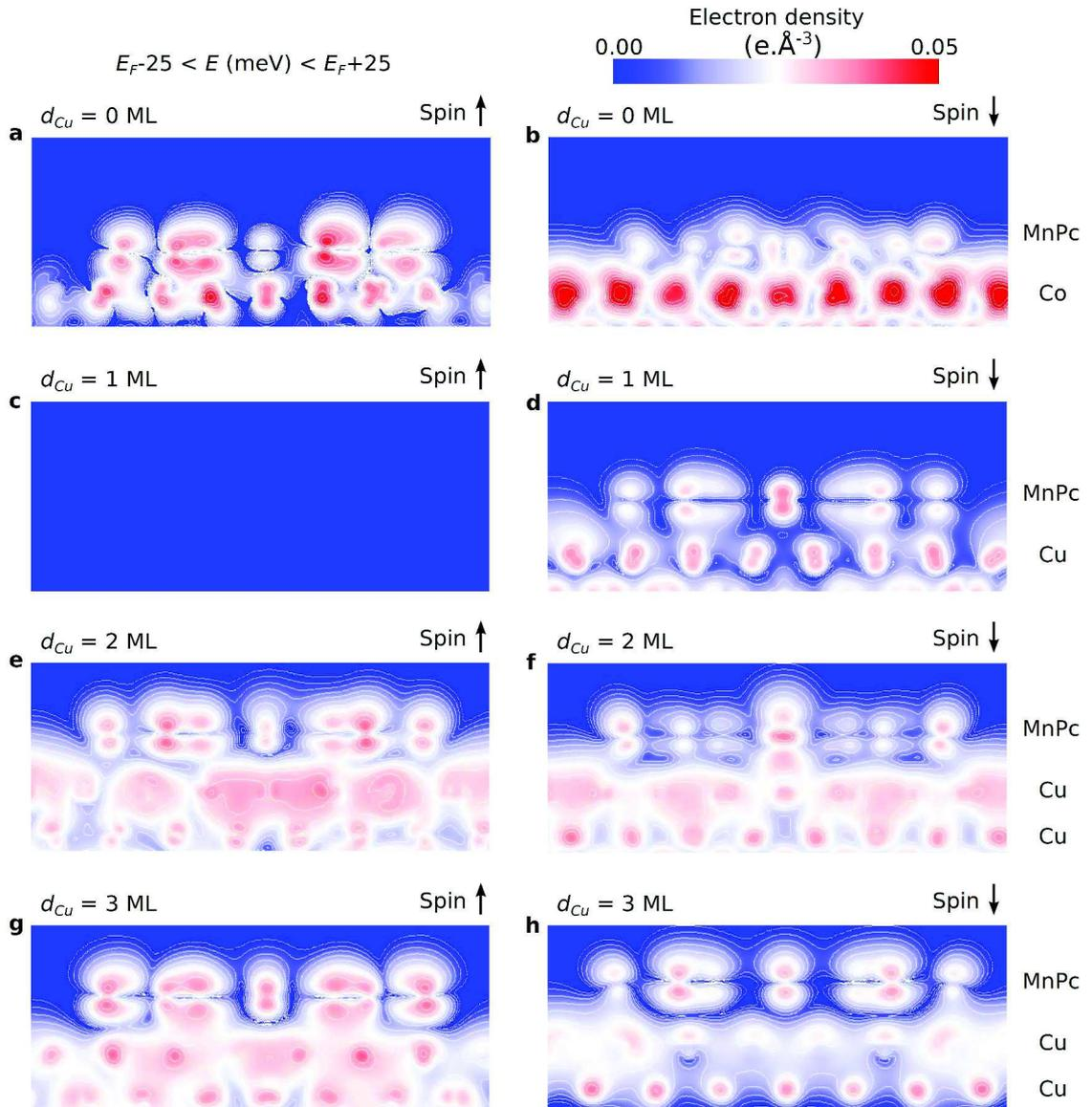
**Figure 5.17: Spin-polarized spatial DOS maps of Co/Cu/MnPc for various Cu spacer thicknesses  $d_{\text{Cu}}$ .** The calculations were performed within the  $\pm 25$  meV around the Fermi energy for (a),(b)  $d_{\text{Cu}} = 0$  ML, (c),(d)  $d_{\text{Cu}} = 1$  ML, (e),(f)  $d_{\text{Cu}} = 2$  ML, and (g),(h)  $d_{\text{Cu}} = 3$  ML. Figure taken from the Supplementary Information to ref. 349.
