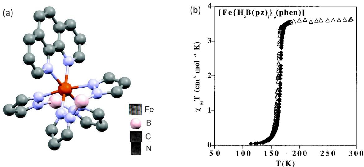
**Figure 7.15:  $\text{Fe}(\text{bpz})_2(\text{phen})$ .** (a) Molecular model of  $\text{Fe}(\text{bpz})_2(\text{phen})$ . The hydrogen atoms are omitted for clearance. (b) Thermal spin transition of the  $\text{Fe}(\text{bpz})_2(\text{phen})$  powder measured with pendulum-type susceptometer. Figure taken from ref. 402.
