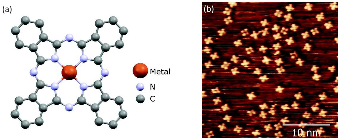
**Figure 5.1: Metal-phthalocyanine (MPc).** (a) Model of metal-phthalocyanine molecule. (b) I-const. room temperature STM image of MnPc on Cu(100) surface revealing planar adsorption of molecules on the surface. Area:  $29 \times 29 \text{ nm}^2$ ,  $I = 500 \text{ pA}$ ,  $V = -0.8 \text{ V}$ .
