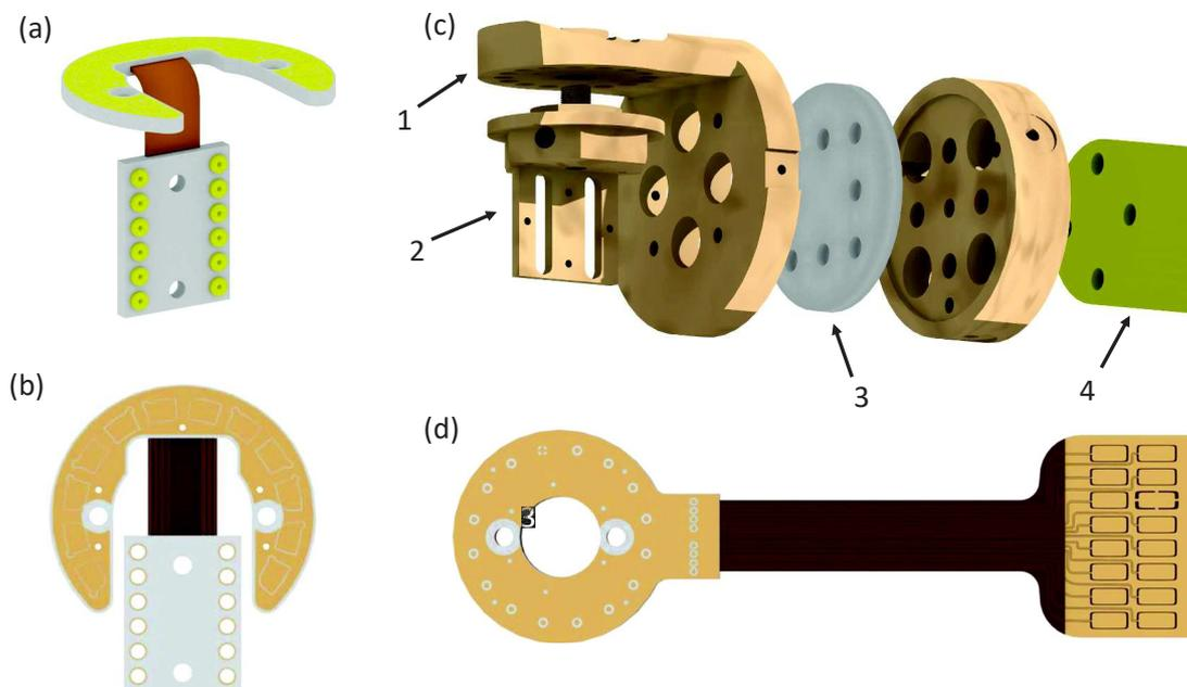
**Figure 4.24: Versatile Variable Temperature Insert (V<sup>2</sup>TI).** (a) Sample holder PCB and (b) its top view. (c) Exploded view of the insert with: 1 - head, 2 - sample holder, 3 - sapphire disk, and 4 - cold finger. (d) The top PCB of the insert's head. Figures taken from ref. 33.
