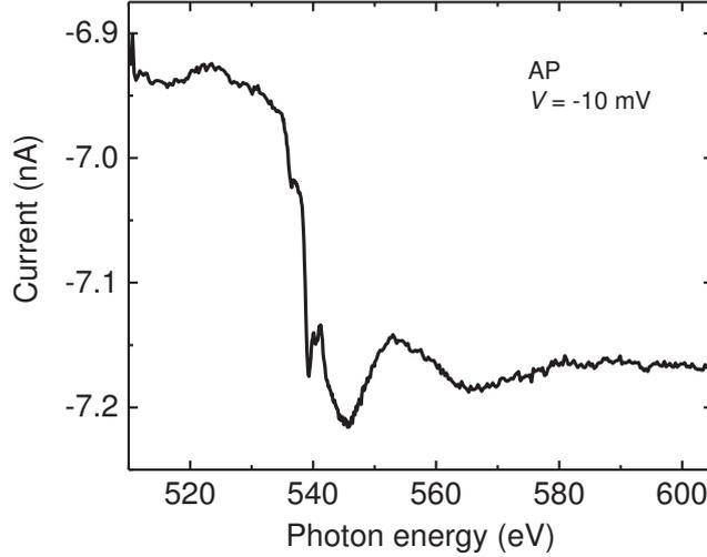
**Figure 4.31: Synchronized XAS and magnetotransport measurement.** The exemplary raw transport curve as a function of the photon energy resulting from the synchronized measurement of  $I(t)$  and  $XAS(E)$ . The large signal variation around 537 eV arises from the contribution of the photocurrent.
