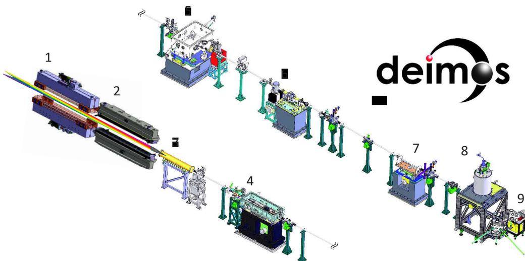
**Figure 4.23: DEIMOS beamline elements.** 1 - EMPU65, and 2 - APPLE II HU52 undulators, 3 - buffer chamber, 4 - optics chamber, 5 - monochromator, 6 - exit slits, 7 - refocusing chamber, 8 - cryo-magnet endstation, 9 - sample preparation environment. The MK2T endstation which is installed behind the cryo-magnet is not present on the drawing.<sup>237</sup>
