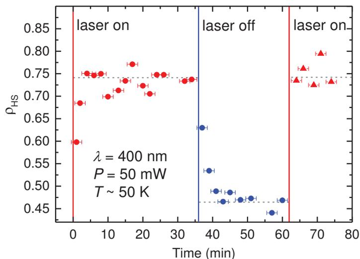
**Figure 7.10: Reversible switching of the HS proportion in the Fe-pyrz film provoked by the laser.** The high spin proportion  $\rho_{\text{HS}}$  evolution with time during the consecutive opening and closing of the 400 nm laser shutter. Note the non-zero  $\rho_{\text{HS}}$  level after relaxation (in absence of laser) resulting from the concurrent SOXIESST effect.
