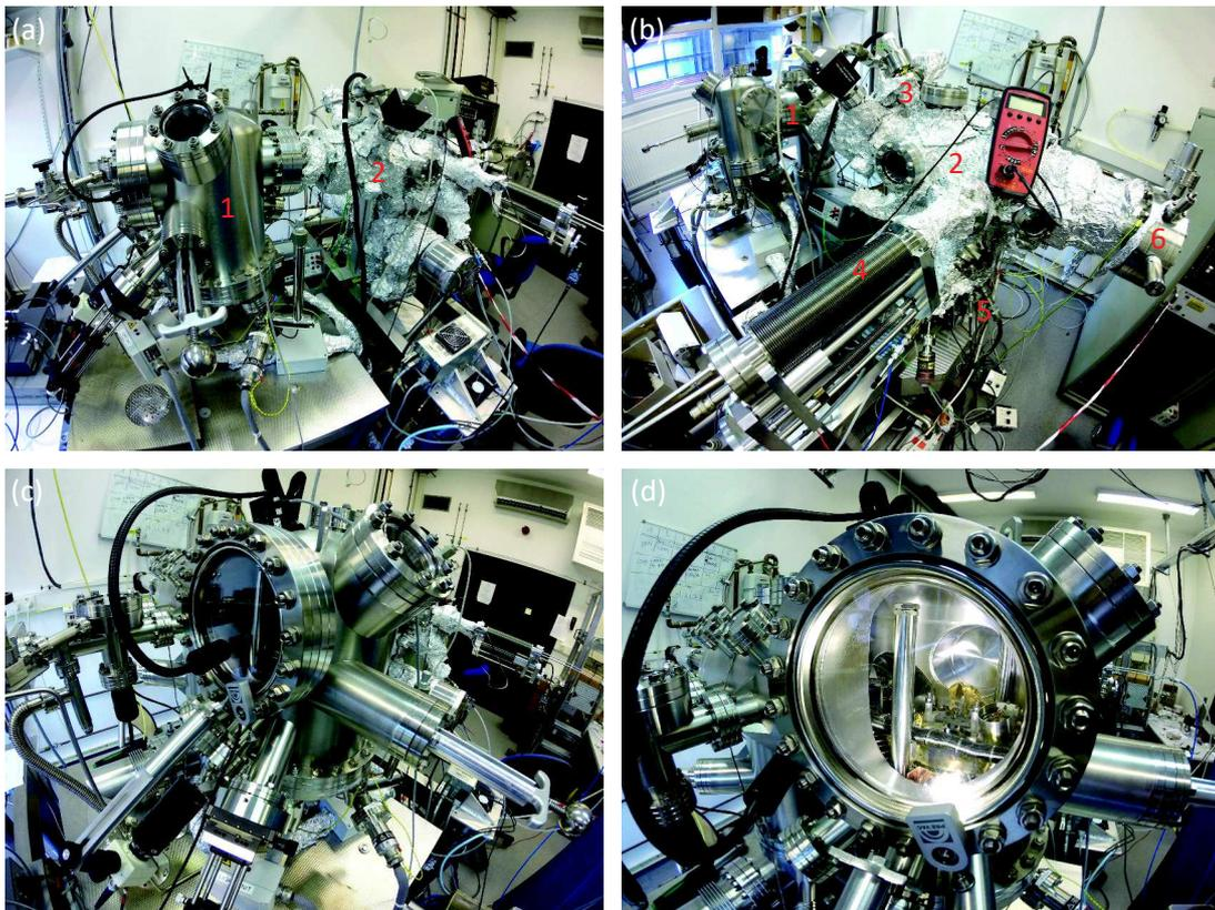
**Figure 3.1: Multi-Probe system.** (a)-(b) The Multi-Probe system consisting of (1) scanning probe microscopy chamber, and (2) preparation chamber. (c)-(d) The Omicron UHV variable temperature AFM XA station. 3 -  $\text{Ar}^+$ -ion sputtering gun, 4 - quartz microbalance, 5 - Tectra double e-beam evaporator, 6 - AES and LEED analyzer.
