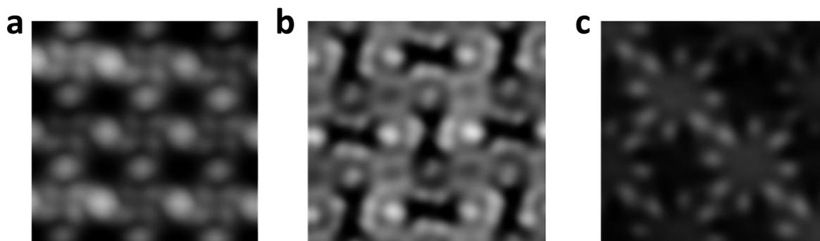
Fig. 4.8 From left to right, constant current topography of a  $\text{TbPc}_2$  film adsorbed on Cu (111), Ag (111) and Au (111) respectively. Each image contains nine molecules where four full molecules are identified at the center. All substrates were represented with a grey-scale to highlight the difference.
