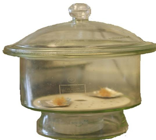
*Figure 54: Water absorption measurement*
