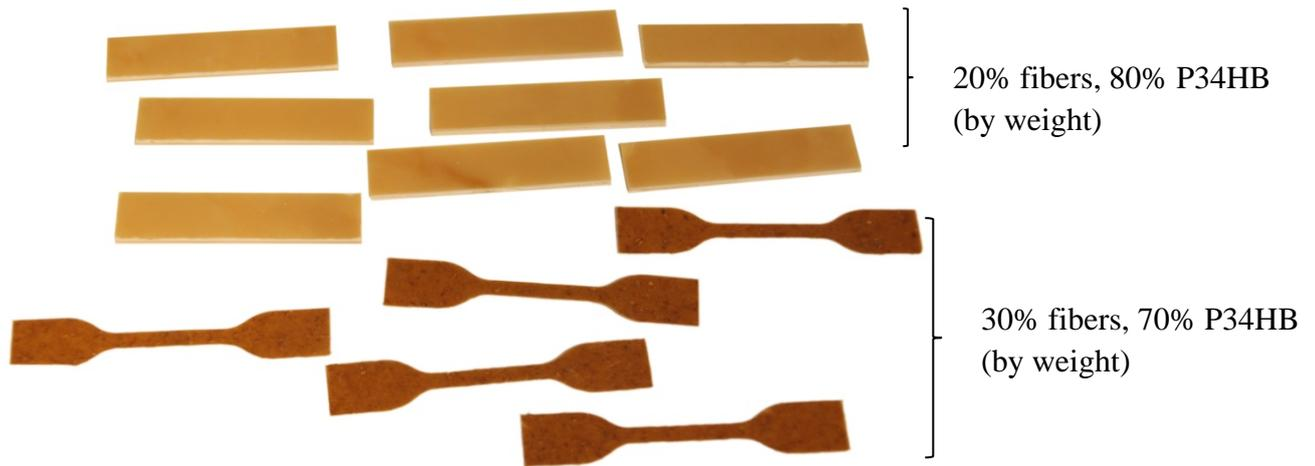
*Figure 71: Samples from the obtained polymer composite plates*
