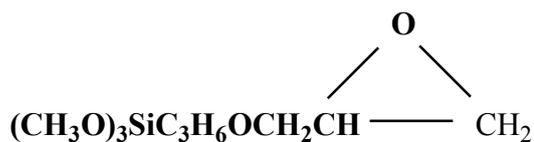
Figure 48: Structure of GF 80
