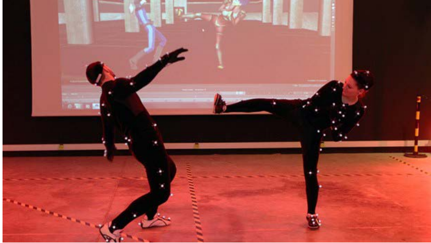
FIGURE 2.1 – Marker-based motion capture (source: 3IS - Institut International de l’Image et du Son)
