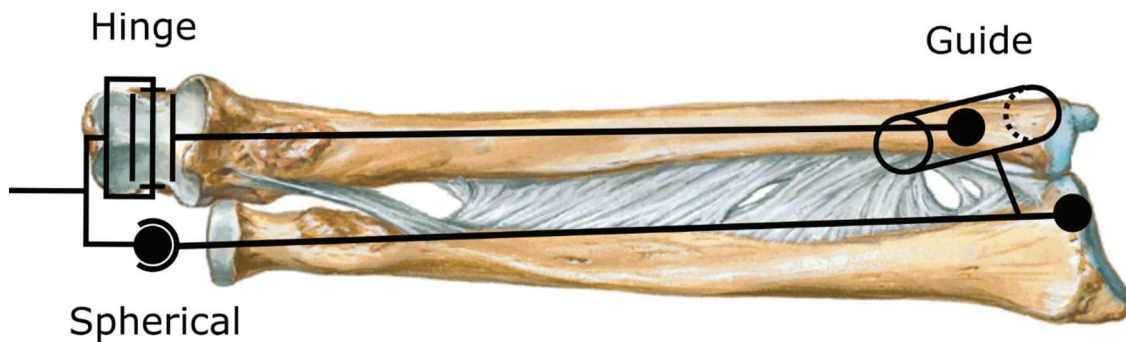
Figure 20 : Pennestri's model (adapted from Netter (2006))
