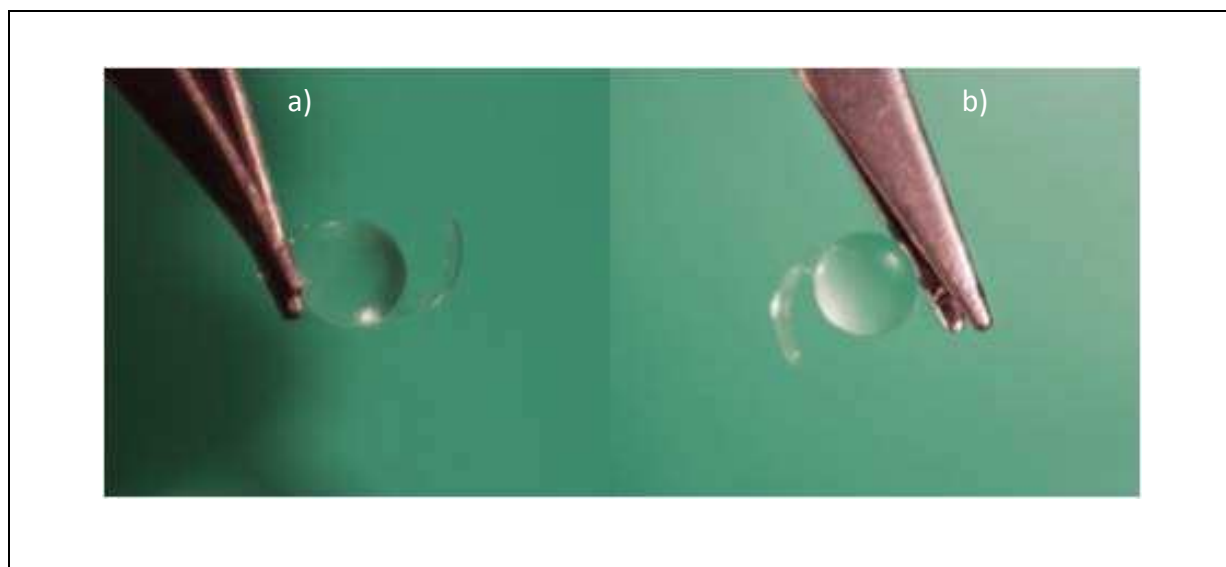
Figure III. 20 Influence of the pressurization flow rate (0.25 kg.h -1 ) on the visual aspect of IOLs treated with scCO 2 at 20 MPa: a) in the presence of ethanol (5 %mol), b) in the absence of co-solvent.
