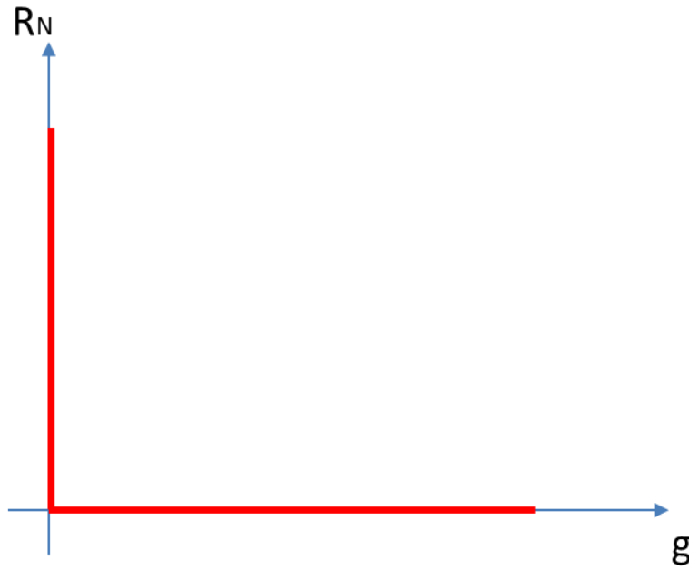
Figure 26: Graphic representation of the frictionless contact law. In the local referential the compression force R_N is defined positive.
