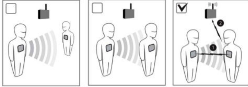
Figure 1.2: Schematic illustration of the RFID sensor system. RFID badges are worn by the participants to the study. A contact is detected when two individuals are close enough and facing each other. The signal of the contact is then sent to an antenna.
