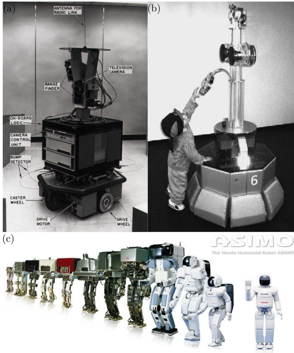
Figure 1.1: (a) The Shakey robot created by the Artificial Intelligence Center at the Stanford Research Institute. Adapted from [3]. (b) The Robox cobot (collaborative robot) developed by BlueBotics SA and EPFL Autonomous Systems Lab and shown at the Swiss National Exhibition Expo 2002. Adapted from [4]. (c) The Asimo robot created by Honda with its ancestors.
