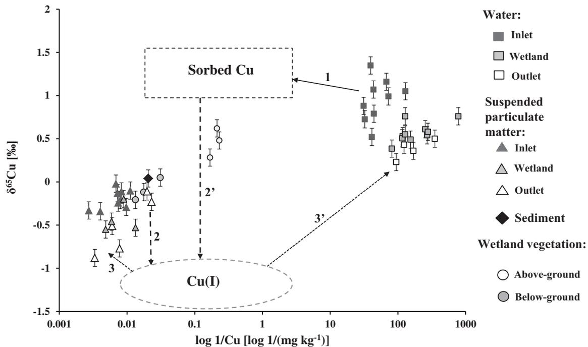
**Figure IV-4:** Conceptual model of Cu transport and transformation in the wetland. **1)** Sorption of dissolved Cu to the sediment and enrichment in  $^{65}\text{Cu}$  of the sorbate, **2+2')** Reduction of Cu(II) within the sediment of the sorbed (2') and retained particulate (2) Cu forming an isotopically lighter Cu(I) pool, **3+3')** Contribution of the isotopically lighter Cu(I) to Cu associated with the dissolved phase (3') and SPM (3) outflowing the wetland under high-flow conditions.
