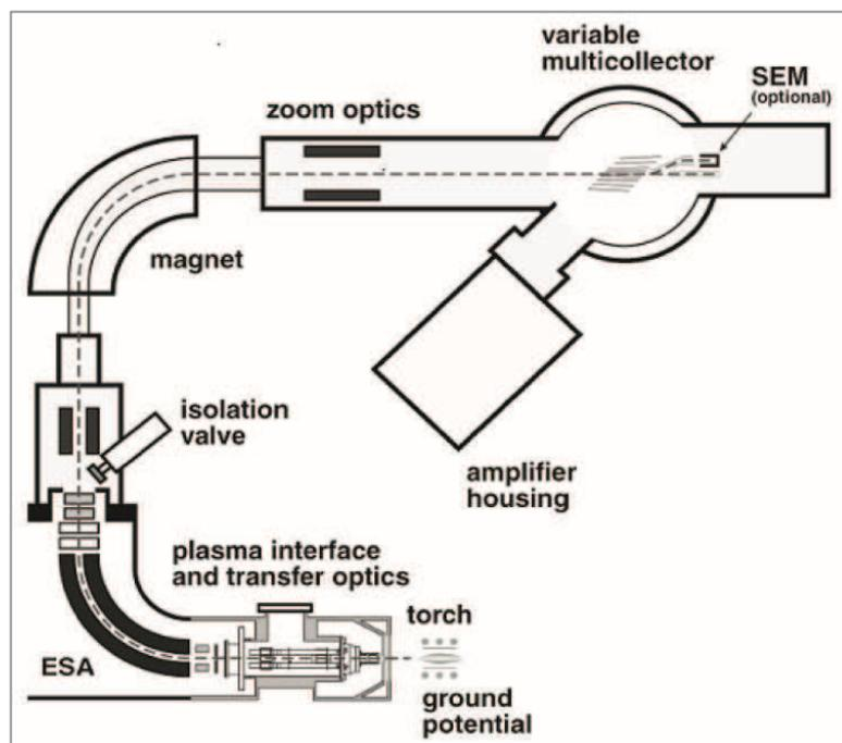
**Figure II-8:** The schematic image of a double focusing multicollector ICP-MS (ESA: Electric sector analyzer (Figure from Goldstein and Stirling, 2003)).<sup>36</sup>
