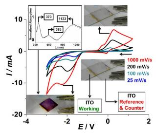
Figure 33. Variable scan cyclic voltammograms of a solution of HV<sup>12+</sup>•12Cl, in 1 M NaCl H<sub>2</sub>O, sandwiched between two ITO coated glass slides (4-8 Ohms, 1500–2000 Å nominal coating thickness). One of the ITO slides is used as a working electrode while the other is used as counter and reference electrode. A colour change (colourless to purple) is observed upon reduction. Inset: UV-Vis-NIR spectrum of the device switched at −2 V.
