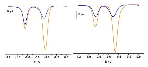
**Figure 54.** Square Wave voltammograms of **C23**<sup>4+</sup>, [**C23**<sup>4+</sup>] = 0.05 mM (left) and **C24**<sup>4+</sup>, [**C24**<sup>4+</sup>] = 0.05 mM (right) in the absence (orange line) and the presence of **CB[7]** (blue line, respectively 3 and 4 equivalents of **CB[7]**). All voltammograms were recorded in Argon-purged phosphate buffer solutions (pH 7) at 298 K (*E versus* Ag/AgCl).
