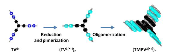
**Figure 39.** Schematic representation of the pimerization and oligomerization of **TV**<sup>6+</sup> upon reduction with sodium dithionite.
