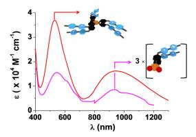
**Figure 31.** Electronic UV-Vis-NIR absorption spectra of  $HV_D^{6(++)}$  compared to that of  $(BV^{++})_2$  in water. Solvent: water buffered at pH 7.0 with 0.1 M Na<sub>2</sub>HPO<sub>4</sub>/NaH<sub>2</sub>PO<sub>4</sub>. *T* = 25.0(1) °C.
