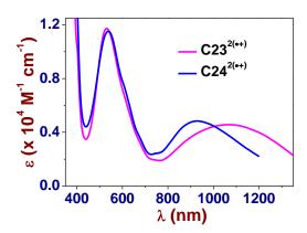
**Figure 51.** Electronic UV-Vis.-NIR absorption spectra of  $C23^{2(+)}$  and  $C24^{2(+)}$  in water. Solvent: water buffered at pH 7.0 with 0.1 M Na<sub>2</sub>HPO<sub>4</sub>/NaH<sub>2</sub>PO<sub>4</sub>. *T* = 25.0(1) °C.
