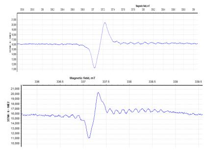
**Figure 41.** EPR spectra measured for (top) **MC3**<sup>++</sup> and (bottom) **MC3**<sup>++</sup> and 4 equivalents of **CB[7]**. Solvent: water.
