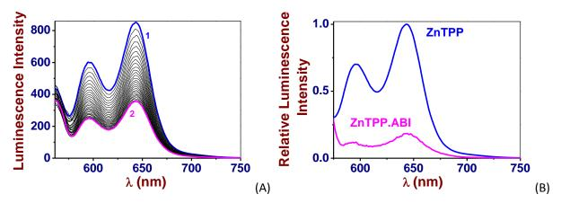
**Figure 8.** (A) Spectrofluorimetric titration of Zn**TPP** receptor by azo-benzene-imidazole (**ABI**).  $\lambda_{exc} = 560 \text{ nm}$ ; exc. and em. slits 15/20 nm; (1) [Zn**TPP**]<sub>tot</sub> = 3.40 × 10<sup>-5</sup> M; (2) [**ABI**]<sub>0</sub>/[Zn**TPP**]<sub>tot</sub> = 63.5. (B) Relative reconstituted emission spectra of Zn**TPP** and its pentacoordinated complex with **ABI**.
