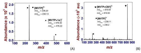
**Figure 12.** (A) ESI mass spectrum of free  $MVTP^{2+}$ .  $[MVTP^{2+}]_0 = 4 \times 10^{-6}$  M. Solvent: H<sub>2</sub>O; positive mode. V<sub>c</sub> = 100 V. • =  $[MVTP]^{2+}$ ,  $m/z_{exp} = 238.20$ ,  $m/z_{theo} = 238.11$ . • =  $[MVTP+1e^{-}]^{+}$ ,  $m/z_{exp} = 476.30$ ,  $m/z_{theo} = 476.22$ .
