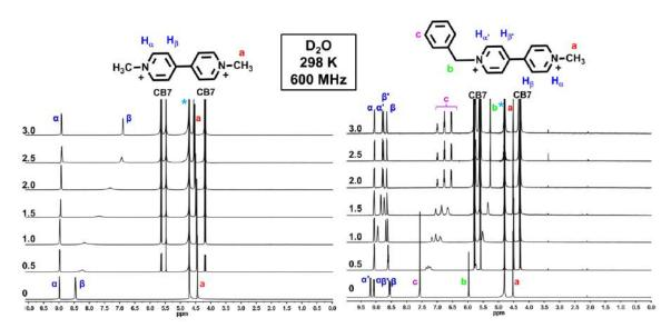
**Figure 11.** Full <sup>1</sup>H NMR spectra (600 MHz, D<sub>2</sub>O, 298 K) of **MV**<sup>2+</sup> (left) and **BMV**<sup>2+</sup> (right) in the presence of increasing amounts of **CB[7]**. \*Solvent peak.
