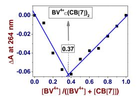
**Figure 8.** Job plot ( $\Delta A$  at 264 nm) upon mixing **BV**<sup>4+</sup> and **CB[7]**. ([**BV**<sup>4+</sup>]<sub>0</sub> + [**CB[7]**]<sub>0</sub>) = 5.80 × 10<sup>-5</sup> M; Solvent: water pH 7.0 (0.1 M Na<sub>2</sub>HPO<sub>4</sub>/NaH<sub>2</sub>PO<sub>4</sub>); *I* = 1 cm; *T* = 25.0(1) °C.
