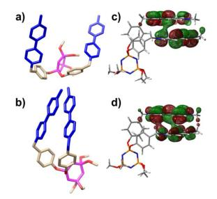
**Figure 32.** Optimized geometries of the **BV**<sup>4+</sup> a) and **BV**<sup>2(•+)</sup> b) models, and representations of SOMO c) and SOMO-1 d) in **BV**<sup>2(•+)</sup> computed in aqueous solution at the M06/6-31G(d,p) level.
