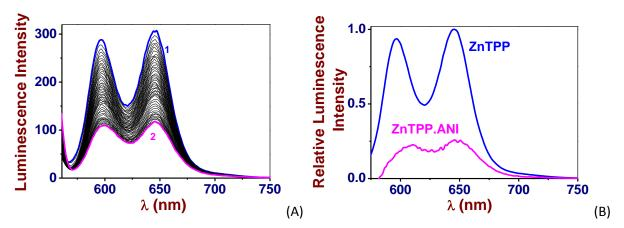
**Figure 9.** (A) Spectrofluorimetric titration of Zn**TPP** receptor by azo-naphthyl-imidazole (**ANI**).  $\lambda_{\text{exc}} = 555 \text{ nm}$ ; exc. and em. slits 10/10 nm; (1) [Zn**TPP**]<sub>tot</sub> = 7.10 × 10<sup>-6</sup> M; (2) [**ANI**]<sub>0</sub>/[Zn**TPP**]<sub>tot</sub> = 93. (B) Relative reconstituted emission spectra of Zn**TPP** and its pentacoordinated complex with **ANI**.
