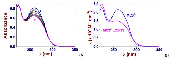
Figure 17. A) UV-Vis. absorption titration of  $MC3^{2+}$  by CB[7]. B) Electronic spectra of  $MC3^{2+}$  and its inclusion complex with CB[7] ( $MC3^{2+} \square CB[7]$ ). Solvent: water pH 7.0 (0.1 M  $Na_2H_2PO_4/NaH_2PO_4$ ).[ $MC3^{2+}$ ]<sub>0</sub> = 3.8 × 10<sup>-5</sup> M; (1) [CB[7]]<sub>0</sub>/[ $MC3^{2+}$ ]<sub>0</sub> = 0; (2) [CB[7]]<sub>0</sub>/[ $MC3^{2+}$ ]<sub>0</sub> = 2.9; *I* = 1 cm; *T* = 25.0(1)°C. The absorption spectra are not corrected from dilution effects.
