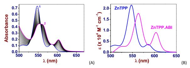
Figure 2. (A) UV-Vis. absorption spectrophotometric titration of ZnTPP by azo-benzene-imidazole (ABI). Solvent: 1,2-dichloroethane; T = 25.0(2) °C; / = 1 cm. (1) [ZnTPP]<sub>0</sub> = 3.4 × 10<sup>-5</sup> M; (2) [ABI]<sub>0</sub>/[ZnTPP]<sub>0</sub> = 131. (B) Electronic spectra of ZnTPP and its pentacoordinated species with ABI.
