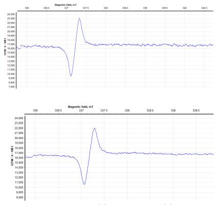
**Figure 44.** EPR spectra measured for (top) **C24**<sup>2(++)</sup> and (bottom) **C24**<sup>2(++)</sup> and 4 equivalents of **CB[7]**. Solvent: water.
