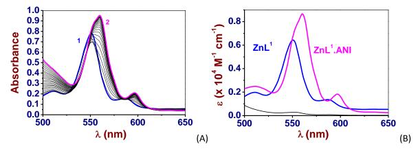
Figure 6. (A) UV-Vis. absorption spectrophotometric titration of ZnL<sup>1</sup> by azo-naphthyl-imidazole (ANI). Solvent: 1,2-dichloroethane; T = 25.0(2) °C; I = 1 cm. (1) [ZnL<sup>1</sup>]<sub>0</sub> = 4.80 × 10<sup>-6</sup> M; (2) [ANI]<sub>0</sub>/[ZnL<sup>1</sup>]<sub>0</sub> = 3.97. (B) Electronic spectra of the ZnL<sup>1</sup> receptor and its pentacoordinated species with ANI.
