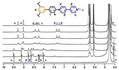
**Figure 19.** Full <sup>1</sup>H NMR spectra (600 MHz,  $D_2O$ , 298 K) of **TV**<sup>6+</sup> in the presence of increasing amounts of **CB[7]**.
