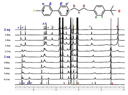
Figure 28. <sup>1</sup>H NMR spectra (600 MHz,  $D_2O$ , 298 K) of MC3<sup>2+</sup> (3.5 mM) in the presence of increasing amounts of CB[7].
