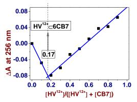
**Figure 10.** Job plot ( $\Delta A$  at 256 nm) upon mixing HV<sup>12+</sup> and CB[7]. ([HV<sup>12+</sup>]<sub>0</sub> + [CB[7]]<sub>0</sub>) = 4 × 10<sup>-5</sup> M; Solvent: water pH 7.0 (0.1 M Na<sub>2</sub>HPO<sub>4</sub>/NaH<sub>2</sub>PO<sub>4</sub>); *I* = 5 mm; *T* = 25.0(1) °C
