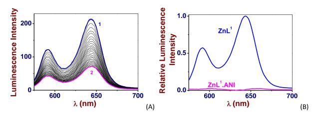
**Figure 11.** (A) Spectrofluorimetric titration of  $ZnL^1$  receptor by azo-naphthyl-imidazole (ANI).  $\lambda_{exc} = 555 \text{ nm}$ ; exc. and em. slits 10/10 nm; (1)  $[ZnL^1]_{tot} = 1.20 \times 10^{-5} \text{ M}$ ; (2)  $[ANI]_0/[ZnL^1]_{tot} = 58.3$ . (B) Relative reconstituted emission spectra of  $ZnL^1$  and its pentacoordinated complex with ANI.
