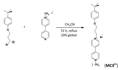
**Figure 9.** Synthesis of 1-(3-4-(*tert*-butyl) phenoxy)propyl)-1-methyl-[4,4'-bipyridin]-1,1'-diium bromide iodide (**MC3**<sup>2+</sup>)
