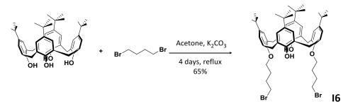
Figure 15. Synthesis of 1,3-bis(4-bromobutoxy)-p-tert-butyl-calix[4]arene (I6).
