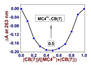
**Figure 20.** Job plot (ΔA at 263 nm) upon mixing **MC4**<sup>2+</sup> with **CB[7]** at pH 7.([**MC4**<sup>2+</sup>]<sub>0</sub> + [**CB[7]**]<sub>0</sub>) = 7.0 × 10<sup>-5</sup> M; Solvent :water pH 7.0 (0.1 M Na<sub>2</sub>H<sub>2</sub>PO<sub>4</sub>/NaH<sub>2</sub>PO<sub>4</sub>); I = 1 cm;  $T = 25.0(1)^{\circ}$ C.
