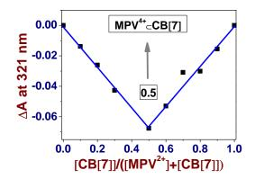
**Figure 3.** Job plot (ΔA at 321 nm) upon mixing **MPV**<sup>2+</sup> with **CB[7]** at pH 7.([**MPV**<sup>2+</sup>]<sub>0</sub> + [**CB[7]**]<sub>0</sub>) =  $9.5 \times 10^{-5}$  M; Solvent :water pH 7.0 (0.1 M Na<sub>2</sub>H<sub>2</sub>PO<sub>4</sub>/NaH<sub>2</sub>PO<sub>4</sub>); *I* = 1 cm; *T* = 25.0(1)°C.
