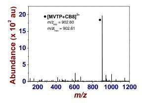
**Figure 13.** ESI mass spectrum of inclusion complexes of  $MVTP^{2+}$  with CB[8].  $[MVTP^{2+}] = 1 \times 10^{-4}$  M;  $[CB[7]] = 1 \times 10^{-4}$  M. Solvent: H<sub>2</sub>O; positive mode. V<sub>c</sub> = 120 V. • =  $[MVTP+CB[8]]^{2+}$ ,  $m/z_{exp} = 902.60$ ,  $m/z_{theo} = 902.61$ . The ESI-MS spectra were limited to the areas of interest. No peaks were detected in the excluded m/z regions.
