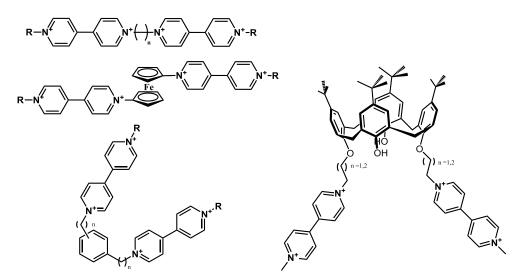
**Figure 1.** Chemical structures of *bis*-viologen compounds that favour intramolecular dimerization of their corresponding radical cations.
