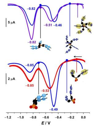
**Figure 39.** Square Wave voltammograms of  $HV^{12+}$ ,  $[HV^{12+}] = 0.024$  mM (top) and  $BV^{4+}$ ,  $[BV^{4+}] = 0.065$  mM (bottom) in the absence and the presence of **CB[7]** (respectively 18 and 4 equivalents of **CB[7]**). All voltammograms were recorded in Argon-purged phosphate buffer solutions (pH 7) at 298 K with 0.1 M TBACI. *E versus* Ag/AgCI.
