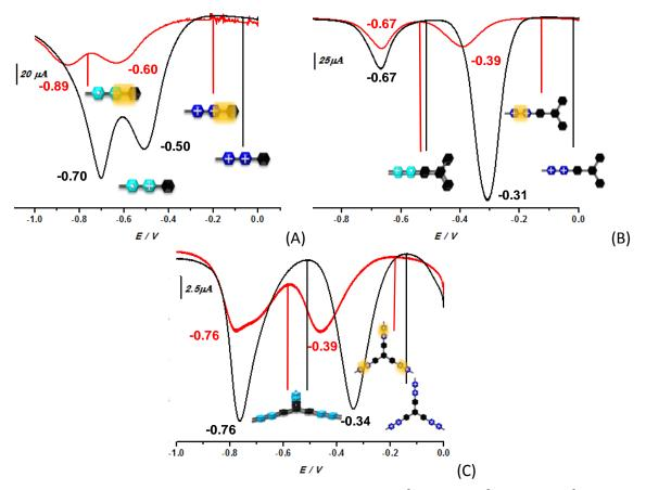
**Figure 30.** Square wave voltammograms (SWVs) of (A) **MPV**<sup>2+</sup>, (B) **MVTP**<sup>2+</sup>, and (C) **TV**<sup>6+</sup> in the absence and the presence of **CB[7]** (respectively 2, 4, and 8 equivalents of **CB[7]**). All voltammograms were recorded in Argon-purged phosphate buffer solutions (pH 7) at 298 K. The scan rate was set at 1000 mVs<sup>-1</sup>. *E versus* Ag/AgCl.
