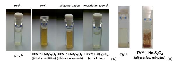
**Figure 25.** Solutions of (A)  $DPV^{2+}$  and (B)  $TV^{6+}$  before and after addition of Na<sub>2</sub>S<sub>2</sub>O<sub>4</sub> showing the formation of an insoluble aggregate that re-dissolves upon re-oxidation under open air conditions.
