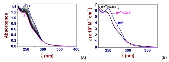
Figure 7. (A) UV-Vis. Absorption titration of  $BV^{4+}$  by CB[7]. (B) Electronic spectra of  $BV^{4+}$  and of its inclusion complexes with CB[7] ( $BV^{4+} \subset CB[7]$  and  $BV^{4+} \subset (CB[7])_2$ ). Solvent: water pH 7.0 (0.1 M Na<sub>2</sub>HPO<sub>4</sub>/NaH<sub>2</sub>PO<sub>4</sub>). [ $BV^{4+}$ ]<sub>0</sub> = 2.32 × 10<sup>-5</sup> M; (1) [CB[7]]<sub>0</sub>/[ $BV^{4+}$ ]<sub>0</sub> = 0; (2) [CB[7]]<sub>0</sub>/[ $BV^{4+}$ ]<sub>0</sub> = 4.66; *l* = 1 cm; *T* = 25.0(1) °C.
