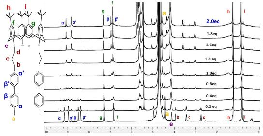
Figure 30. <sup>1</sup>H NMR (600 MHz,  $D_2O$ , 298 K) titration of C23 with an excess of CB[7].
