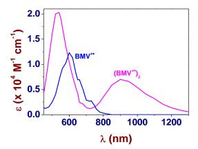
**Figure 17.** UV-Vis.-NIR electronic spectra of **BMV**<sup>++</sup> under its monomeric or dimeric form. Solvent: Water pH 7.0 (0.1 M Na<sub>2</sub>HPO<sub>4</sub>/NaH<sub>2</sub>PO<sub>4</sub>); T = 25.0(1) °C.
