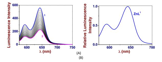
**Figure 10.** (A) Spectrofluorimetric titration of  $ZnL^{1}$  receptor by azo-benzene-imidazole (**ABI**).  $\lambda_{exc} = 554$  nm; exc. and em. slits 15/20 nm; (1)  $[ZnL^{1}]_{tot} = 4.7 \times 10^{-6}$  M; (2)  $[ABI]_{0}/[ZnL^{1}]_{0} = 9.66$ . (B) Relative reconstituted emission spectra of  $ZnL^{1}$  and its pentacoordinated complex with **ABI**.
