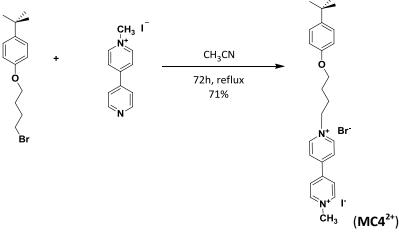
**Figure 11.** Synthesis of 1-(4-(4-(*tert*-butyl)phenoxy)butyl)-1'-methyl-[4,4'-bipyridin]-1,1'-diium bromide iodide (**MC4**<sup>2+</sup>)
