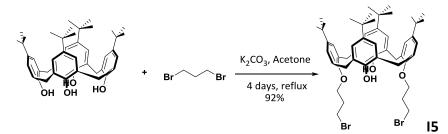
Figure 13. Synthesis of 1,3-bis(3-bromopropoxy)-p-tert-butyl-calix[4]arene (I5)
