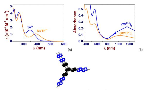
**Figure 38.** (A) UV-Vis. electronic absorption spectra of **TV**<sup>6+</sup> and **MVTP**<sup>2+</sup> and (B) UV-Vis.-NIR electronic absorption spectrum of a diluted **TV**<sup>3(++)</sup> solution. Solvent: Water pH 7.0 (0.1 M Na<sub>2</sub>HPO<sub>4</sub>/NaH<sub>2</sub>PO<sub>4</sub>); **TV**<sup>3(++)</sup> was generated from **TV**<sup>6+</sup> using freshly prepared sodium dithionite solution at *ca*. 10<sup>-2</sup> M under O<sub>2</sub> free conditions.
