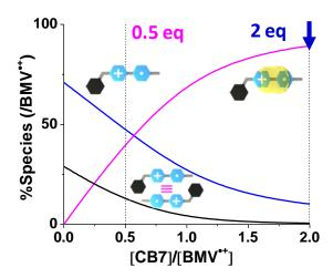
**Figure 38.** Distribution diagrams of the **BMV**<sup>•+</sup>/**CB[7]** system. Solvent: water buffered at pH 7.0 with 0.1 M Na<sub>2</sub>HPO<sub>4</sub>/NaH<sub>2</sub>PO<sub>4</sub>; T = 25.0(1) °C.
