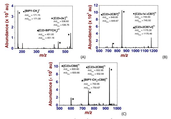
Figure 26. (A) ESI mass spectrum of free C23<sup>4+</sup>. [C23<sup>4+</sup>]<sub>0</sub> =  $4.9 \times 10^{-5}$  M. Solvent: H<sub>2</sub>O; positive mode. V<sub>c</sub> = 150 V. ● = [BIPY-CH<sub>3</sub>]<sup>+</sup>,  $m/z_{exp}$  = 171.15,  $m/z_{theo}$  = 171.09. ♥ = [C23<sup>4+</sup>-BIPY-CH<sub>3</sub>]<sup>2+</sup>,  $m/z_{exp}$  = 451.00,  $m/z_{theo}$  = 451.18. ♦ = [C23<sup>4+</sup>+2e<sup>-</sup>]<sup>2+</sup>,  $m/z_{exp}$  = 536.60,  $m/z_{theo}$  = 536.76.
