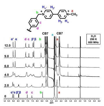
**Figure 13.** <sup>1</sup>H NMR partial spectra (600 MHz, 1.0 M NaCl/D<sub>2</sub>O) of **HV**<sup>12+</sup> in the presence of 0 equiv, 1 equiv, 3 equiv, 7 equiv, 9 equiv, and 12 equiv of **CB[7]**.
