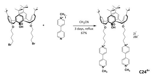
**Figure 16**. Synthesis of 1,3-*bis*(3-(1'-methyl-[4,4'-bipyridin]-1,1'-diium)butoxy)-*p*-*tert*-butyl-calix[4]arene dibromide diiodide (**C24**<sup>4+</sup>)
