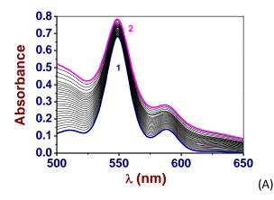
**Figure 4.** UV-Vis. absorption spectrophotometric titration of Zn**TPP** by azo-phenanthryl-imidazole (**API**). Solvent: 1,2-dichloroethane; T = 25.0(2) °C; I = 1 cm. (1) [**ZnTPP**]<sub>0</sub> =  $3.4 \times 10^{-5}$  M; (2) [**API**]<sub>0</sub>/[Zn**TPP**]<sub>0</sub> = 1015.7.
