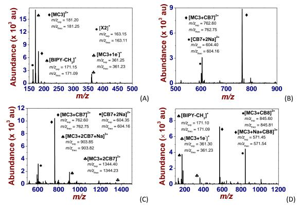
Figure 24. (A) ESI mass spectrum of free  $MC3^{2+}$ .  $[MC3^{2+}]_0 = 5.5 \times 10^{-5}$  M. Solvent: H<sub>2</sub>O; positive mode.  $V_c = 100 \text{ V}. \bullet = [X2]^+, m/z_{exp} = 163.15, m/z_{theo} = 163.11$  with  $X2 = {}^+CH_2-O-C_6H_4-C(CH_3)_3. \bullet = [BIPY-CH_3]^+, m/z_{exp} = 171.15, m/z_{theo} = 171.09. \bullet = [MC3]^{2+}, m/z_{exp} = 181.20, m/z_{theo} = 181.25. \bullet = [MC3+1e^-]^+, m/z_{exp} = 361.25, m/z_{theo} = 361.23.$
