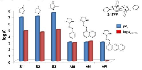
**Figure 13.** Schematic representation of the log  $K_{ZnTPP.S}$  values as a function of the p $K_a$  sequence (simulated with ChemAxon pK<sub>a</sub> calculator) which demonstrate the steric effects induced by the bulkiness of the azo-chromophore substituents.
