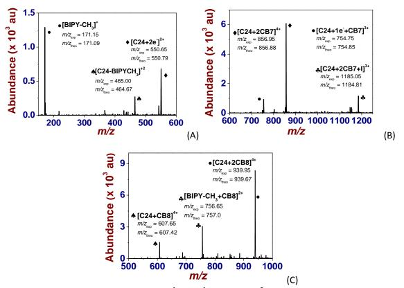
Figure 27. (A) ESI mass spectrum of free C24<sup>4+</sup>. [C24<sup>4+</sup>]<sub>0</sub> = 4.7 × 10<sup>-5</sup> M. Solvent: H<sub>2</sub>O; positive mode. V<sub>c</sub> = 150 V. • = [BIPY-CH<sub>3</sub>]<sup>+</sup>,  $m/z_{exp}$  = 171.15,  $m/z_{theo}$  = 171.09. ♥ = [C24<sup>4+</sup>-BIPY-CH<sub>3</sub>]<sup>2+</sup>,  $m/z_{exp}$  = 465.00,  $m/z_{theo}$  = 464.67. ♦ = [C24<sup>4+</sup>+2e<sup>-</sup>]<sup>2+</sup>,  $m/z_{exp}$  = 550.65,  $m/z_{theo}$  = 550.79.
