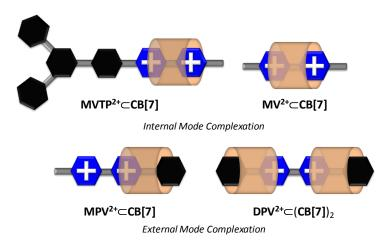
**Figure 35.** Schematic representation of the internal (**MV**<sup>2+</sup> and **MVTP**<sup>2+</sup>, the hydrophobic cavity of **CB[7]** mainly resides on the bipyridinium group) and external (**MPV**<sup>2+</sup> and **DPV**<sup>2+</sup>, the hydrophobic cavity of **CB[7]** mainly resides on the terminal phenyl group).
