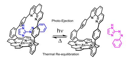
**Figure 18.** Schematic representation of the principle of photo-ejection of the azo-arylimidazole from the pentacoordinated species with ZnL<sup>1</sup>.
