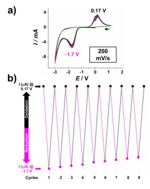
Figure 34. a) Reversible Redox cycles of the ITO device and b) change in the current intensity as a fuction of reduction/oxidation processes.
