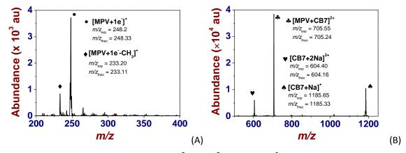
**Figure 10.** (A) ESI mass spectrum of free  $MPV^{2+}$ .  $[MPV^{2+}]_0 = 5.5 \times 10^{-5}$  M. Solvent: H<sub>2</sub>O; positive mode. V<sub>c</sub> = 100 V. • =  $[MPV+1e^{-}]^+$ ,  $m/z_{exp} = 248.20$ ,  $m/z_{theo} = 248.33$ . • =  $[MPV+1e^{-}-CH_3]^+$ ,  $m/z_{exp} = 233.20$ ,  $m/z_{theo} = 233.11$ .
