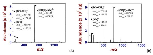
**Figure 14.** ESI mass spectra of the  $MV^{2^+}$  complex formed with (A) **CB[7]** and (B) **CB[8]**. (A)  $[MV^{2^+}]_0 = 55 \mu$ M with 1 equivalent of **CB[7]**; V<sub>c</sub> = 300 V. (B)  $[MV^{2^+}]_0 = 100 \mu$ M with 1 equivalent of **CB[8]**. V<sub>c</sub> = 150 V. Solvent: water; positive mode.
