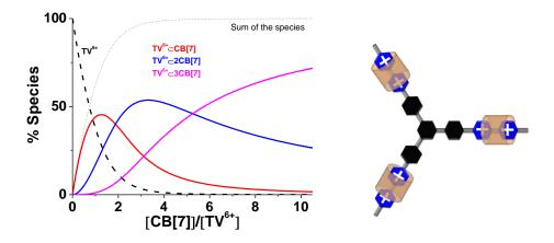
**Figure 36.** Distribution curves of the inclusion complexes which might be formed when  $TV^{6^+}$  is mixed with **CB[7]**. The dash line corresponds to the sum of all the species. Distribution diagram calculated using log  $K_{TV6+CCB[7]} = \log K_{MVTP2+CCB[7]} = 4.8$  and a statistical binding process. Solvent: water pH 7.0 (0.1 M Na<sub>2</sub>HPO<sub>4</sub>/NaH<sub>2</sub>PO<sub>4</sub>); [TV<sup>6+</sup>] = 10<sup>-4</sup> M; T = 25.0(1) °C.
