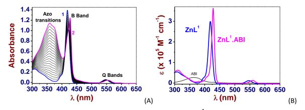
**Figure 5.** (A) UV-Vis. absorption spectrophotometric titration of  $\text{ZnL}^1$  by azo-benzene-imidazole (**ABI**). Solvent: 1,2-dichloroethane; T = 25.0(2) °C; I = 1 cm. (1)  $[\text{ZnL}^1]_0 = 4.69 \times 10^{-6}$  M; (2)  $[\text{ABI}]_0/[\text{ZnL}^1]_0 = 35.18$ . (B) Electronic spectra of the  $\text{ZnL}^1$  receptor and its pentacoordinated species with **ABI**.
