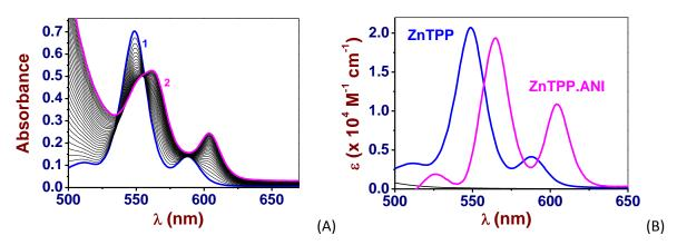
Figure 3. (A) UV-Vis. absorption spectrophotometric titration of ZnTPP by azo-naphthyl-imidazole (ANI). Solvent: 1,2-dichloroethane; T = 25.0(2) °C; I = 1 cm. (1) [ZnTPP]<sub>0</sub> = 3.4 × 10<sup>-5</sup> M; (2) [ANI]<sub>0</sub>/[ZnTPP]<sub>0</sub> = 82. (B) Electronic spectra of ZnTPP and its pentacoordinated species with ANI.
