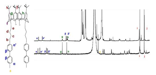
Figure 31. <sup>1</sup>H NMR spectra (600 MHz, D<sub>2</sub>O, 298 K) of C24 without and with and excess of CB[7].
