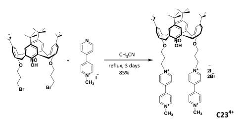
**Figure 14.** Synthesis of 1,3-*bis*(3-(1'-methyl-[4,4'-bipyridin]-1,1'-diium)propoxy)-*p*-tert-butyl-calix[4]arene dibromide diiodide (**C23**<sup>4+</sup>).
