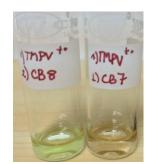
**Figure 34.** Solutions of **TV**<sup>3(•+)</sup> and **CB[8]** (no precipitation, green colour, left) and **TV**<sup>3(•+)</sup> and CB[7] (precipitation, reddish colour, right).
