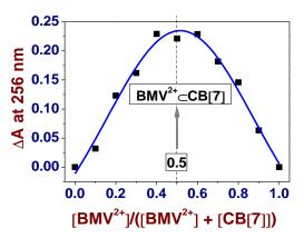
Figure 6. Job plot ( $\Delta A$  at 256 nm) upon mixing BMV<sup>2+</sup> and CB[7]. ([BMV<sup>2+</sup>]<sub>0</sub> + [CB[7]]<sub>0</sub>) = 10<sup>-4</sup> M; Solvent: water pH 7.0 (0.1 M Na<sub>2</sub>HPO<sub>4</sub>/NaH<sub>2</sub>PO<sub>4</sub>); *I* = 5 mm; *T* = 25.0(1) °C.
