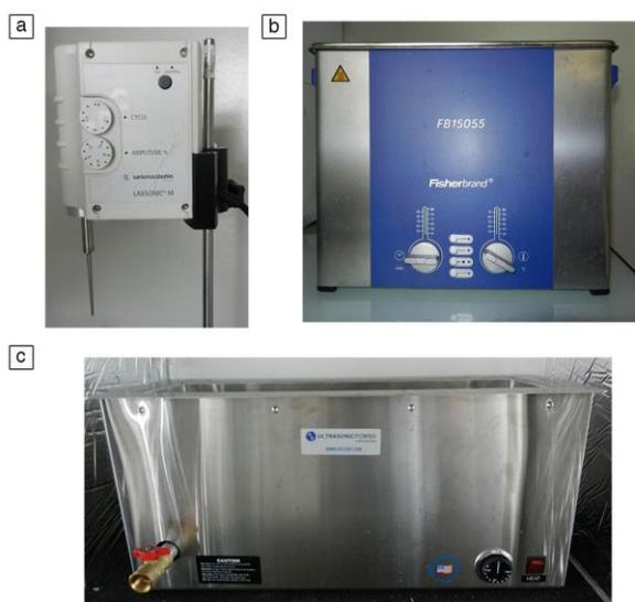
**Figure 4.3.** Photograph of the different setups used for graphite exfoliation: a) probe sonication, b) constant intensity bath sonication and c) advanced ultrasonic bath with frequency and intensity controller.
