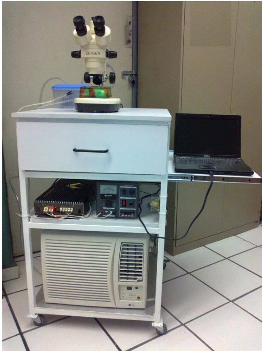
Figure 2.8 System currently used for stimulation of Entamoeba cell cultures
