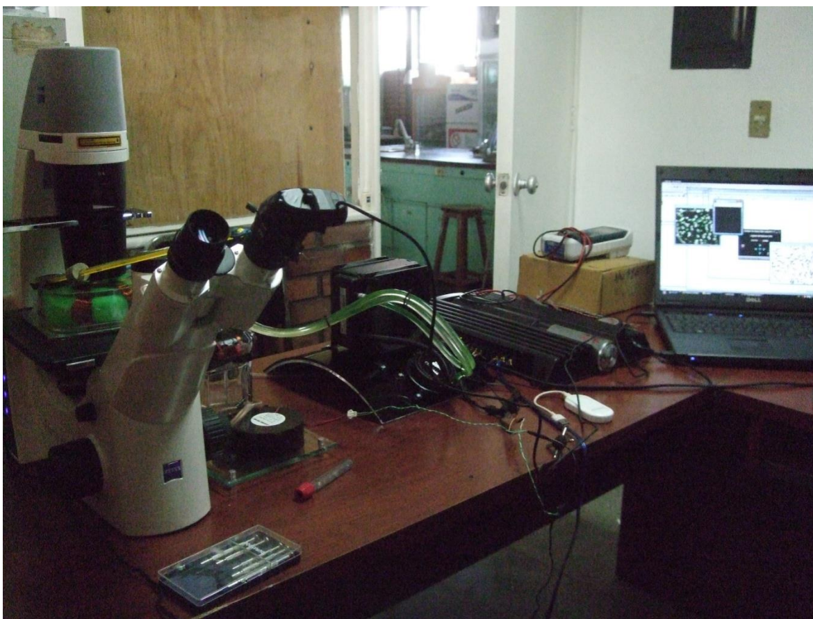
Figure 2.3: Magnetic field stimulation system to study the motility of Entamoeba cell cultures.
