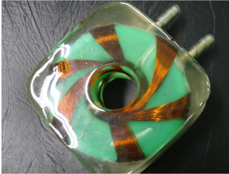
Figure 2.16. Copper winding's vortex type coil that generates the magnetic stimulation field.
