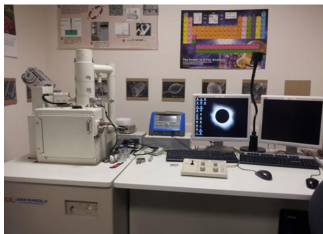
Figure.3.11. Set up of Scanning Electron Microscope
