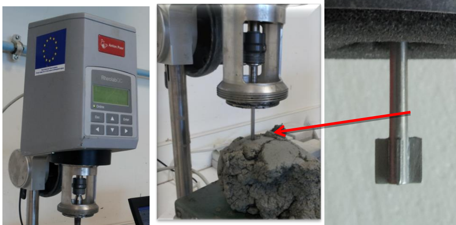
Figure 3.18. The Anton Paar Rheolab QC Rheometer
