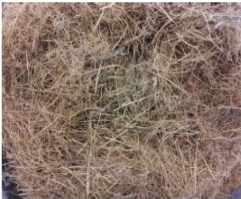
Figure. 4.1. Untreated coir fiber
