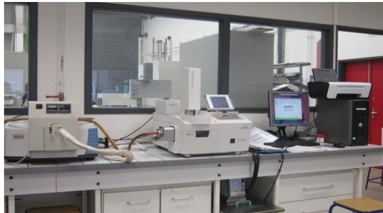
Figure.3.12. Thermogravimetric analyses device.
