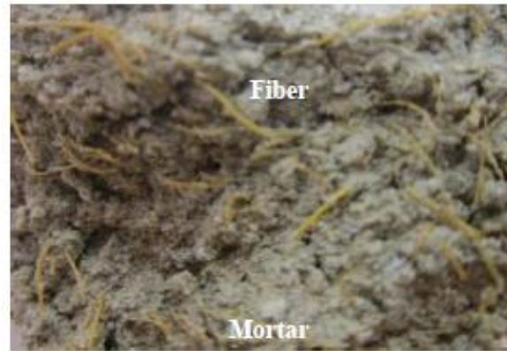
Figure. 5.14. Morphology of fiber-reinforced cementitious composites after mixing.
