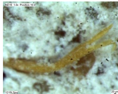
Figure 6.23. Micrograph composite after failure compression of static loading, for broken fiber.
