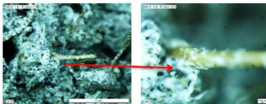
Figure. 5.18. Microstructure adhesion of fiber out of matrix
