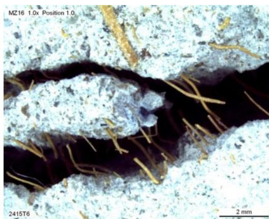
Figure 6.28. Micrograph of CFRCC composite, after the tensile failure of static loading.
