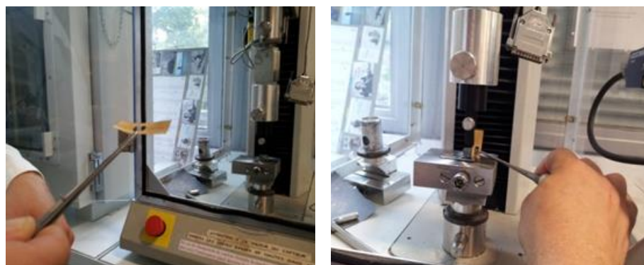
Figure.3.9. Preparation of specimen for the tensile test
