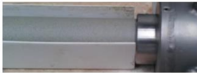
Figure. 5.13. Surface of the extruded cement mortar
