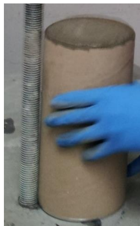
Figure.3.22. Vibrating of cylinder
