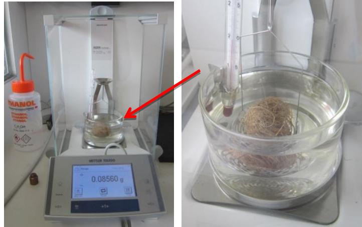
Figure 3.6. Density measurement using balances device.
